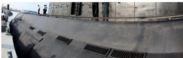
Figure 1. Free board, deck and free flooding space in submarine
