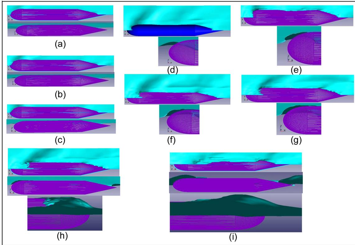
**Figure 8.** Up view and side view of free surface at  $h=0\text{m}$ : (a)  $F_n=0.2$  ( $v=1.4\text{m/s}$ ), (b)  $F_n=0.25$  ( $v=1.75\text{ m/s}$ ), (c)  $F_n=0.29$  ( $v=2.03\text{ m/s}$ ), (d)  $F_n=0.33$  ( $v=2.31\text{ m/s}$ ), (e)  $F_n=0.35$  ( $v=2.45\text{ m/s}$ ), (f)  $F_n=0.38$  ( $v=2.66\text{ m/s}$ ), (g)  $F_n=0.42$  ( $v=2.94\text{ m/s}$ ), (h)  $F_n=0.46$  ( $v=3.22\text{ m/s}$ ) and (i)  $F_n=0.5$  ( $v=3.5\text{ m/s}$ ).
