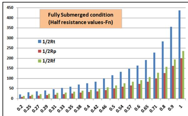
**Figure 9.** Resistance versus Froude numbers in fully submerged condition.
