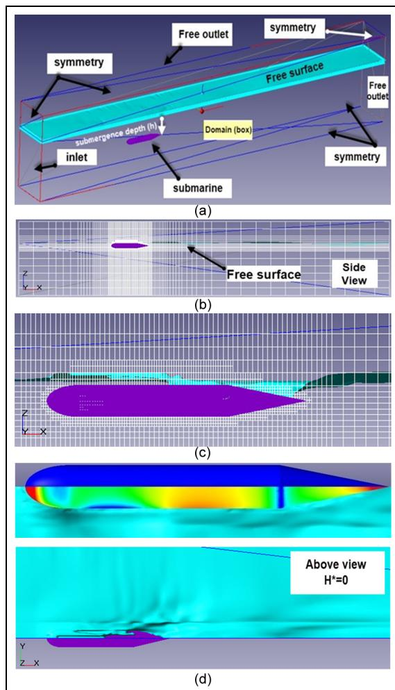
**Figure 6.** (a) Domain and structured grid, (b) tiny cell around free surface, (c) very tiny cells near the wall for boundary layer modeling and keeping  $y^+$  about 30 and (d) half modeling because of axis-symmetry and free surface variations.
