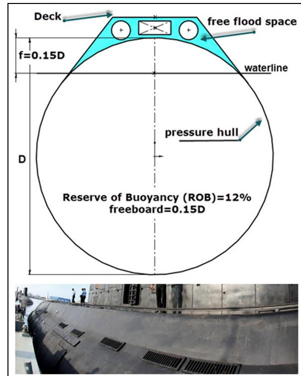
**Figure 1.** Freeboard, deck and free-flooding space in submarine.
