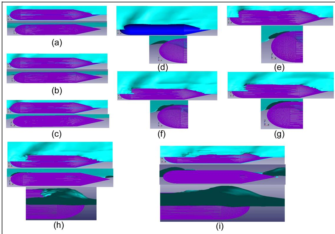
**Figure 8.** Up view and side view of free surface at  $h=0$  m: (a)  $F_n = 0.2$  ( $v = 1.4$  m/s), (b)  $F_n = 0.25$  ( $v = 1.75$  m/s), (c)  $F_n = 0.29$  ( $v = 2.03$  m/s), (d)  $F_n = 0.33$  ( $v = 2.31$  m/s), (e)  $F_n = 0.35$  ( $v = 2.45$  m/s), (f)  $F_n = 0.38$  ( $v = 2.66$  m/s), (g)  $F_n = 0.42$  ( $v = 2.94$  m/s), (h)  $F_n = 0.46$  ( $v = 3.22$  m/s) and (i)  $F_n = 0.5$  ( $v = 3.5$  m/s).
