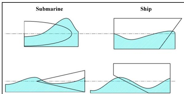
**Figure 3.** Comparison of wave system in submarines and ships.
