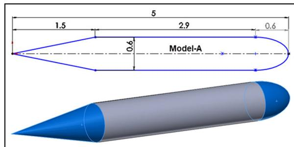
**Figure 4.** General configuration of the model.
