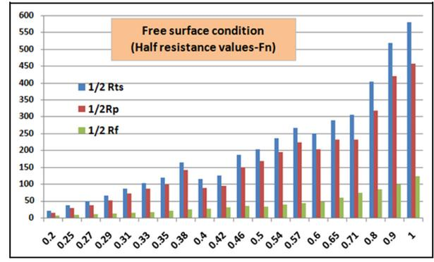
**Figure 10.** Resistance versus Froude numbers in free surface condition.
