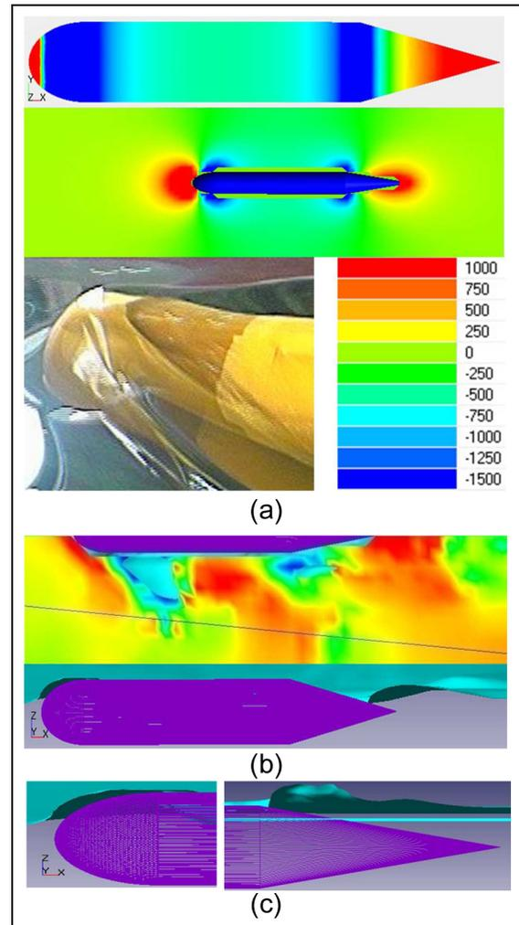
**Figure 2.** Pressure field and wave shape: (a) pressure field around a submarine at fully submerged depth, (b) free surface elevation according to the pressure field and (c) bow and stern wave in high pressure area.
