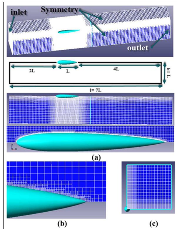
**Figure 7.** Quarterly modeling because of axis-symmetry at fully submerged condition (without free surface effect). (a) dimensions of domain (b) fine meshes around the body (c) quarterly modeling of the domain.
