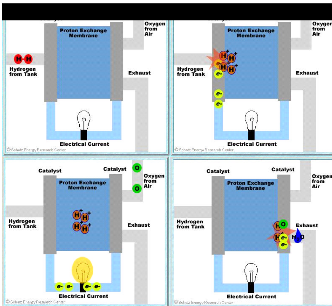
Figure 6 - Basic functionality for PEM Fuel Cell
