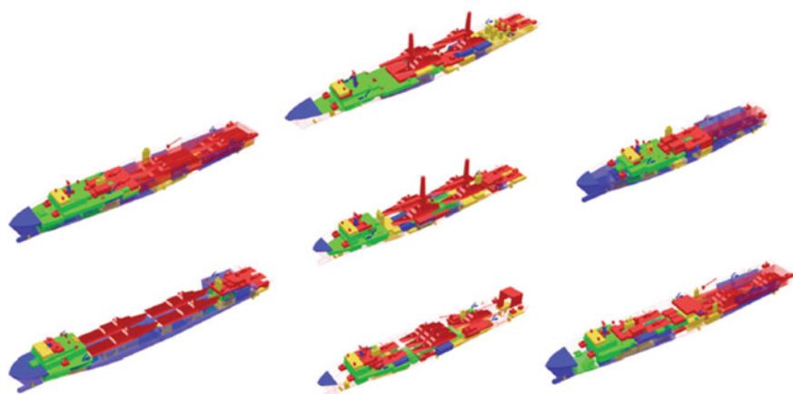
Fig. 10.14 Configuration of a vessel from building blocks from a library, for rapid evaluation and requirements elucidation in early design stages (Andrews 2011)
