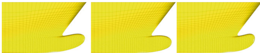
Fig. 6.44 Effect of form parameter “bulb length”
