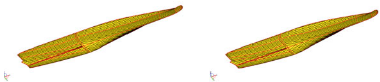
(C) Panel meshes for seakeeping analysis (input to NEWDRIFT+)
