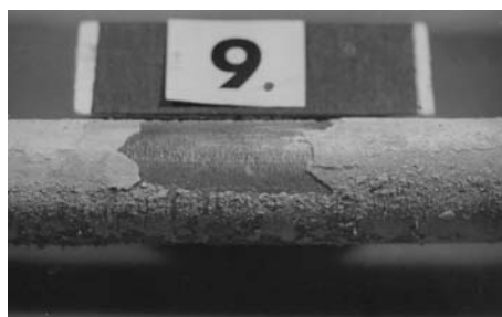
Figure 8. Titanium heat-exchanger with natural oxide film.
