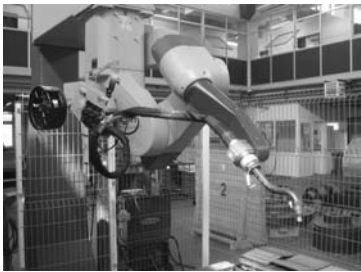
Figure 1. The welding robotic arm used in the experiments.
