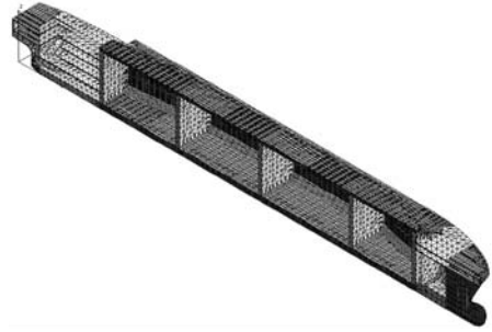
Figure 5a. The LNG 150000 m 3 carrier 3D-FEM hull model.
