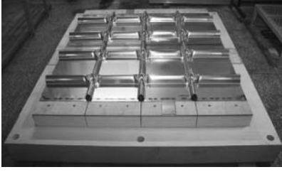
Figure 2. A real structure of MARK III type LNG cargo containment system on the full scale tested in the present study.
