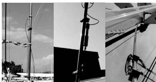
Figure 15. First installation of LVDTs onboard a 45 m ship.
