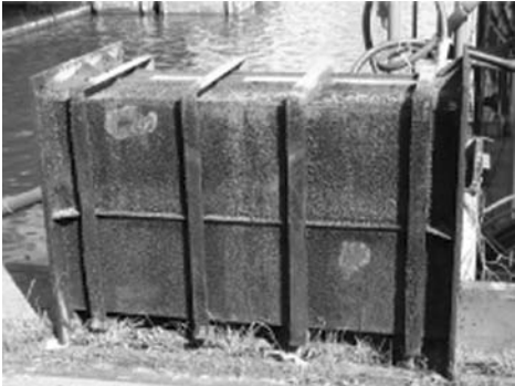
Figure 7. Box girder after test in hot sea water without anodic polarization.
