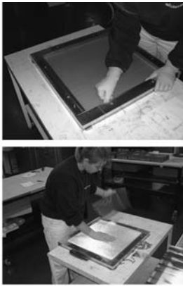
Figure 3. Hand lay-up in a double sided mould used for DTU panels (top, upper mould not positioned yet). Peel ply being removed prior to positioning of upper mould (bottom).
