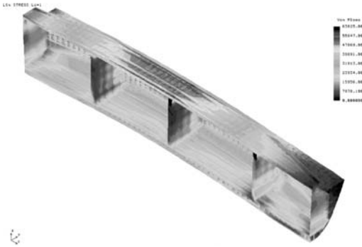
Figure 9b. \sigma_{vonM} [KN/m 2 ], h_w = 10.715 m, x = 53.6\text{--}246.4 m, hogging, full.
