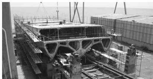
Figure 20. The assembling of the modules on the building slip.
