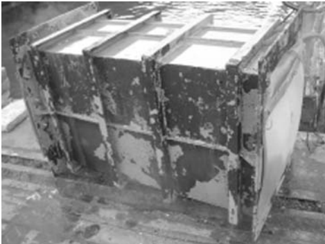
Figure 8. Box girder after test in hot sea water with anodic polarization.
