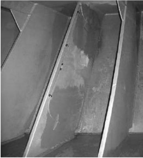
Figure 4. Mounting of sensors on a frame.
