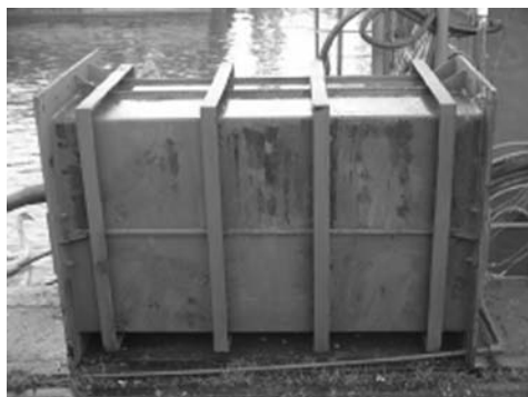
Figure 9. Box girder after test in cold sea water with anodic polarization.
