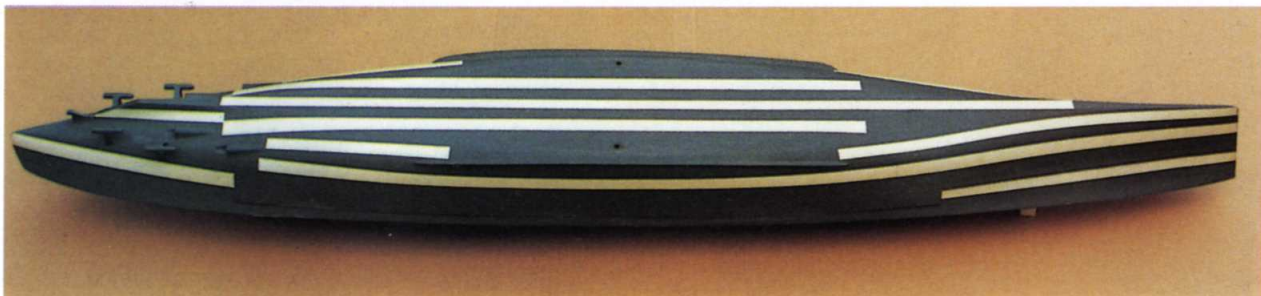
Fig. 9.6. Hull of Anson sprayed with primer and plated with cartridge paper.
