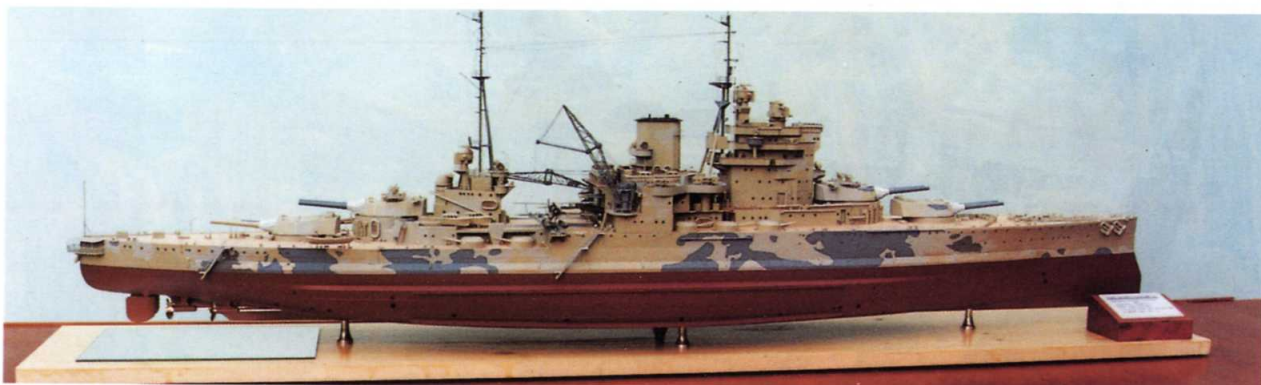
Fig. 1.12. Substantial brass standoffs can be seen supporting authors 1 : 150 scale model of HMS Queen Elizabeth
