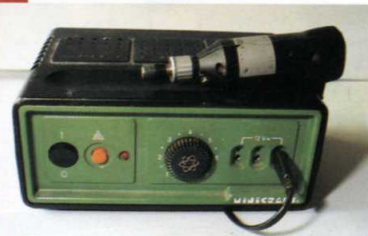
Fig. 3.23. Minicraft transformer/speed controller unit for low voltage hand-held tools.
