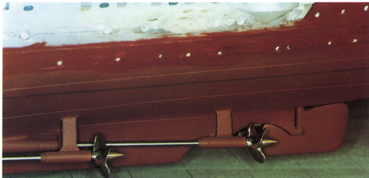
Fig. 9.2. Red anti-fouling sprayed by car aerosol.
