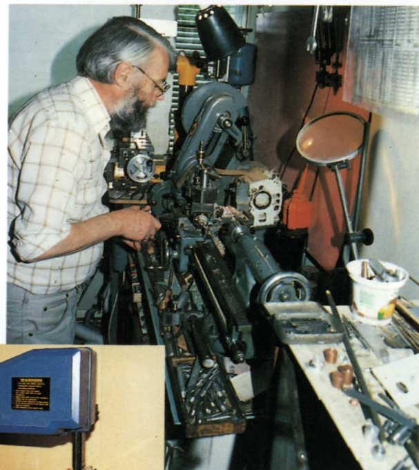
Fig. 3.13 Lathe (3.5" Myford), probably the single most useful machine tool for fine model building to be found in the author's workshop.
