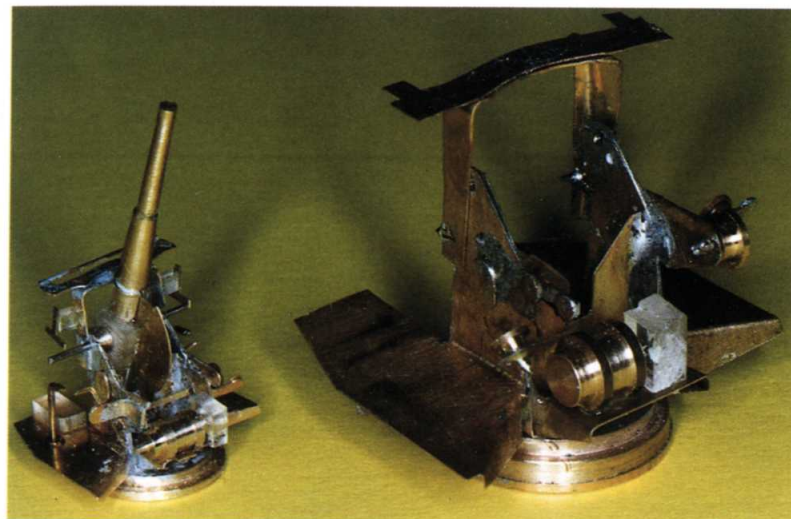
Fig. 7.29. Left, the final un-painted version of a 4.7in dual-purpose HA/LA gun for Glorious. Right, twice full-size mock up using the etching drawings as a pattern to check for accuracy. (The etching drawings are drawn twice final size). This is an example of a totally open gun position with no turret or shields.
