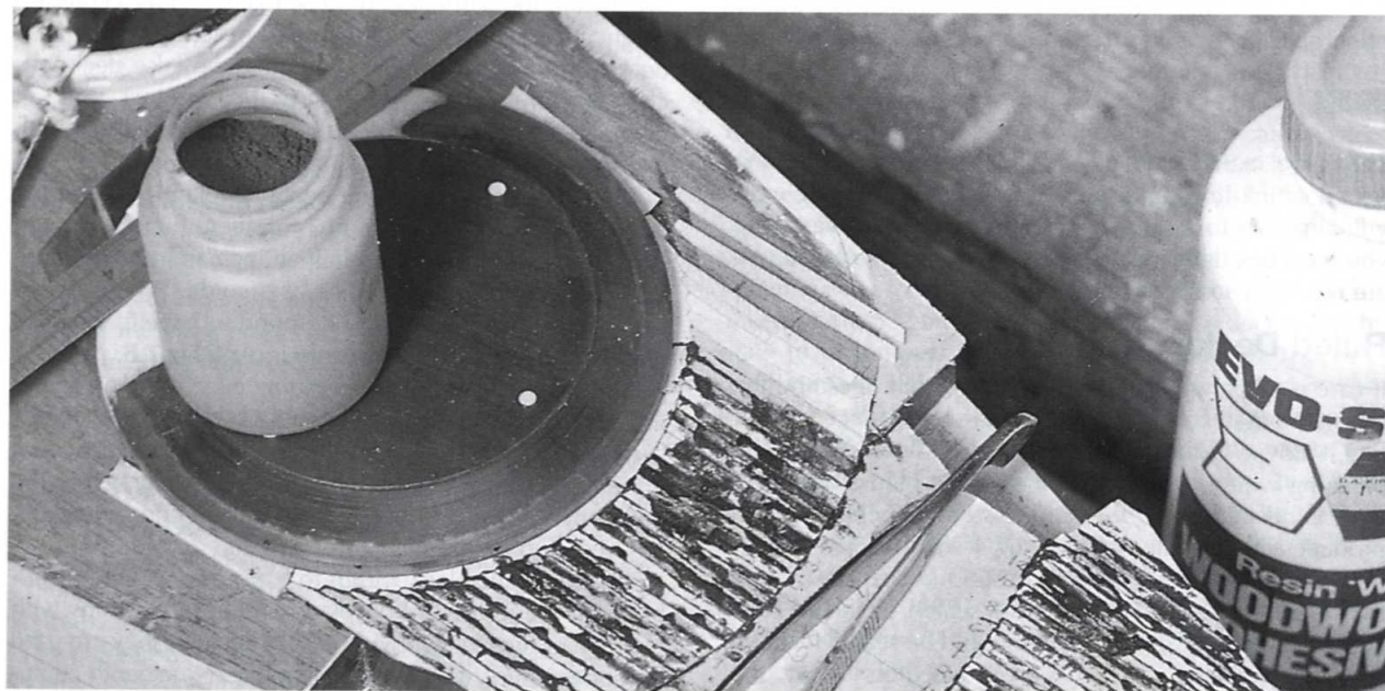
Fig. 6.21 Deck laid with black poster colour before cleaning off
