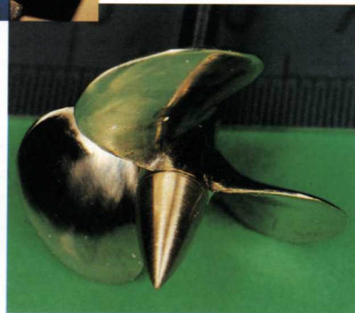
Fig. 3.33. Cast metal propeller for Belfast with replacement machined exit cone.
