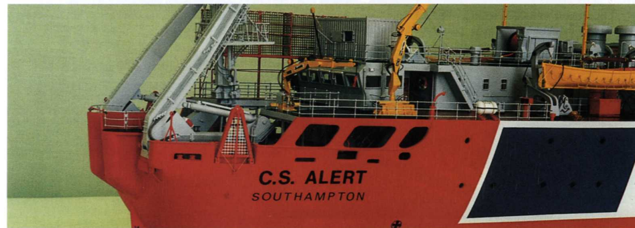
Fig. 4.6. Jimmy Wood - CS Alert showing aft 'A' frame gantry in stowed position. (J Wood photo).
