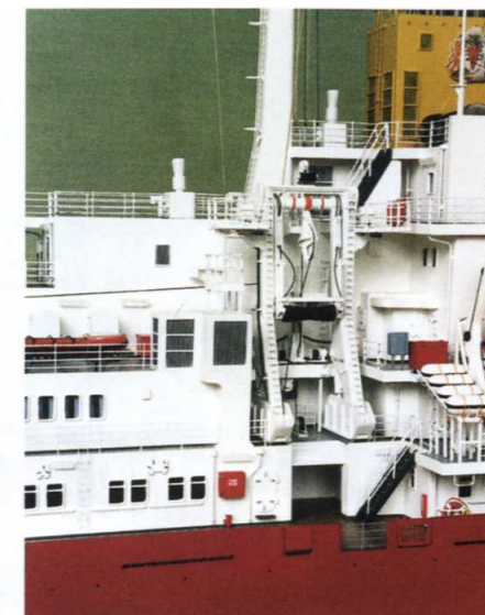
Fig. 4.4 Detail of starboard side - midships scientific gantry on RRS James Clark Ross by Jimmy Wood. (J Wood photo).
