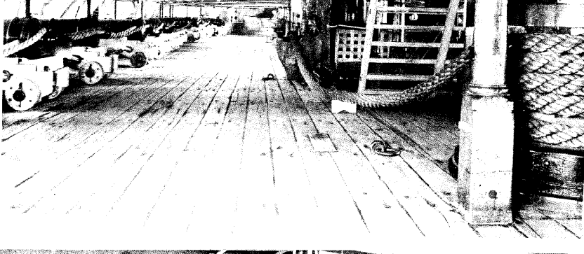
13. Lower deck, port. The photo was taken in 1953 from just aft of the main capstan. Note the messenger and removable pillars. The guns ranged along the ship's side are 32-pounders. Wright & Logan
