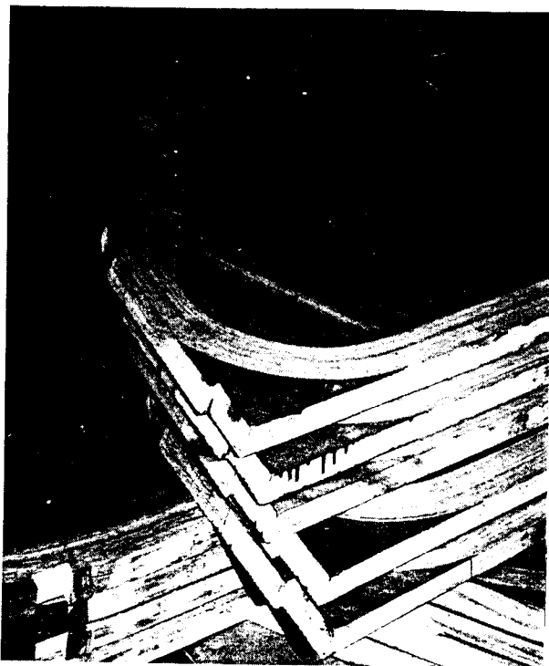
Plate 1.47 Several of the ring frames showing how solid timber is incorporated into corners that are too tight to laminate.
