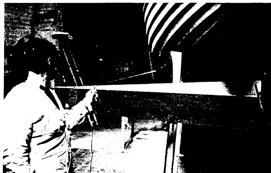
Plate 1.56 A flared boot top is marked by gradually moving the string up a wedge placed on top of the straight edge.
