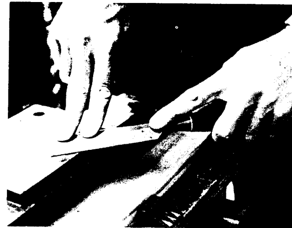
Plate 3.16 With the back of the blade pressed flat against the stone a few strokes remove the 'burr'.
