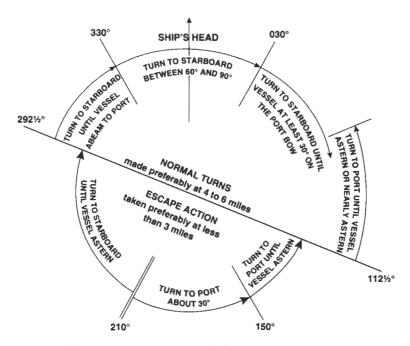
Course Alteration Diagram intended primarily for use in avoiding a vessel detected by radar but not in sight Journal of the Institute of Navigation, Vol. 25, Page 105
