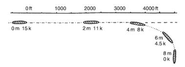
The diagram shows the path traced out by a vessel of about 23,000 tons displacement when making a crash stop after going at her full speed of approximately 15 knots.
