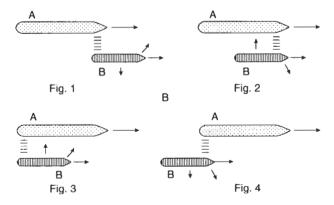
When the sterns of the two vessels come together there will be a repulsive force between them so that once again there will be a tendency for the bows of vessel B to swing inwards, (fig. 3). The Olympic-Hawke collision may have been caused by this effect.
