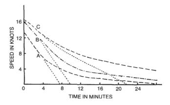
power is likely to be less than maximum ahead power. For diesel engines the proportion will usually be over 80% but for geared steam turbines it may only be about 40%.
