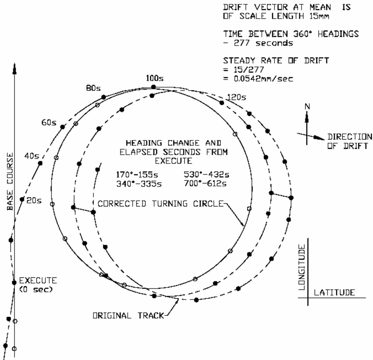
Figure B1: Correcting Turning Circle For Drift
