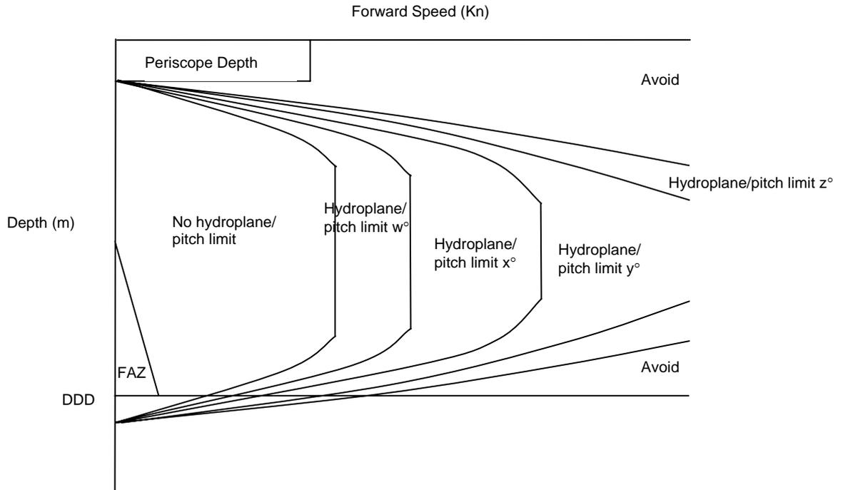
Figure 6.1 Example of a Manoeuvring Limitation Diagram
