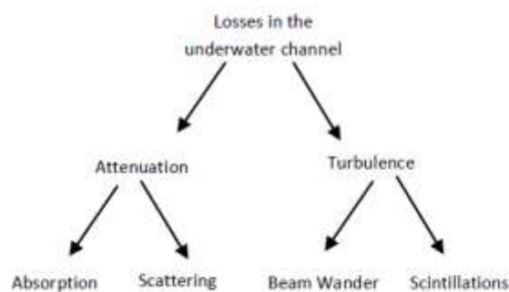
Figure 7 – Losses Encountered by an Optical Beam in Water
