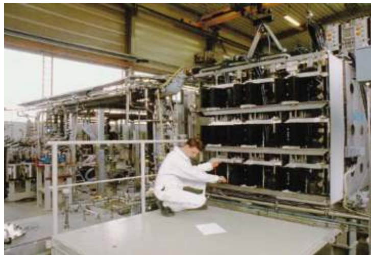
Figure 4: A Siemens 300 kW PEMFC Stack Assembly as used on the German 212 AIP Submarine (Copyright Jane's Information Group; Source: HDW)
