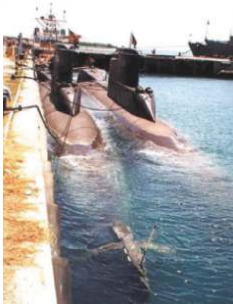
Figure 9 – German Navy's Type 206A submarines with 1.3964.9 nonmagnetic steel hull [2]
