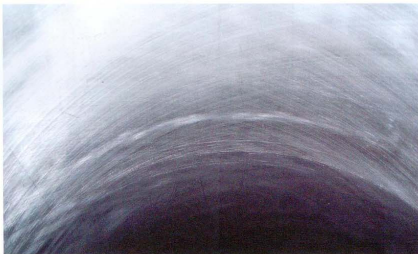
◀ Honing gives a precise finish of the cylinder-liner running surface.
