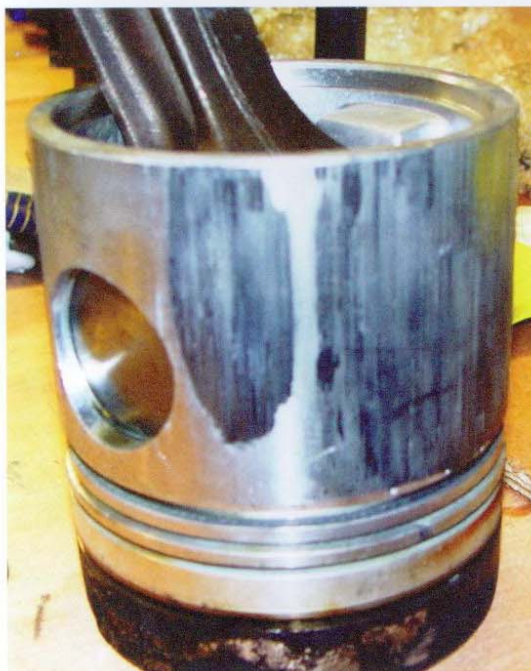
◀ 'Fretting' of a piston due to poor lubrication.
