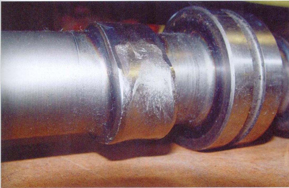
◀ An overheated and distorted cam.
