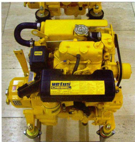
▲ Vibration dampers below a two-cylinder high-speed four-stroke diesel engine for yacht propulsion.
