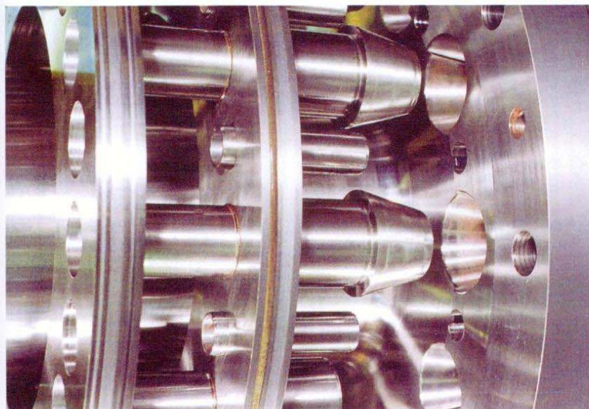
◀ The conical coupling bolts of the mechanical coupling of MAN-B&W.
