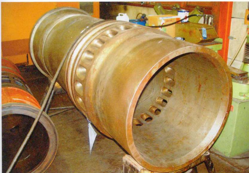
A modern cylinder liner with inlet ports.
