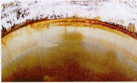
◀ A worn cylinder liner.
