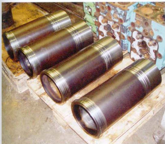
▲ Cylinder liners prior to honing.
