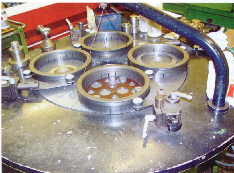
A polishing machine for trueing up parts of atomisers and fuel pumps.
