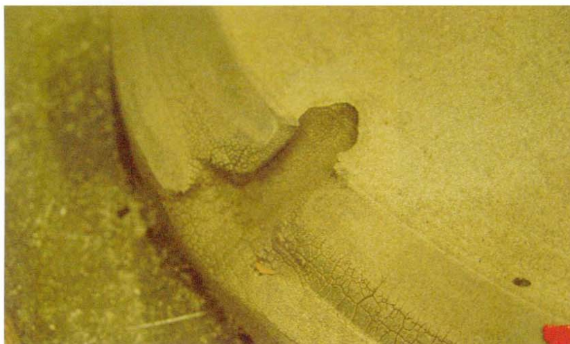
▲ If repairs are postponed for too long, an exhaust valve may start to leak severely, the so-called blow-through.
