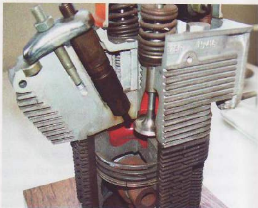
▲ Cooling fins on the cylinder liner of a small high-speed diesel engine.
