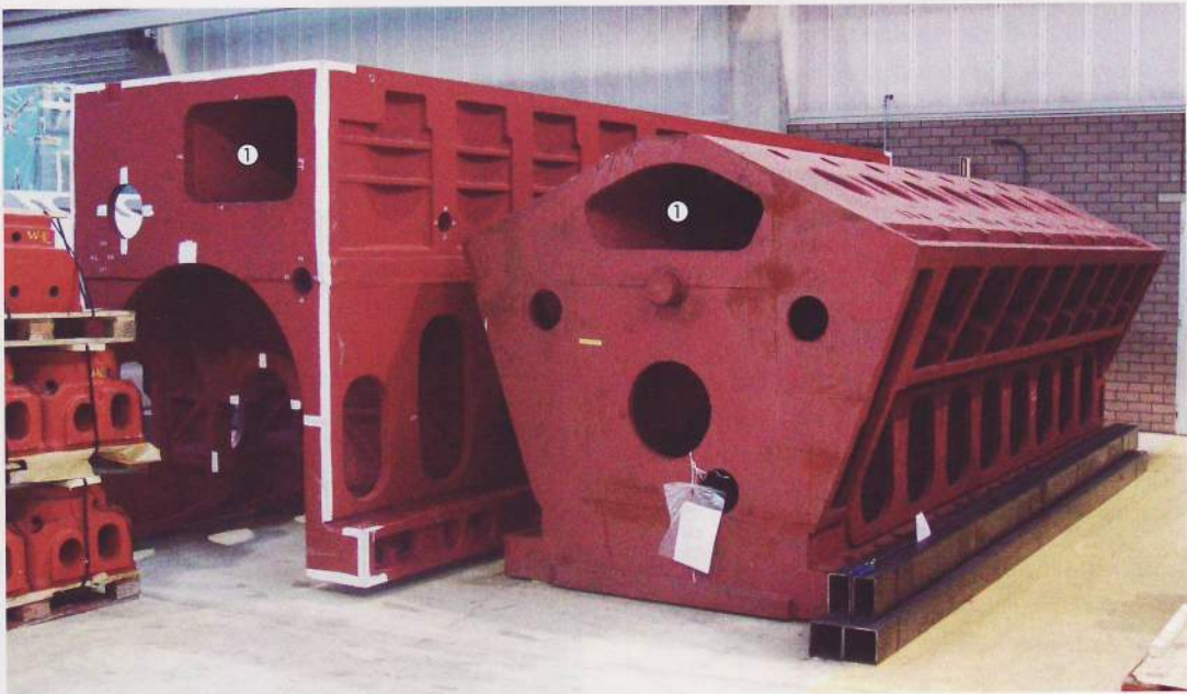
▶ The inlet manifold of two medium-speed V-type engines.
