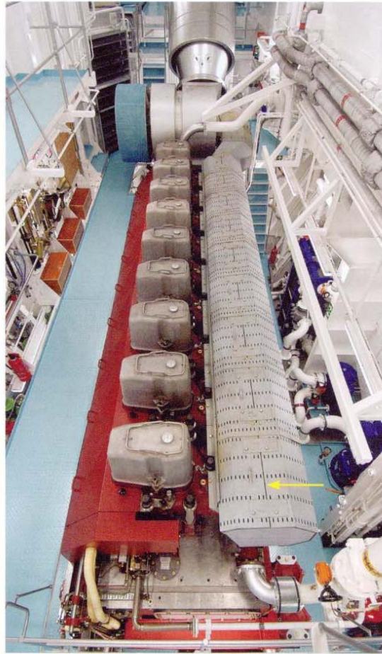
The steel sheet protection of the exhaust-gas line of this propulsion engine may attain a maximum surface temperature of 220 °C.
