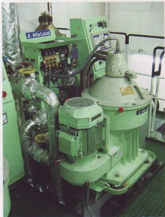
► An automatic lubricating oil centrifuge.
