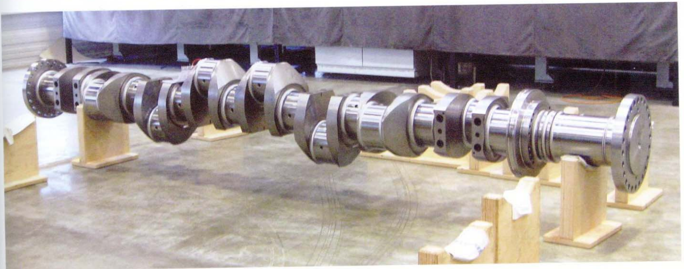
▲ A finished crankshaft for an eight-cylinder in-line engine, Category III. The crankshaft is prepared for transport to the engine manufacturer.
