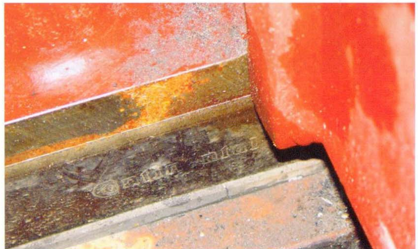
A flexible rubber mounting below a large Caterpillar-MAK 43-L propulsion engine.
