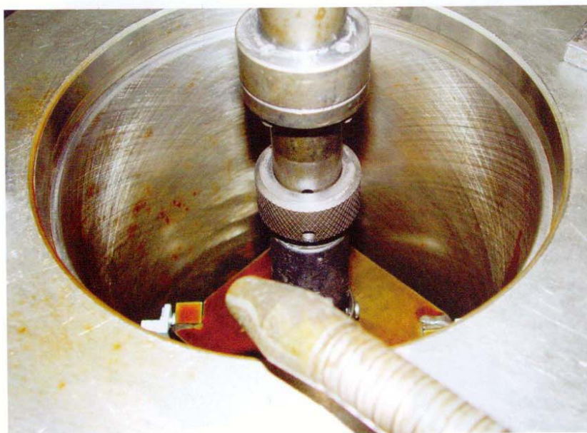
▼ Honing a cylinder liner in the engine.
