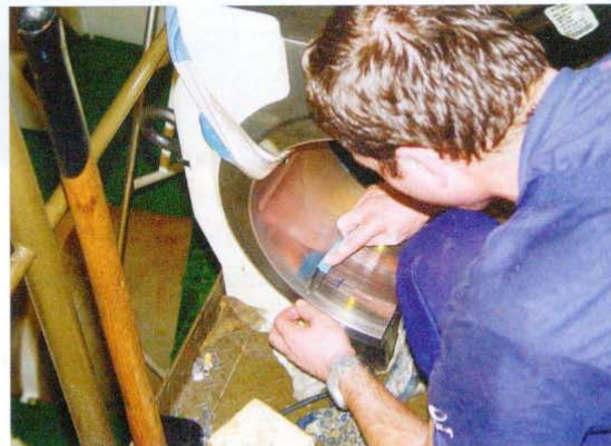
▲ Manual finish of a camshaft bearing.
