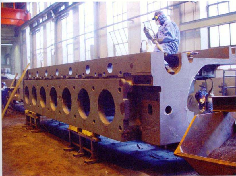
◀ Finishing of the casting, a seven-cylinder line-engine block.
