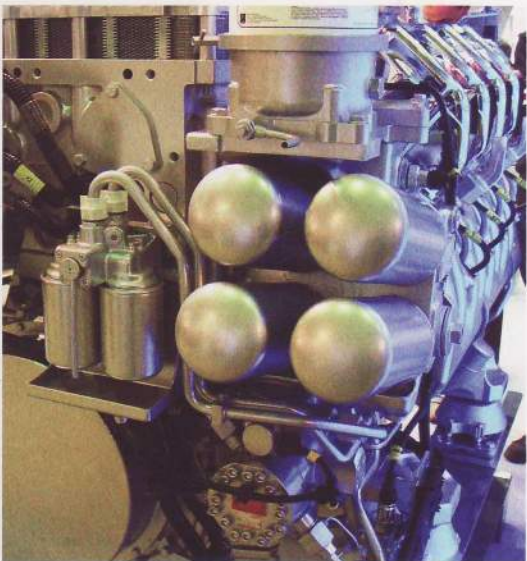
▲ Four lubricating fine oil filters in a diesel engine from MTU.
