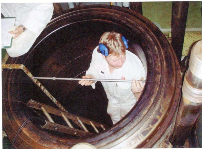
▲ Measuring cylinder liner wear.
