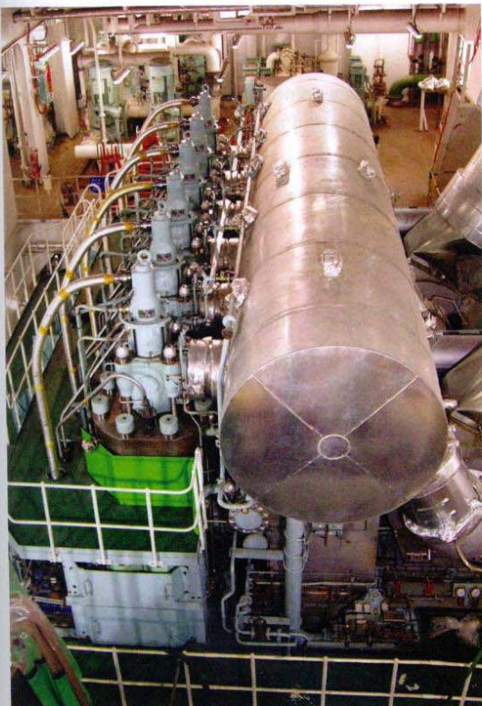
One of the two-stroke crosshead engines, used for the propulsion of a large LNG tanker, a MAN-B&W 6S70ME-C engine with a shaft power of 18,660 kW.
