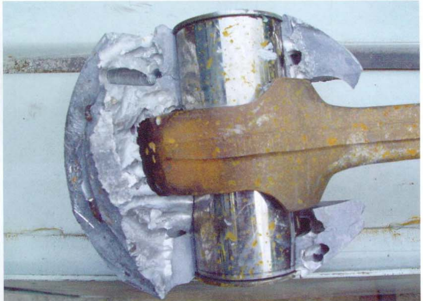
▲ A damaged piston with connecting rod.
