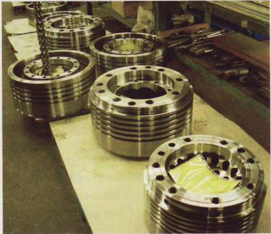
▲ All the pistons of modern two-stroke crosshead engines are cooled with lubricating oil.
