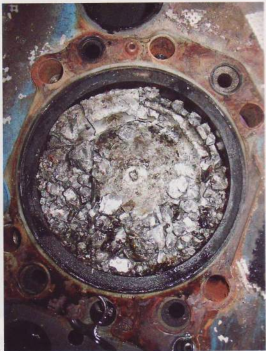
▲ A completely seized piston.
