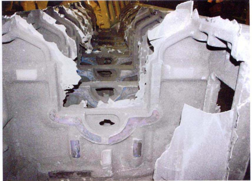
◀ Finishing of the casting, a seven-cylinder line-engine block.
