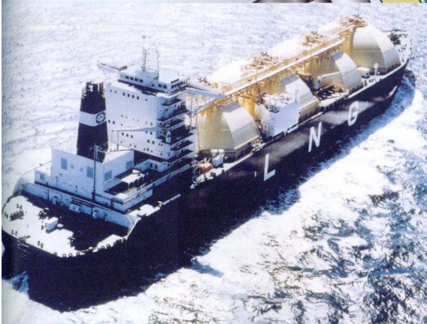
A modern LNG tanker, driven by dual-fuel engines.
