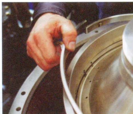
CentriLock lifts out and snaps in easily – without any threads to wear.
