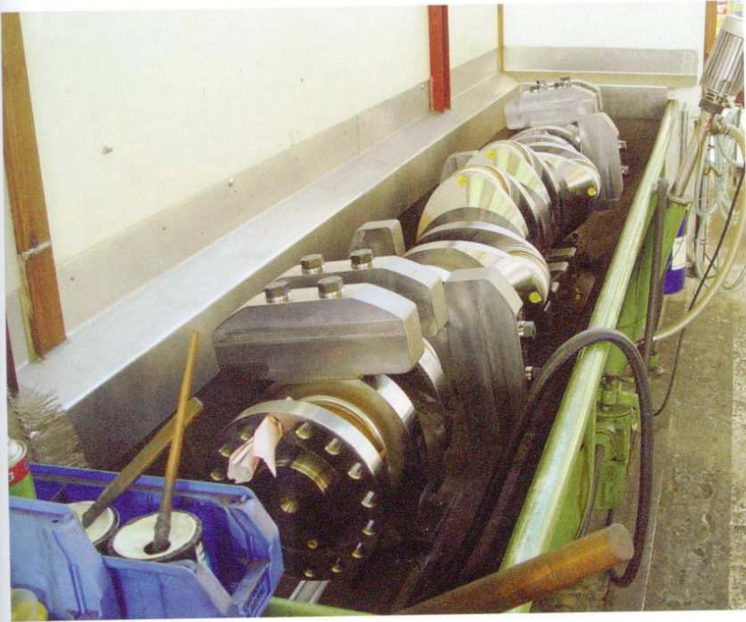
◀ A new crankshaft is placed in a washing machine to remove the final dirt particles before the crankshaft is placed in the engine block. Caterpillar Mak, Kiel, Germany.
