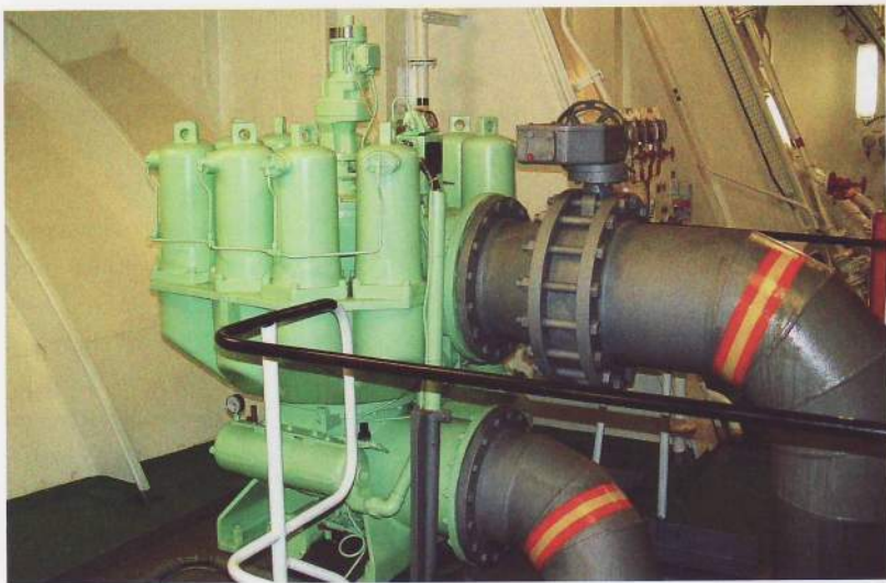
▲ An automatic lubricating fine oil filter.
