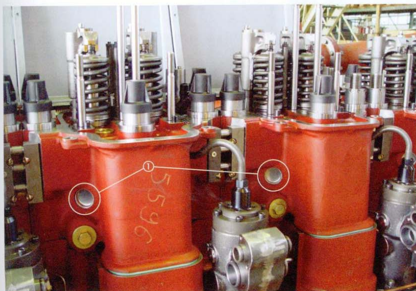
Cylinder heads of a Caterpillar-MaK engine under construction.
