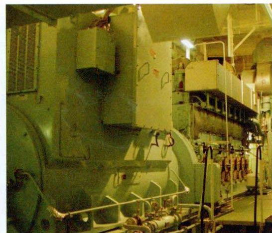
▲ A large 3.5 MW diesel genset on a container ship.
