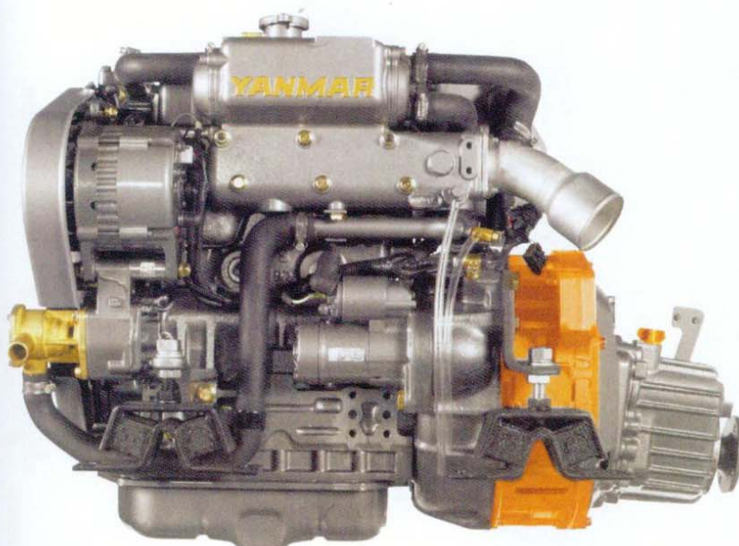
◀ An electric generator (yellow) between a Yanmar diesel engine and gearbox with reverse clutch.
