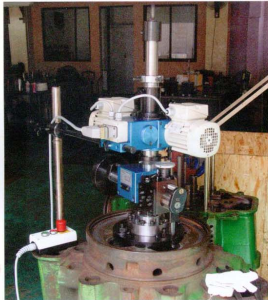
◀ Levelling a cylinder head with a portable planing machine.
