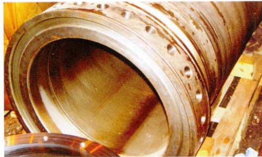
◀ A cylinder liner of a large four-stroke engine for repair.
