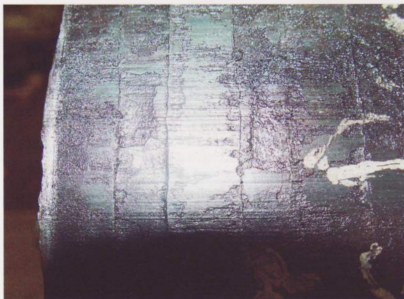
▲ A severely damaged piston in a two-stroke crosshead engine.
