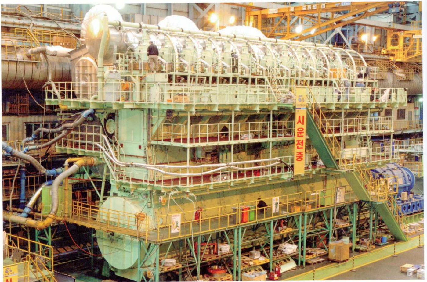
▲ One of the largest diesel engines being tested; the 'blue' water brake is being used as a load. This is a Wärtsilä Sulzer RT Flex 96 C.
