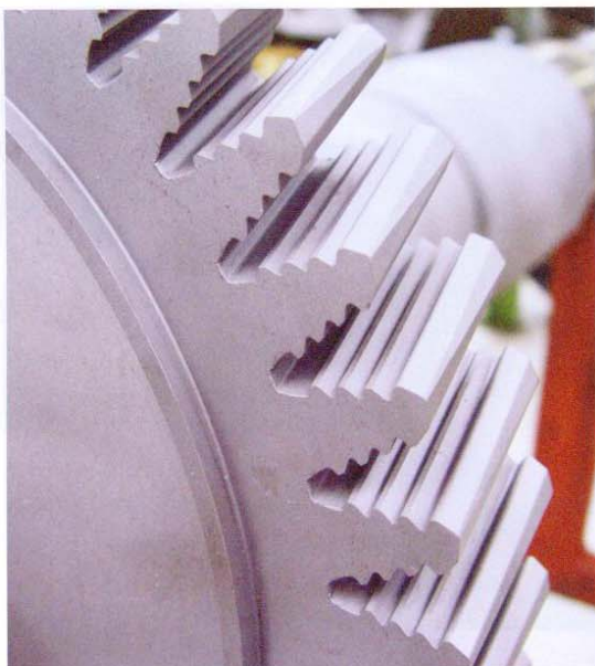
▲ A blade-attachment system of the exhaust-gas turbine on the turbine wheel. This is called the 'Christmas tree configuration'.
