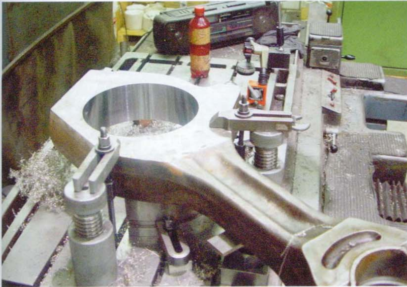
Reconditioning a connecting rod. Line boring the connecting-rod big end/crankpin (in the background) and the line boring of the connecting-rod head/piston pin (in the foreground).
