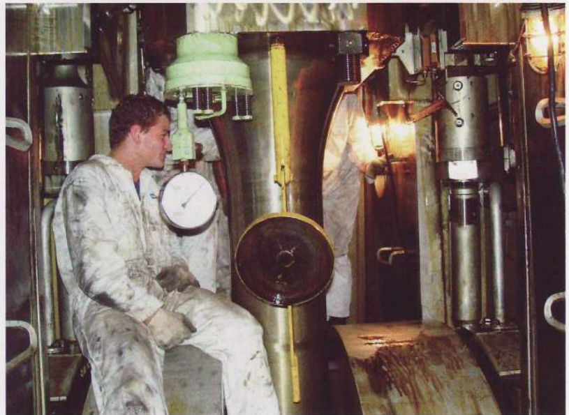
▲ Maintenance on the drive gear in the crank case of a two-stroke crosshead engine.
