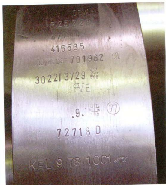
Stamped codes on a crankshaft web.
