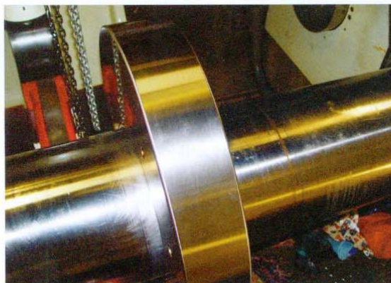
▲ The hydraulically tensioned cams on the camshaft.
