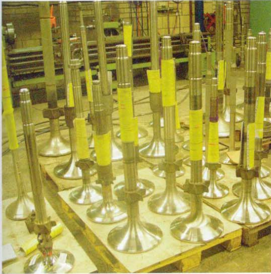
▲ Exhaust valves during reconditioning.
