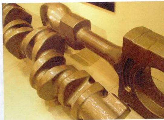
◀ A forged crankshaft of a Category II engine and a connecting rod for a Category III engine.
