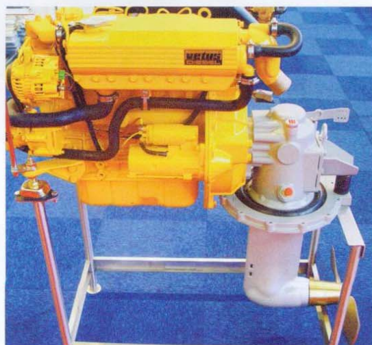
◀ A small four-stroke high-speed diesel engine ('Vetus') with an angle gear set through the yacht's hull.
