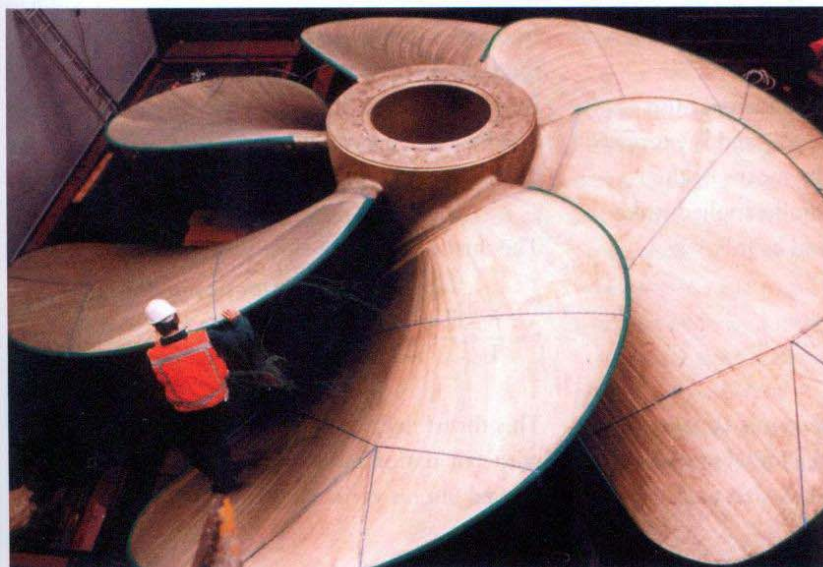
◀ A large six-blade fixed-pitch propeller for a large containership (Wärtsilä Propulsion).
