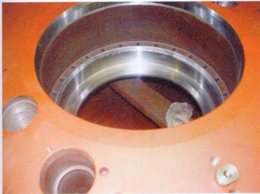
▲ A cylinder cover. In the middle, place for the central exhaust valve.
