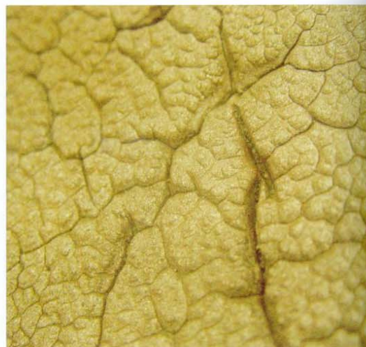
▲ A microscopic view of an exhaust valve on the combustion-chamber side, seriously affected by high-temperature corrosion.
