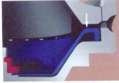
STEP TWO: During sludge discharge, the edge of the slide flexes downward, exposing the ports.
