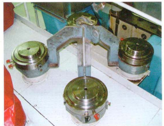
The four hydraulic jacks with hoisting equipment for a Wärtsilä 46 diesel engine category III.
