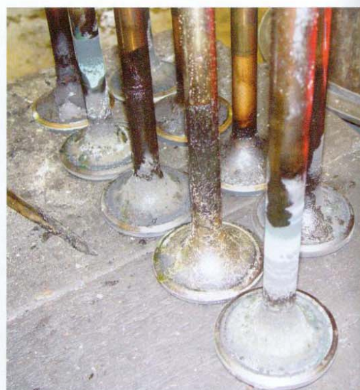
▲ Soiled exhaust valves are checked for wear, hair cracks and size, after cleaning.
