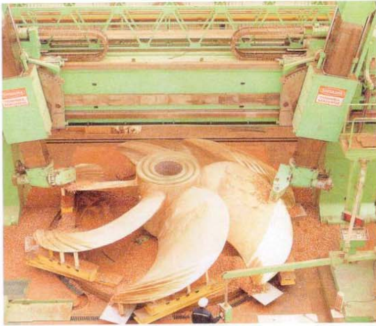
▲ Machining a large six-bladed fixed-pitch propeller for a container ship.
