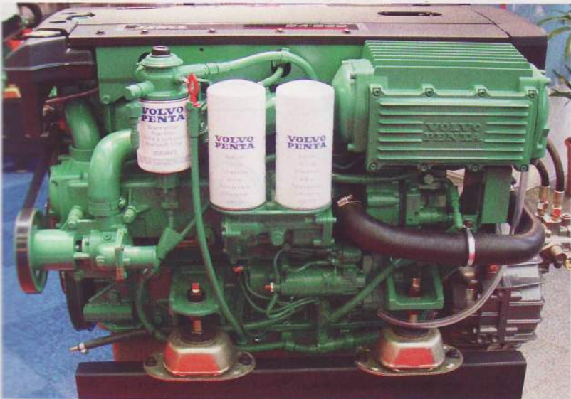
▲ Two lubricating oil fine filters in a diesel engine from Volvo Penta.
