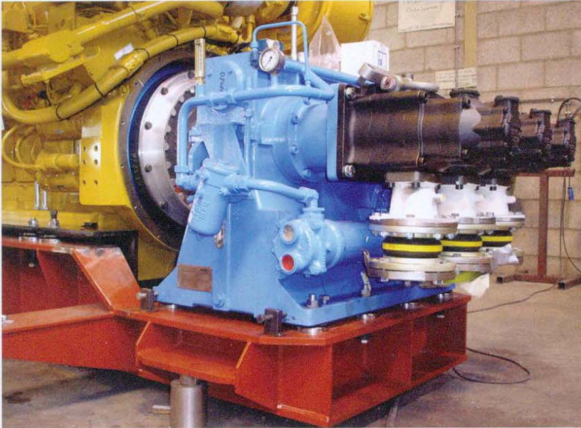
◀ Vibracon Low Profile chocks below Stork gearboxes and high-pressure pumps. Driven by a Caterpillar 3512 diesel engine, Category II.
