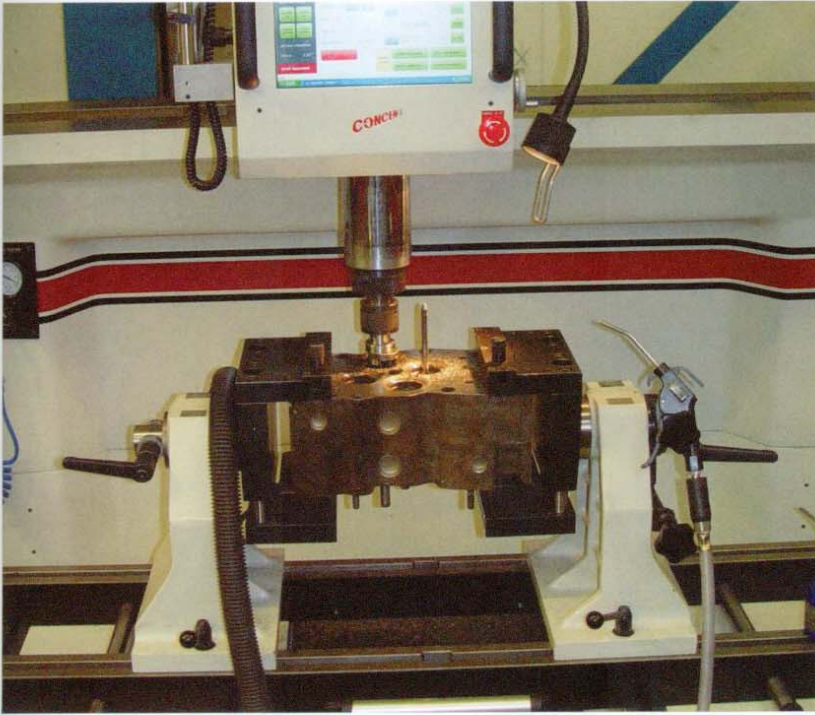
◀ A Rottler machine for trueing up the valve seats.
