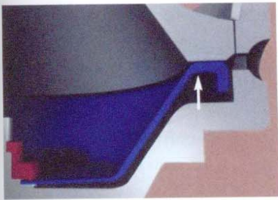
STEP ONE: The CentriShoot discharge slide is fixed at the centre. During separation it blocks the discharge ports.
