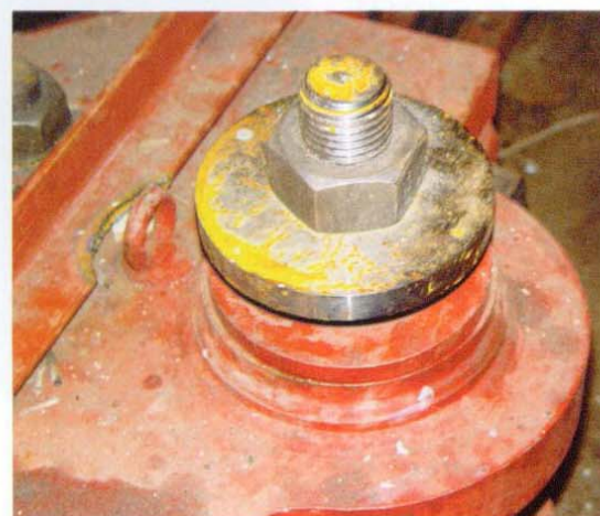
A side-support bolt for the same Caterpillar 43-L propulsion engine.
