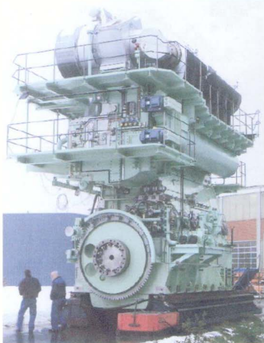
▲ A relatively small two-stroke crosshead engine of MAN-B&W, type ME.
