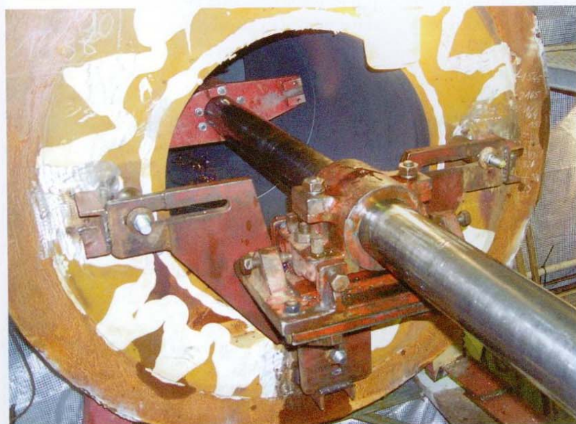
Line boring a stern tube.
