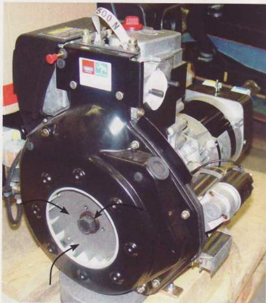
▲ A small single cylinder air-cooled diesel power unit (arrow = air supply).
