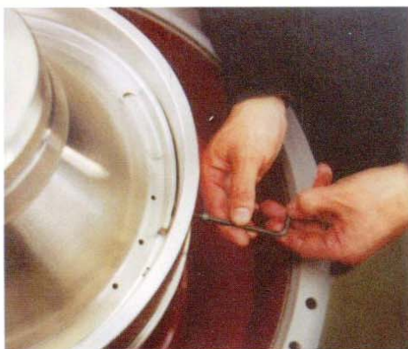
CentriLock can be only removed with an Allen key. No sledge hammer is necessary.
