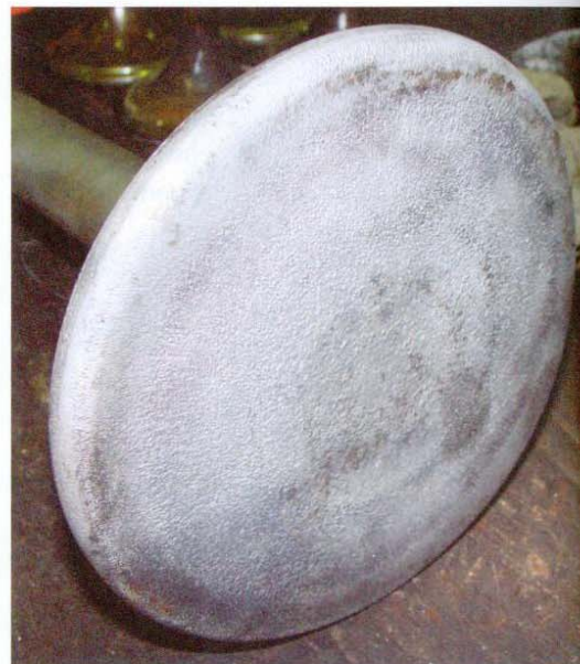
▲ An exhaust valve affected by high-temperature corrosion.
