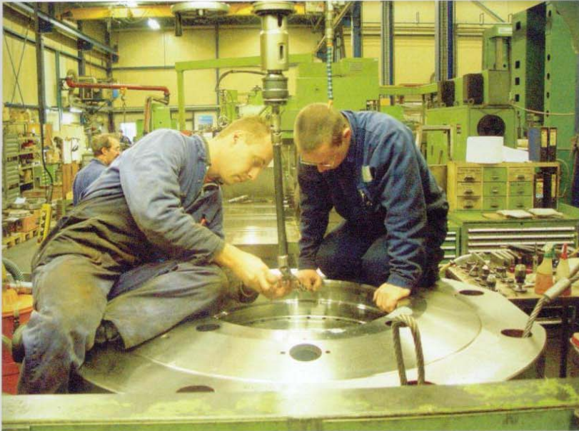
▲ Machining a cylinder cover.
