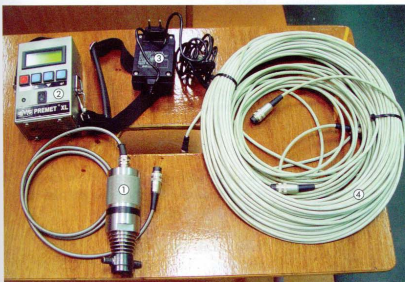
◀ A Lemag electronic pressure sensor, the Premet XL.
