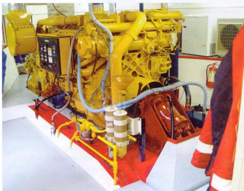
◀ A propulsion installation with a four-stroke high-speed Caterpillar diesel engine running on M.D.O.. Used for inland navigation.
