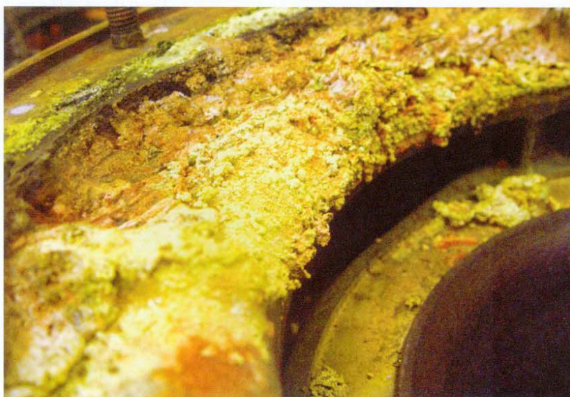
▲ A filthy turboblower casing.
