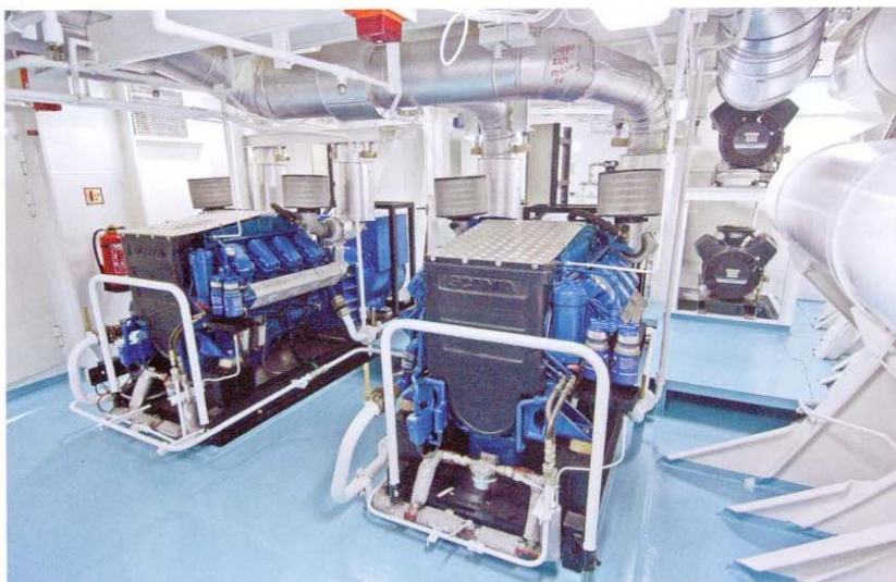
▲ The arrangement of two diesel power units, category II.
