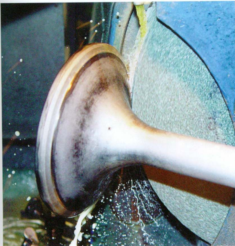
◀ Grinding of a valve seat using a grinding stone mounted on a grinding machine.
