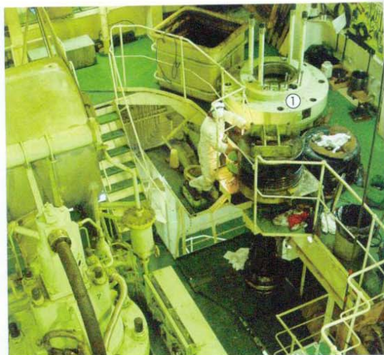
Top right: a disassembled cylinder head (1) is cleaned for inspection.
