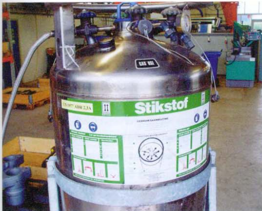
▲ An insulated liquid-nitrogen drum.
