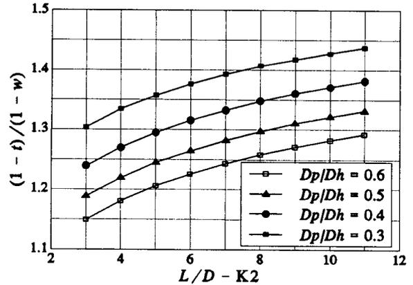
Figure 13.  $(1 - t)/(1 - w)$  vs  $(L/D - K2)$
