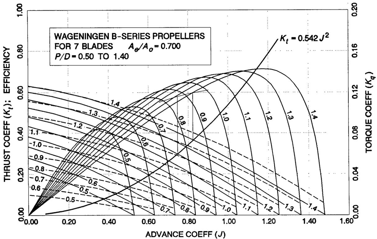
Figure 14. Propeller Thrust and Torque
