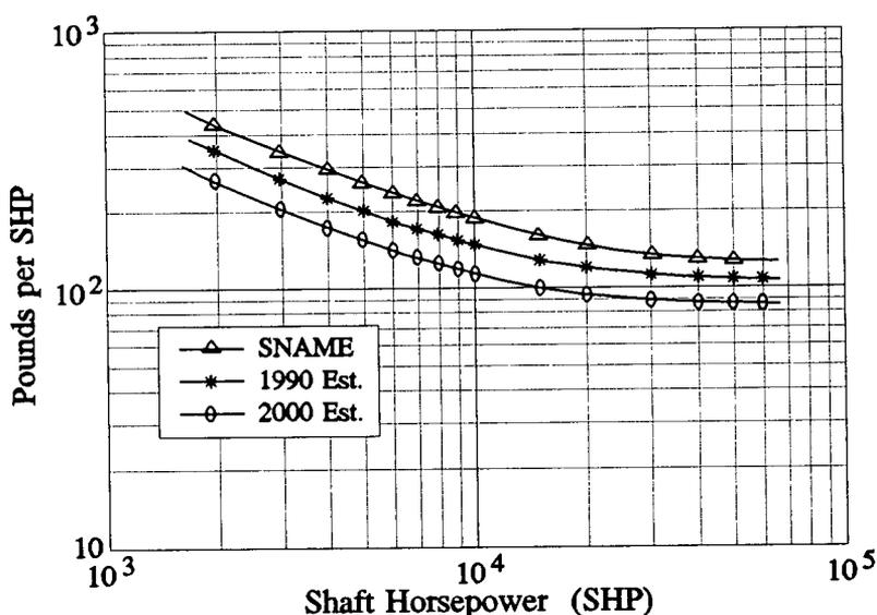
Figure 4. Machinery Weight Predictions
