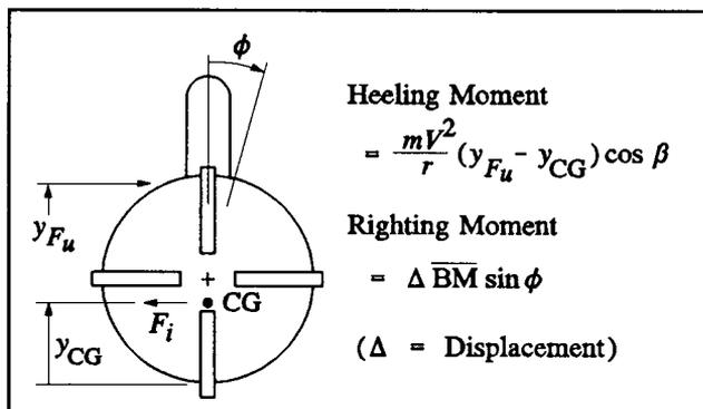
Figure 20. Heel Due to a Turn
