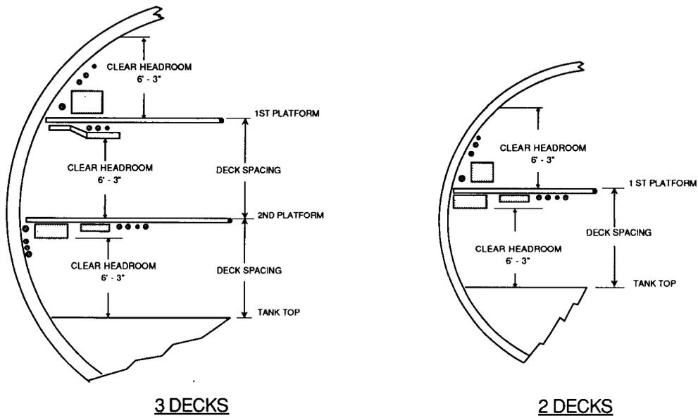
Fig. 25 Typical submarine arrangement sections
