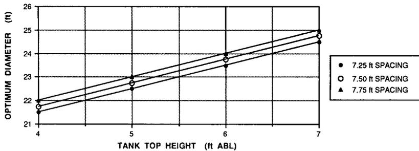
Fig. 27 Optimum diameter curves for two-deck submarines
