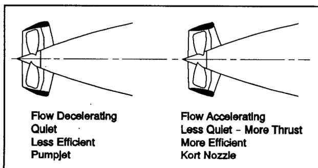
Figure 15. Pumpjet vs Kort Nozzle
