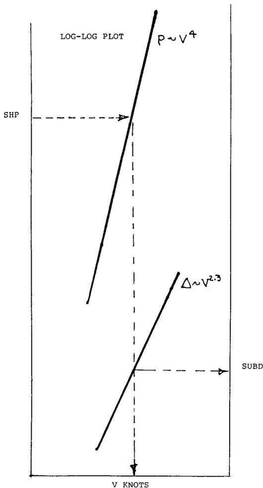
Fig. 31 Speed-power-displacement curves
