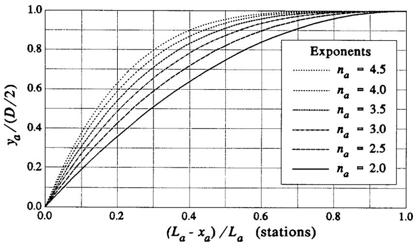
**Figure 23. Run Offsets (Equation (3))**
