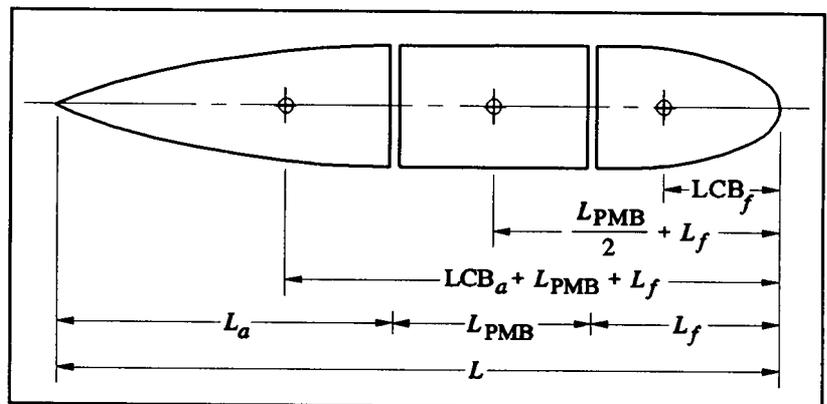
Figure 8. Centers of Various Parts of a Body of Revolution
