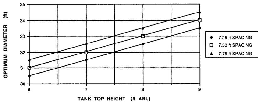
Fig. 28 Optimum diameter curves for three-deck submarines
