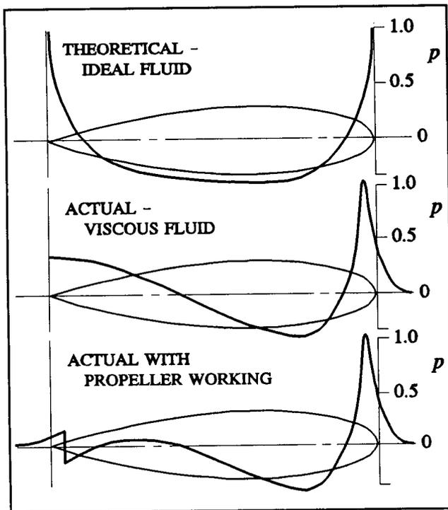
Figure 10. Pressure Distribution Around Hull, Related to Ambient
