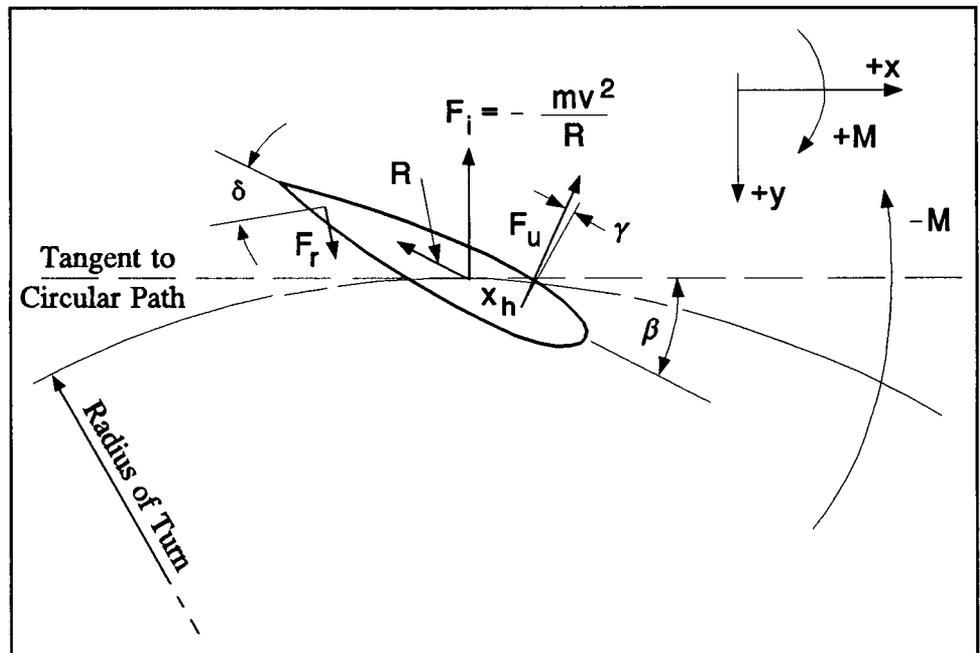
Figure 19. Hydrodynamics Forces on a Turning Submarine
