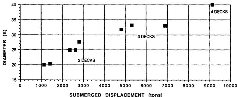
**Fig. 24** Typical submarine diameter trends
