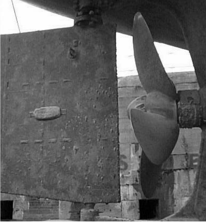
Figure 4 The rudder and propeller of a small vessel in dry dock
