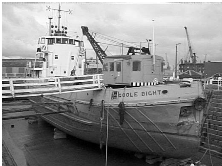
Figure 2 A small grab dredger in a graving dock
