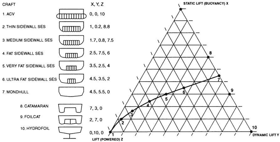
**Fig. 1.18** Proportions of different lift force for high-performance marine vessels (HPMV) concepts
