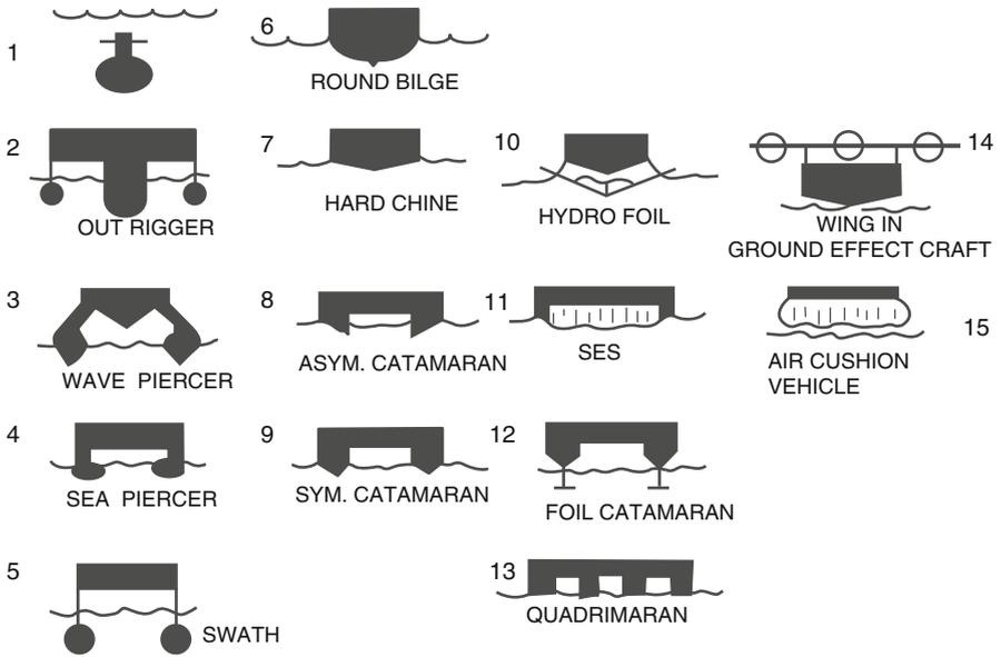
Fig. 1.19 HPMV hull section geometries
