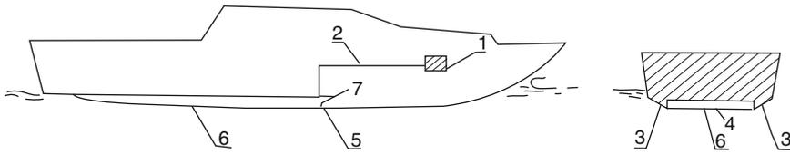
**Fig. 7.1** Air cavity craft (ACC) system diagram
