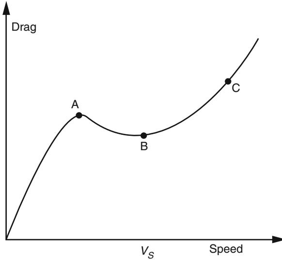
**Fig. 2.66** Drag curve of ACV with speed
