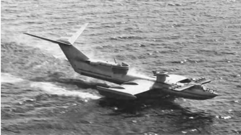
**Fig. 1.15** Alexeyev SM-8 wing in ground effect (WIG)
