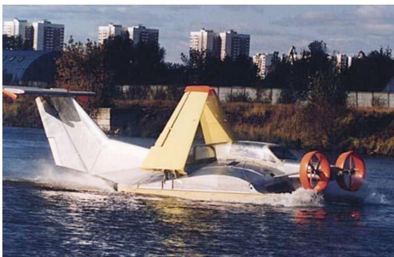
Fig. 3.21 Ivolga with wings retracted
