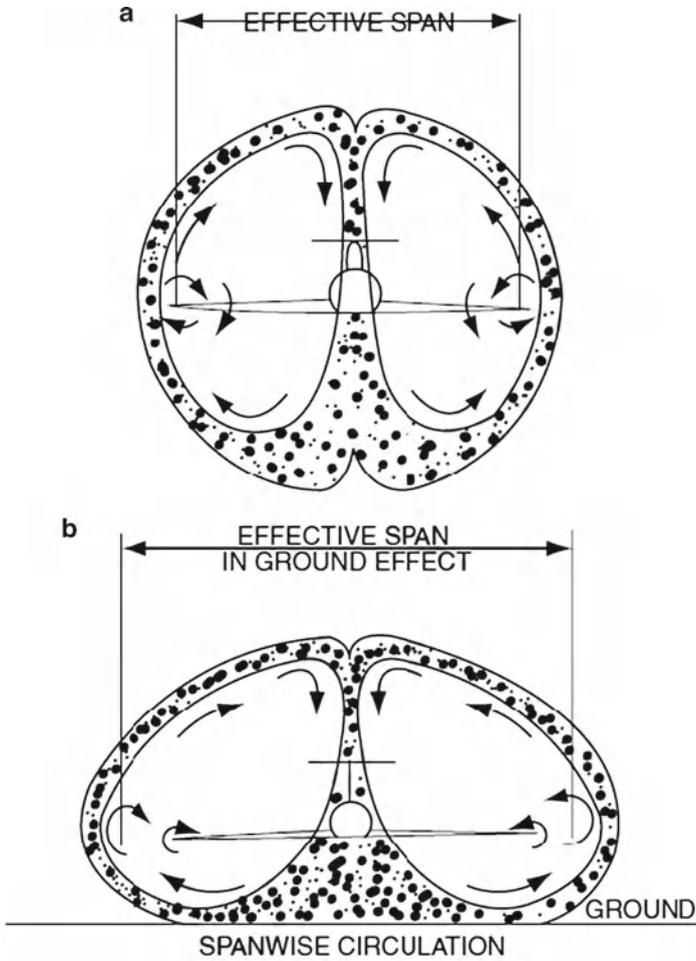
Fig. 3.3 Wing blockage phenomena in ground effect
