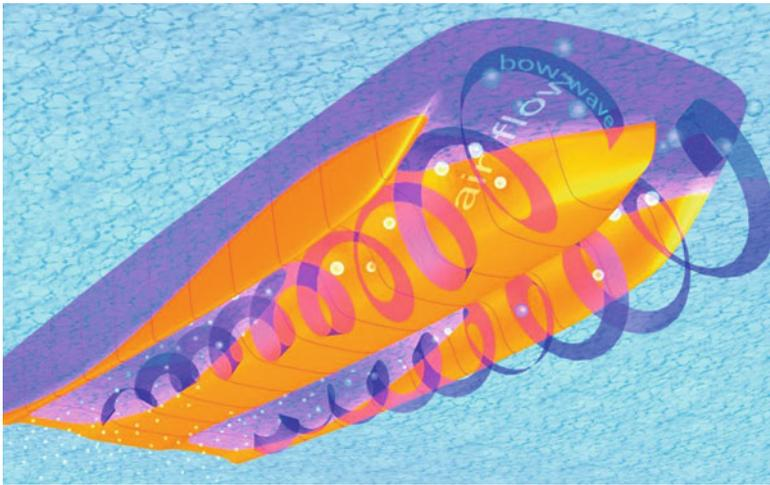
**Fig. 7.25** M craft spiral between hulls
