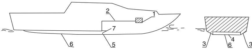
**Fig. 7.1** Air cavity craft (ACC) system diagram
