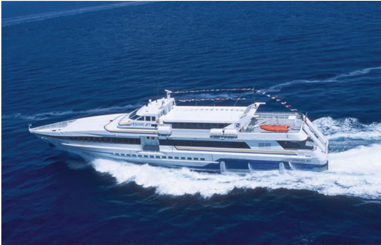
**Fig. 4.18** High-speed monohull ferry Vesuvio Jet 4
