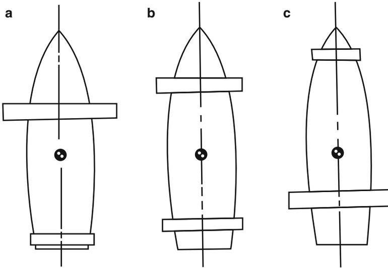
**Fig. 5.9** Shallow-submerged foil arrangements for longitudinal stability
