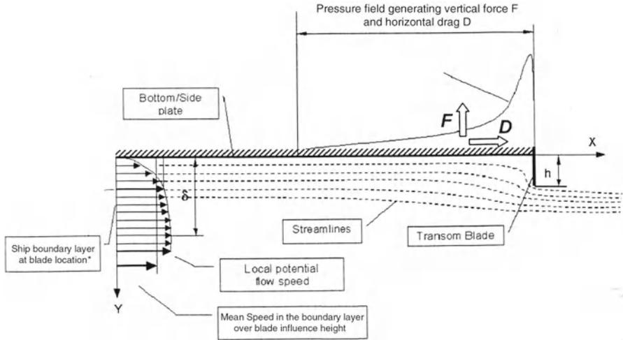
Fig. 7.11 Interceptor schematic
