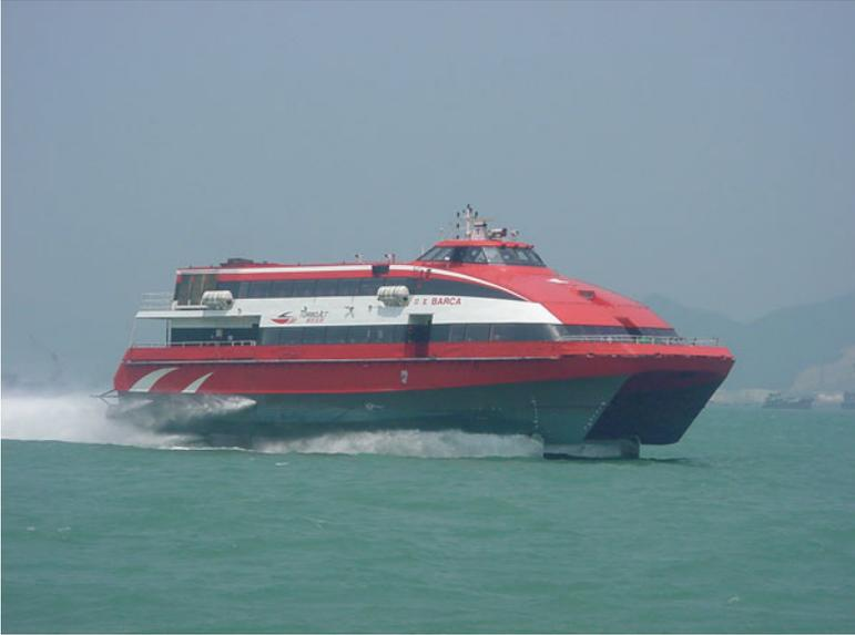
**Fig. 8.12** Fjellstrand 35 m Foilcat “Barca”
