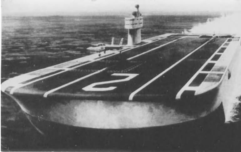
**Fig. 2.51** SES 10,000 mini aircraft carrier
