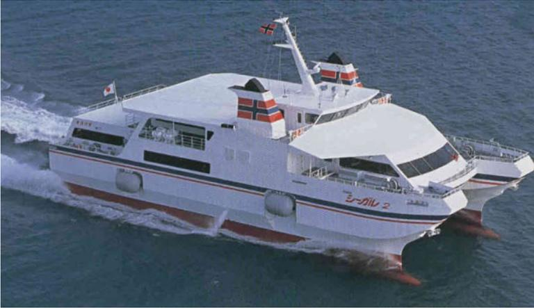
**Fig. 1.16** High-speed small water plane twin hull (SWATH), Seagull 2
