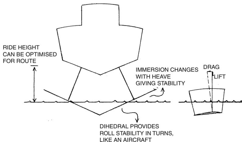
**Fig. 5.1** Hydrofoil principle
