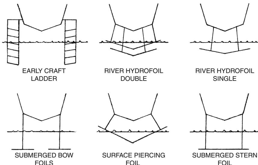
Fig. 5.7 Hydrofoil configurations
