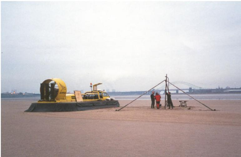
Fig. 2.42 G2000TD seismic survey on tidal sandbank, preparing a shot
