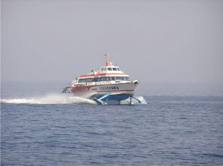
**Fig. 1.12** Surface piercing hydrofoil
