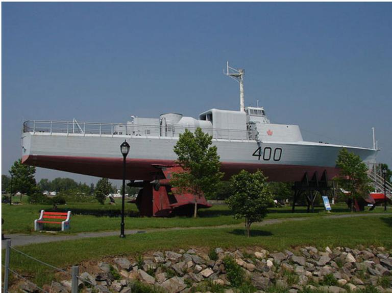
**Fig. 5.10** Single main lifting foil configuration—Bras D'Or
