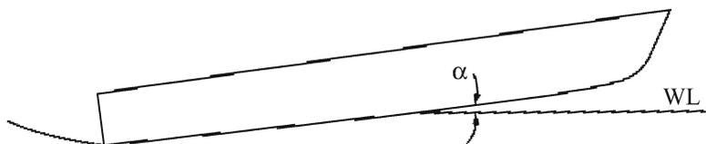
Fig. 4.5 Planing hull without steps
