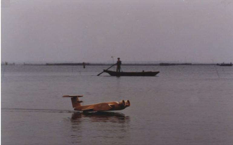
**Fig. 3.27** Free flight model of DACWIG “Swan”
