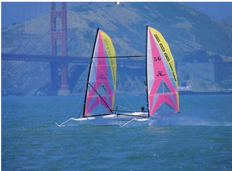
**Fig. 1.1** High-speed sailing hydrofoil trimaran
