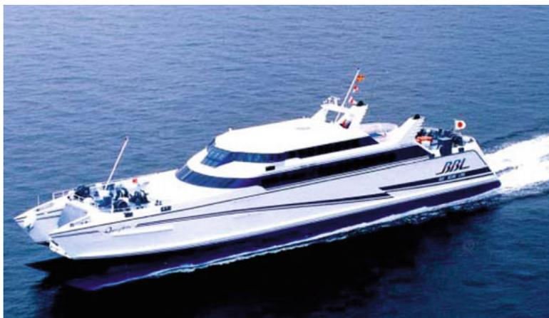
Fig. 6.32 Super Slender Twin Hull Ferry "Ocean Arrow"
