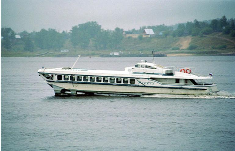
**Fig. 5.5** Alexeev Raketa hydrofoil
