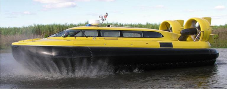
**Fig. 2.67** Airlift hovercraft P34 hovering static over water
