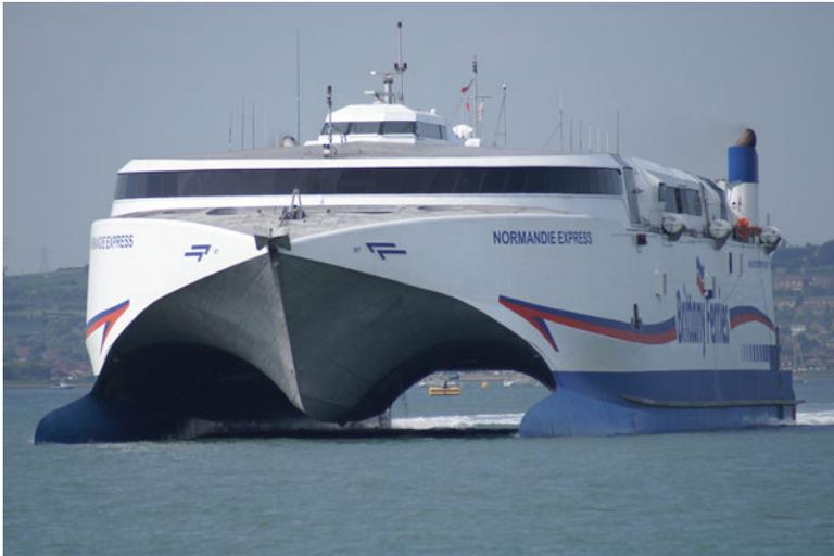
**Fig. 8.9** WPC cross channel operation
