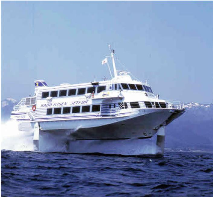
**Fig. 1.13** Fully submerged hydrofoil
