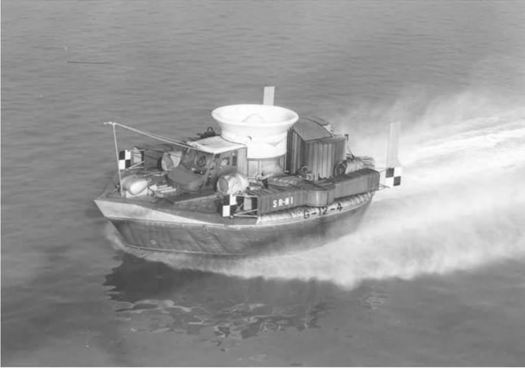
**Fig. 2.4** SR-N1 deep skirt and jet propulsion
