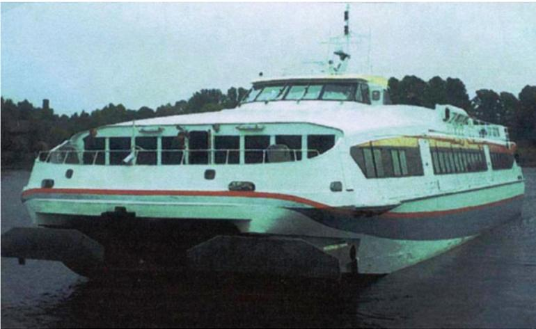
Fig. 7.10 Foils retracted front view
