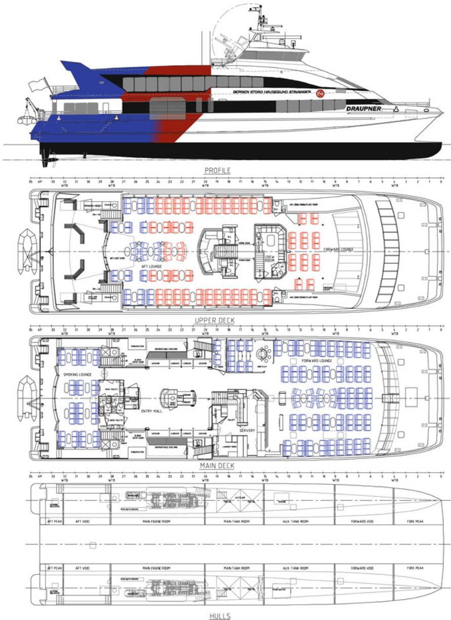
Fig. 6.4 General arrangement of a catamaran Passenger Ferry, Austal 42 m delivered 1999
