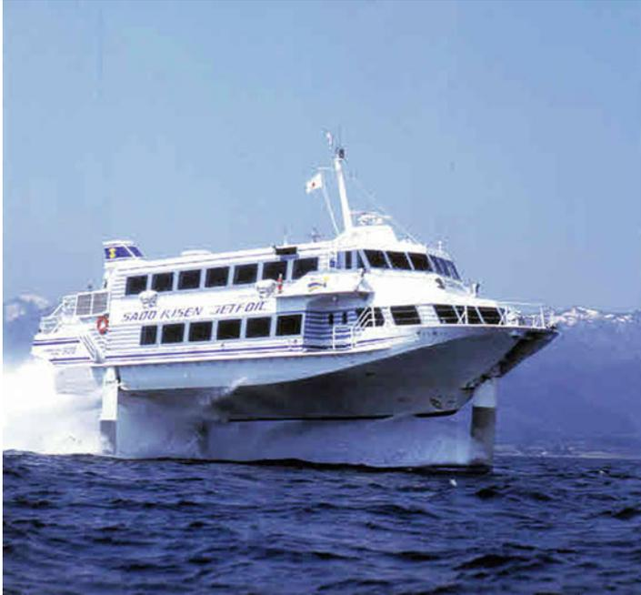
**Fig. 1.13** Fully submerged hydrofoil
