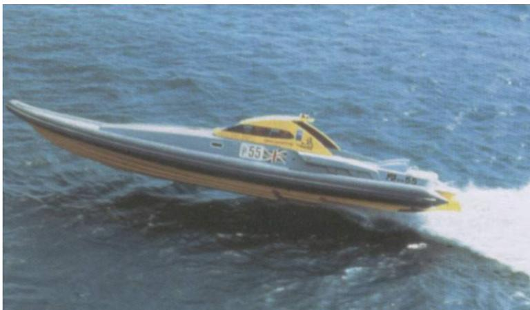
**Fig. 4.9** Stepped hull craft at high speed
