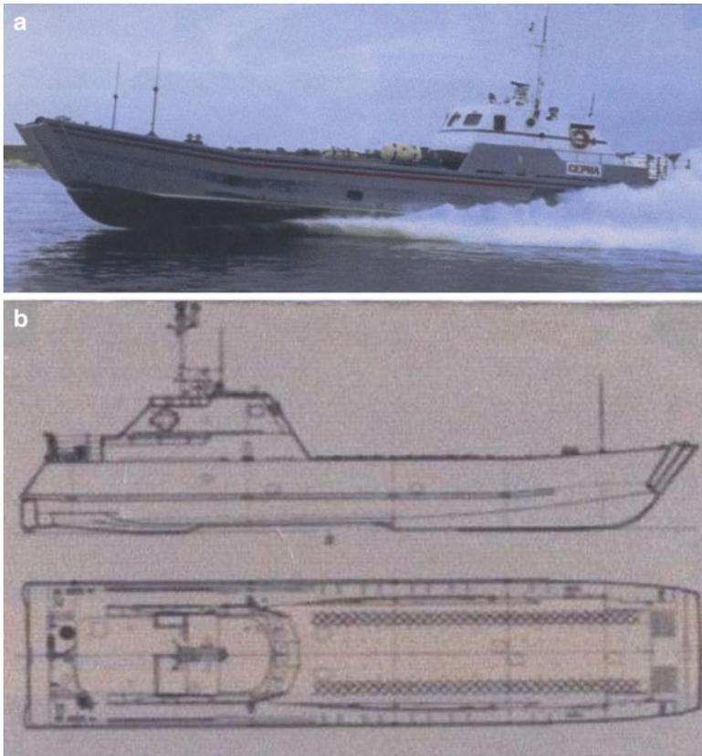
**Fig. 7.5** (a) ACC landing craft. (b) General arrangement
