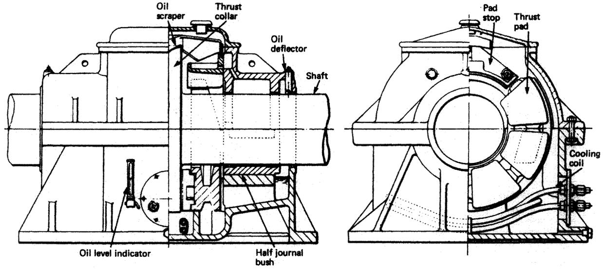
Figure 11.2 Thrust block
