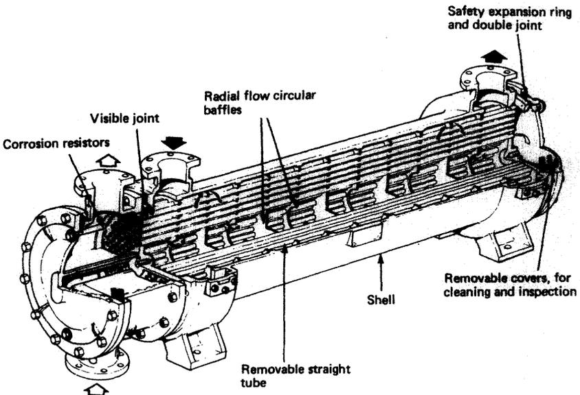
Figure 7.4 Shell and tube heat exchanger
