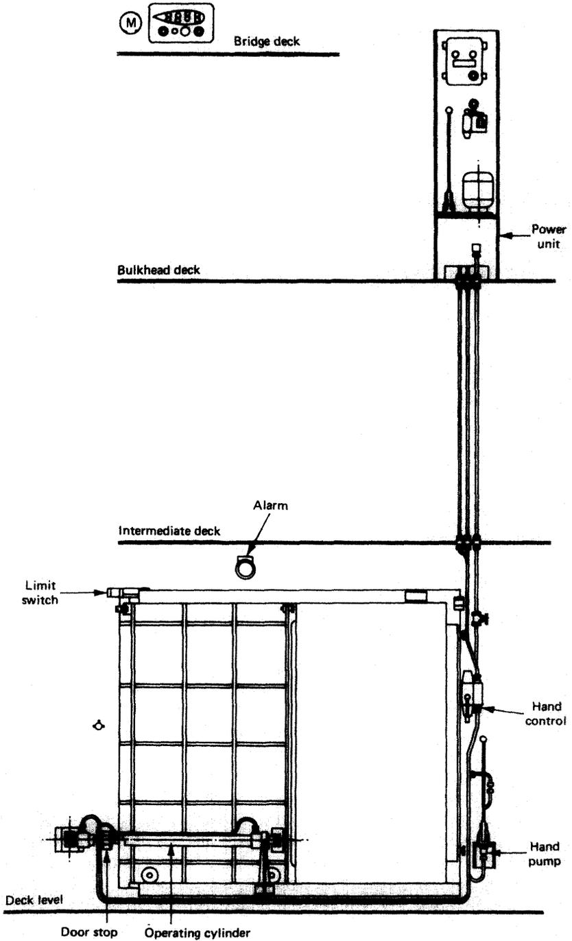
Figure 10.9 Horizontal sliding watertight door
