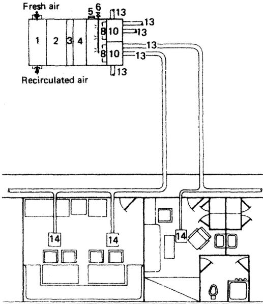
Figure 9.10 Single-duct system
