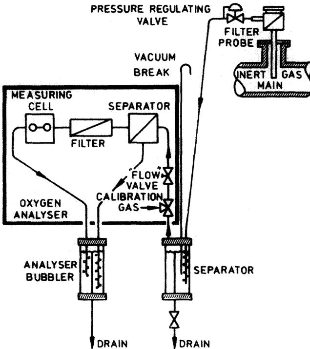
Figure 15.22 Oxygen analyser
