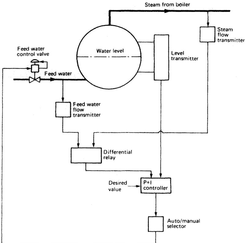
Figure 15.36 Boiler water level control
