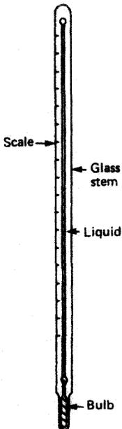
Figure 15.6 Liquid-in-glass thermometer
