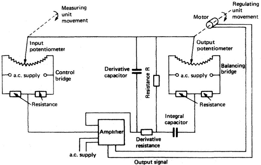
**Figure 15.33** Electronic three-term controller
