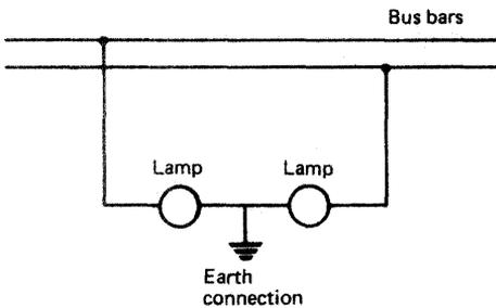
Figure 14.3 Earth lamp circuit
