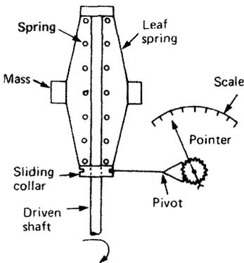
Figure 15.15 Mechanical tachometer
