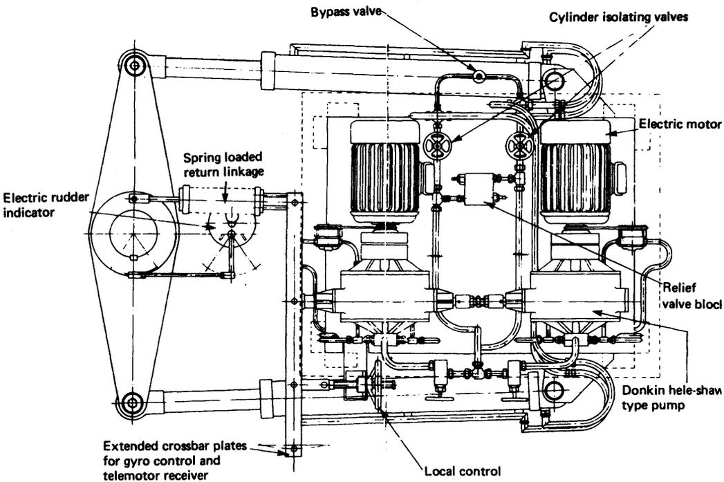
Figure 12.6(b) Actual arrangement of two-ram steering gear
