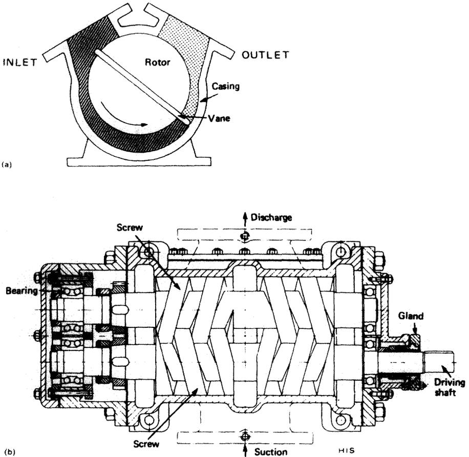
**Figure 6.4** Rotary displacement pumps: (a) rotary vane displacement pump, (b) screw displacement pump
