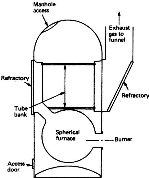
Figure 4.8 Cochran spheroid boiler
