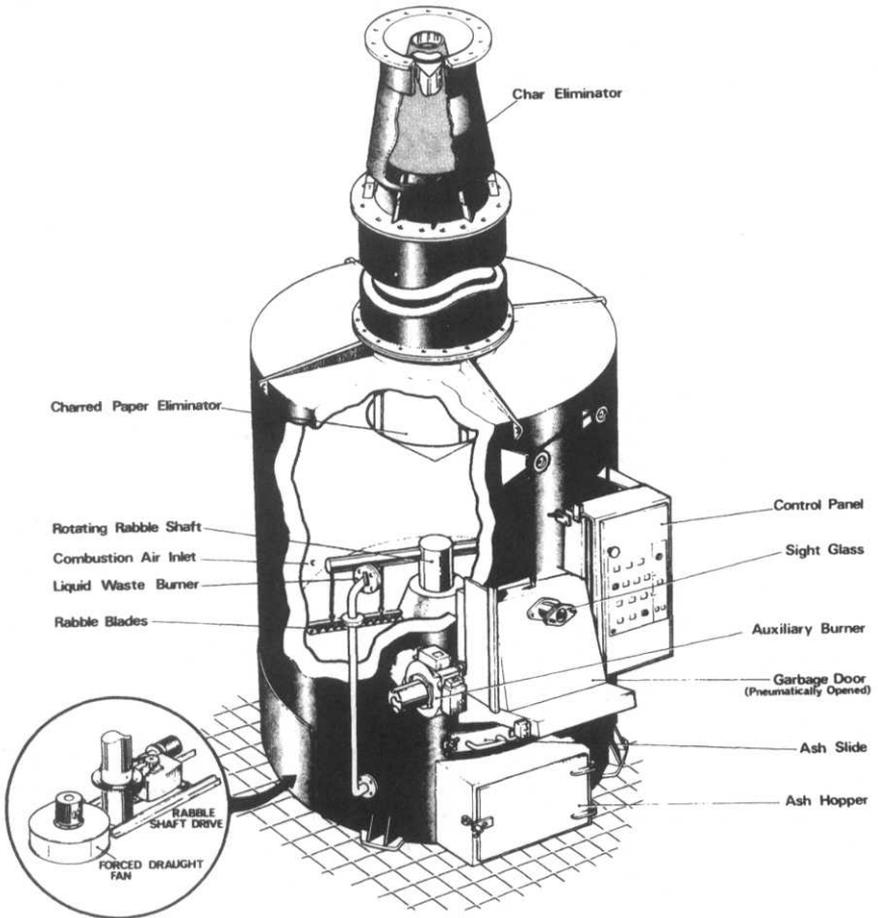
**Figure 7.11** Incinerator
