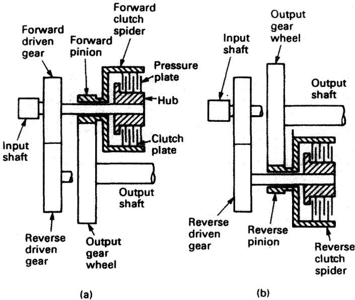
Figure 2.26 Plate-type clutch
