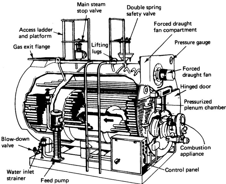
Figure 4.7 Package boiler
