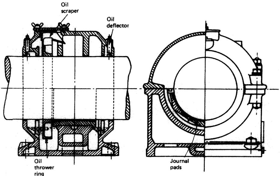
Figure 11.3 Tunnel bearing
