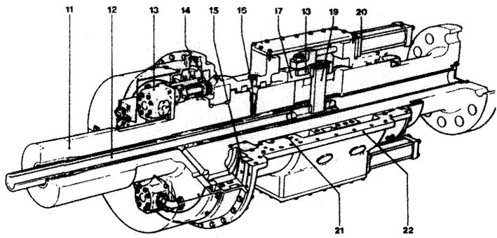
**Figure 11.7** Controllable-pitch propeller
