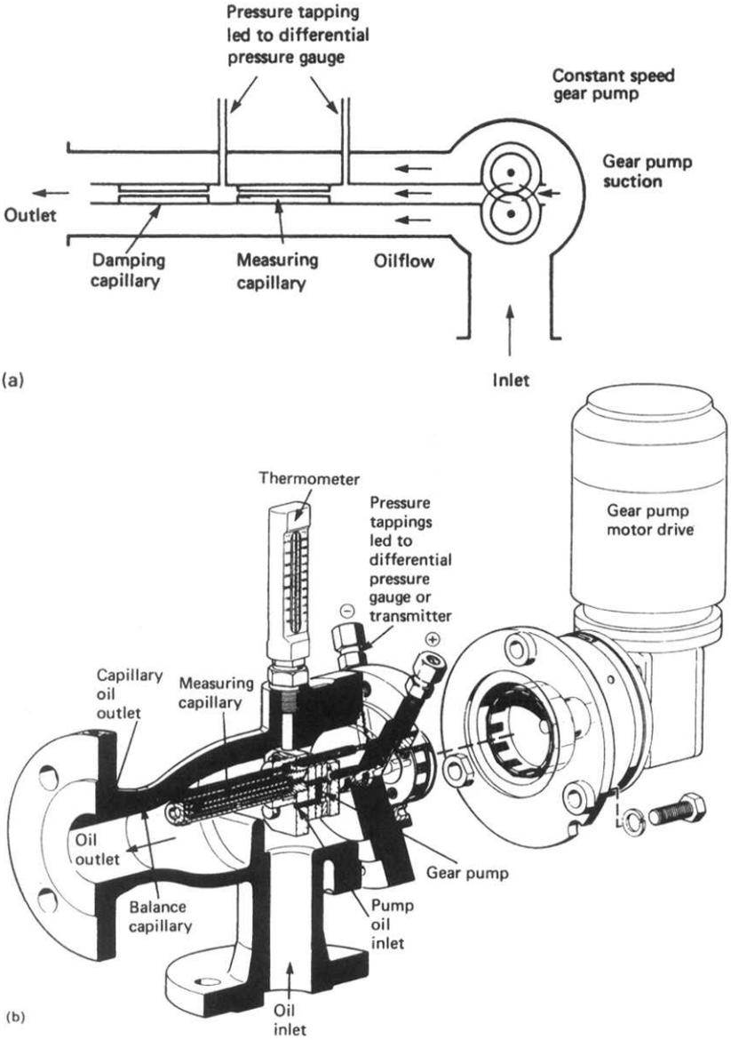
**Figure 15.20** Viscosity sensor, (a) diagrammatic; (b) actual
