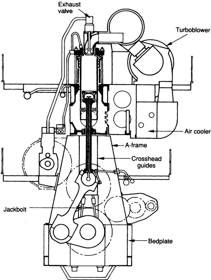
Figure 2.28 Sulzer RTA72U engine
