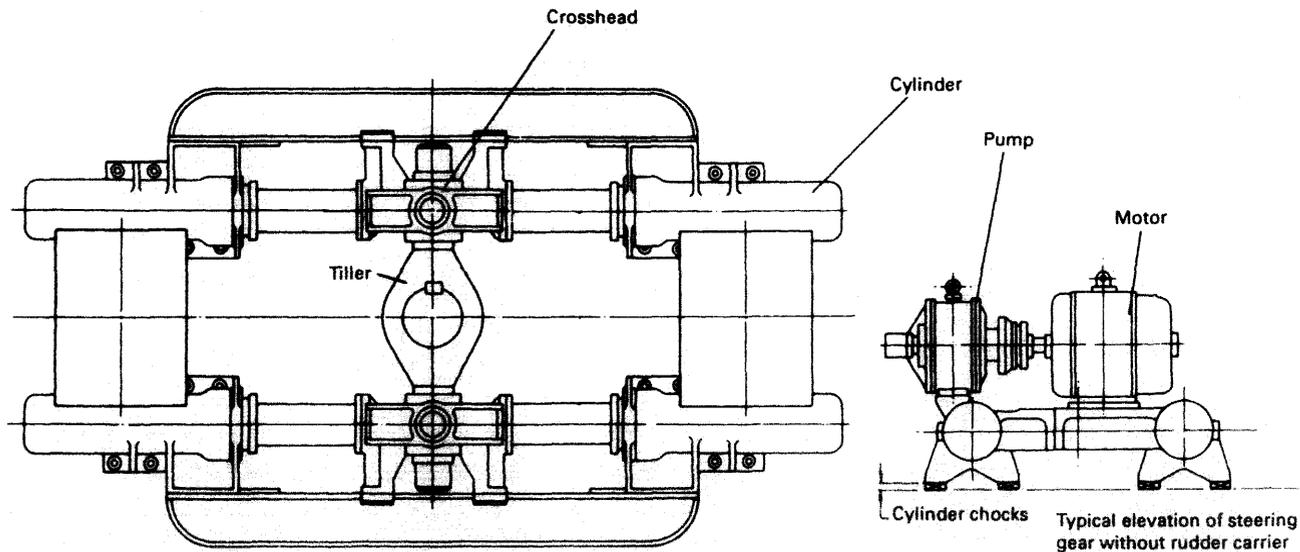
Figure 12.7 Four-ram steering gear—actual arrangement
