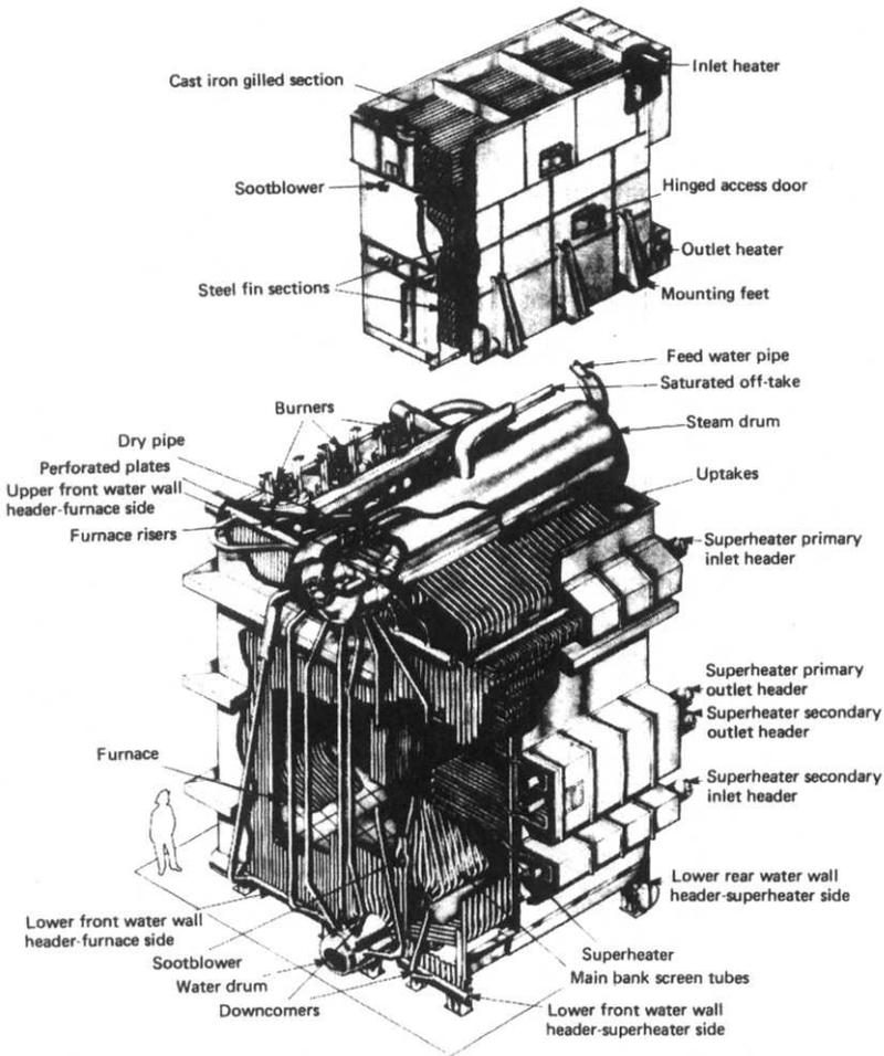
**Figure 4.4** Foster Wheeler Type ESD III monowall boiler
