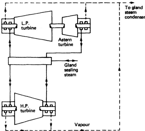
Figure 3.9 Gland steam sealing system
