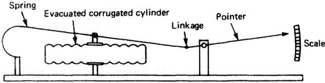
**Figure 15.3** Aneroid barometer
