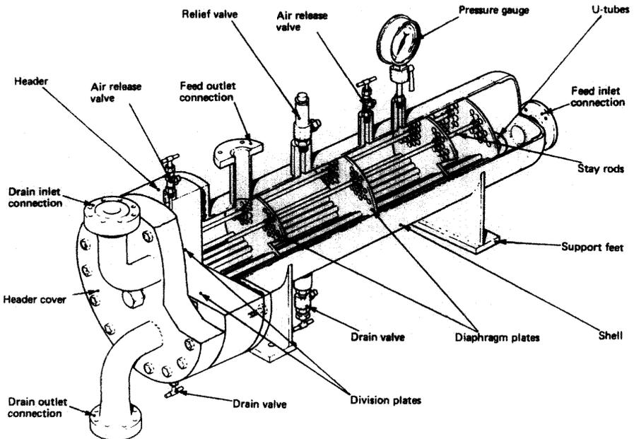
**Figure 5.8** Drains cooler
