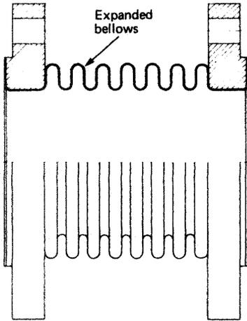
Figure 6.18 Expansion bellows piece
