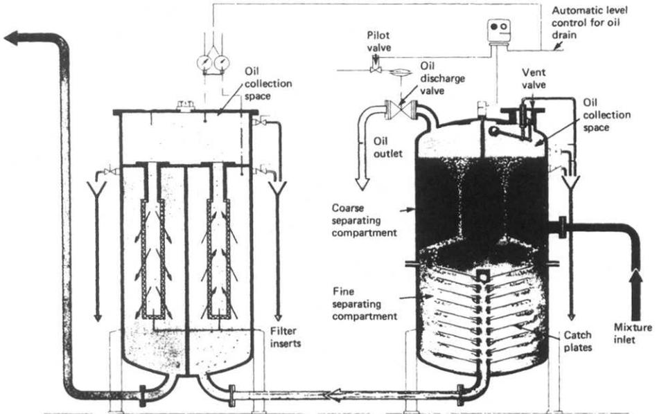
**Figure 7.8** Oily water separator
