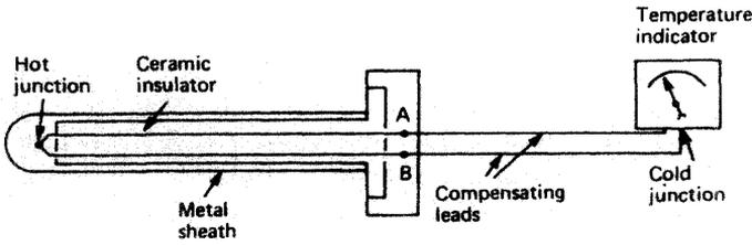
Figure 15.8 Thermocouple
