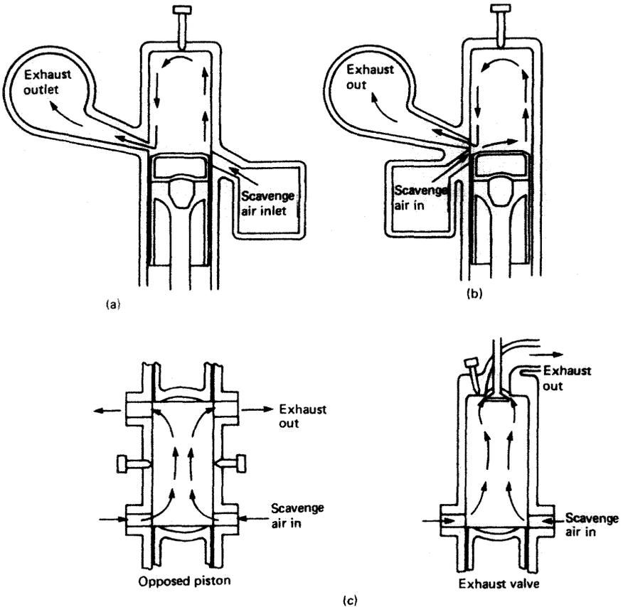
**Figure 2.10** Scavenging methods. (a) Cross-flow scavenging, (b) loop scavenging, (c) uniflow scavenging
