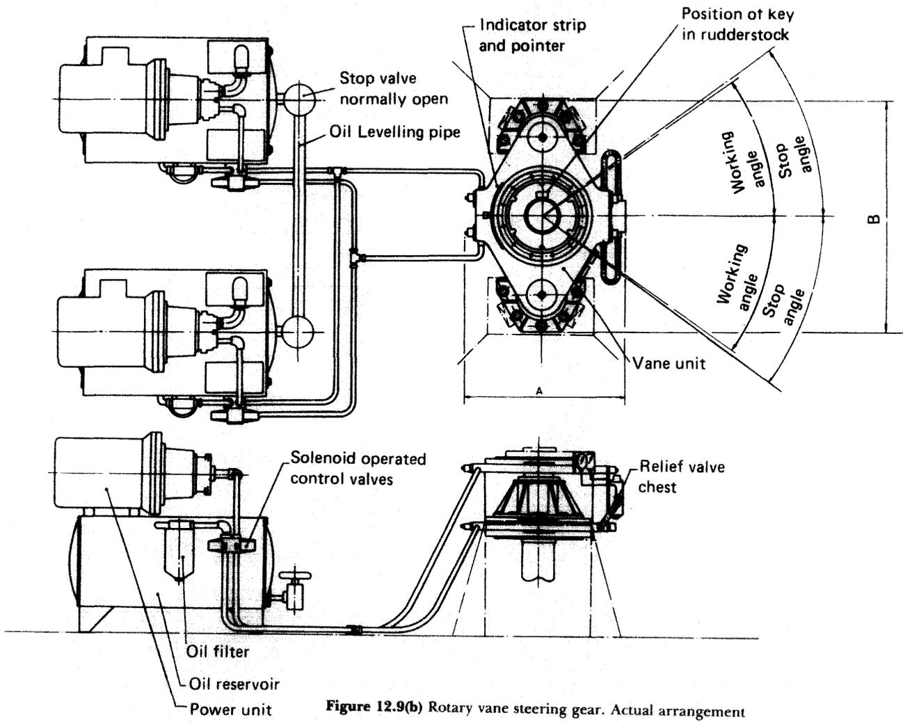
Figure 12.9(b) Rotary vane steering gear. Actual arrangement
