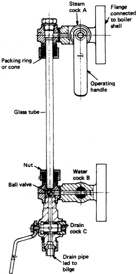
**Figure 4.11** Tubular gauge glass
