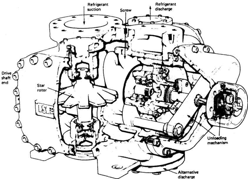
Figure 9.3 Single-screw compressor
