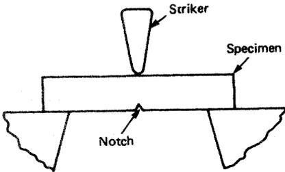
Figure 16.3 Impact test
