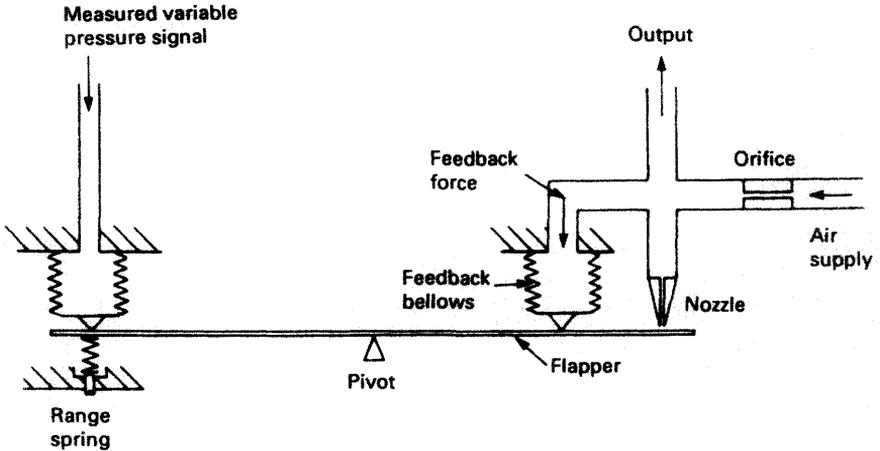
Figure 15.26 Force balance transmitter with feedback
