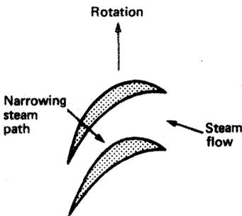
Figure 3.3 Reaction blading
