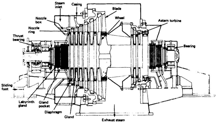
Figure 3.5 Impulse turbine
