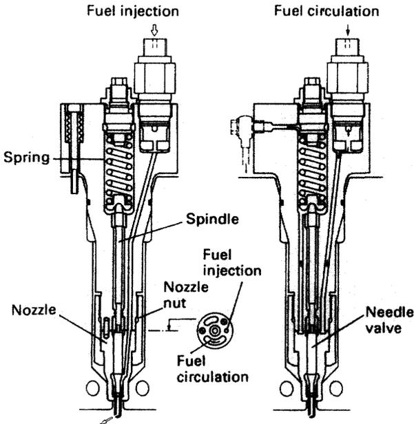
Figure 2.16 Fuel injector
