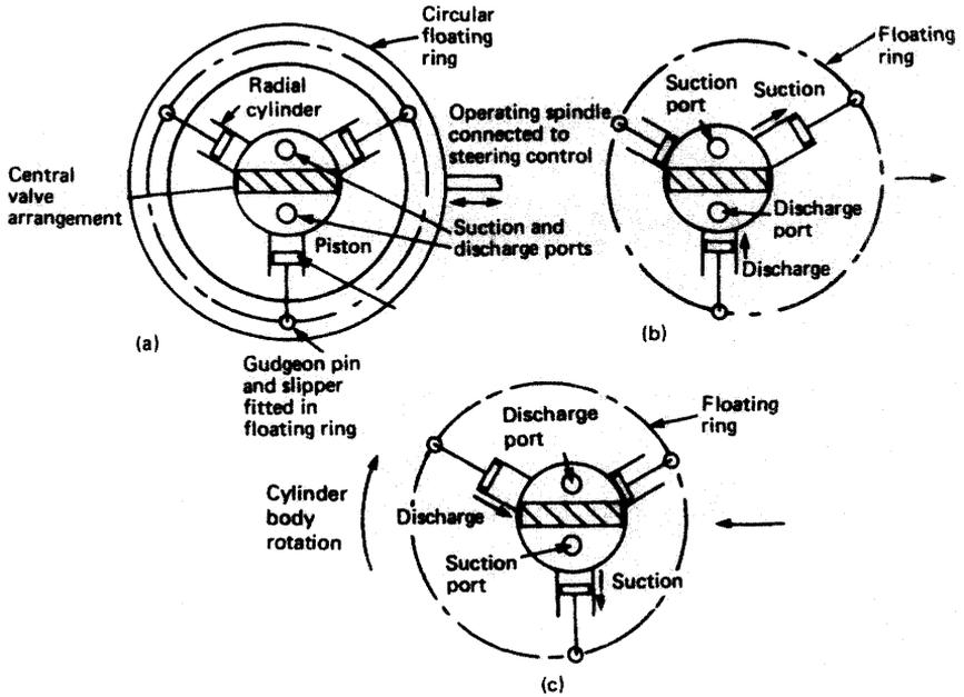
**Figure 12.2** Hele-Shaw pump—operating principle
