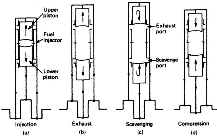
Figure 2.5 Opposed piston engine cycle
