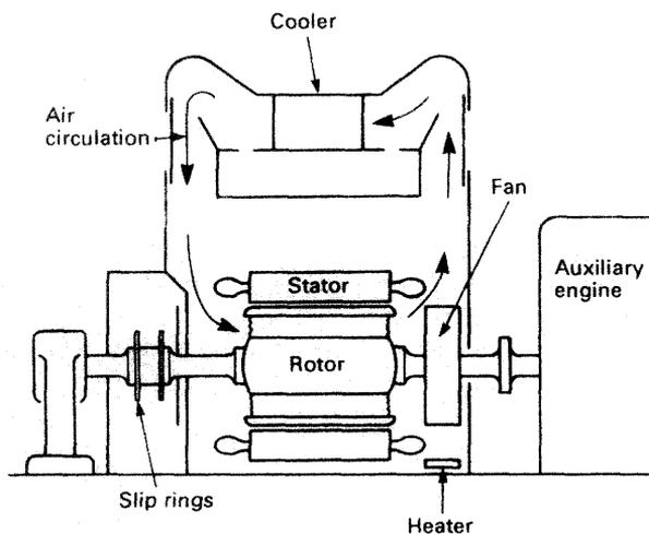
Figure 14.7 Alternator construction
