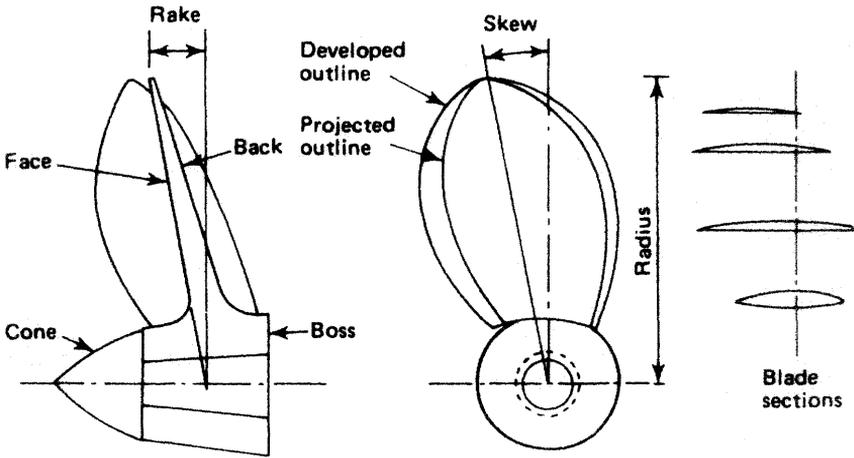
Figure 11.5 Solid propeller
