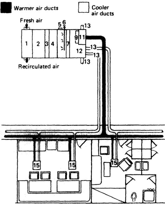
Figure 9.11 Twin-duct system
