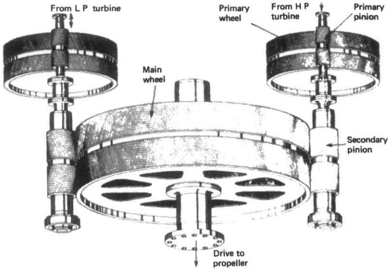
Figure 3.14 Double reduction system of gearing
