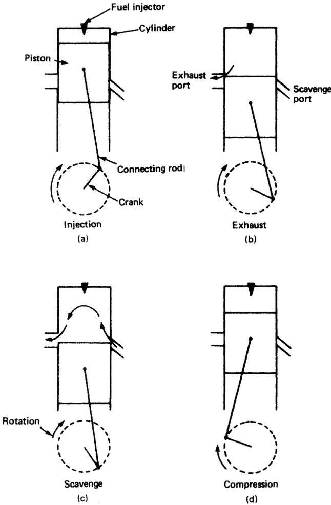
**Figure 2.3** Two-stroke cycle
