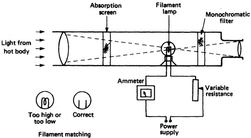
Figure 15.9 Optical pyrometer
