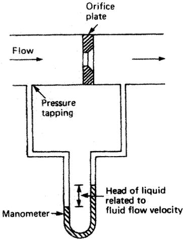
Figure 15.13 Orifice plate
