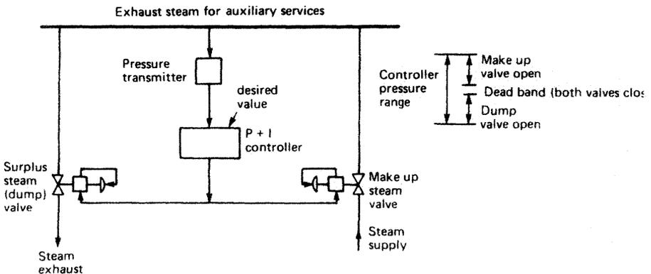
Figure 15.37 Exhaust steam pressure control
