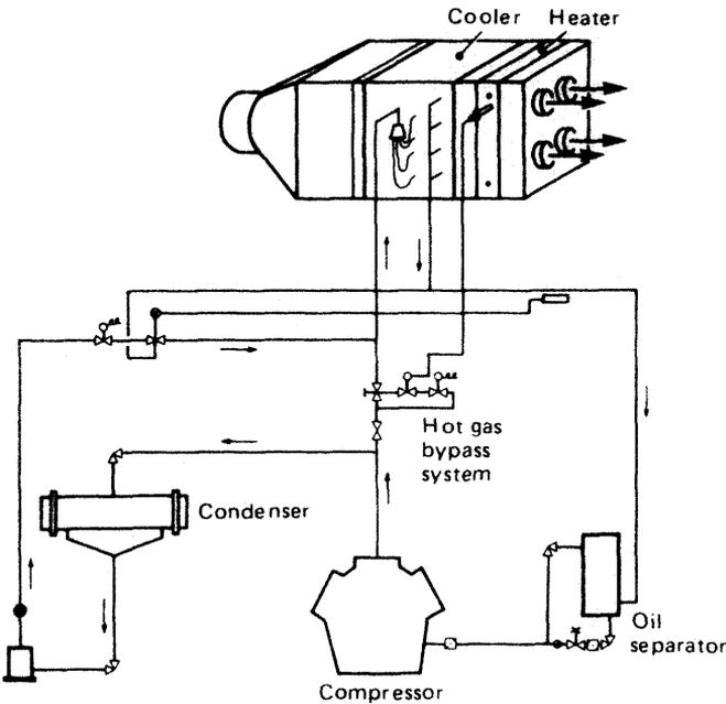
**Figure 9.12** Direct-expansion refrigeration system for an air cooler
