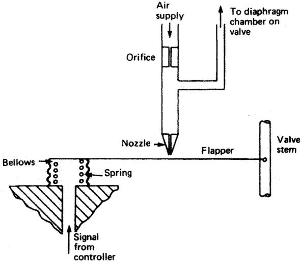
Figure 15.35 Valve positioner
