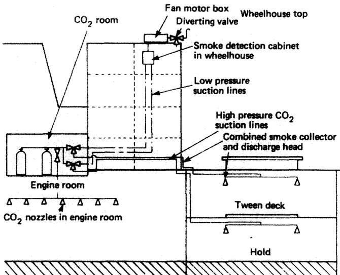
Figure 13.12 Carbon dioxide detection and flooding system
