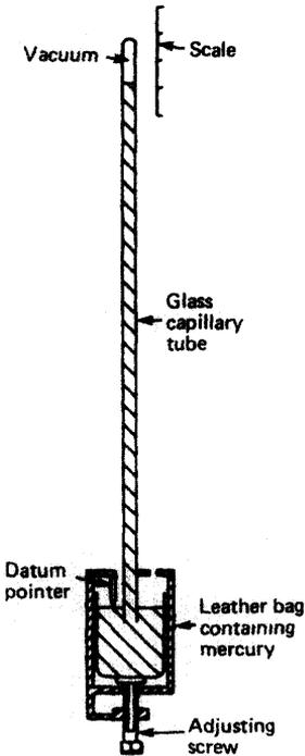
**Figure 15.2** Mercury barometer
