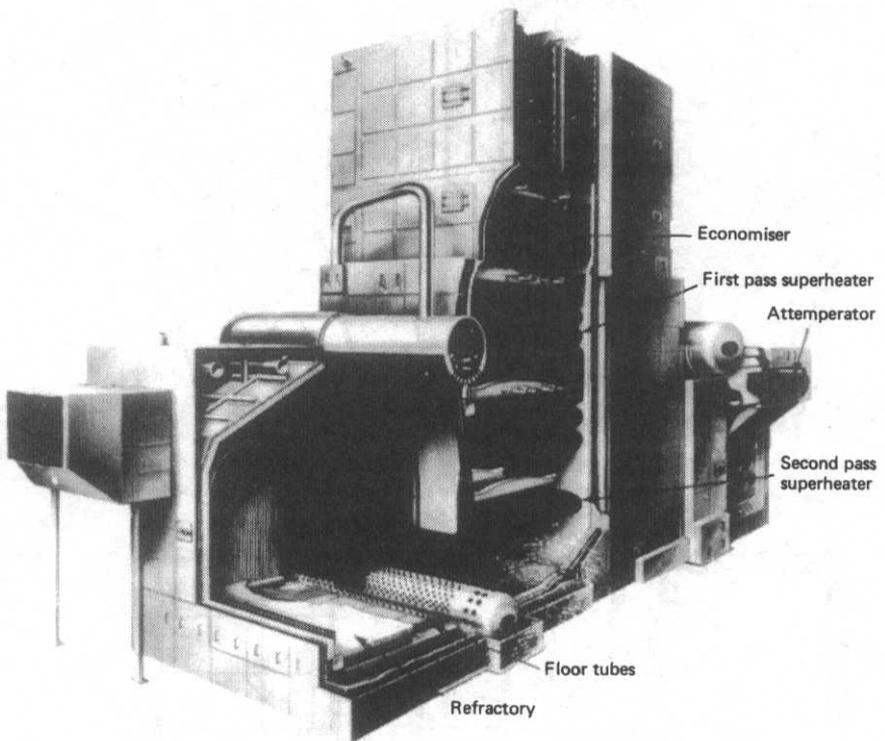
**Figure 4.3** Foster Wheeler Type ESD I boiler
