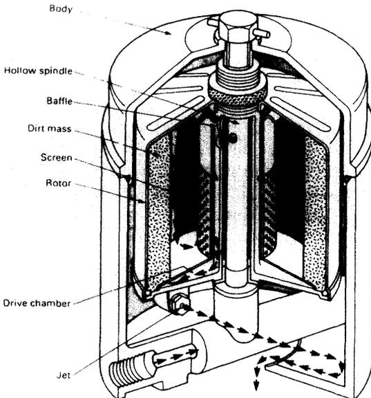
Figure 8.6 Centrifugal filter
