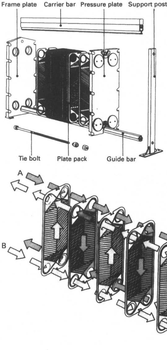
**Figure 7.5** Plate-type heat exchanger: (a) construction, (b) operation
