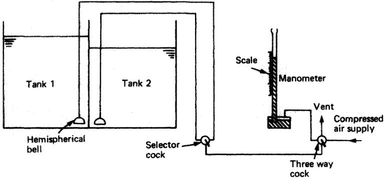
Figure 15.10 Pneumatic gauge
