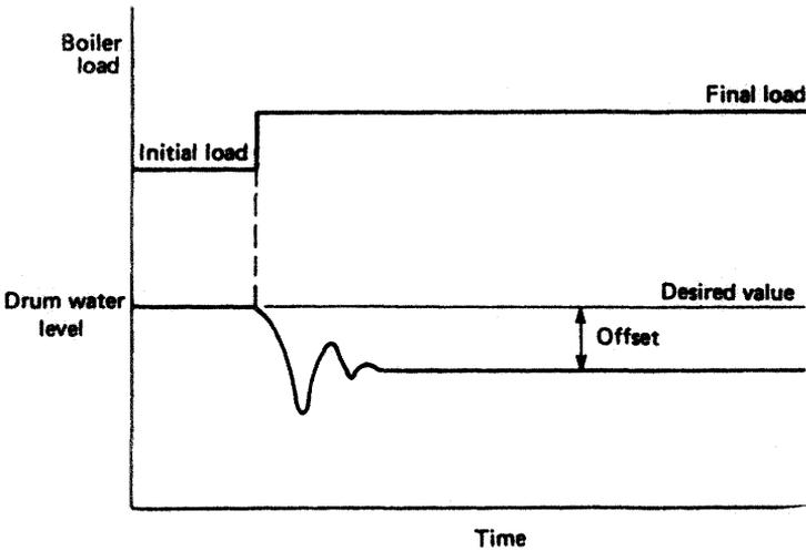
Figure 15.30 System response to proportional controller action
