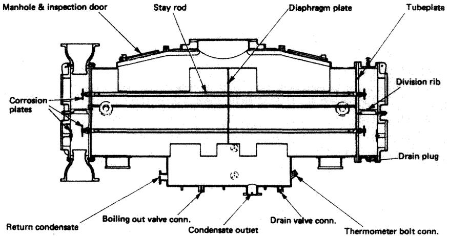
**Figure 5.5** Auxiliary condenser
