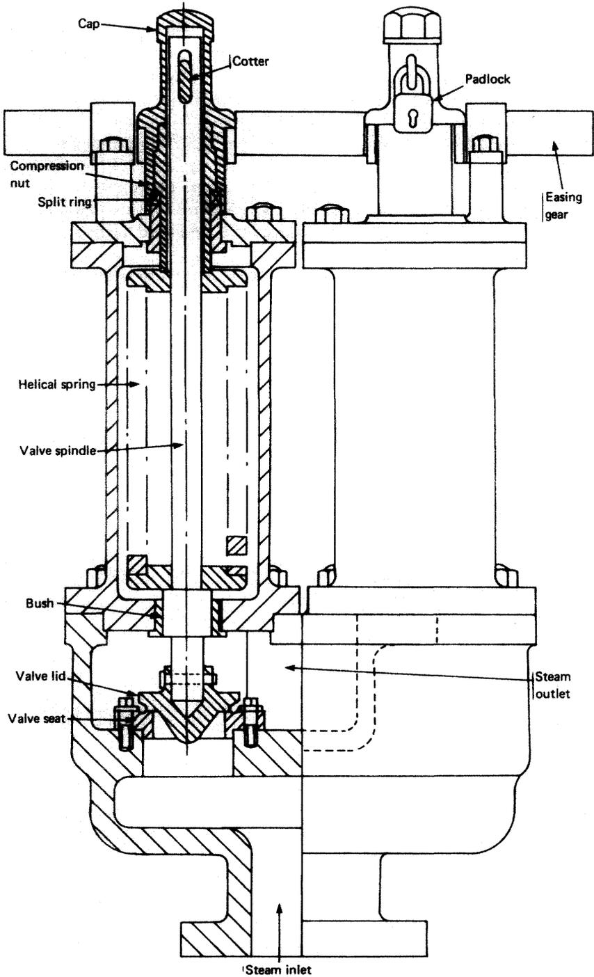
Figure 4.13 Ordinary spring-loaded safety valve
