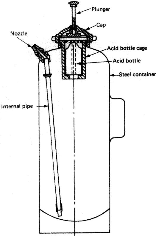
**Figure 13.4** Soda-acid extinguisher
