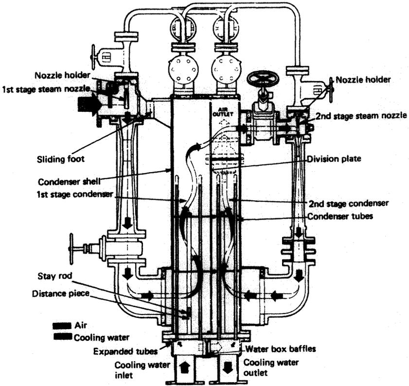
Figure 5.7 Air ejector
