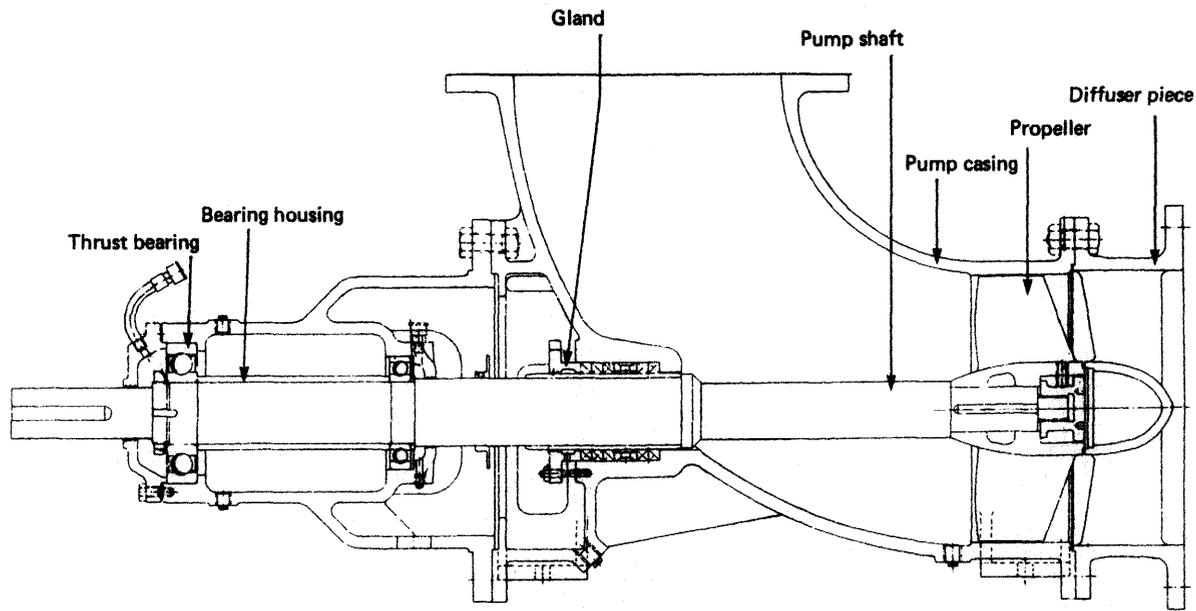
Figure 6.5 Axial-flow pump
