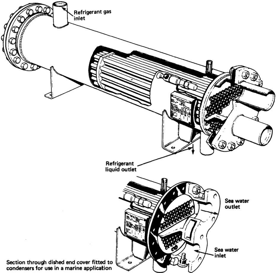
Section through dished end cover fitted to condensers for use in a marine application
