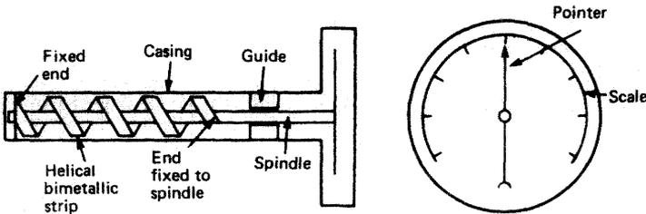
Figure 15.7 Bimetallic strip thermometer
