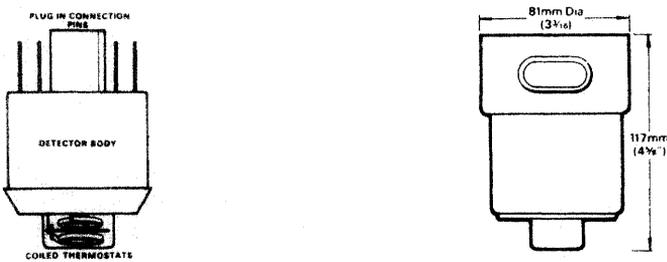
Figure 13.3 Heat detector
