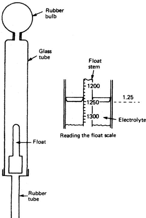
Figure 14.13 Syringe-type hydrometer
