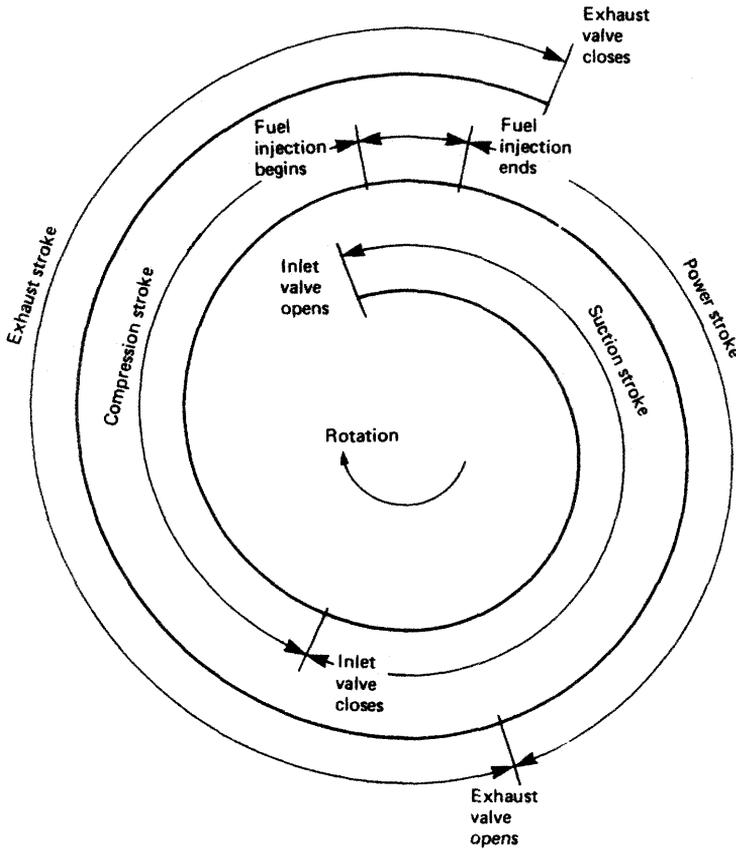
Figure 2.2 Four-stroke timing diagram
