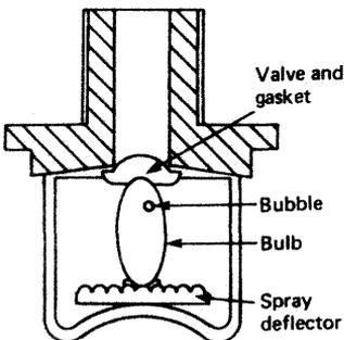
**Figure 13.9** Sprinkler head
