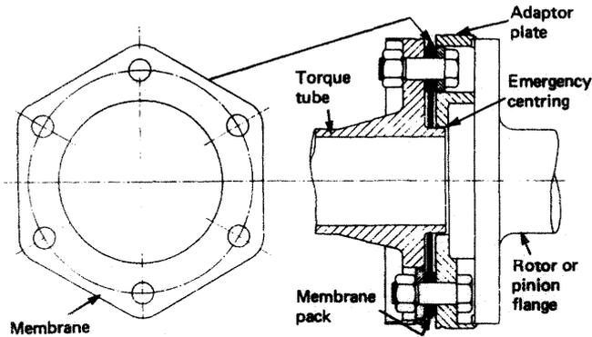
Figure 3.15 Flexible coupling
