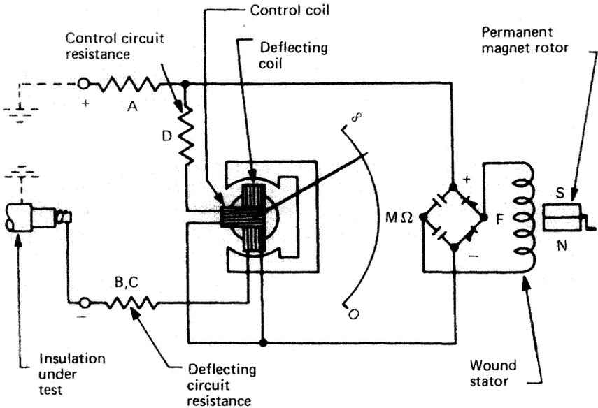
**Figure 14.16** Insulation tester
