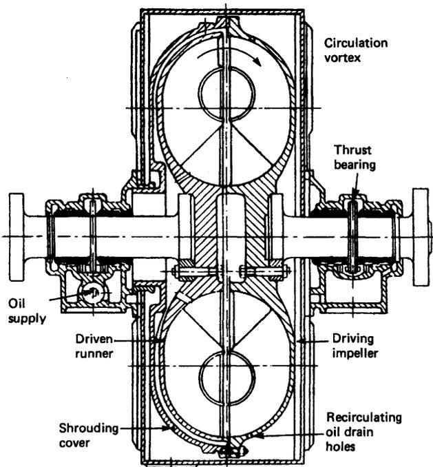
**Figure 2.25** Hydraulic coupling
