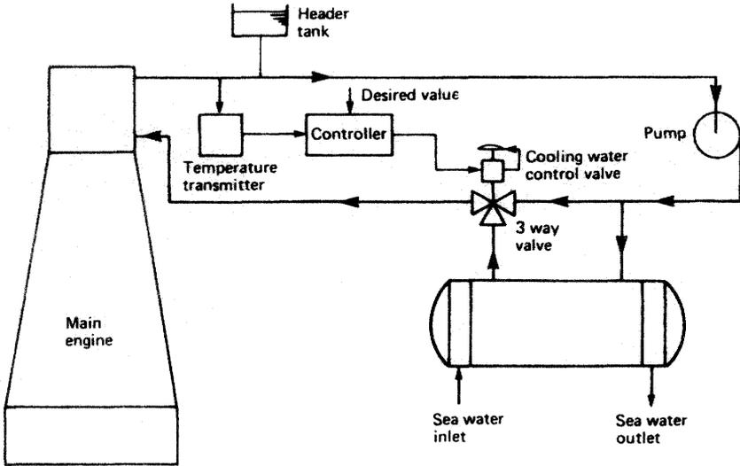
Figure 15.41 Cooling water temperature control
