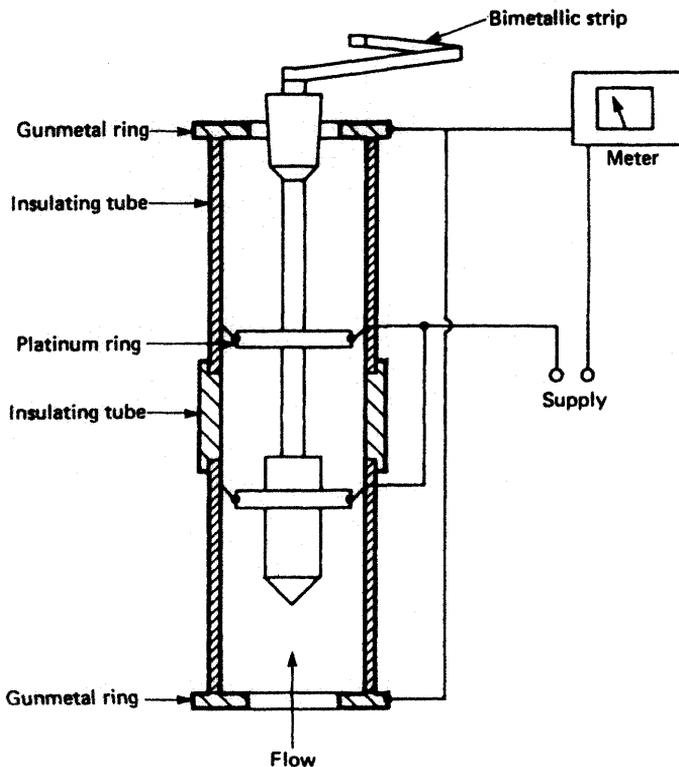
Figure 15.21 Salinometer
