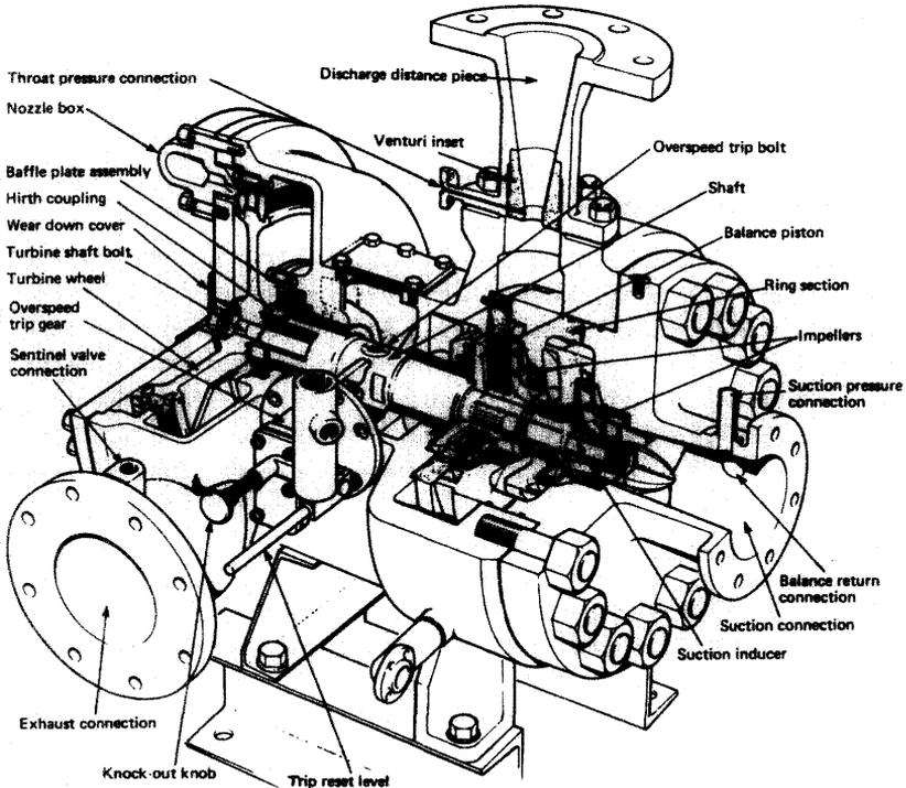
Figure 5.10 Turbo-feed pump
