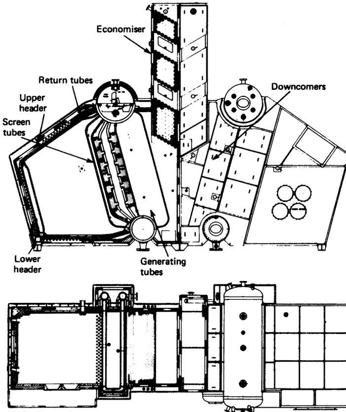
Figure 4.2 Foster Wheeler D-Type boiler
