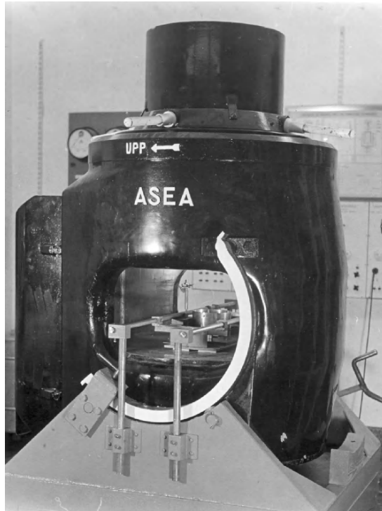
Fig. 1. The electromagnet at Alfvén's Department of Electronics at the Royal Institute of Technology in Stockholm. An almost homogeneous magnetic field up to about 1 T can be generated in the gap. The experimental arrangement is placed on a fixed stand. The magnet can be turned around a horizontal axis, such as to generate a magnetic field which forms any angle with the vertical direction
