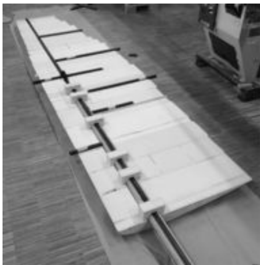
Figure 4. Wing under construction with internal tubing and other fasteners visible.
