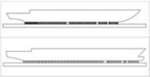
Figure 7. Keel block distribution of the prospective ship. The hullform is modified for publishing.
