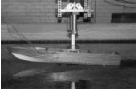
Figure 6. The wooden model, denominated M20, used in the towing tests.
