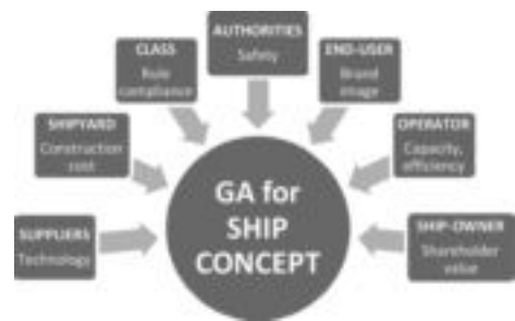
Figure 1. GA requirements and different stakeholders that have a major influence on the ship concept development and their dominant viewpoints. The naval architect confirms that all relevant requirements are considered in the ship concept.
