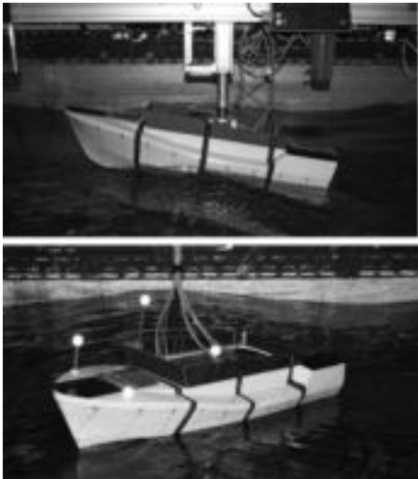
Figure 10. Experiments setup. Model towed by a carriage for tests at forward speed (top). Model constrained by mooring lines for tests at zero speed (bottom).
