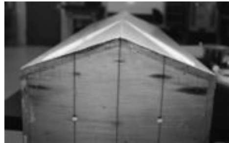
Figure 8. The add-on deflectors applied on the hull of the M20 model, view from behind to highlight their tapered design.
