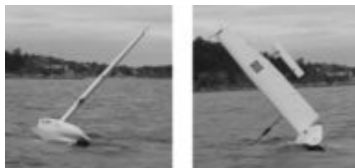
Figure 20. Pictures of the boat at two extreme heel angles during the same instance of exaggerated roll.
