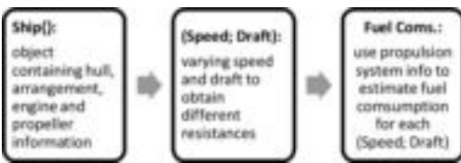
Figure 9. Basic fuel consumption calculation based on a Ship{} , varying speed and draft to calculate resistance and consequently fuel consumption.
