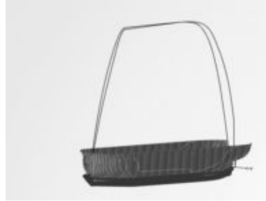
Picture 1. Finalized hullform after Lackenby variation.
