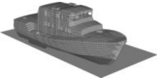
Figure 4. Finite Element (FE) global model of the Severn Class lifeboat.
