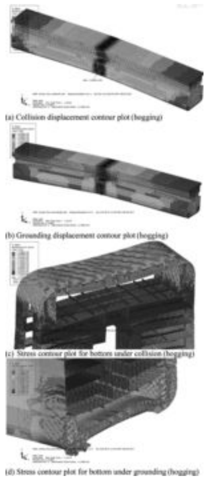
Figure 5. Displacement and stress contour of damaged condition (hogging).
