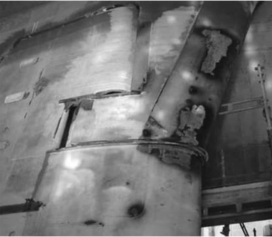
**Figure 9.39** Example of rudder erosion
