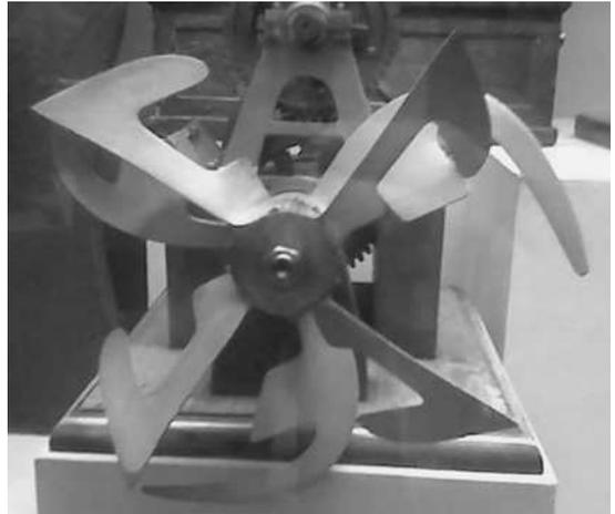
**Figure 1.11** de Bay's contra-rotating propeller design
