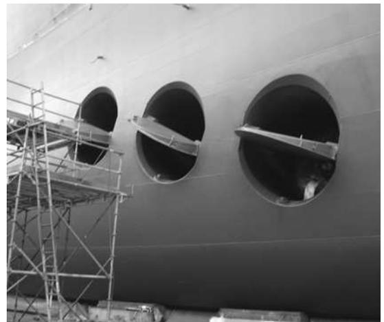
**Figure 14.13** Doors fitted to a set transverse propulsion unit openings
