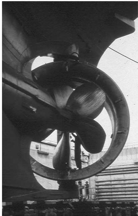
**Figure 2.5** Steerable ducted propeller
