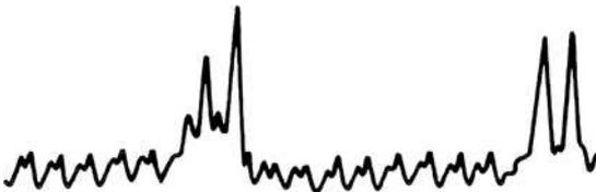
**Figure 23.7** Typical hull pressure fluctuation indicating possible presence of PHV cavitation
