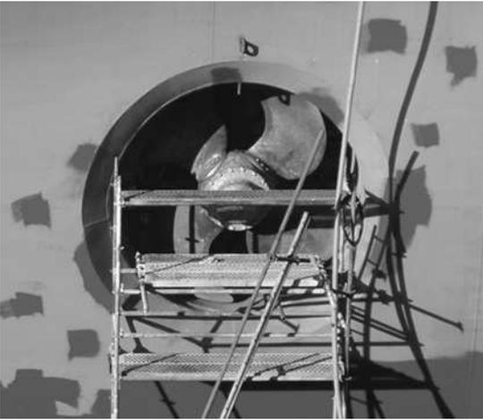
**Figure 14.14** Use of skew with transverse propulsion unit blades
