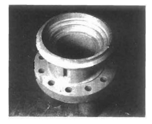
Figure 16.142 Replicast 8-inch ball valve body after shake-out from the mould and fine shot-blasting
