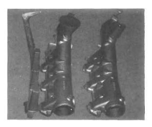
Figure 16.133 Sand cast aluminium alloy inlet manfold. The casting on the left requires a 3 kg running system and a 2 kg riser. On the right the same casting passed through a Dypur unit has a 1 kg riser and needs no running system
