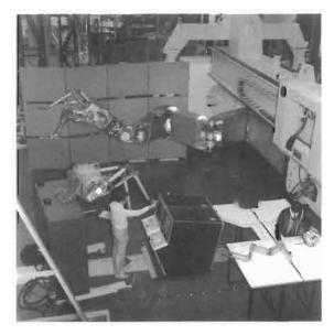
Figure 13.7 Remote manipulator for JET fusion experiment (courtesy JET Joint Undertaking)
