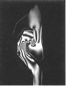
Figure 8.36 Fringe pattern for a tension coupling in a sodium light source (by permission of Sharples Stress Consultants)
