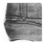
Figure 7.36 Example of 'weld decay' in an austenitic steel
