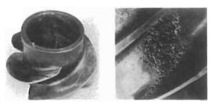
Figure 7.128 Cavitation damage on a disposable stainless steel feed pump inducer. (a) Inducer; (b) cavitation damage
