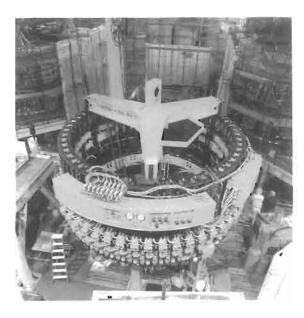
Figure 13.5 Pressure vessel stud tensioner
