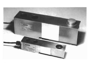
Figure 3.58 Photograph of load cells (courtesy Defiant Weighing)
