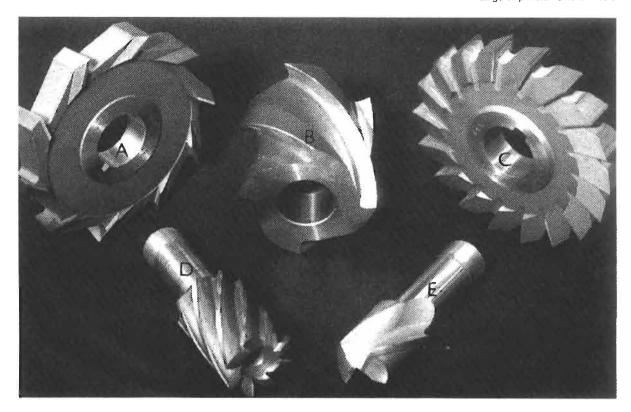
Figure 16.5 Peripheral cutters: (A) high radial rake cutter, (B) helical cutter, (C) side and face cutter, (D) end milling cutter, (E) slot drill
