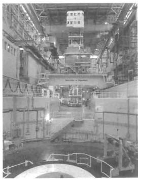
Figure 13.6 AGR refuelling machine at Heysham II Power Station (courtesy Strachan & Henshaw)
