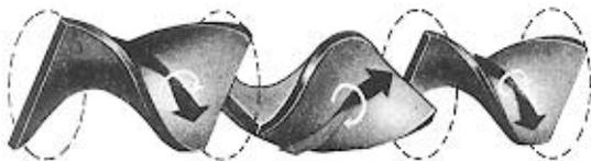
**Figure 8.35** *Twisted-blade type of static mixer elements*
