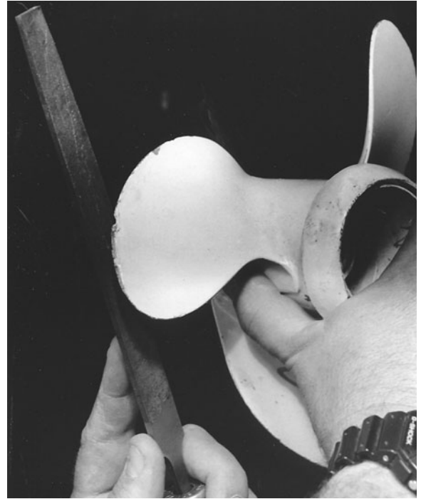
Figure 3-7. Filing out a nick in a propeller.
