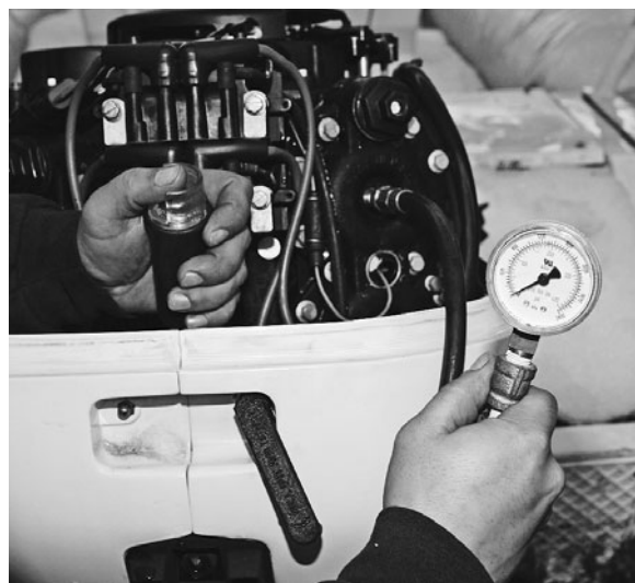
Figure 3-16. A compression test in progress.
