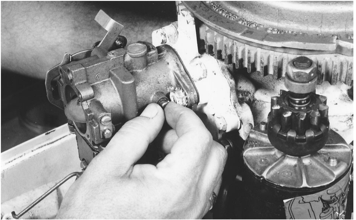
Figure 7-10. Checking for throttle-shaft wear.
