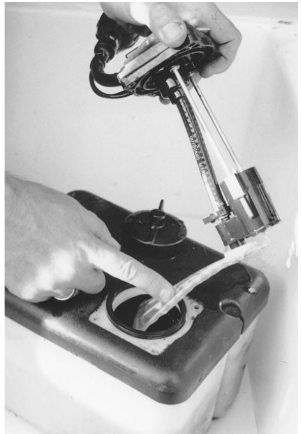
Figure 7-16. Inspecting the oil reservoir filter screen.
