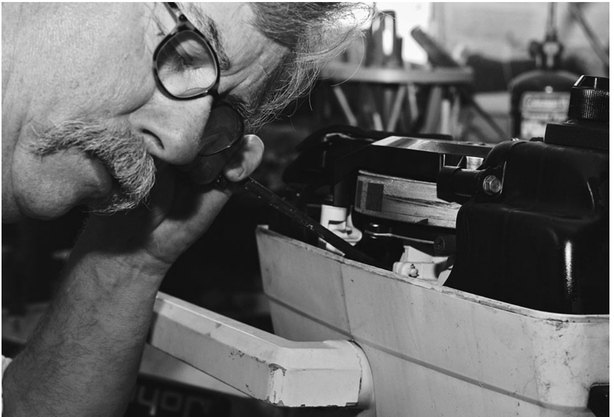
Figure 4-1. Using a screwdriver to pinpoint noises.
