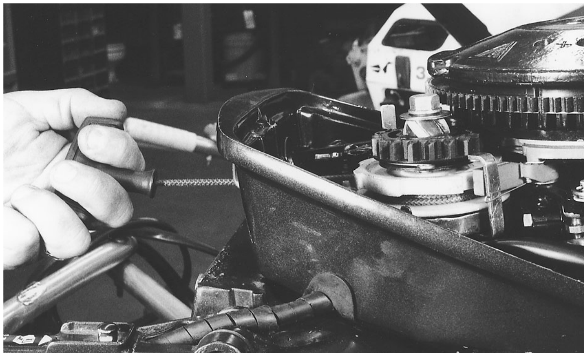
Figure 6-18. Winding on a new pull cord.
