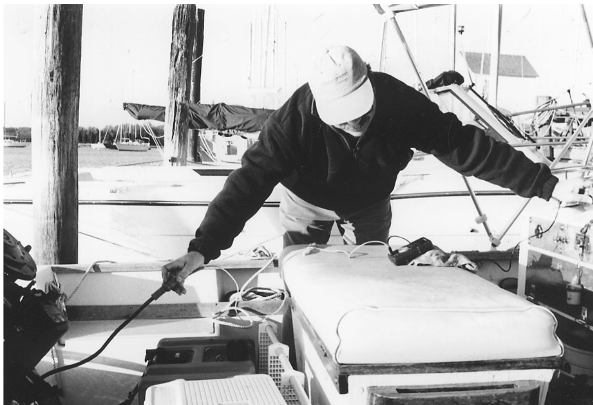
Figure 6-13. Extension harness ohmmeter test.
