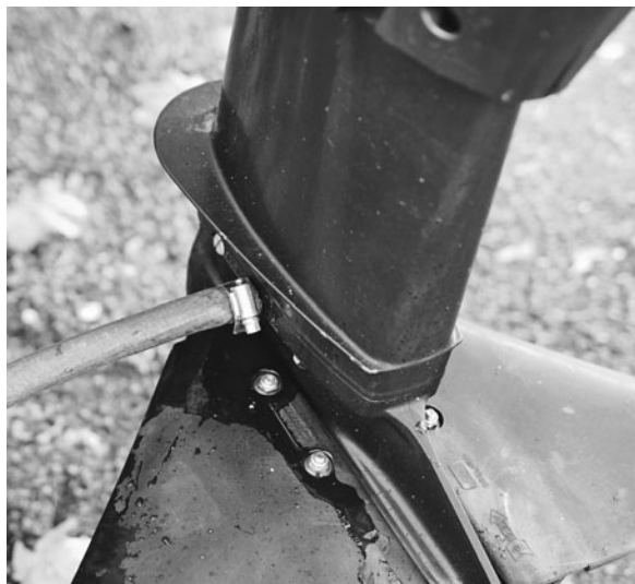
Figure 3-13. Hose attached for flushing the cooling system.
