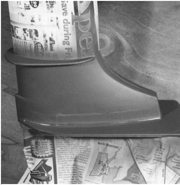
Figure 10-6. The corroded area masked off and ready to spray.
