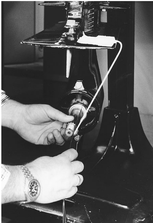
Figure 9-9. Checking for propeller-shaft run-out.
