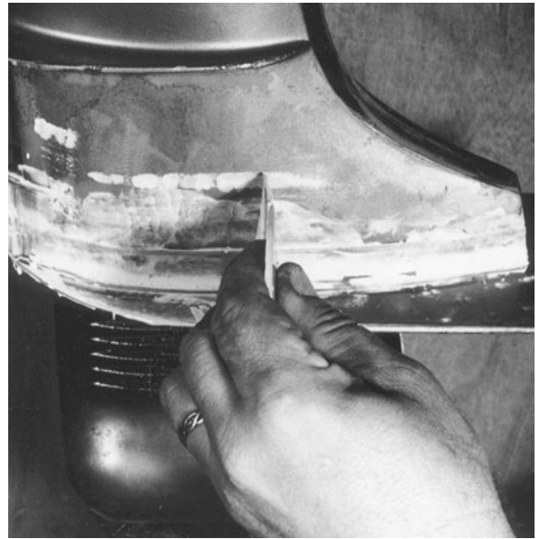
Figure 10-5. Filling corrosion pockets with epoxy putty.
