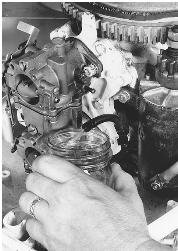
Figure 4-2. Checking that fuel is reaching the carburetor.
