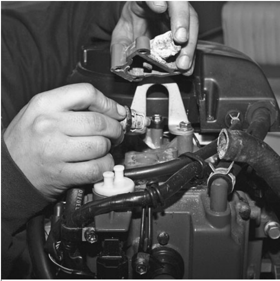
Figure 3-15. Thermostat removed for cleaning and inspection.
