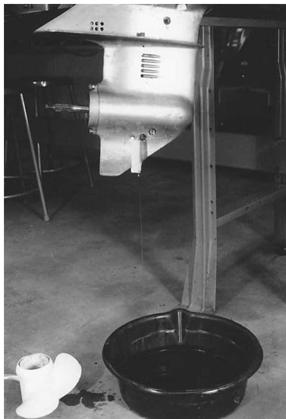
Figure 3-10. Gearcase oil drains down masking tape.
