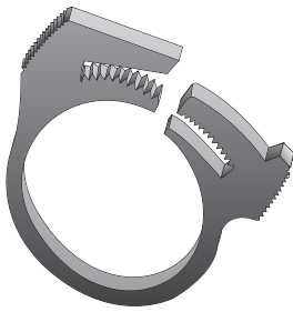
Figure 7-15. A ratchet-style hose clamp.
