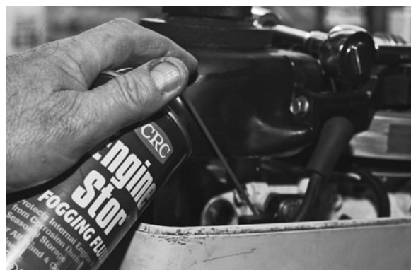
Figure 3-21. Spraying fogging oil into carburetor intake.
