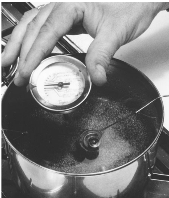
Figure 9-3. Testing a thermostat on the stove top.
