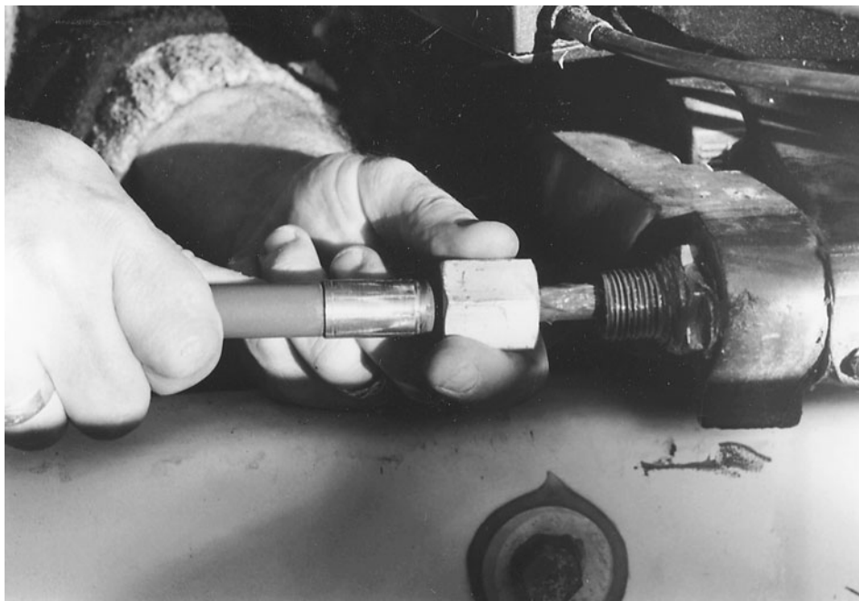
Figure 8-4. Removing a steering cable from the tilt tube.
