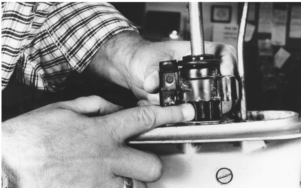
Figure 9-6. Pre-bending the new water pump impeller blades.
