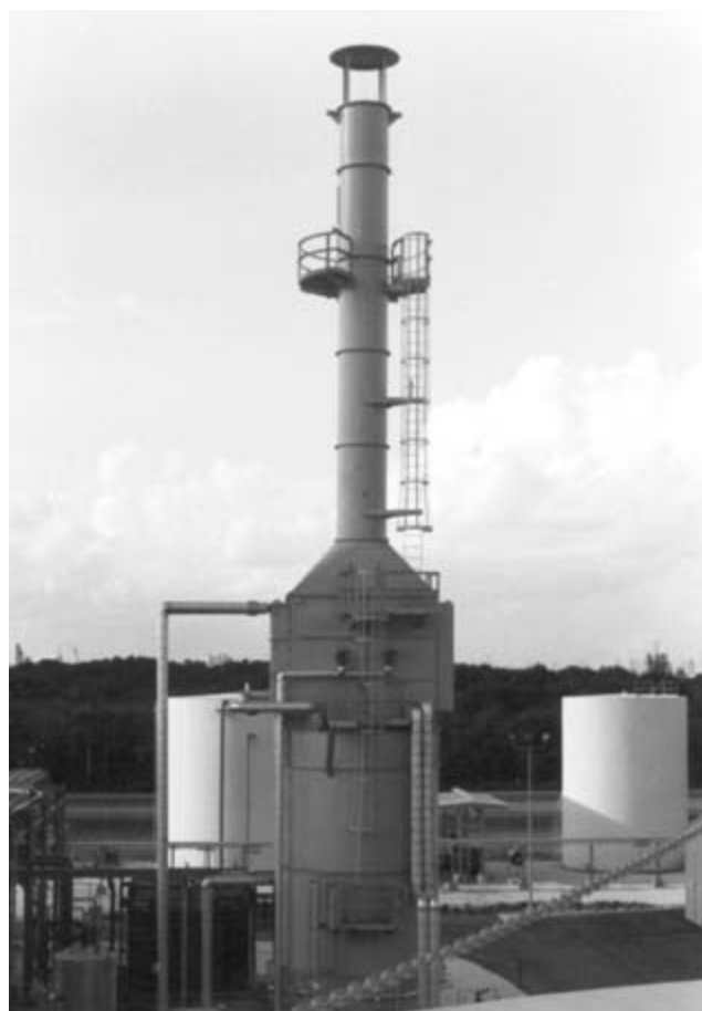
Figure 6-19. Vertical heater. Courtesy of Nisseki Chemical Texas, Inc., Bayport, Texas.
