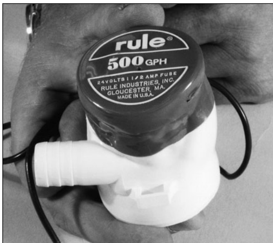
Fig. 9-2. Melted bilge pump, caused by installing a fuse that was overrated for the motor. Notice that the wiring survived unscathed.
