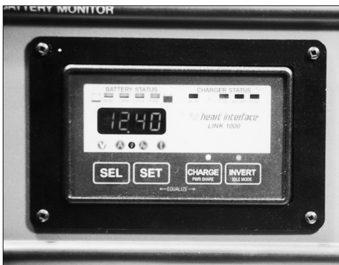
Fig. 11-21. A typical inverter monitoring panel, the Xantrex “Link” 1000.
