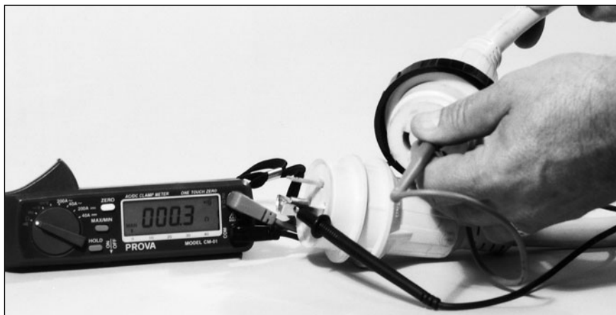
Fig. 11-14. The “wiggle test” on a shore-power cord.
