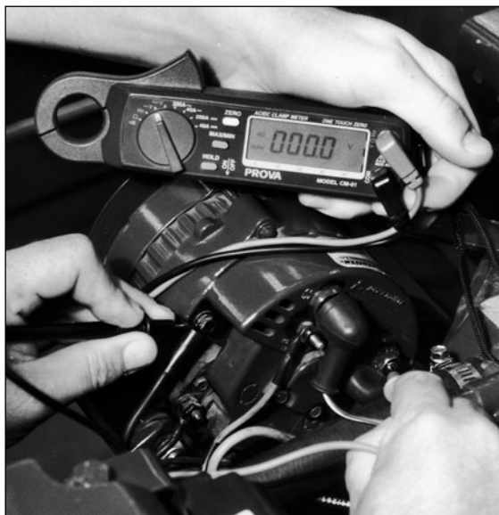
Fig. 6-7. Checking for field-excitation voltage at the alternator. Remember, the ignition key must be switched on when making this test. You should get a reading of approximately 12 volts. The meter red lead is connected to the F terminal and the black lead to a good ground, in this case, the GND terminal on this particular alternator. The key switch isn't on yet, but a reading of about 12 volts will show on the meter if all is well.
