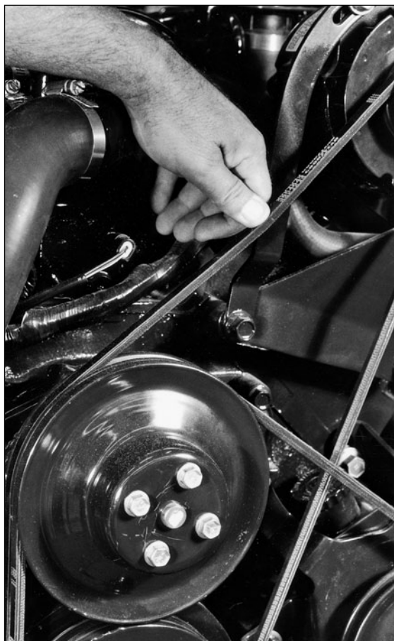
Fig. 6-2. Checking belt deflection. This belt is adjusted just about right!
