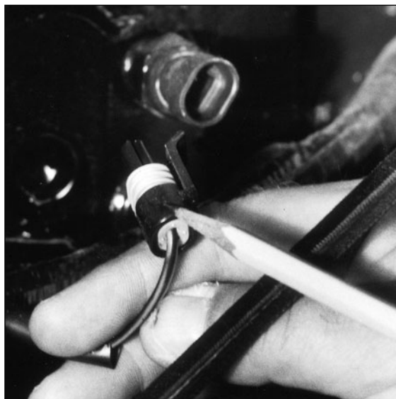
Fig. 7-4. Photo of Deutsch-type gang plug. These offer the best waterproof connections and are now widely used by engine makers.
