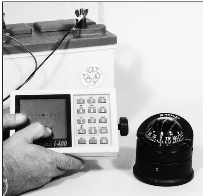
Fig. 12-1. Checking compass deviation with a temporary hookup to an electronic instrument.
