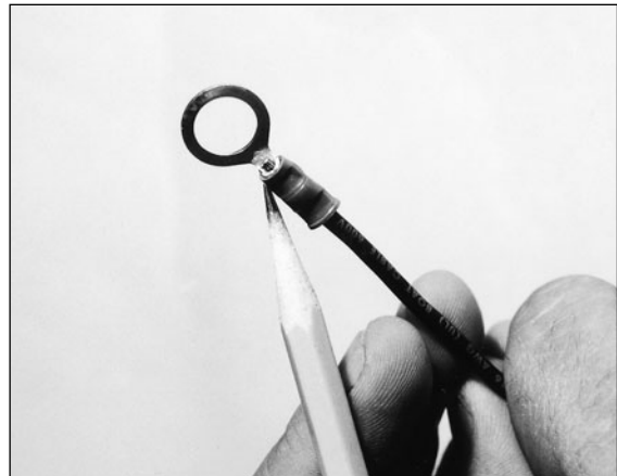
Fig. 4-28. The correct amount of wire protrusion through the barrel of the connector.
