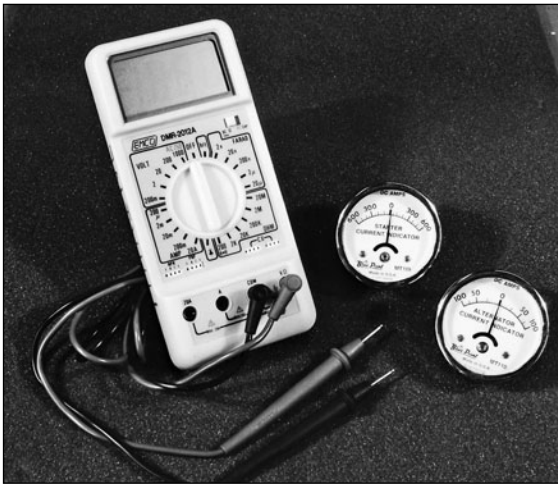
Fig. 3-1. A 20-amp multimeter with Snap-On inductive meter set offers a fairly economical solution for measuring amperage up to 500 amps. The combination can be purchased for under $100.
