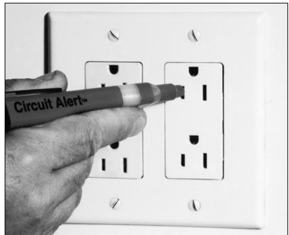
Fig. 11-10. Using the inductive AC tester to check voltage at an outlet.
