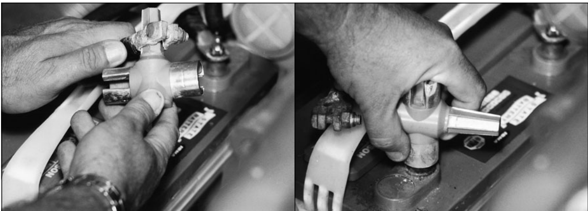
Figs. 5-6, 5-7. Steps to cleaning the battery post and clamp, using a battery service brush. Use these tools until you see shiny surfaces on both the post and inside the clamp. Figure 5-6 shows the terminal being cleaned; figure 5-7 shows the battery post being cleaned.
