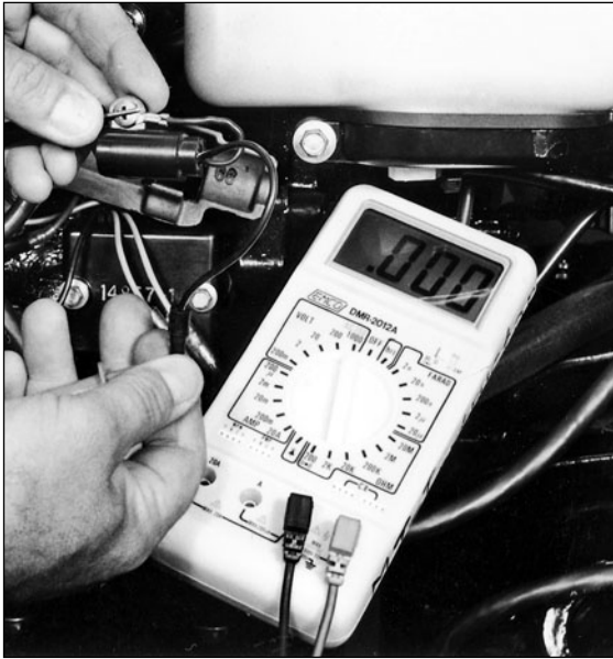
Fig. 7-21. Mercury tilt switch. This switch is designed to prevent engine starting with the prop out of the water. If it malfunctions (open-circuits), your engine won't start with the prop in the water, either! In this picture I've removed the switch and am testing its function with a multimeter set to check continuity when the switch is tilted manually. I'm verifying with the meter that the switch turns off and on.
