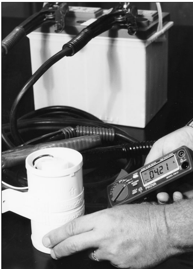
Fig. 4-2. Battery jumper cables being used to determine amperage draw for a new electrical installation. In this case, I'm checking the actual draw for a new bilge blower.
