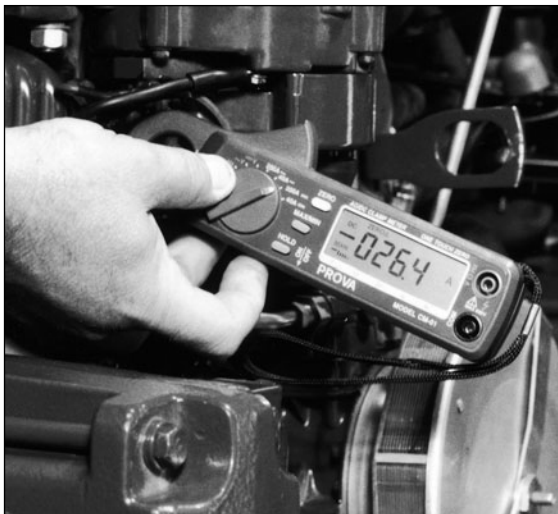
Fig. 6-8. Using an inductive ammeter to check alternator output. When checking amperage output in this fashion, turn on all your DC accessories and see if the alternator can keep up to the demand.
