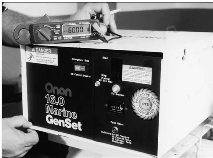
Fig. 11-22. Checking frequency with the multimeter.
