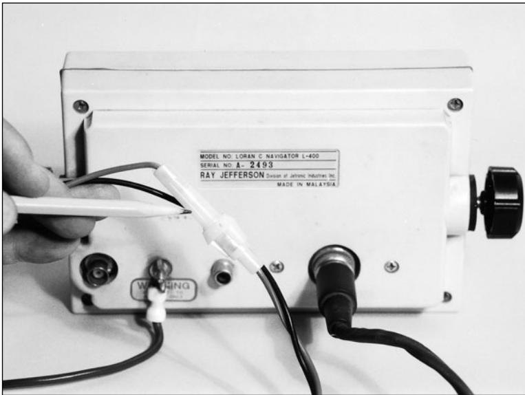
Fig. 12-2. A typical factory harness, with in-line fuse holder installed.
