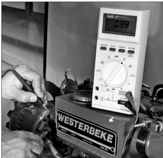
Fig. 6-10. AC ripple-voltage test. Your black meter lead should be connected to a known good ground and the red lead to the B+ (output) lead on the back of your alternator. Remember to make sure that your meter is set to the AC volt scale.
