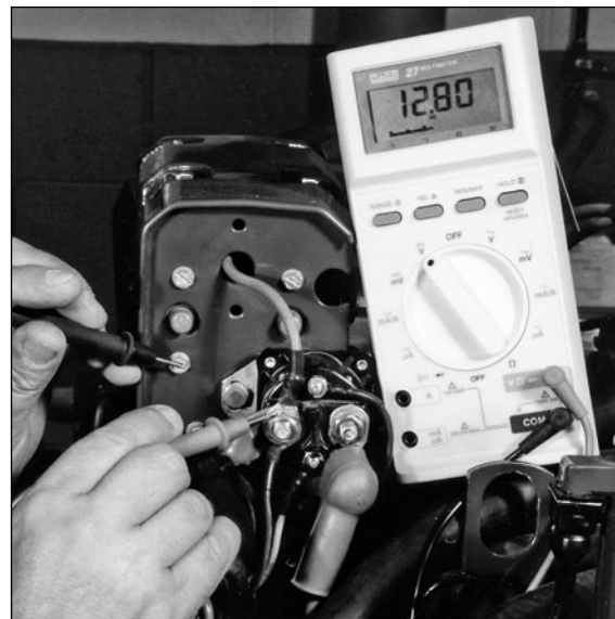
Fig. 8-5. Checking for voltage supply to a starter-motor solenoid. You should get a reading of approximate battery voltage here.
