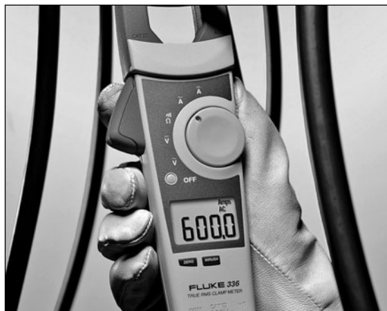
Fig. 3-3. Fluke Model 336 clamp-type meter. This is a true RMS (root-mean-square) meter that can read up to 600 AC or DC amps. This is an excellent choice if you do a lot of AC work. Its shortcoming is that its ohms scale is not as sensitive as other meters I've used. This model sells for about $275.
