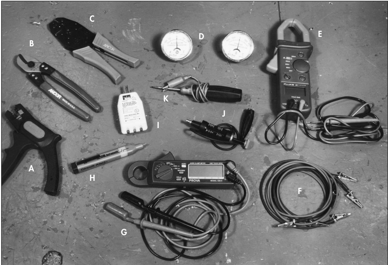
Fig. 1-9. Some basic and not-so-basic electrical tools from my collection. Beginning at the lower left and moving clockwise are (A) wire stripper, (B) cable cutter, (C) ratcheting crimping tool, (D) inexpensive Snap-On inductive ammeters, (E) Fluke 36 high-amperage inductive multimeter (true RMS), (F) miscellaneous jumper leads used for various tests, (G) the Ancor/Prova inductive ammeter with frequency scale, (H) AC probe pen, (I) AC LED socket (outlet) tester, (J) Snap-On ignition spark tester, (K) 12 V test light/probe.
