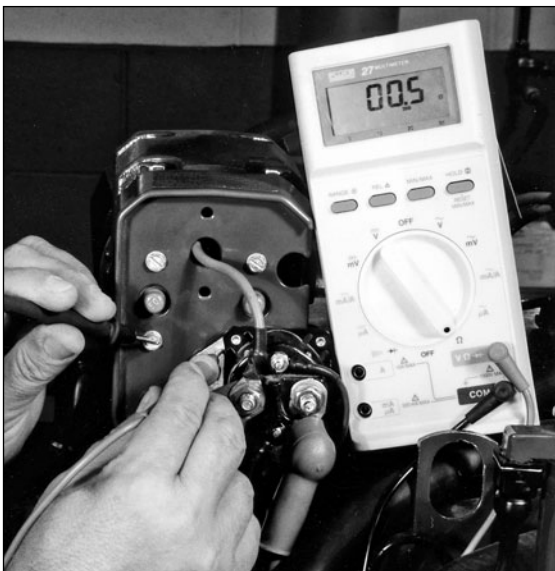
Fig. 8-4. Using an ohmmeter to check ground continuity at the solenoid.
