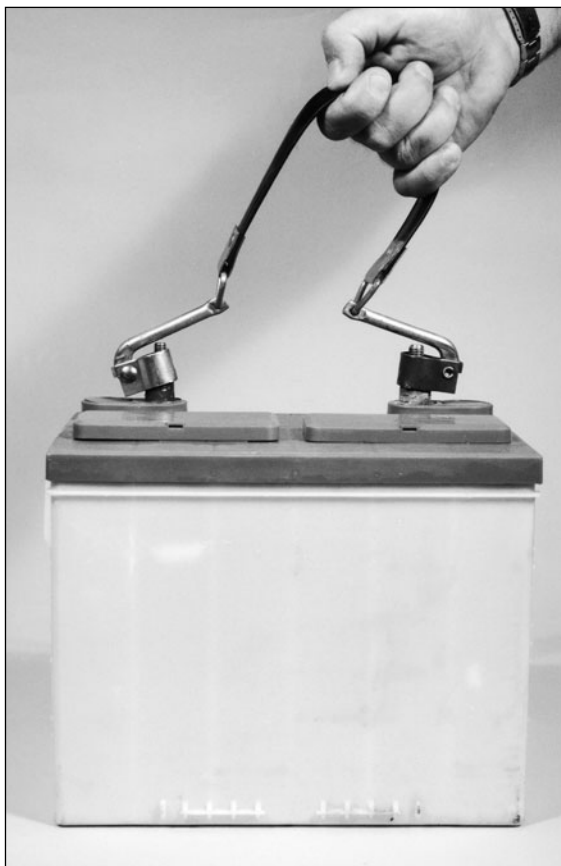
Fig. 5-3. Battery carrying strap in use. This type of strap assembly will only work for smaller group 24 and 27 batteries. Larger batteries all have carrying handles attached, and should be handled by two people.
