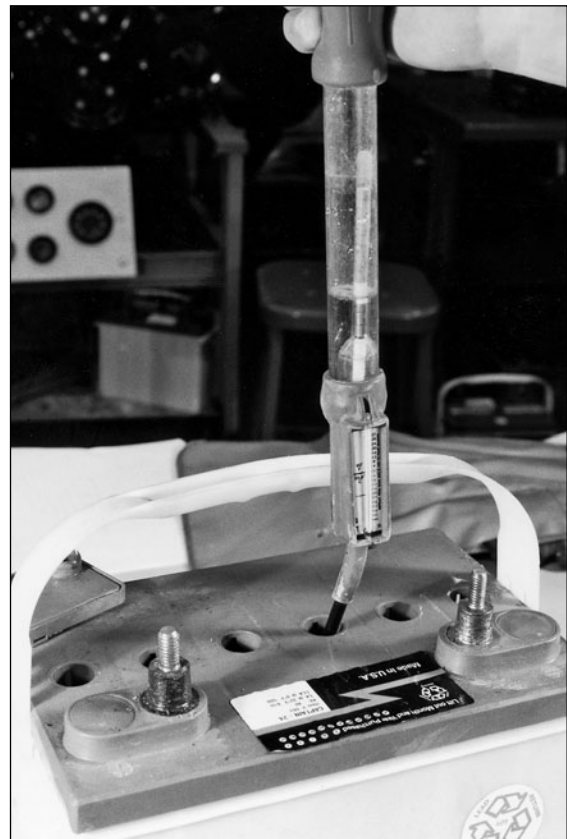
Fig. 5-16. Temperature-compensated hydrometer in use.
