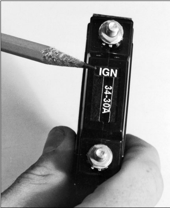
Fig. 4-13. “Ign. protected” label on a protected breaker. This is the only breaker type that should be used in an engine room or compartment where CNG or LPG are stored.
