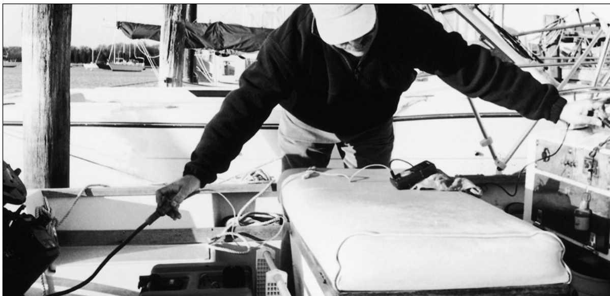
Fig. 8-8. Checking the wiring harness for continuity between the remote control and the engine. In this picture I've disconnected the plug at the back of the ignition switch and at the engine, and am using my ohmmeter to check for breaks in the wiring harness.
