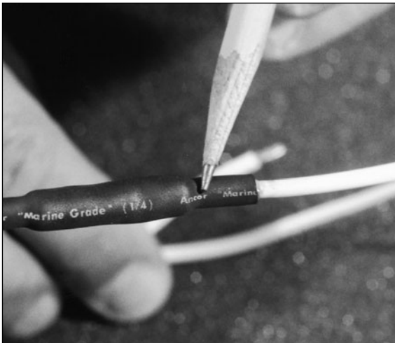
Fig. 4-32. Butt connection with waterproof heat-shrink tubing. This is the highly recommended method for joining two wires together, especially in the area of the bilge.
