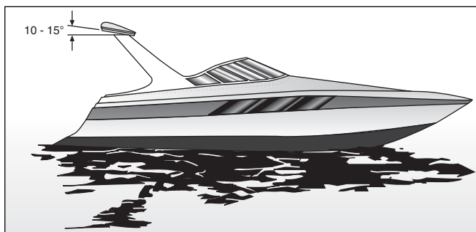
Fig. 12-15. Static angle for powerboat radar antenna installation.
