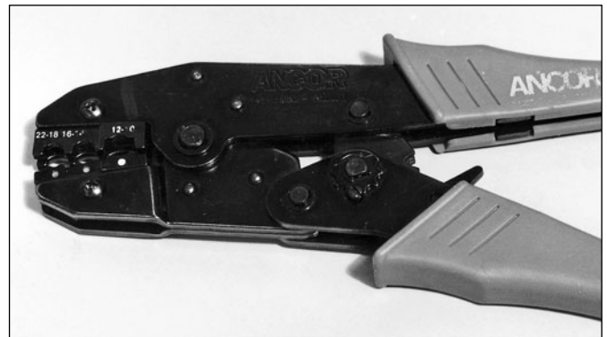
Fig. 4-24. Ancor ratcheting crimper. By using this type of crimper, you can be assured that all your connections will be crimped properly as long as you use the tool correctly.
