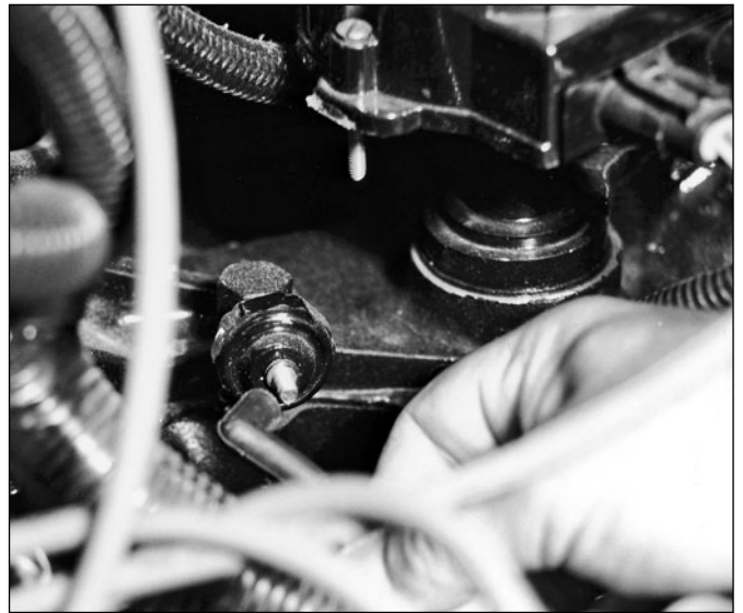
Fig. 10-9. An oil-pressure sending unit on a GM V8 engine. On this engine it's located next to the ignition distributor.
