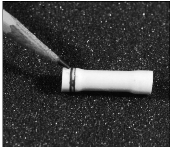
Fig. 4-33. "Stepped"-type butt connector. These are the only way to go when you need to join two wires of different gauges.
