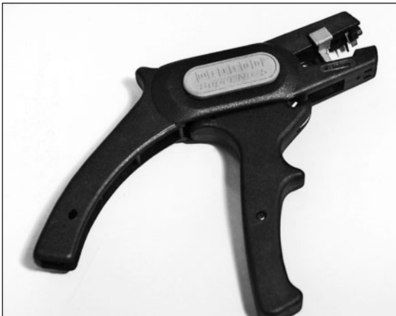
Fig. 4-25. End stripper. I love these tools because you can adjust the amount of insulation to remove for a really good match to the crimp connector. One drawback is that they only work on wire up to 10 AWG.
