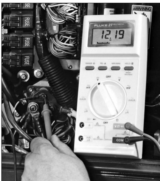
Fig. 8-9a. Checking voltage supply to an outboard-engine solenoid with the key in the start position. Remember, with the key in the start position, if the engine is cranking, the voltage reading will drop down to as little as about 9.6 volts.
