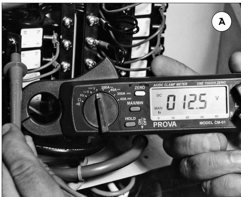
Figs. 4-14a, b. Meter test sequence for a circuit breaker. With one meter lead attached to a known good ground, check the feed side of the breaker for 12 volts. With the breaker turned on, you should have 12 volts at the adjacent terminal on the breaker. If not, the breaker is faulty and must be replaced.
