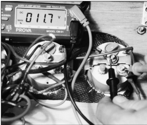
Fig. 10-5. Verifying voltage and good ground at the volt-meter.
