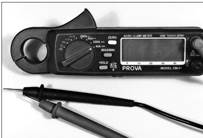
Fig. 3-2. Ancor/Prova clamp-type meter. This unit retails for around $300 and offers amperage reading capability up to 200 amps and a frequency-checking function, useful for some AC tests. Made by Prova, marketed in the United States by Ancor.
