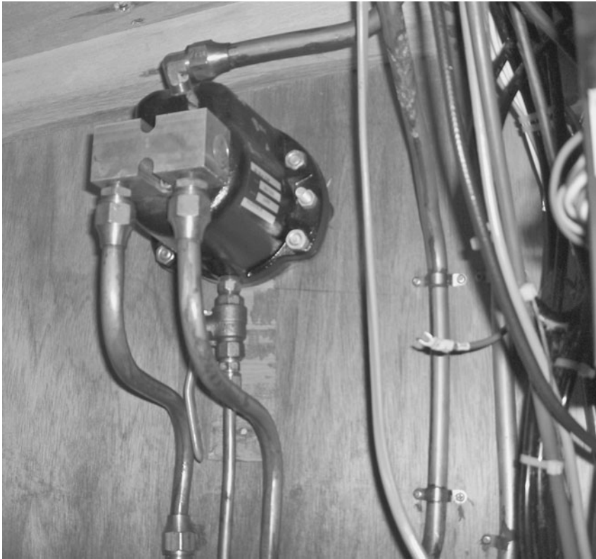
Fig. 15-5. A hydraulic helm pump viewed from behind the bulkhead where it's mounted. There are many potential sources of steering-fluid leaks throughout the system.
