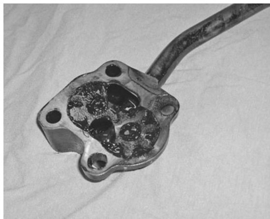
Fig. 5-8. Congealed oil in an oil pump is clearly visible in this photo of the pump's endcap.
