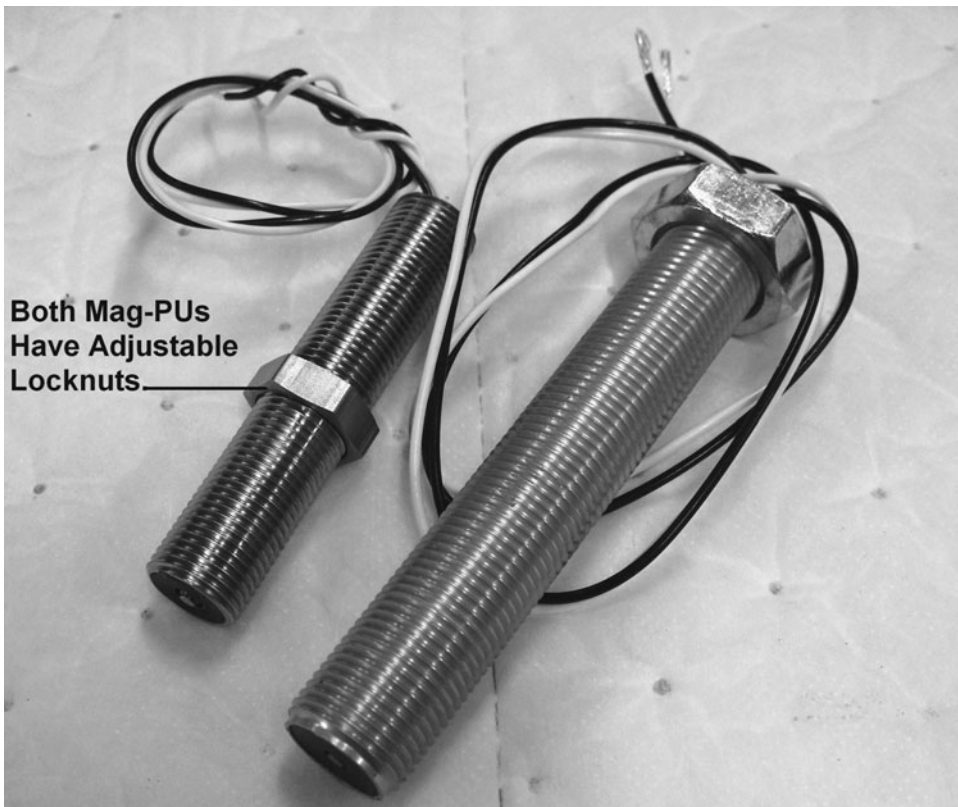
Fig. 7-13. Electric tachometer senders, also known as magnetic impulse pickups, are used in generator engine speed-control systems.
