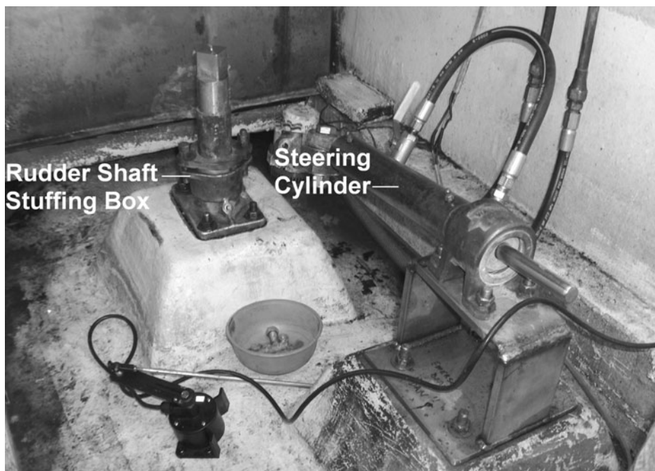
Fig. 9-4. The top of the rudderpost and a hydraulic steering cylinder are clearly visible in this photo. The rudder arm has been detached from the post so that the rudderpost stuffing box can be repacked. The arm is hanging from the far end of the cylinder and is not clearly visible.
