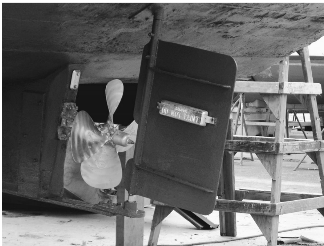
Fig. 9-7. Rudder with a 2:1 aspect ratio.
