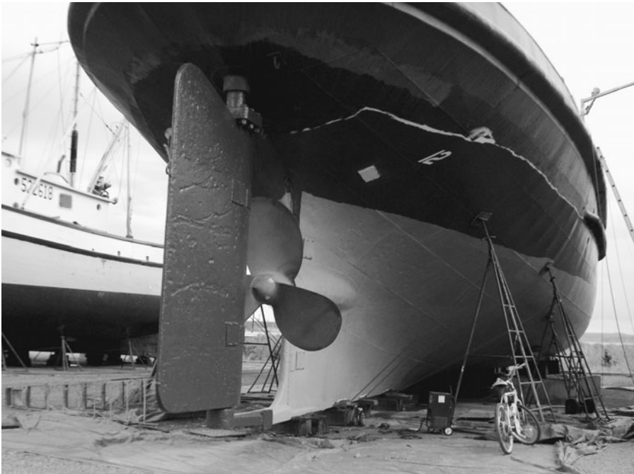
Fig. 9-1. The rudder of this steel motoryacht is mounted on a vertical rudderpost, or shaft. A shoe extends aft from the keel to capture and support the post's bottom end.
