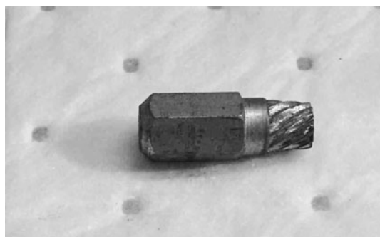
Fig. 1-19. An extractor for broken bolts and fittings, showing the helical grooves in its business end. Figure 1-21 shows it in use.
