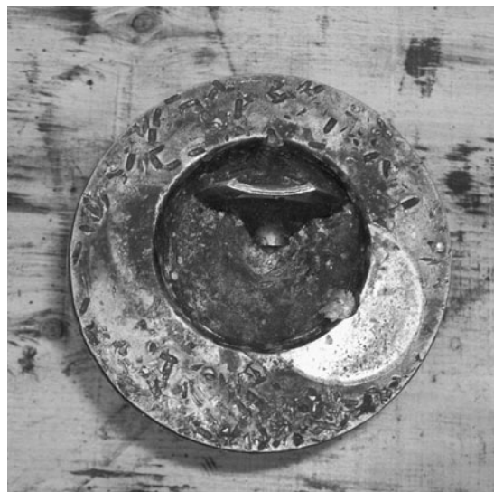
Fig. 10-15. Broken valve head embedded in a piston.
