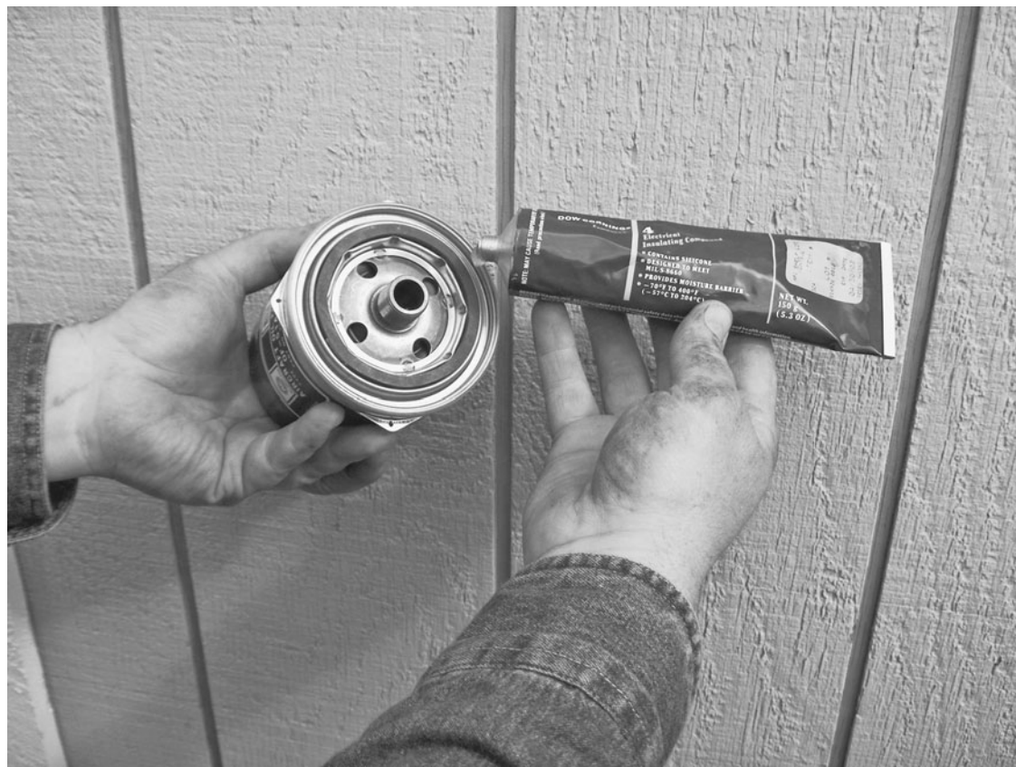
Fig. 5-13. Lube the oil filter seal with silicone grease.
