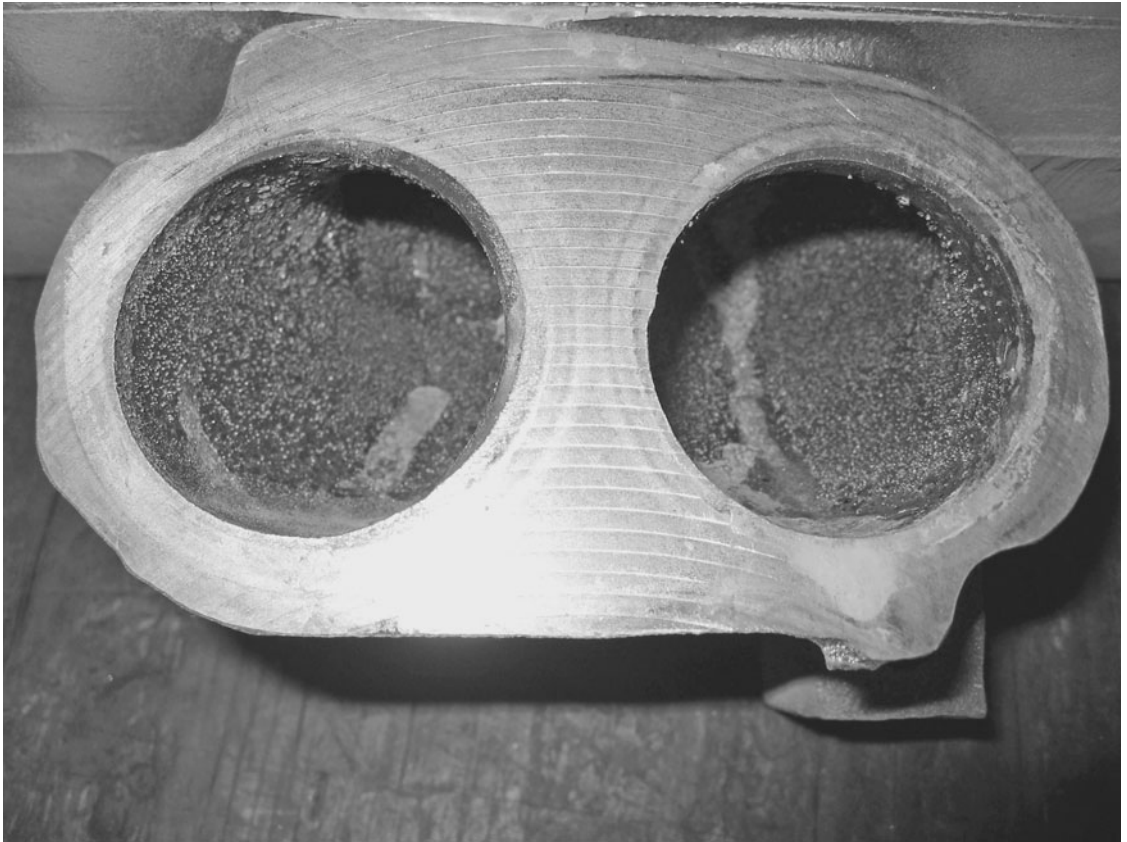
Fig. 12-9. The exhaust ports shown in this section of exhaust manifold were badly rusted. Rainwater had invaded the cylinders through a vertical stack.
