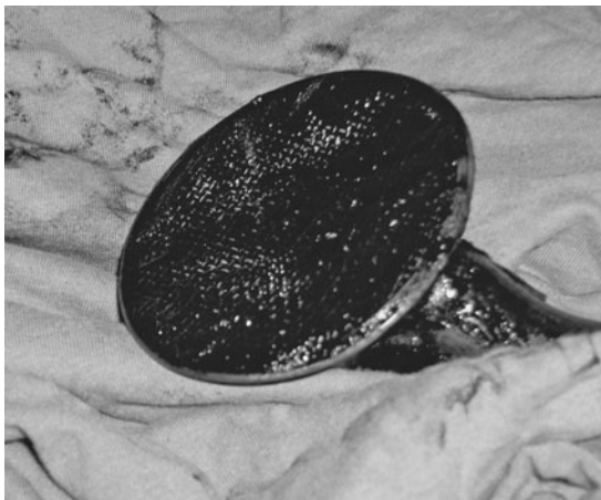
Fig. 5-5. A partially plugged oil pump suction pipe.
