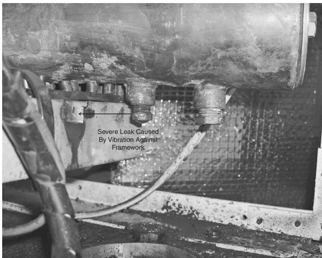
Fig. 12-8. A coolant leak into the bilge can be caused by excessive vibration of the heat exchanger. Here a mechanic has pulled the heat exchanger away from its point of contact with the engine bed. (Courtesy MER Equipment, Seattle, Washington)
