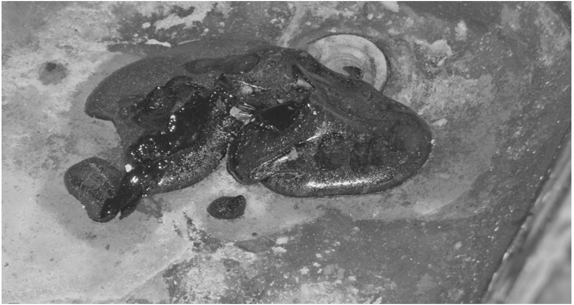
Fig. 5-4. An example of sludge created by antifreeze leaking into crankcase oil.
