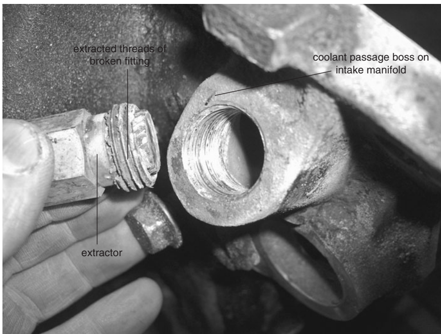
Fig. 1-21. An extractor in action.
