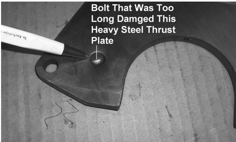
Fig. 10-9. Bolts that are too long can exert great force and damage the engine. The dimple in this camshaft thrust bearing was made by an overly long bolt. In this case it did not cause an engine failure, but it could have.
