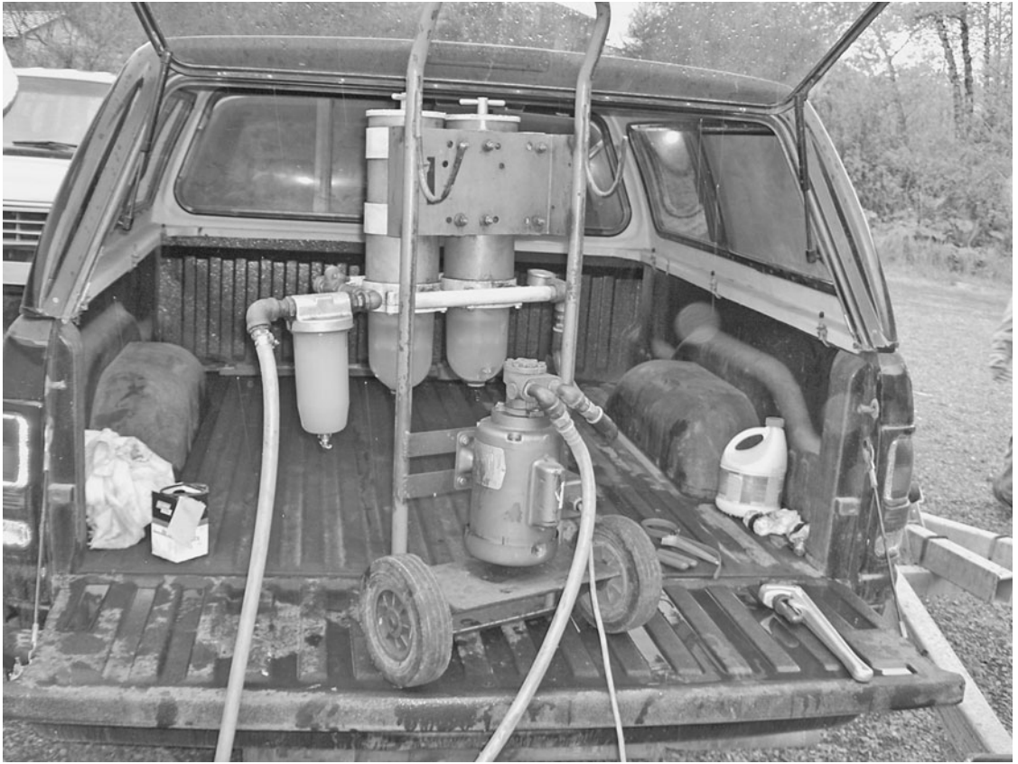
Fig. 5-1. A filter buggy removes water from fuel.
