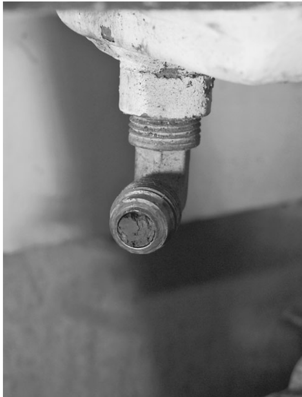
Fig. 12-5. This plugged coolant passage could have been avoided by regular changing of the coolant. (Courtesy MER Equipment, Seattle, Washington)
