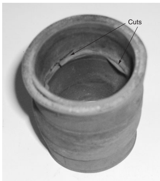
Fig. 4-8. Too much clamping force cut the inside of this silicone rubber hose. (Courtesy MER Equipment, Seattle, Washington)
