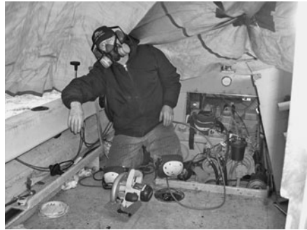
Fig. 5-3. Cutting a deck open to remove a fuel tank.
