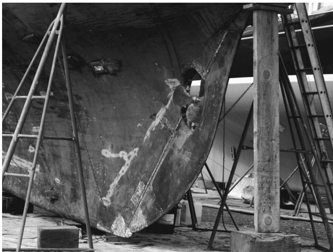
Fig. 9-2. A rudder hung from the after edge of the full keel on a traditional sailboat.
