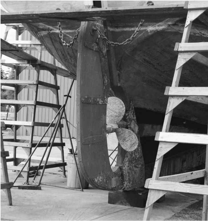
Fig. 9-3. This wooden rudder hung on the back of a keel looks like a jerry-built arrangement.
