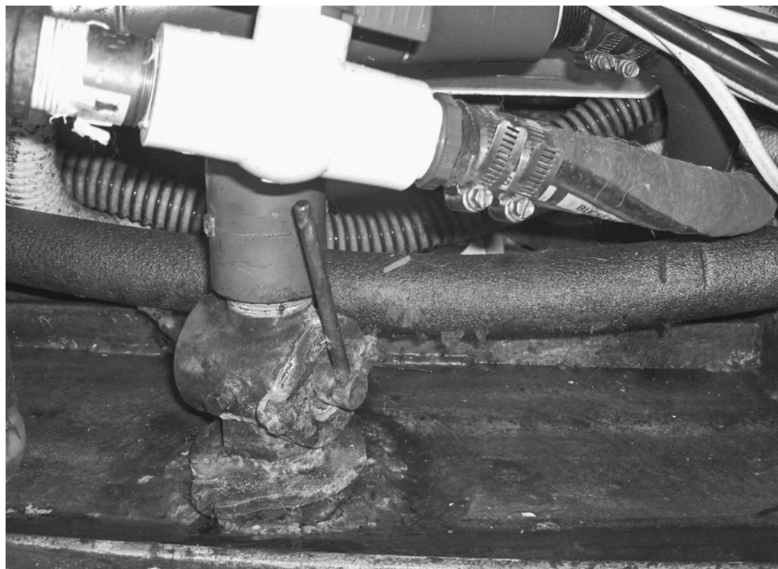
Fig. 1-7. Watch for corrosion where dissimilar metals meet.
