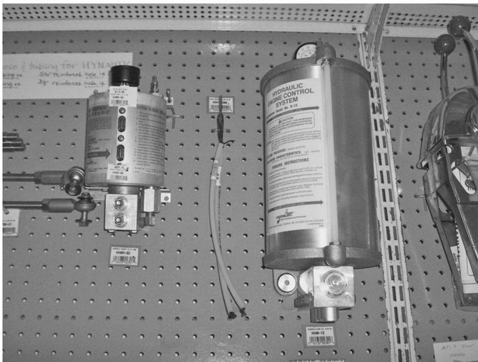
Fig. 15-4. Hydraulic throttle and shift controls require reservoirs like the two shown here. The smaller one at left is for single helm-station controls. The larger one at right is for multiple-station controls. These reservoirs need refilling and pressurizing after repairs and before the controls are bled. The bleeding isn't easy. Consult your manual, and use the fluid specified there.
