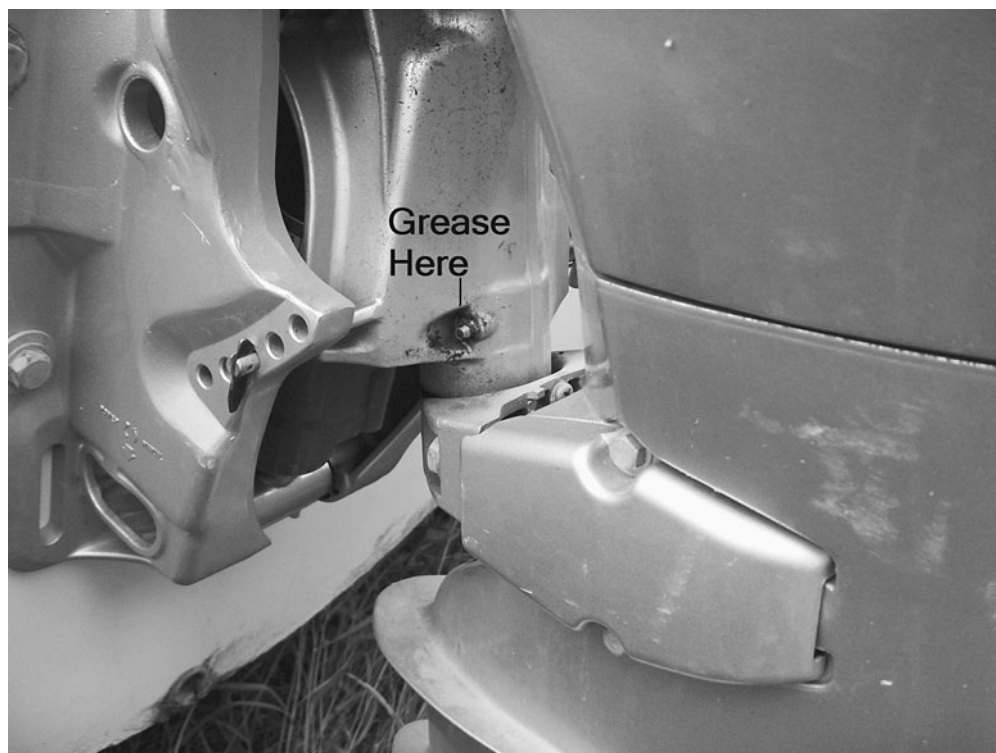
Fig. 14-8. Grease the steering pivot (using the zerk fitting shown here) and the tilt mechanism to ensure smooth operation.
