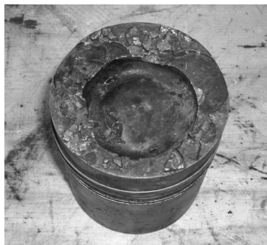
Fig. 10-16. Debris embedded in a piston.
