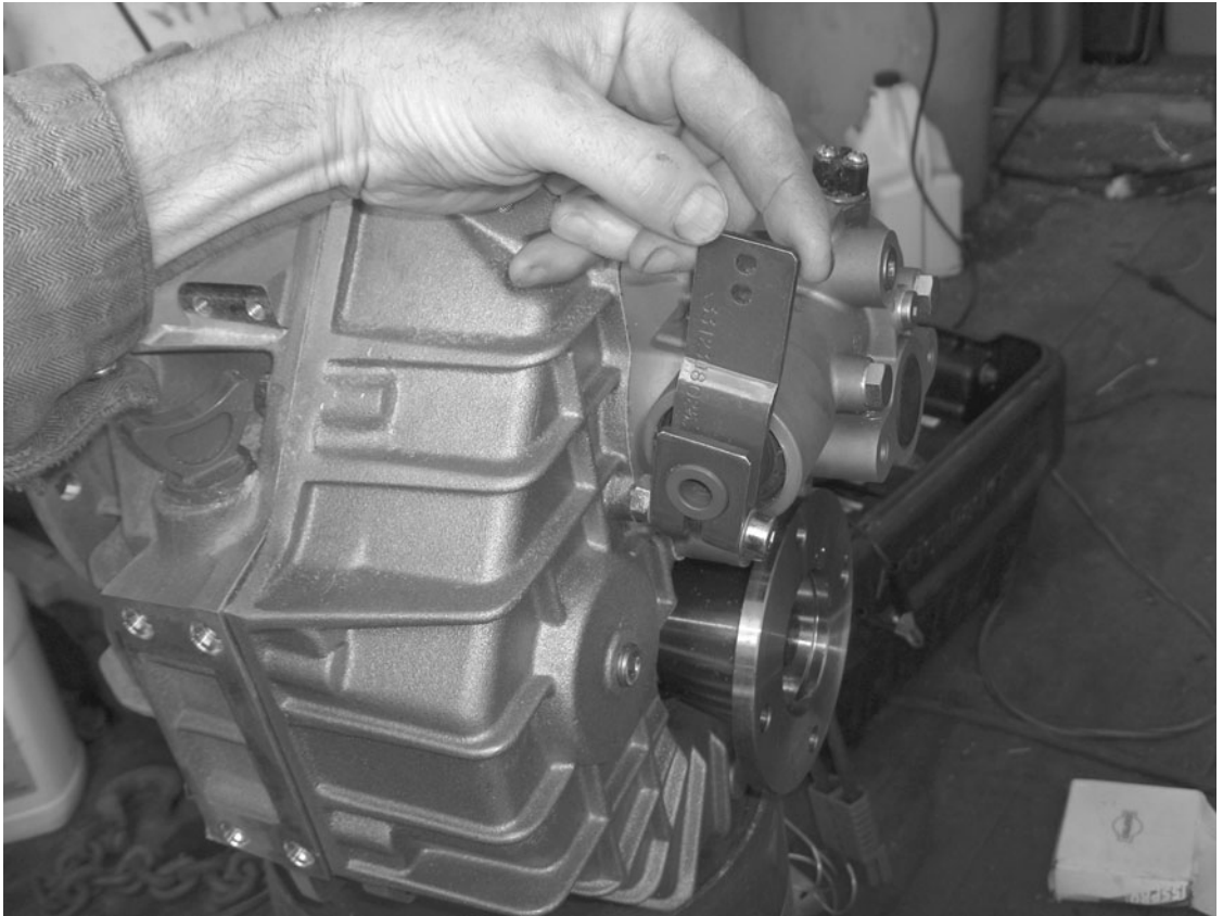
Fig. 14-2. Center the transmission control to neutral.
