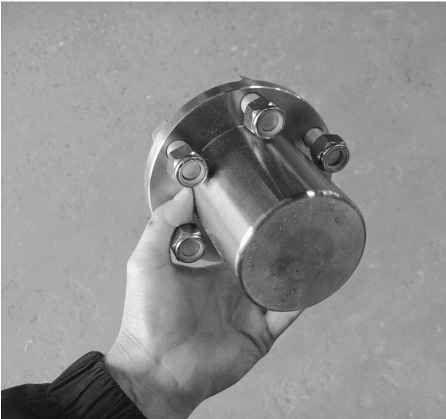
Fig. 14-5. New couplings are made with self-locking nuts. This coupling has yet to be bored for the shaft it will fit. (Courtesy MER Equipment, Seattle, Washington)
