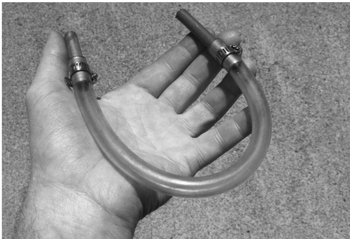
Fig. 10-7. Use a see-through hose to check for air in the fuel.
