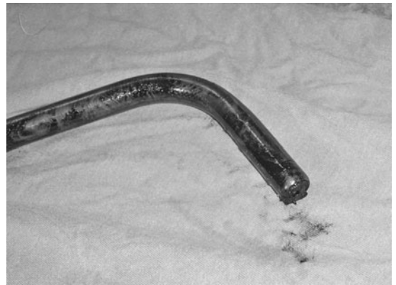
Fig. 5-7. A plugged outlet tube from an oil pump.
