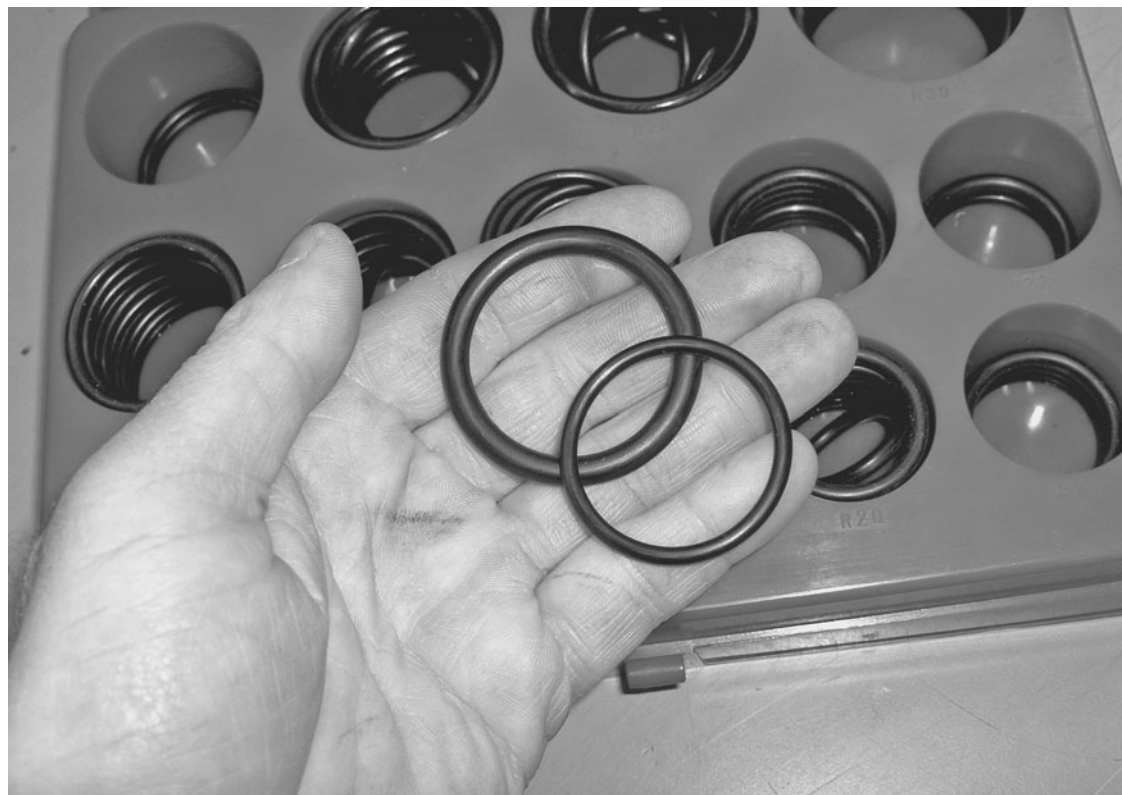
Fig. 12-10. Inspect O-ring seals carefully—they should be pliable and have smooth surfaces.
