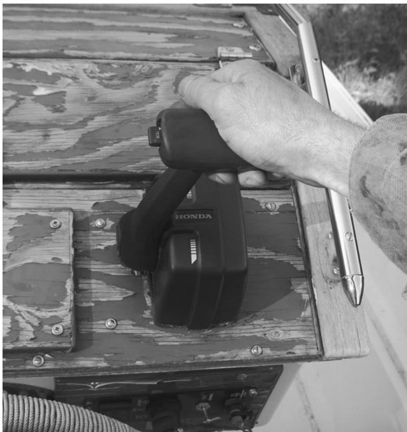
Fig. 14-6. Check the outboard throttle and shift controls for signs of breakage and for full range of movement. Shown here is a combination throttle and shift control. (The two functions are often separated.)
