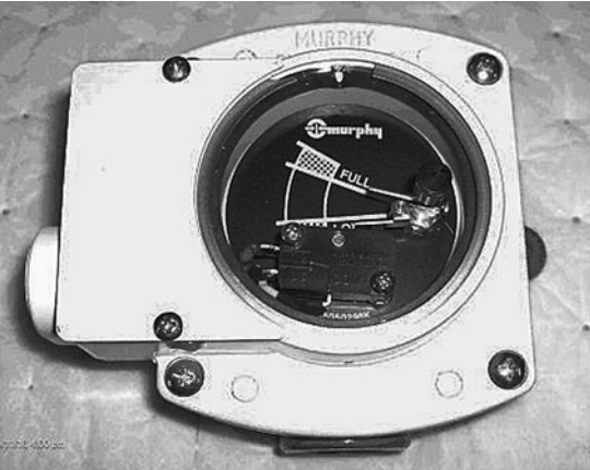
Fig. 3-4. A Murphy coolant level alarm switch is just visible on the bottom rim of this coolant level gauge. When the coolant level gets dangerously low, the switch activates an alarm (propulsion engine) or shuts down the engine (if a generator). See also Chapter 7.
