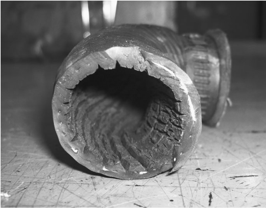
Fig. 10-2. Faulty coolant will destroy hoses. (Courtesy MER Equipment, Seattle, Washington)
