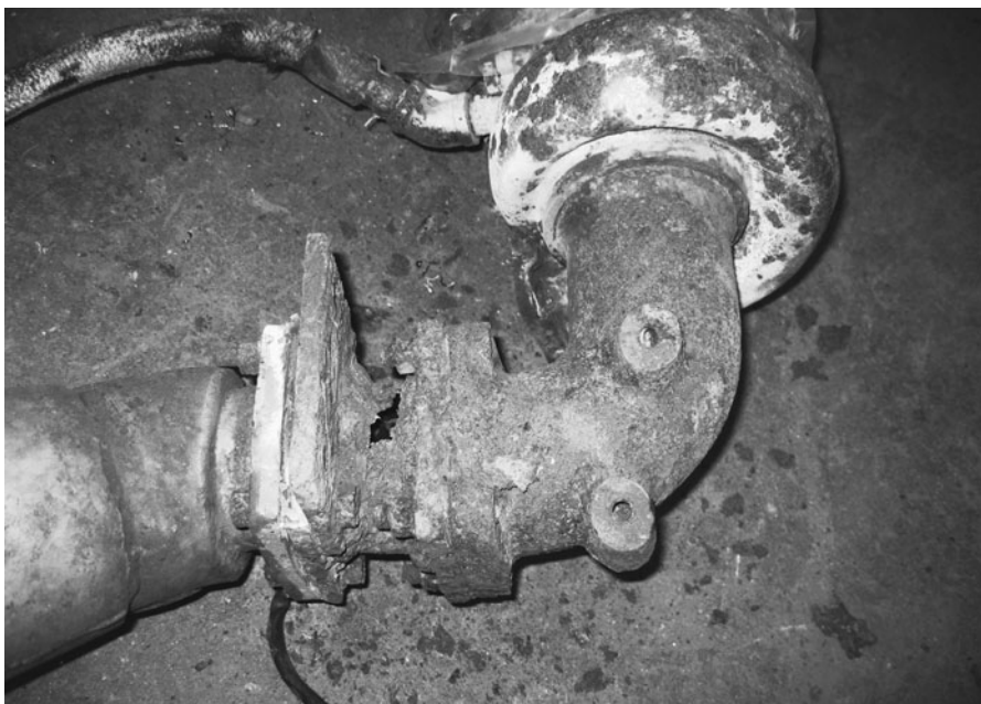
Fig. 13-2. Check the exhaust system tubing for holes. This section of exhaust pipe rusted through from the outside.
