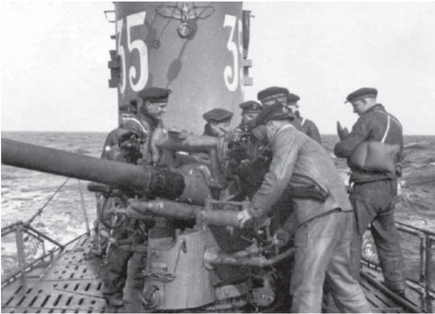
Here the gun crew of U 35 undergo training. Guns would either use bracketed firing (where a short shot is registered and the range left unaltered until an overshoot is obtained) or fire for maximum effect (where the gunlayer fires as rapidly as possible without observing the fall of shot, and the observer makes alterations for the next barrage). High-explosive ammunition with nose-fused, internal-fused, or time- and percussion-fused fuses was used. (Cody Images)
