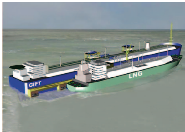
Fig. D.43 Floating LNG terminal EC FP7 research project GIFT (2005–2007) (coordinator: Doris Engineering, France, partner: NTUA)
