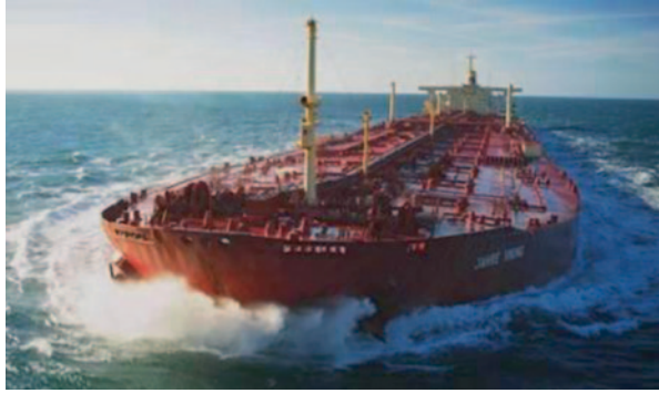
Fig. D.37 The MV Hellenpont Metropolis is the largest built double-hull ULCC (Daewoo Heavy Industries). It has a length of 380 m, a beam of 68 m, a draft of 24.5 m and 442,000 dwt.
