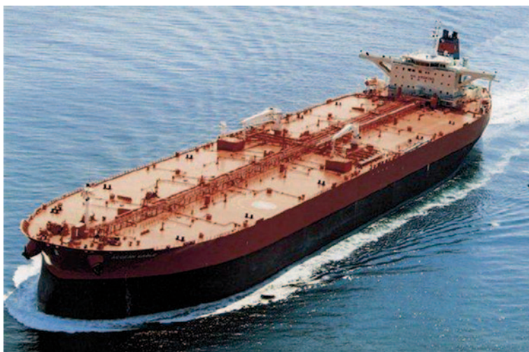
Fig. 3.60 Example of parabolic bow on tanker
