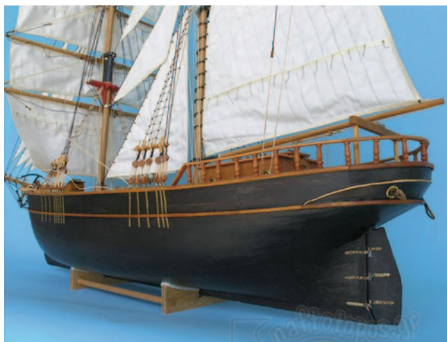
Fig. 3.62 Traditional Greek wooden boat of type “καραβόσκαρο” (karavoskaro) with elliptical/elevated stern
