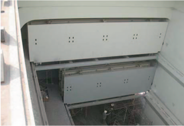
Fig. 2.86 Folding type tween deck hatch covers
