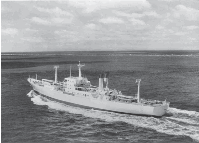
Fig. 4.12 Reefer ship “Polar Ecuador,” built in 1967 by the German yard Blohm & Voss for Hamburg Südamerikanische Dampfschiffahrts-Gesellschaft; operated later for a Greek owner as “Chios Spirit”; is representative of a successful series of fast reefer ships (service speed at banana draft: 23.5 knots) built by Blohm & Voss in the 60s, transporting bananas from South America to Europe (in German: Banana-Dampfer)
