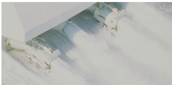
Fig. 5.26 Installation of waterjets on high-speed craft
