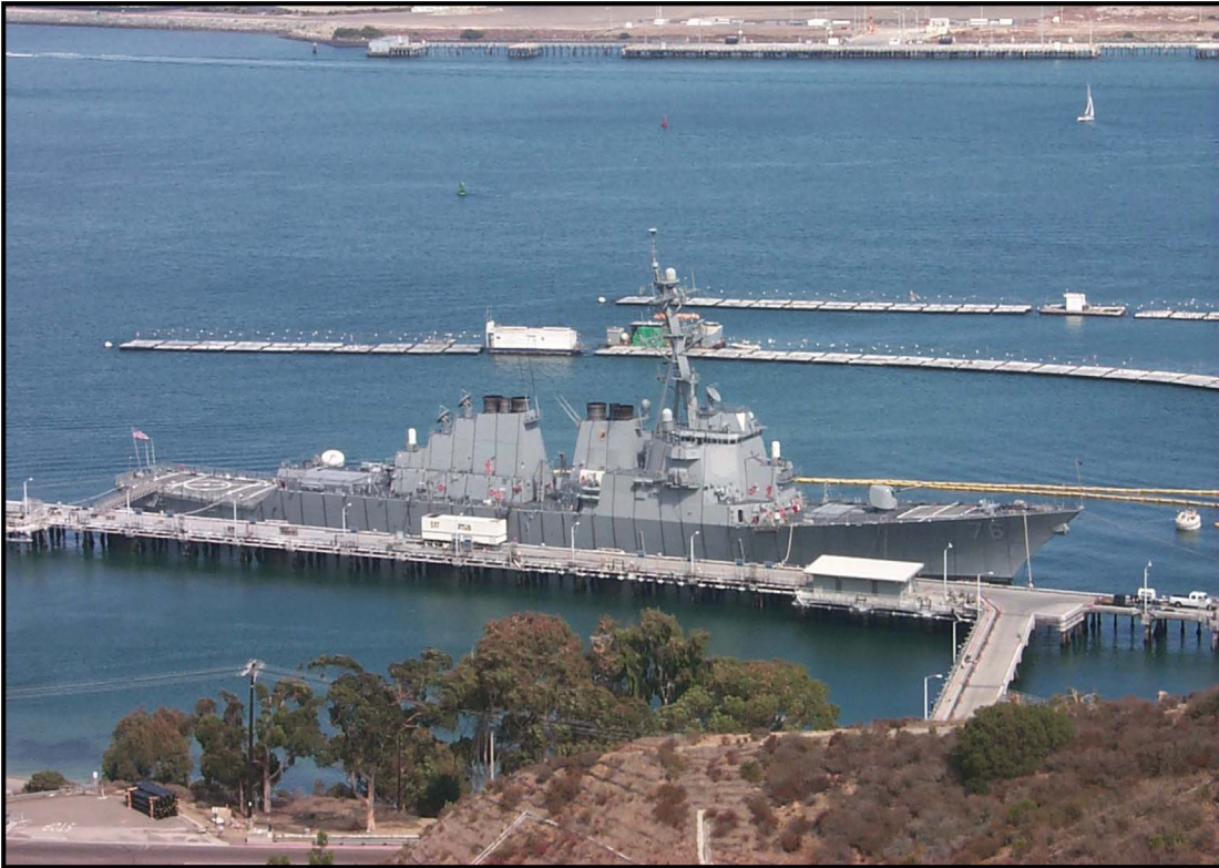
FIGURE 2.9: The USS Higin (DDG-76) being depermed at a close-wrap magnetic treatment facility.
