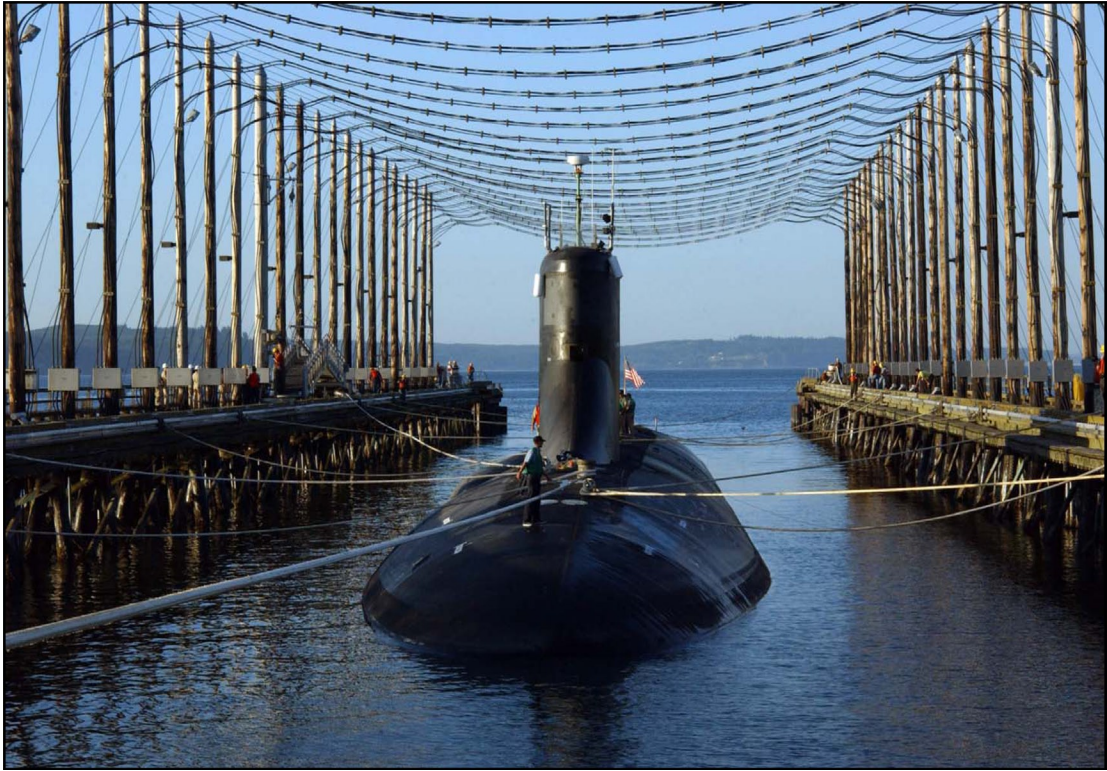
FIGURE 2.10: The USS Jimmy Carter (SSN-23) being depermed at a drive-in magnetic treatment facility.
