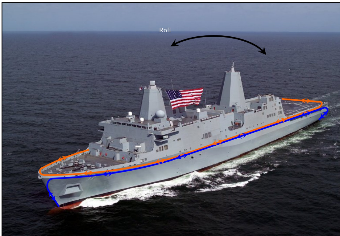
FIGURE 2.17: Eddy current flow induced in a conducting hulled ship due to its roll in the Earth's magnetic field.
