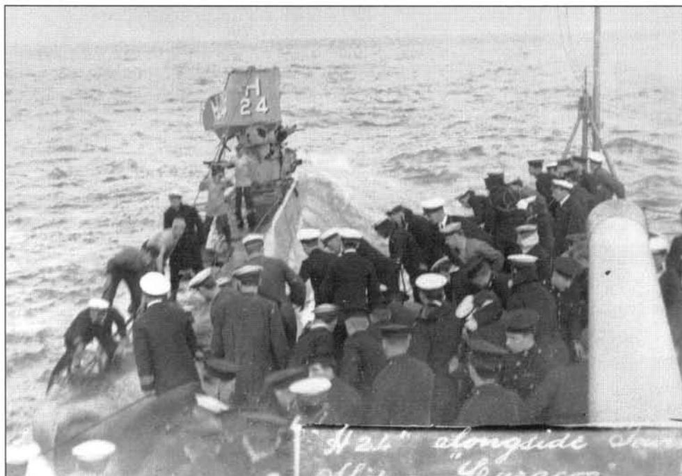
H.24 on the surface and being taken into tow by the cruiser HMS Curacao following her collision with the destroyer Vancouver on 9 February 1922 during the combined Home and Mediterranean Fleets' manoeuvres. Damage to the submarine's conning tower is clearly visible. One month later H.24 was not so lucky. On 23 March 1922 she was rammed and sunk with all hands by the destroyer HMS Versatile .
