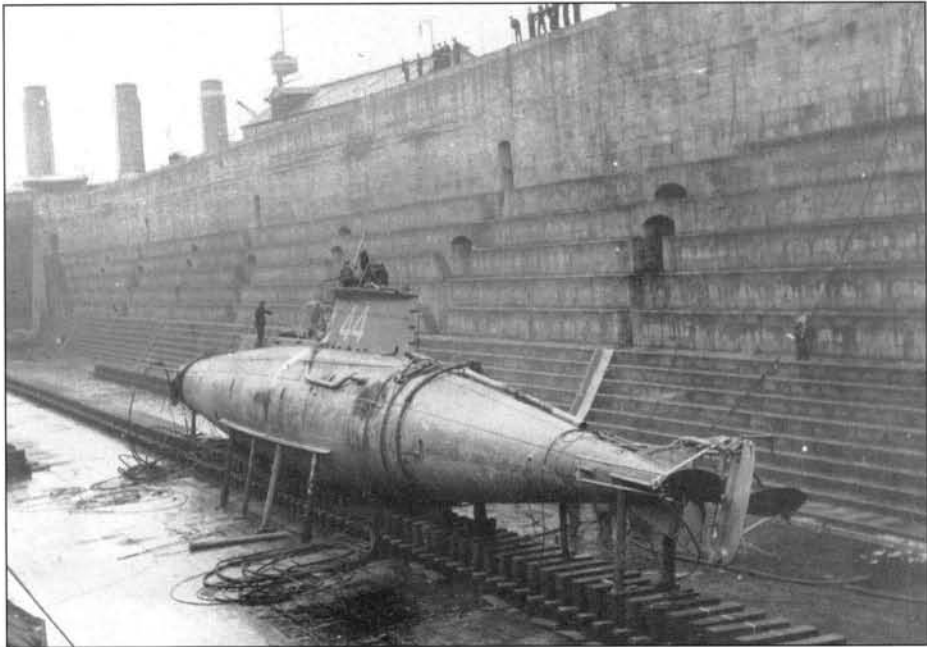
C.14 in dry dock after being salvaged following her collision with Government Hopper No. 29 on 10 December 1913 in Plymouth Sound. This was the seventh occasion on which a British submarine had been sunk in an accident, but the first on which there was no loss of life. The impact point on the submarine's hull can clearly be seen just aft of the conning tower.
