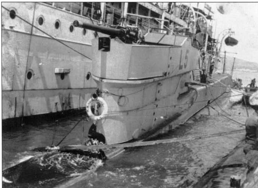
L.5 , showing the gun sited on the bridge, trimmed down by the bow alongside the depot ship Ambrose at Wei-hei-wei in China. The absence of any docking facilities meant that simple repairs to the propellers, rudder or after hydroplanes were often carried out by the simple means of flooding the boat's forward ballast tanks, thus raising the stern.
