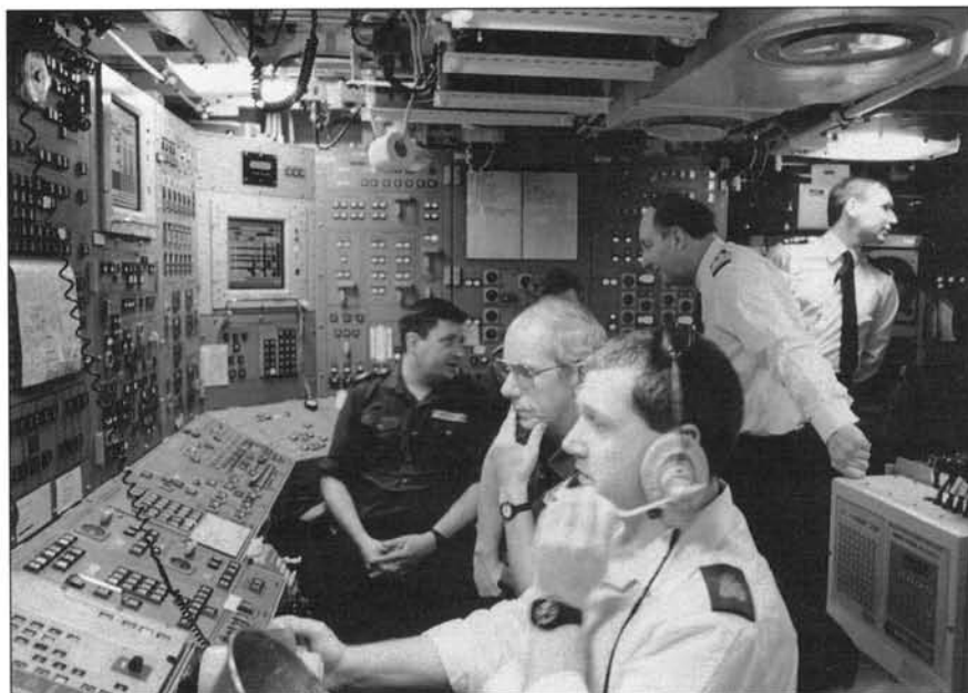
Some key compartments inside the 'Trident' class. The control room, with the remote sensing devices in machinery spaces and their computer-based displays. Admiral Sir Ben Bathurst, the First Sea Lord, visited HMS Vanguard in 1994.
