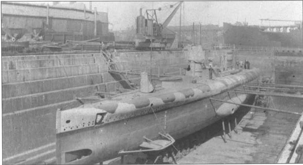
A rare view of G.2 in dry dock. The open aperture for the port side beam tube can be seen in the bulge on the submarine's side. The camouflage pattern was intended to make the submarine less visible from the air as well as to break up the boat's silhouette when on the surface. A number of famous artists, including Norman Wilkinson, were involved in the design of such schemes.
