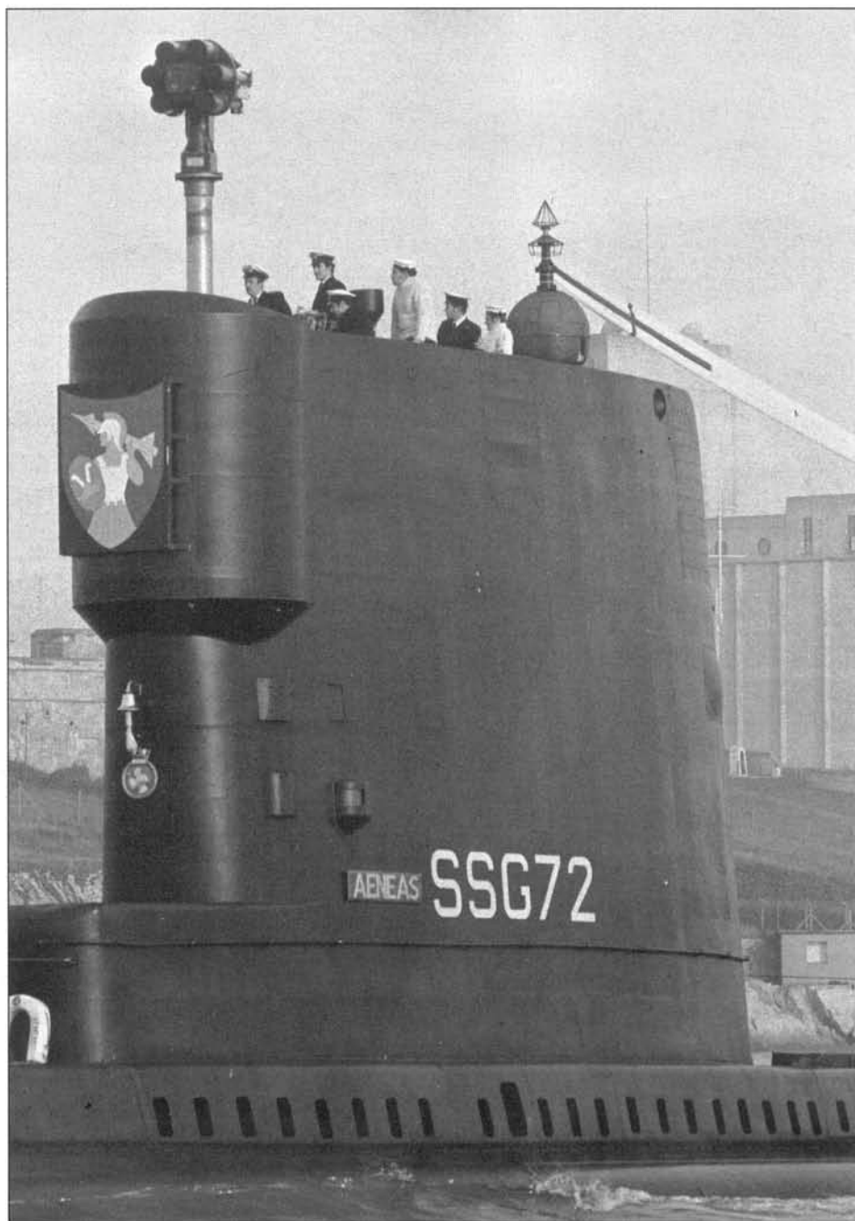
HMS Aeneas with the experimental Submarine Launched Airflight Missile (SLAM) system fitted to her fin. The system consisted of four Blowpipe missiles clustered around a TV camera on a telescopic mast and was designed to thin out prosecuting helicopters which were, and still are, considered a major threat because of their mobility and unpredictability in the close-screening role. The system was never introduced into the Service and when Aeneas paid off in 1972, some wag painted SS Gillette on her after casing – a realistic forecast of her fate.
