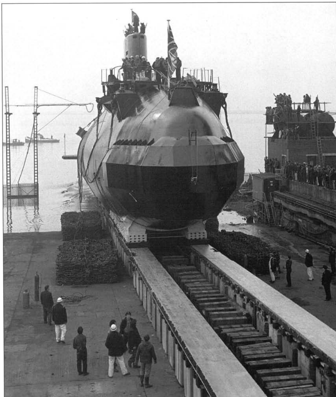
HMS Torbay being launched in March 1985 at Vickers Plc, Barrow in Furness. These submarines are capable of speeds in excess of 30 knots, depths in excess of 1,000 ft, are fitted with the latest sonar 2020, and armed with Spearfish torpedoes and Royal Navy Sub-Harpoon missiles.
