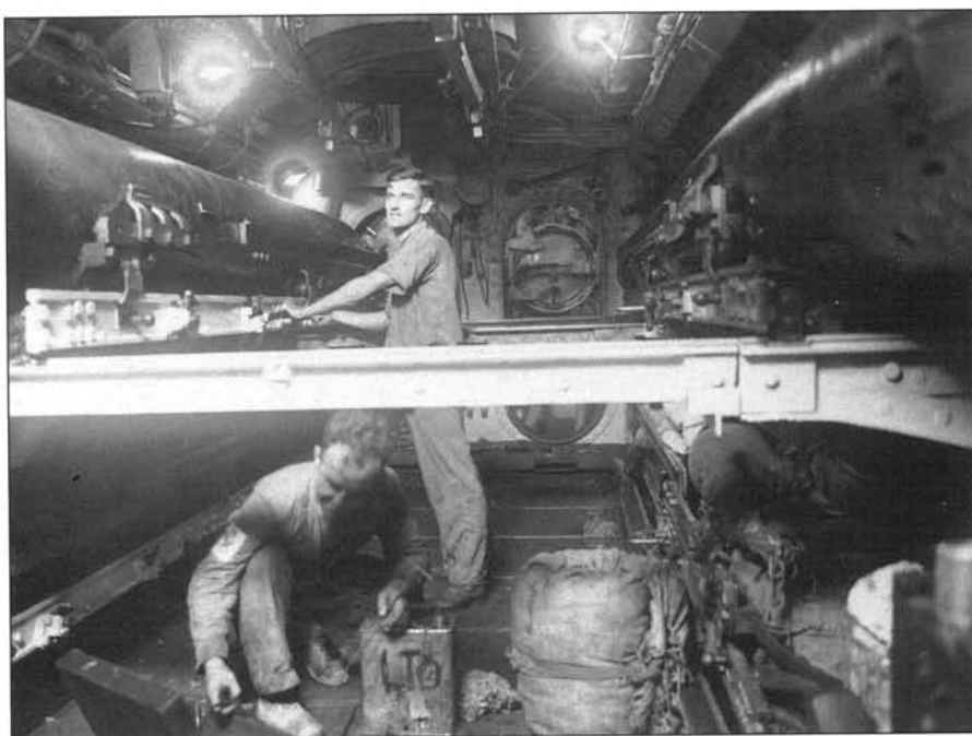
A rare photograph taken in Traveller's fore ends showing the compartment rigged for loading torpedoes. The torpedoes were swung out on their trolleys on the transverse loading rails and then rammed forward into the tube. The reload torpedo for No. 2 is pulled out into the loading position.
