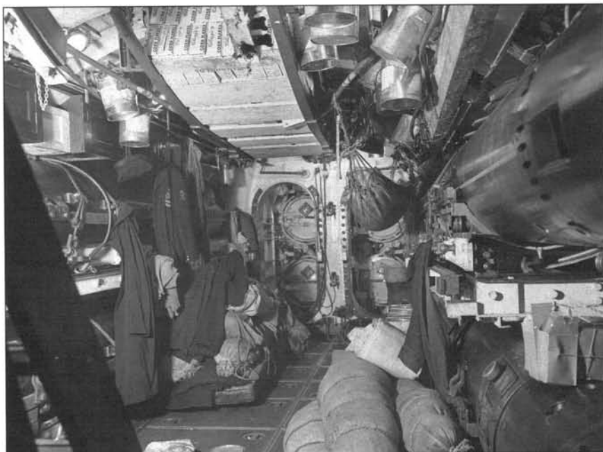
The fore ends in Tribune showing the hideous confusion of hammocks, clothing, spare torpedoes, food (note the cornflakes lodged in the torpedo loading rails) and cooking utensils. The rear doors of six of the four internal bow tubes can be seen in the background.
