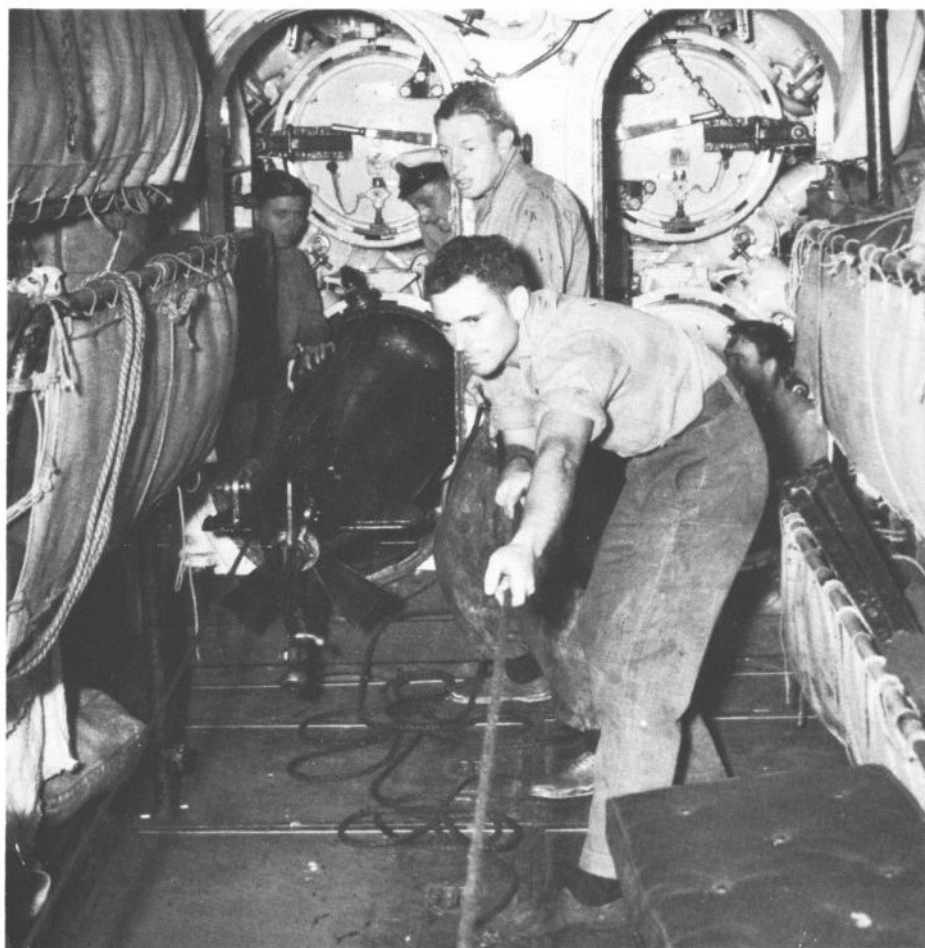
View looking forward in Telemachus' fore-ends in a carefully posed scene showing a torpedo being loaded into No. 4 tube. Of interest are the collapsible berths shown triced up against the reload racks. (Gus Britton)
