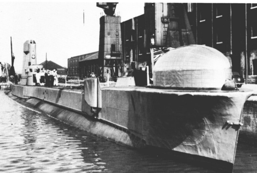
◀ The converted Thermopylae alongside during a visit to London in June 1955, showing the dome for the ill-fated 171 'Four Square' set.
