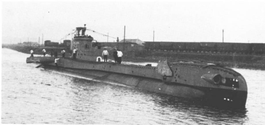
◀ Tapir under way on completion in December 1944, showing the seaguard aerial for the 267W set at the forward end of the periscope standards. The airguard aerial, not visible in the photograph, remains at the after end of the conning tower.
