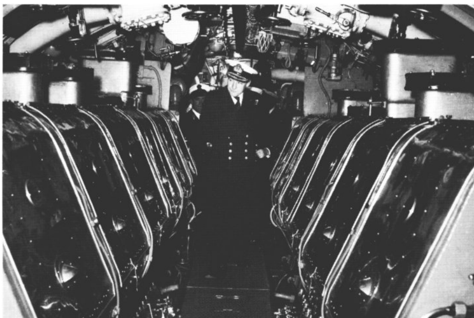
◀ Rear-Admiral Viscount Kelburn, Flag Officer Malta, inspects Token's extremely clean engine room in February 1962 after the submarine had recommissioned. Note the covers in place over the rocker arms of the Admiralty engines.
