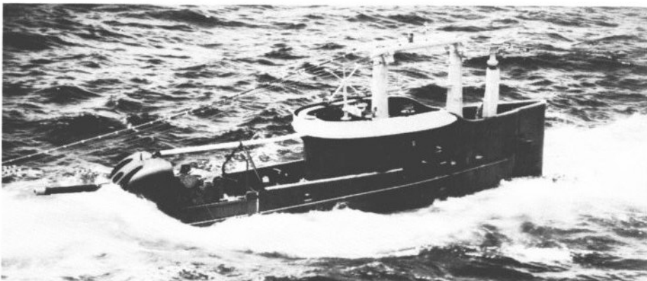
◀ Tactician diving while serving with the Far East Fleet in the early 1950s, and showing the arrangement of the 267MW radar with the X-shaped airguard aerial forward of the periscope standards and the 'cheese' seaguard aerial at the after end. (IWM A.32248)
