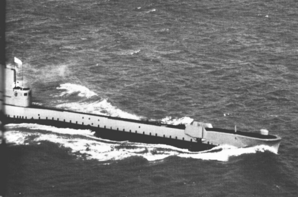
◀ HMS Tiptoe , one of the last four Conversions to be lengthened by 17 feet 6 inches. In this photograph she is shown with both radar W/T masts raised.
