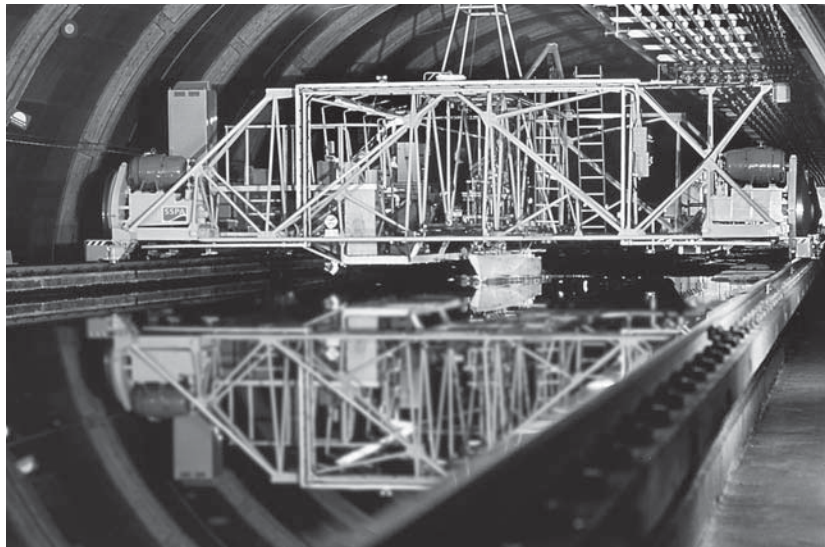
Figure 8.1 Model basin and towing carriage. (Photo: Sven Wessling. Courtesy of SSPA.)
