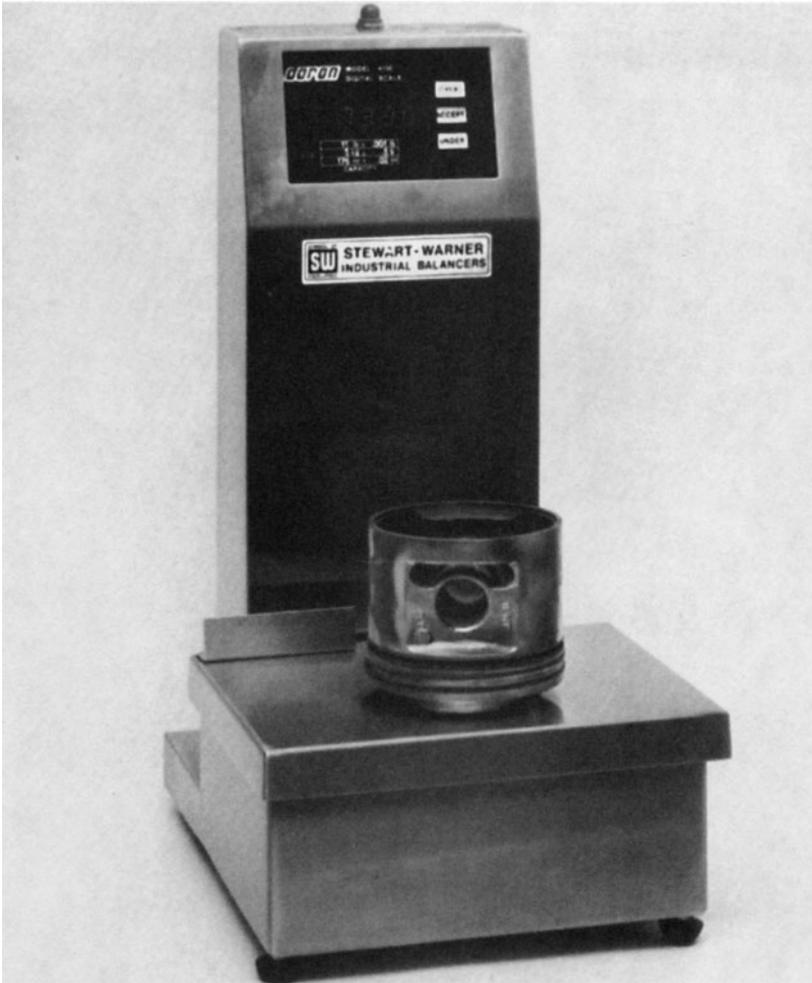
**8-79** Balancing begins with match-weighing piston assemblies.
