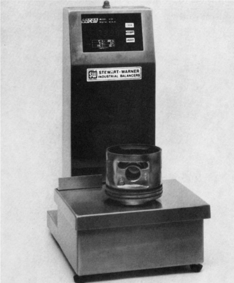
**8-79** Balancing begins with match-weighing piston assemblies.
