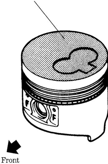
**8-41** Ford 2.3L pistons are insulated with a plasma coating and relieved at areas adjacent to the pins. Note the letter “F” embossed on the relief, which should face the front of the engine when the piston is installed.
