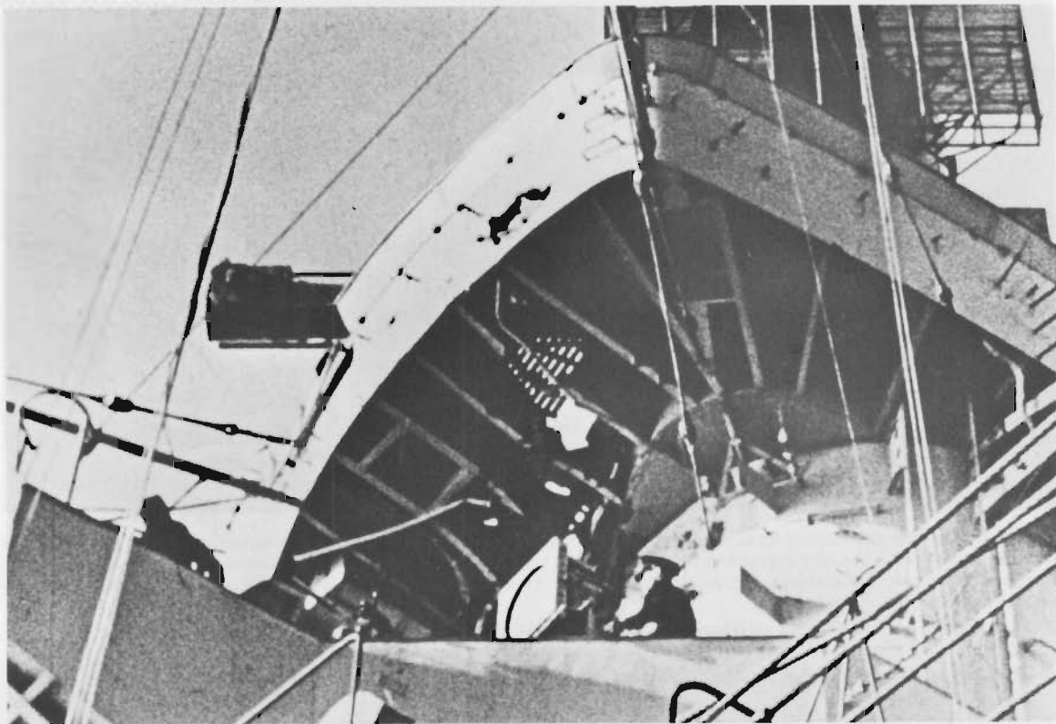
A hit on the foremast of the Gneisenau from a 15in shell fired by HMS Renown off Norway in April 1940. Note the 'mattress' radar aerial showing above the platform (Author's Collection)
