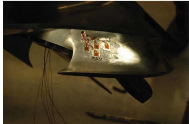
Figure 5. Strain gauges on impeller pressure side.
