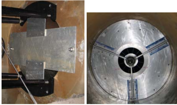
Figure 5: Final test configuration blockage plates.
