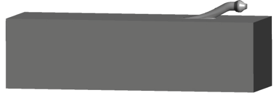
Figure 2: Control volume for waterjet numerical simulation
