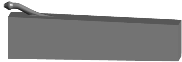
Fig.1 Computational domain of the waterjet
