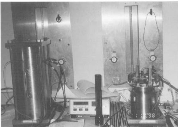
**Figure 16.68** Resonant column test
