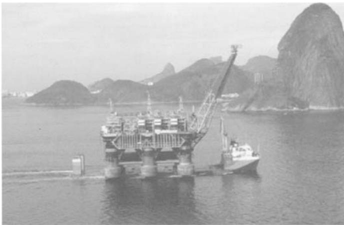
**Figure 14.24 Dry transport of P-40 on self-propelled vessel mighty servant 1**
