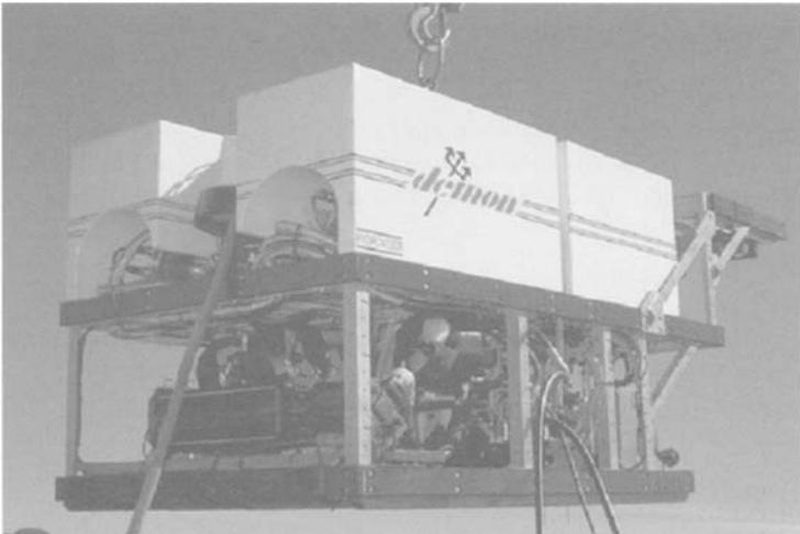
Figure 16.12 Example of an ROV (Sea Demon)
