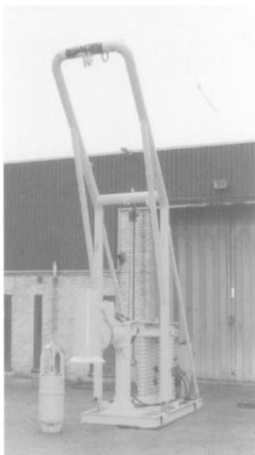
Figure 16.41 Abrams coring system
