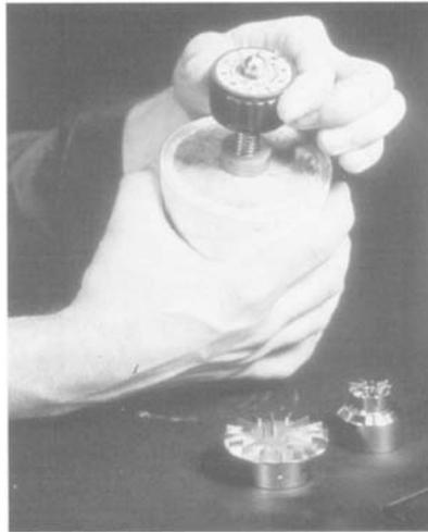
Figure 16.62 Torvane test
