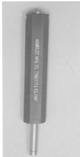
Figure 16.63 Pocket penetrometer
