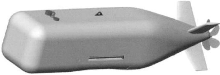
**Figure 16.13** Example of an AUV (The 5.6 m long Boeing-Oceaneering-Fugro AUV)
