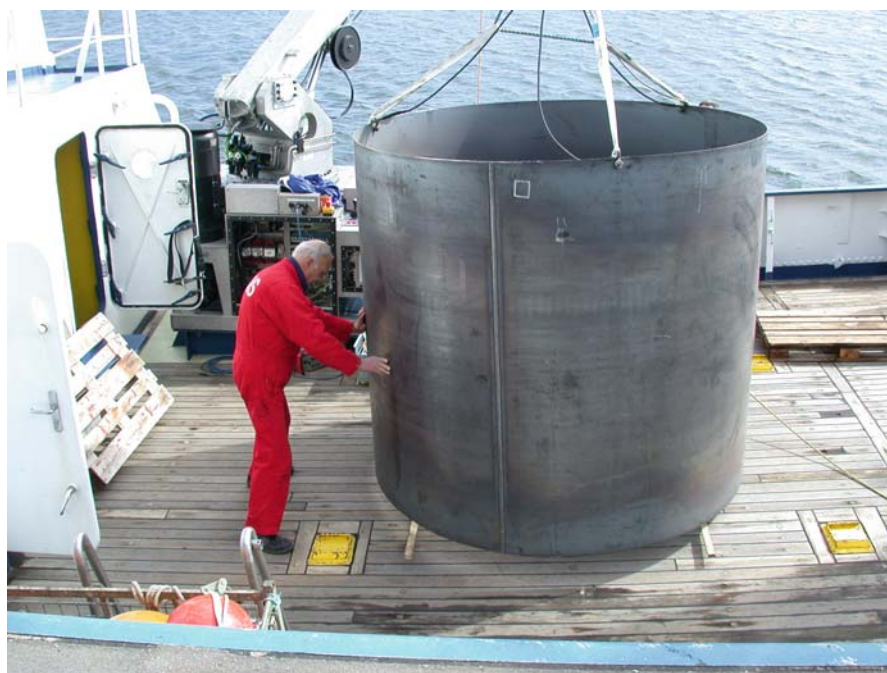
Fig. 2. Steel segment, which was deployed in April 2003 at 20 m depth to simulate the foot area of an offshore wind engine pile
