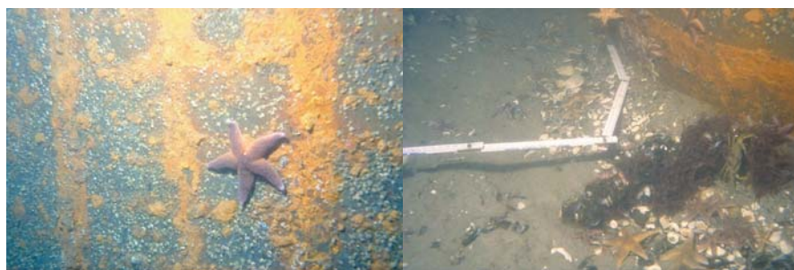
Fig. 8. Settling patterns on the bottom cylinder after 264 days. The starfish ( Asterias rubens ) becomes more frequent on the cylinder walls (1-2 individuals per m 2 ). The left photograph shows that reddish rust flakes have formed, and are starting to peel from the wall, with the attached organisms. The right picture shows the basement of the cylinder, where the currents have created a trough by sediment erosion which has started to fill with the debris from the cylinder walls, thereby attracting large predators, such as crabs ( Carcinus maenas ) and starfish. The larger shells of some mussels have been washed out of the sediment
