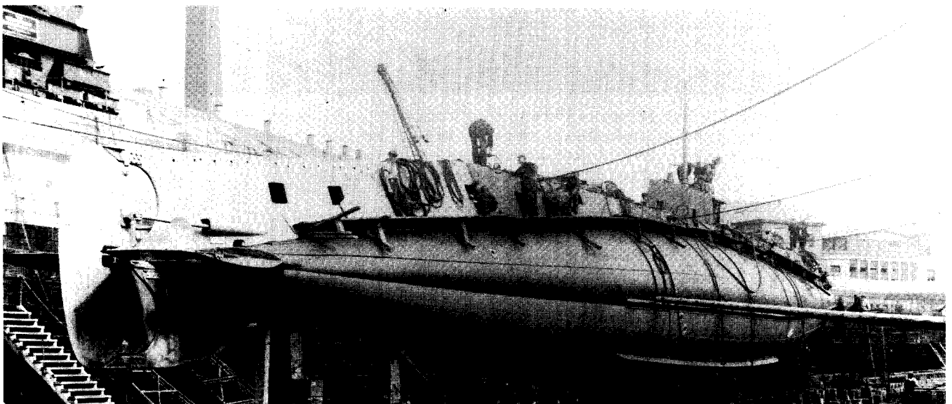
In dry dock at Portsmouth, New Hampshire, 5 September 1918, O-1 displays the standard Holland (Electric Boat) stern, nearly symmetrical around the long axis of the hull, with identical rudders top and bottom and with propellers set in line with the axis of the hull. Note the massive skeg along the top of the hull, aft.
