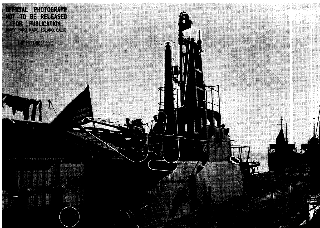
Shown on 23 and 29 November 1944 (overall view), Gato was typical of submarines in mid-war. Her open bridge was cut to a minimum. Numerous extra limber holes were cut into her superstructure for faster diving. Patterns varied from boat to boat. The bridge fairwater accommodates a 20-mm gun forward and a single 40-mm aft. The deck gun is a 4 in/50 taken from an S-boat. Modifications made at the refit she had just completed included installation of a new freestanding mast for her SD radar and relocation of her SJ to a new mast supported by her periscope shears. In some boats the new SJ mast was mounted forward of the periscope shears. The three girders supporting the shears are the only remnants of the prewar enclosed bridge; their height indicates how far the fairwater has been cut down. Note also the ammunition-passing scuttle let into the deck abaft the bridge fairwater.
