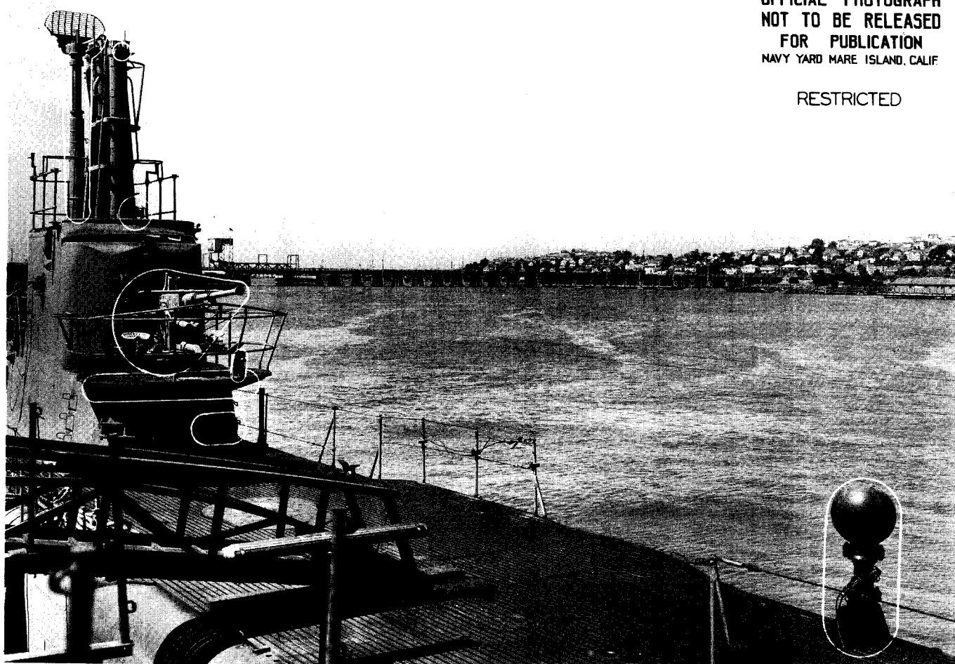
At Mare Island on 20 June 1945, Hoe displays two typical main late-war submarine sonars: the JT line array (left) and a topside WCA in its spherical dome (right). At the end of the war, both were being replaced by the vertical cylindrical dome of the new WFA integrated sonar.
