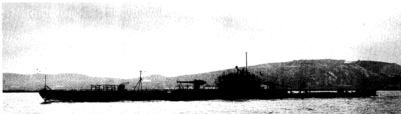
Narwhal , as modified, shown here on 3 April 1943 off Mare Island Navy Yard. Her SD radar mast is raised. Note the external tubes forward and right aft.
