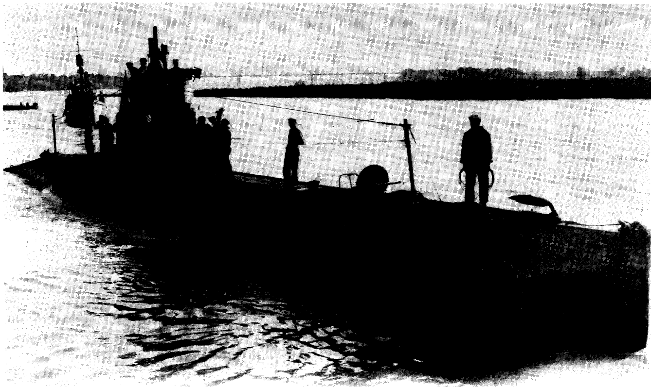
On the Mississippi near St. Louis in 1919, K-5 displays some standard World War I modifications: passive sound gear forward (the three "rats" of a Y tube forward of the forward planes and an SC tube forward of the forward hatch); a permanent chariot bridge; and housing periscopes.
