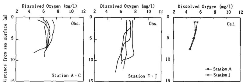
Figure 4: Vertical profiles of dissolved oxygen in August 27-29, 1996 (Case 1).
