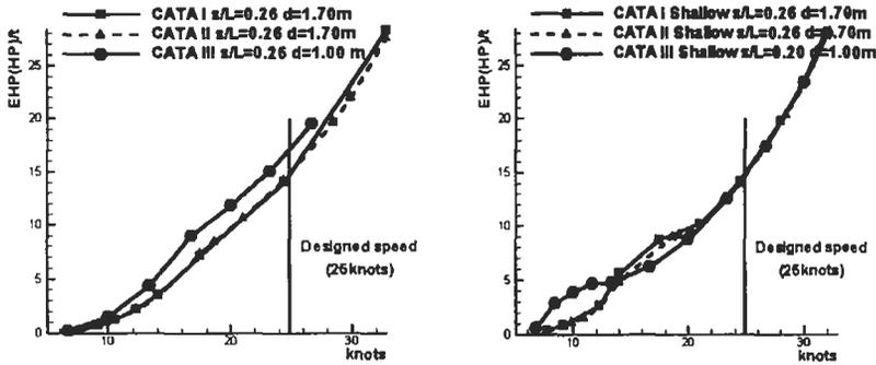
Figure 12: Comparison of Effective Horsepower per unit displacement
