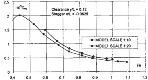
Figure 10: Comparison between geosims results – ITTC '78 correlation
