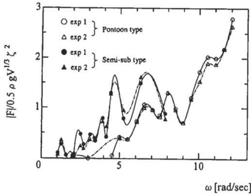
Figure 8: Comparison of measured drift forces of pontoon type and semi-submersible VLFS
