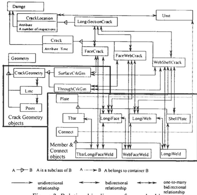
Figure 3: Relationship diagram for crack objects
