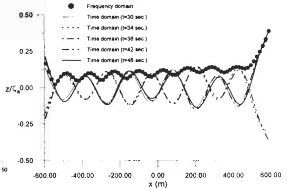
Figure 4: Comparison of relative vertical displacements in frency domain with those in time domain
