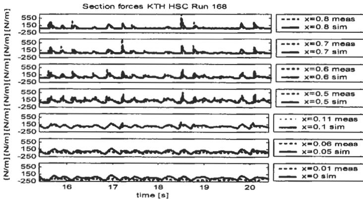
Figure 5: Comparison of calculated section forces and section wise integration of the pressure measurement. The x-position refers to the coordinate system in Figure 1. Quantities are in model scale.
