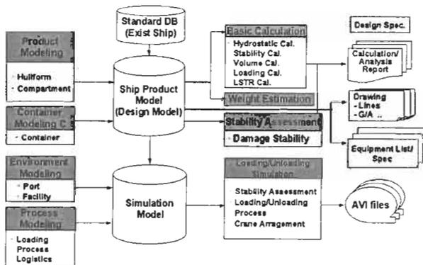
Figure 1. System Configuration of Container Loading/Unloading
