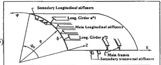
Figure 3: Basic stiffened panel (or basic element).
