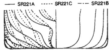
Figure 3 : Body plans of SR221-A,B,C hulls
