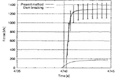
Figure 12: Calculated forces from water impact on deckhouse wall. Water propagation based on boundary conditions from wave kinematics analysis, and on dam breaking.
