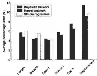
Figure 4: Comparison of average percentage error for power function regression, neural network and Bayesian network.
