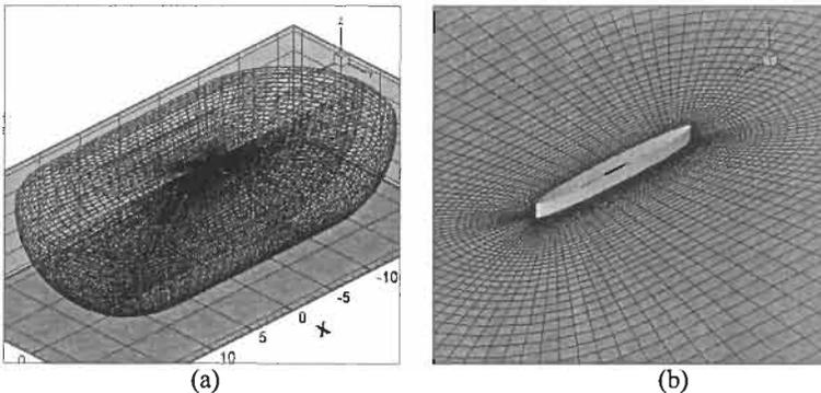
Figure 1. Computational Grid in the Physical Domain: 100x100x40 (a)
