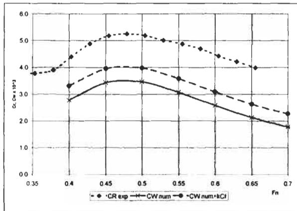
Figure 3: Comparison of  $C_R$ ,  $C_W$ ,  $C_{WK}$  (form factor) vs.  $F_n$
