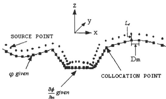
Figure 2: Model for numerical simulation
