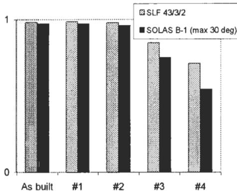
Figure 2: Comparison between Attained Index A obtained by different simplifications of the compartment layout and different probabilistic damage stability regulations
