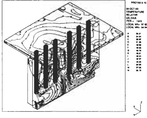
Figure 7 : Temperature distribution by new system
