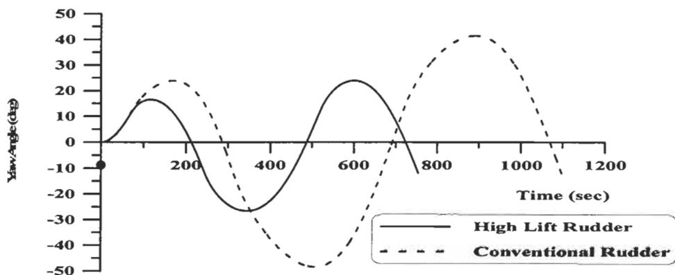
Figure 3: The  $10^{\circ}/10^{\circ}$  zig-zag characteristics for two rudders of 2.3% area
