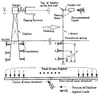
Figure1 Combined model composed of VLFS and mooring system
