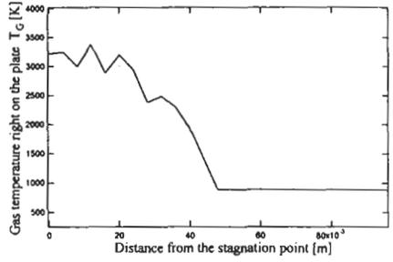
Figure 13: Estimated distribution of gas temperature right on the plate
