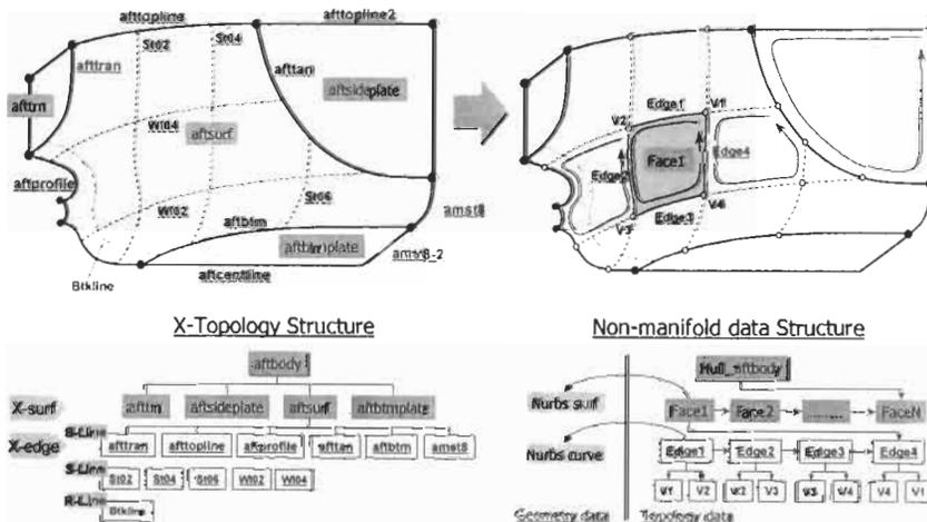
Figure 1: Example of an afterbody wireframe model using the X-topology and corresponding surface model represented by non-manifold data structure
