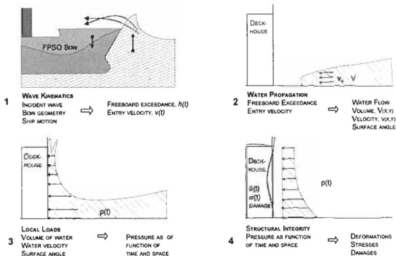
Figure 1: Calculation procedure, water on deck
