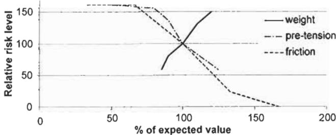
Figure 4: Relative risk of cargo shifting as a function of cargo parameters (route in zone B,  $GM_0 = 0.68$ , 15 knots)
