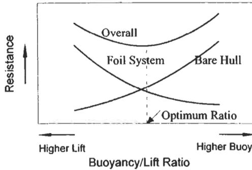
Figure 2: Concept of the Optimum Buoyancy/Lift Ratio
