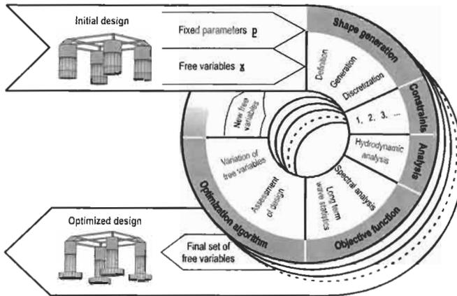
Figure 2. Automated hull shape optimisation framework
