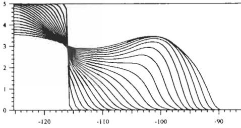
Figure 9: Water flow along centreline of the vessel: Surface elevation according to dam breaking model.
