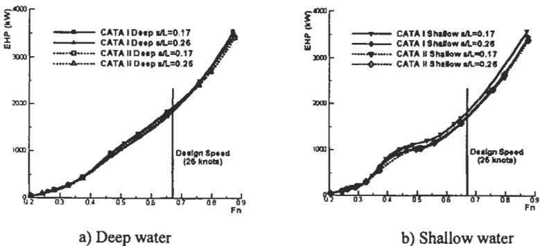
Figure 7: Effective horsepower of CATA I and CATA II (demi-hull spacing  $S/L = 0.17, 0.26$ )
