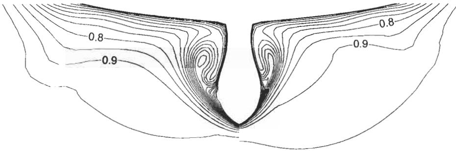
Figure 3: Axial velocity field at Station I ( $x/L_{pp} = 0.95$ ) at model scale (left) and full scale (right)
