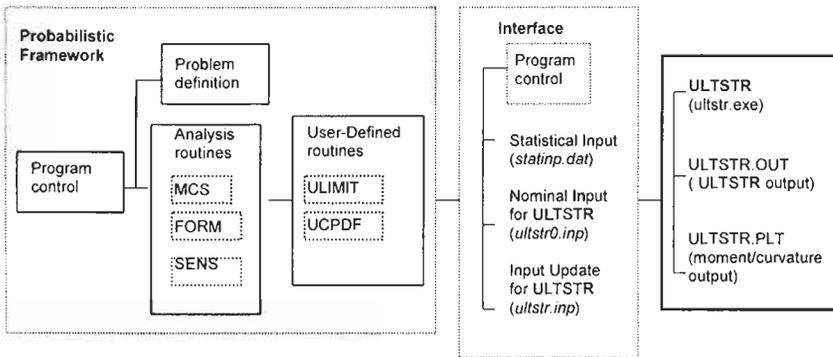
Figure 4: Block Diagram of PULSTR
