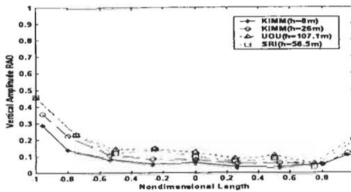
Figure 5 : The Vertical Displacement RAO( $\lambda_{\infty} / L = 0.2$ , Incident Angle=0 degree)
