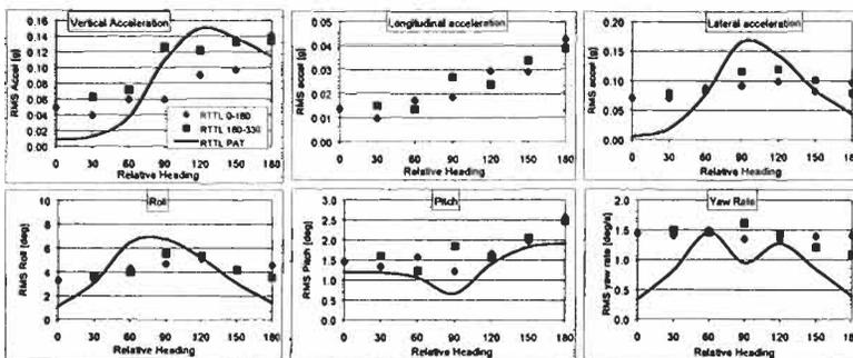
Figure 5: Predicted and measured motions
