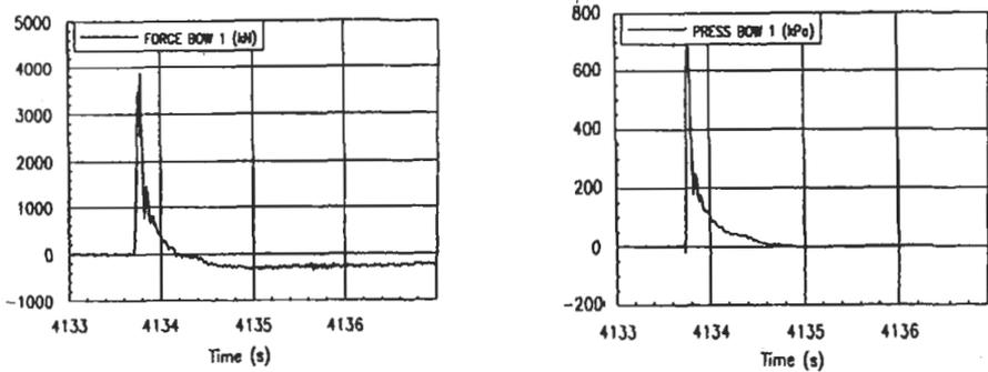
Figure 8: Impact signals from force and pressure sensors on bow
