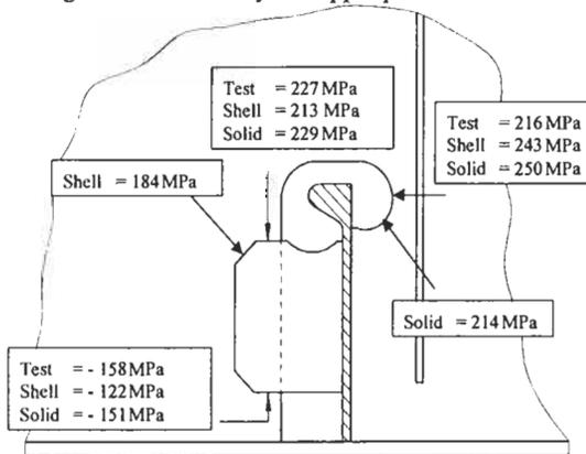
Figure 7: Comparison of calculated hot spot stress with measured stress
