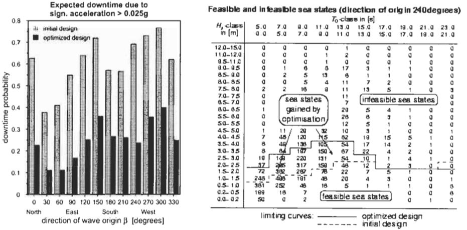
Figure 6. Result of downtime minimization of a semisubmersible
