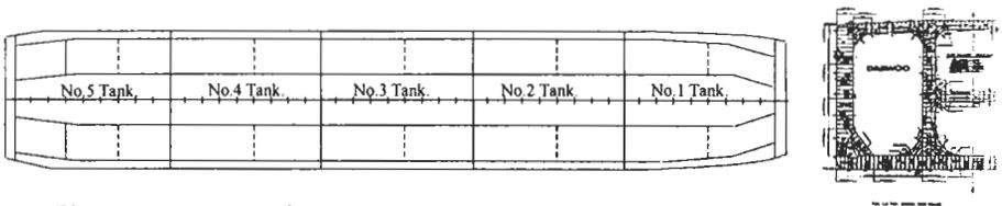
Figure 1: Structural arrangement and Midship section for new VLCC
