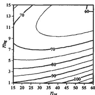
Figure 2: Hull steel weight (ton)
