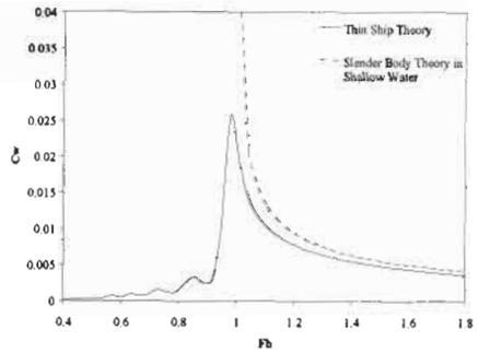
Figure 6: Wave resistance by thin ship theory and the shallow water slender body theory by Tuck (1966) ( $H/L=0.1$ )
