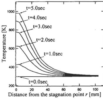
Figure 5: Distribution of plate back face temperature during the spot heating experiment
