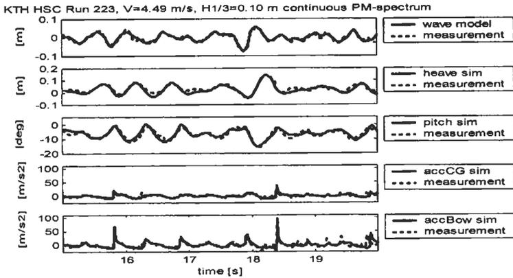
Figure 6: Simulation of a sequence in severe head seas where the complete hull leaves the water and reenters ( $18.1 < \text{time} < 18.5$ ). A wave equation of 30 wave components models the wave measurement of the continuous spectrum.
