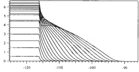
Figure 10: Water flow along centreline of the vessel: Surface elevation with boundary conditions from wave kinematics analysis.
