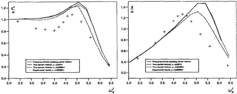
Figure 3: Heave and Pitch RAOs for a NPL5b mono-hull in regular head waves of variable amplitude.  $L=4.5m$ ,  $Fn=0.53$ .
