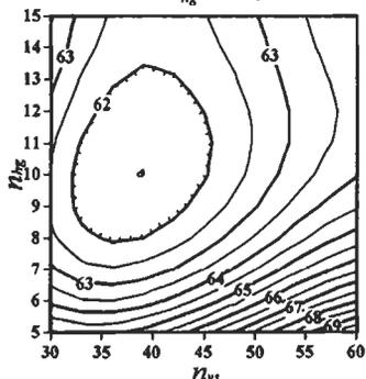
Figure 6: Hull steel weight (ton)
