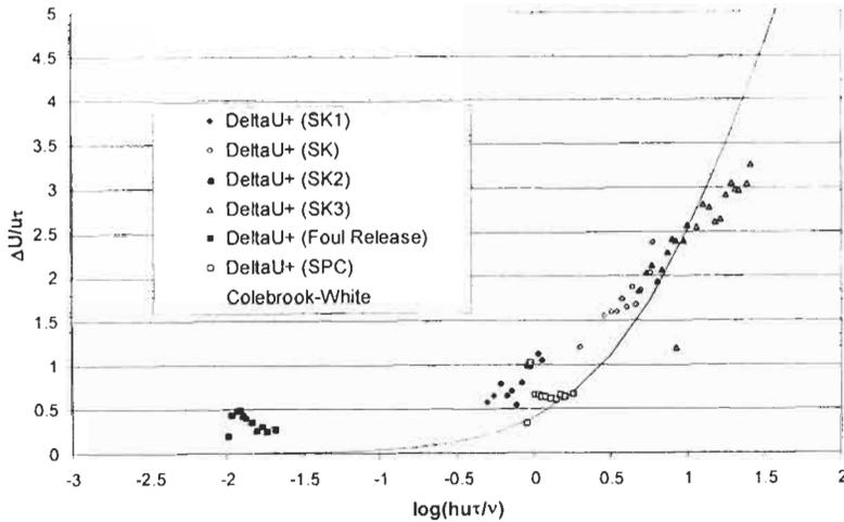
Figure 4: The roughness function of the surfaces tested by the authors and by Dey (1989) plotted against  $\log(hu_r/\nu)$
