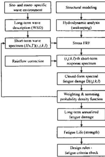
Figure 9: Procedure of spectral fatigue analysis
