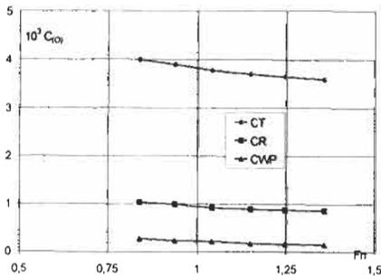
Figure 4: Outrigger;  $C_T, C_R, C_{WP}$  versus  $F_n$
