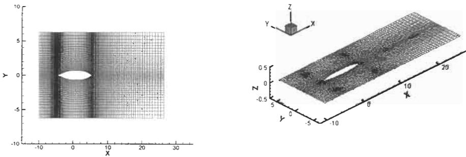
Figure 5: the mesh of the free surface,  $Fn=0.316$ ,  $t=0$ , (Series 60 ship model)
