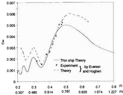
Figure 3: Comparisons of predicted wave resistance with experimental and theoretical results by Everest and Hogben ( $H/L=0.425$ )
