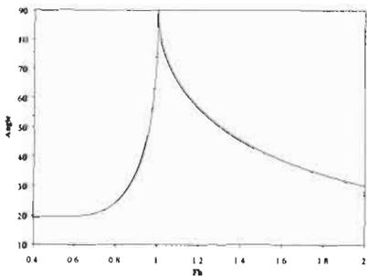
Figure1: The relationship between the wave angle and the water depth Froude number
