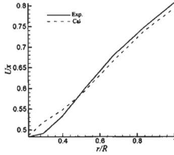
Figure 1: Comparison of numerical circumferential-mean velocity at propeller plane with experimental data
