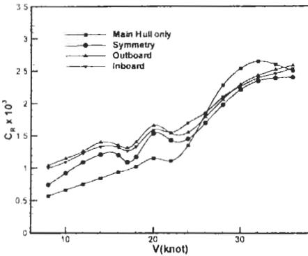
Figure 5:  $C_R$  curves for three side-hull forms
