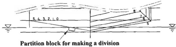
Figure 7: Body plan of the modified model "S" for estimating flow rates of air for the test boat
