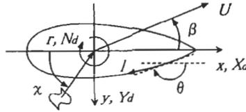
Figure 2: Coordinate system describing ship motion and wave forces and moment
