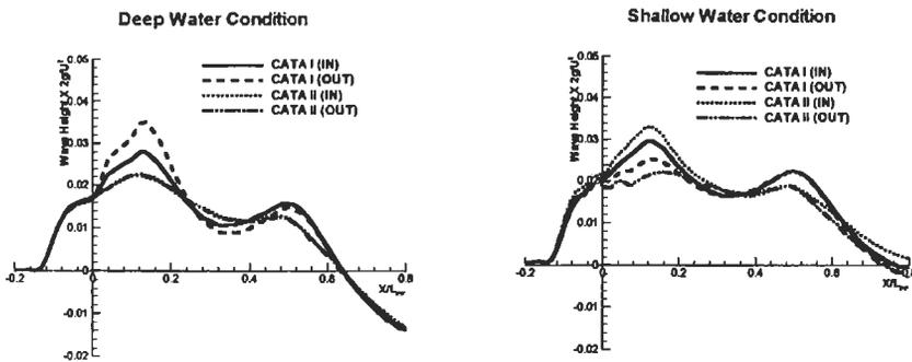
Figure 4: Comparison of computed wave height profiles of CATA I and II for shallow and deep water conditions ( $S/L=0.26$ )
