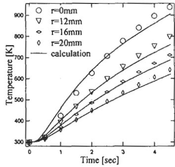
Figure 14: Comparison of calculated and measured plate back face temperatures
