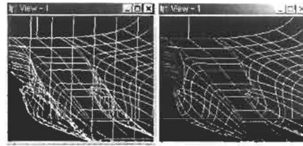
Figure 7: A twin skeg hull without wireframe shading (left) and with wireframe shading
