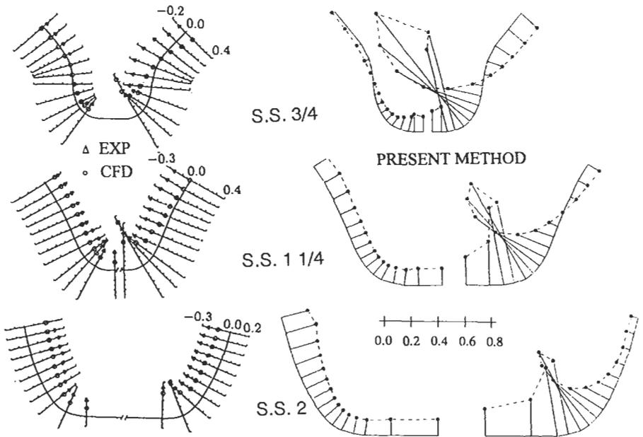
Figure 5 : Comparison of pressure distributions (Ship B)
