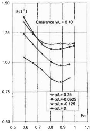
Figure 5: Running trims for different clearances
