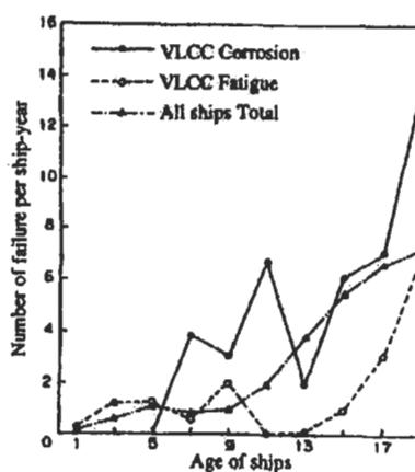
Figure 4: Frequency of failure due to fatigue and corrosion of VLCC per ship-year
