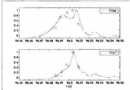
Figure 8: Comparison between laminate strain measured at the full-scale trials and FEA results with the re-constructed pressure distributions. Note that the values given are normalised.
