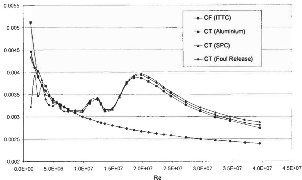
Figure 1: Total resistance coefficients against Reynolds number in the CEHIPAR Calm Water Tank
