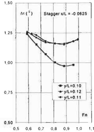
Figure 6: Running trims for different staggers
