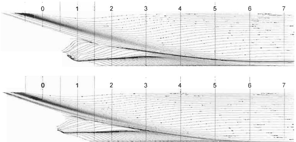
Figure 2: Comparison of limiting streamlines in loaded condition at model scale (top) and at full scale (bottom)
