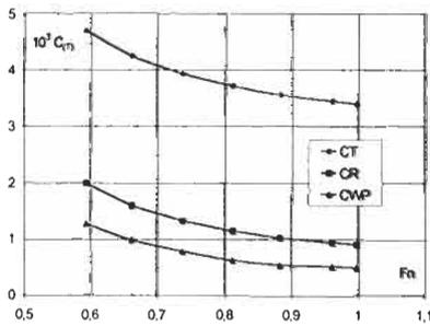
Figure 2: Trimaran hull:  $C_T, C_R, C_{WP}$  versus  $F_n$
