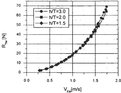
Figure. 3: Total model resistance as a function of the effective speed for the subject inland ship
