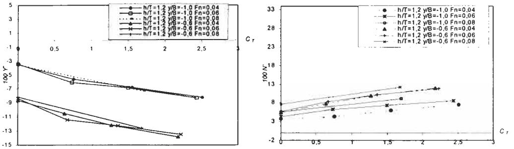
Figure 8: The  $Y'$  and  $N'$  variation with the propeller loading coefficient  $C_T$  at  $h/T=1.2$
