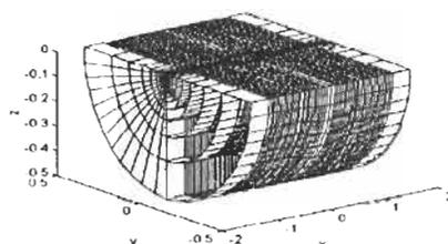
Figure 2: Grid around the Wigley hull
