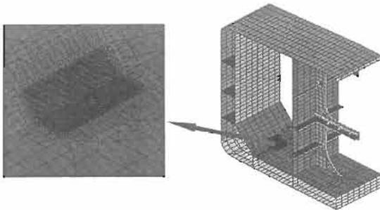
The sub-model extends two transverse floor spaces longitudinally to investigate the effect of docking bracket as shown in Fig. 3. Mesh sizes for critical zones are carefully controlled to get relevant geometric stress even by using  $t \times t$  fine mesh.
