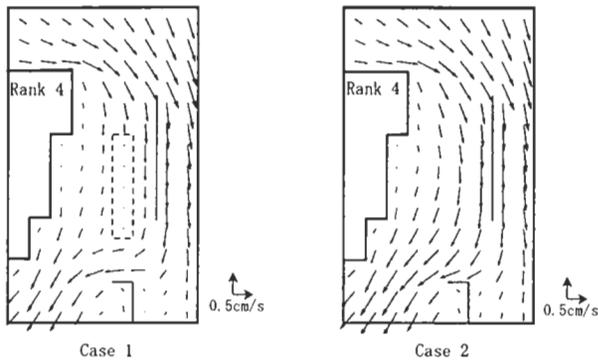
Figure 3: Horizontal distributions of residual current in the sea area adjacent to Mega-Float model.
