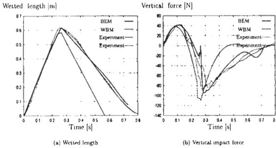
Figure 5: Comparisons between experiments and theory. Wave period  $T=1.25s$ , wave height  $H=0.14m$ , and deck height  $\eta_{ag0} = 0.06 m$ .
