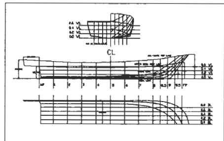
Figure 2: Lines of the developed hull
