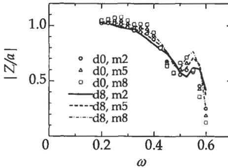
Figures 7: Vertical displacements in 60 degrees wave; zero draft and 8m in draft, (mass effect)
