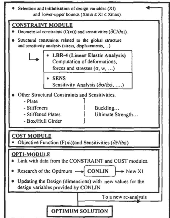
Figure 2: Chart of the LBR-5 model with CONSTRAINT, COST and OPTI modules.
