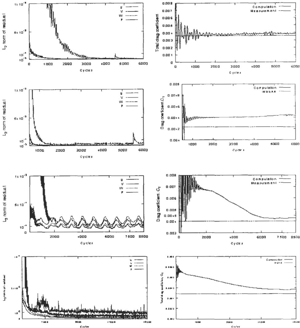
Figure 2: Convergence histories of (U, V, W, P) residuals and  $C_t$  at the fine mesh. The KCS model, the DTMB 5415 model, the tanker model and the HTC model from top to bottom
