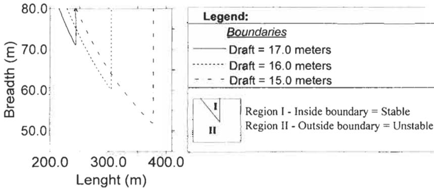
Figure 3: Stability map for three different drafts
