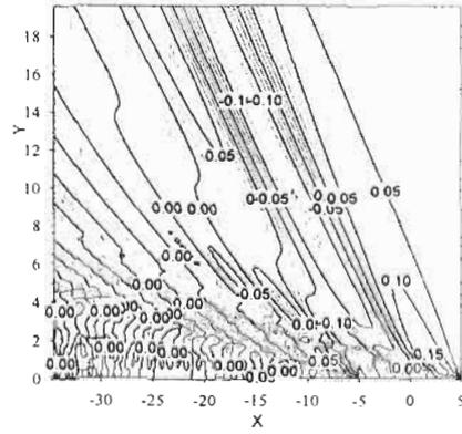
Figure 10: Predicted wash for  $F_h=1.2$ . The ship is located at  $-5 < x < 5$  and  $H/L=0.1$ .
