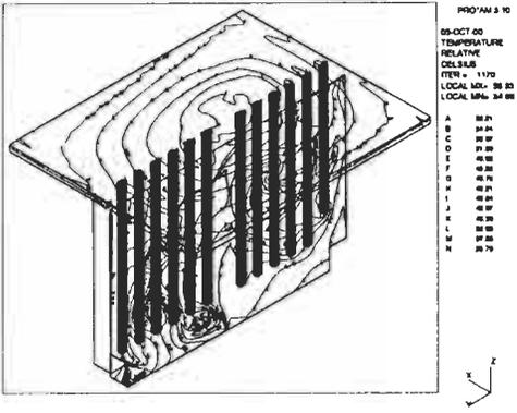
Figure 6 : Temperature distribution by original system
