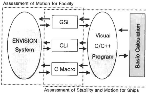
Figure 5. The Process of Interface between ENVISION System and CAE Programs
