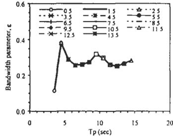
Figure 6: Variation of bandwidth parameters of stress responses vs.  $T_p$  and  $H_s$  (Wave spectrum used : JONSWAP; Wave: W156)
