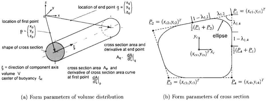
Figure 3. Shape definition of a single component by form parameters
