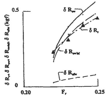
Figure 2: Comparison of estimated stern wave resistance  $\delta R_{sw}$  with measured
