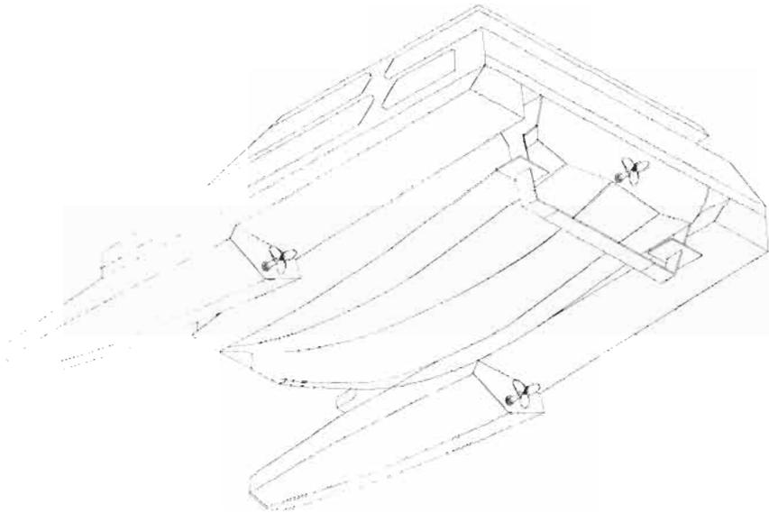
Figure 3 Stepped Hull Hybrid Hydrofoil Catamaran Ferry Concept
