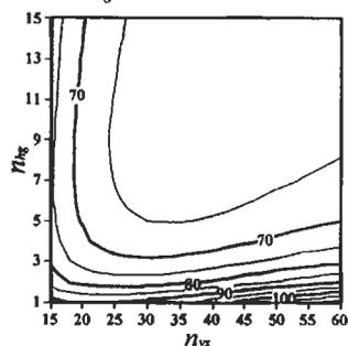
Figure 4: Hull steel weight (ton)
