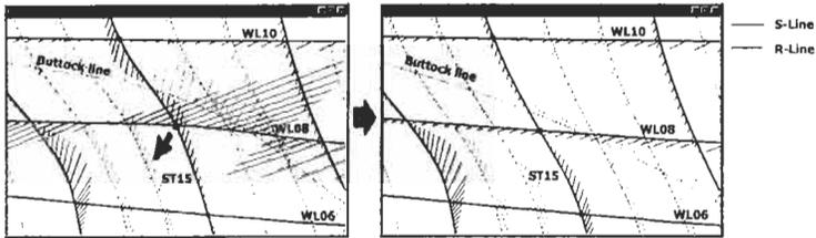
Figure 3: Example of the association based cross fairing showing that all lines related to the changed station line ST15 are updated automatically
