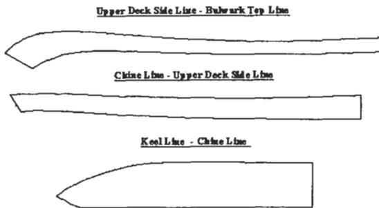
Figure 3: Developed plates of a typical fishing boat
