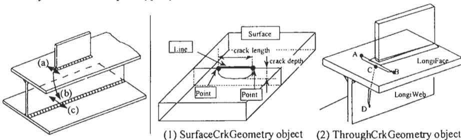
Figure 2: Typical crack propagation and the definition of the crack geometry objects
