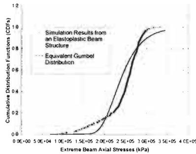
Figure 3b: Statistical Distribution of Extreme Peak Values for the Elastoplastic Beam Model
