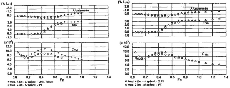
Figure 6: Comparison of  $C_T$ , sinkage and trim among the 2 m IPT/ST Model, 1.5 m U.Tokyo (left) and 4 m SRI Model (right)
