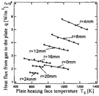
Figure 11: Relation between estimated plate heating face temperature and estimated heat flux
