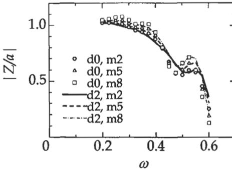
Figures 5: Vertical displacements in 60 degrees wave; zero draft and 2m in draft, (mass effect)
