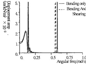
Figure 4: Frequency response amplitude of deflection at the top end of dolphin located at the free end of the structure under low mooring rigidity
