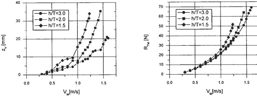
Figure 2: Characteristics of sinkage and measured resistance of the subject inland ship model
