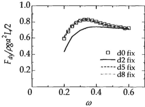
Figures 10: Steady wave drift forces of sway on fixed body in 60 degrees wave (effect of draft)
