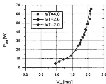
Figure 10: Delivered power at propeller as a function of the blockage speed
