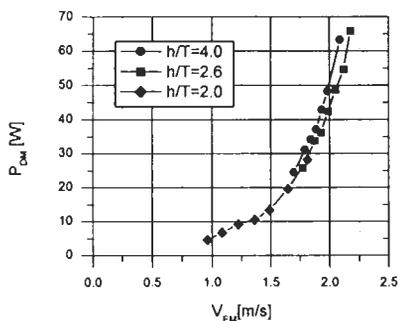
Figure 9: Delivered power at propeller as a function of the effective speed
