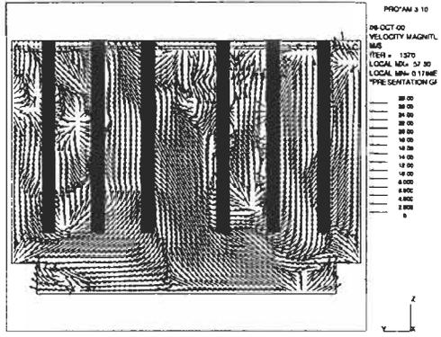
Figure 9 : Flow pattern by modified system
