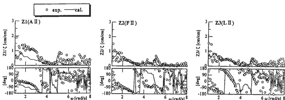
Figure 4: Z-displacements (Z1: fore, Z2: mid, Z3: aft) of semi-submersible type VLFS
