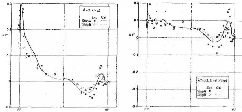
Figure 6 : Longitudinal distribution of lateral force in oblique and turning motions
