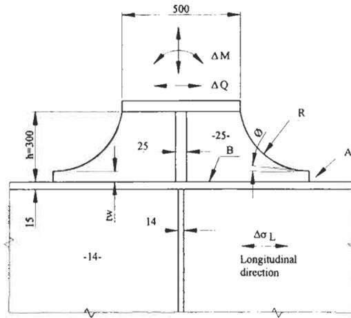
Figure 5: Topside support geometry
