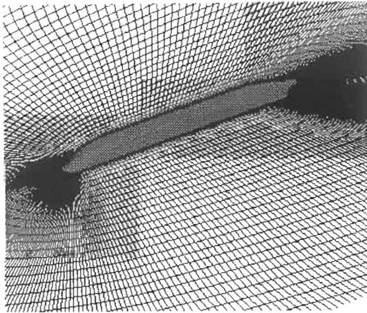
Figure 1: An initial single O-O mesh
