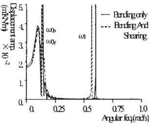
Figure 2: Frequency response amplitude of deflection at the top end of dolphin located at the free end of the structure under low mooring rigidity
