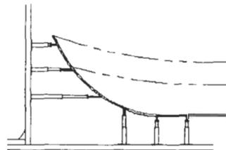
Figure 5: Schematic diagram of the mould system (transverse view)
