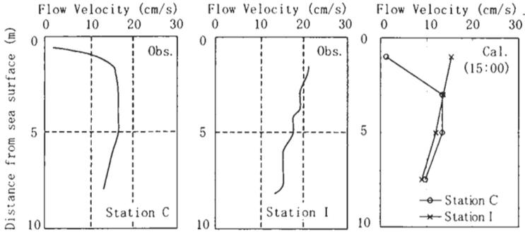
Figure 2: Vertical profiles of the flow velocity at Stations C and I in the flood tide on January 9, 1997 (Case 1).
