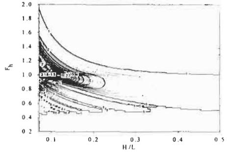
Figure 4: Shallow water wave resistance ratio  $r = R_h / R_{\infty}$  as a function of  $H/L$  and  $F_h$  (see more details in Fig. 5)
