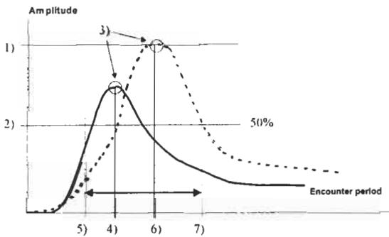
Figure 2: Determination of relevant range of ship motion periods
