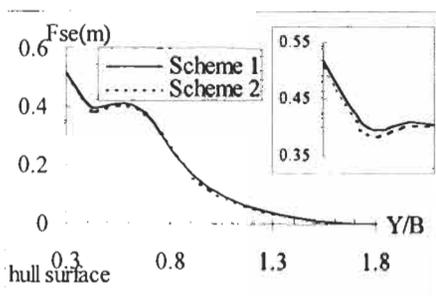
Figure 2: The free surface elevation (Fse) along Y-axis at 19 1/4-station
