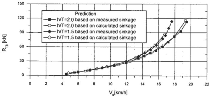
Figure 8: Comparison of the predicted ship-resistance using measured and calculated sinkage
