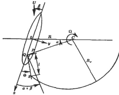
Figure 1 : Coordinate and trailing vortex model
