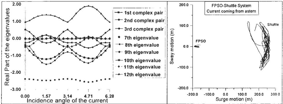
Figure 4: a) Eigenvalues of the system and b) Sway versus Surge motion
