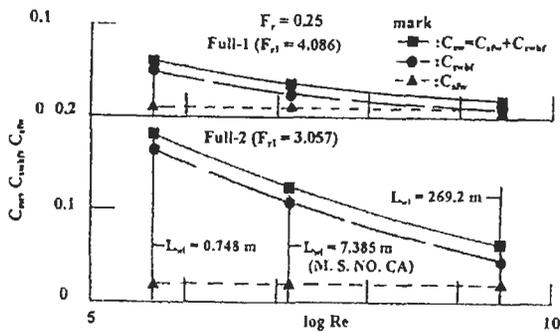
Figure 6: Scale effect of stern wave resistance and its components (M.S.NO.CA and similar hulls)
