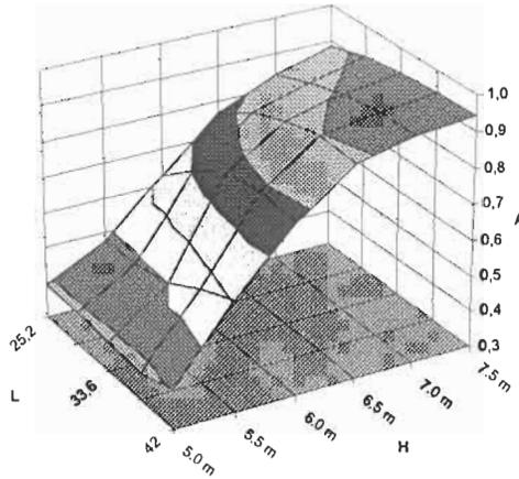
Figure 4: Attained Index A as a function of length L of machinery space and height H from tank top to main deck. SOLAS Part B-1
