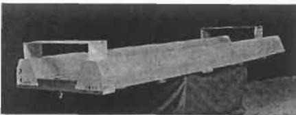
Figure 3: Catamaran Ship Model with Hydrofoil System
