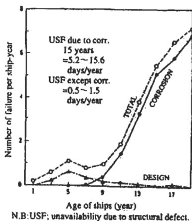
Figure 3: Frequency of failure per ship-year v.s. ship's age (for all ships)
