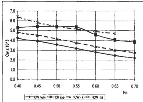
Figure 8: Comparison of  $C_R$ ,  $C_W$ ,  $C_{WK}$  (form factor) and  $C_{WK-s}$ , (form factor + spray factor) vs.  $F_n$
