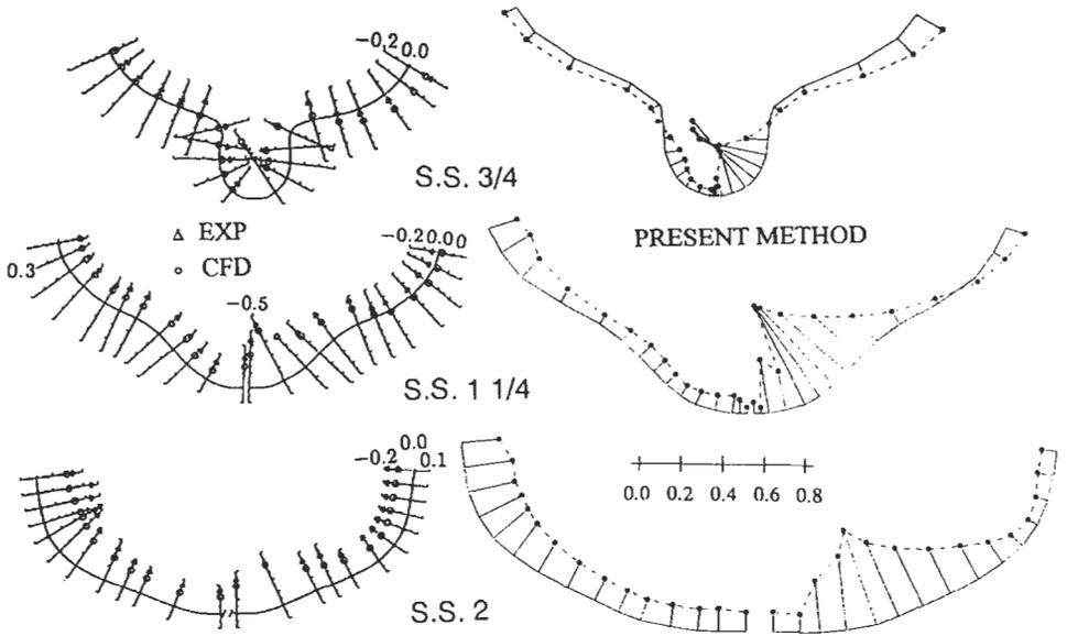
Figure 4 : Comparison of pressure distributions (Ship A)
