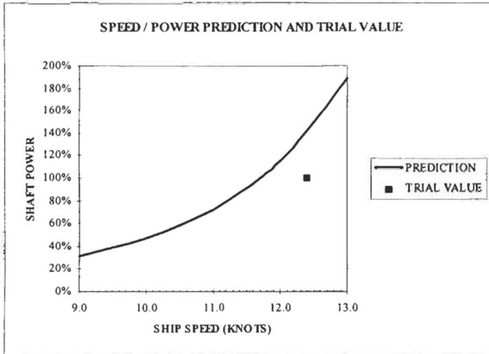
Figure 6: Power prediction together with the attained speed during speed runs
