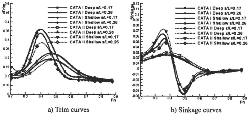
Figure 6: Comparison of hull attitudes of CATA I and II (demi-hull spacing  $S/L = 0.17, 0.26$ )
