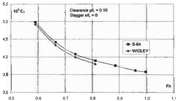
Figure 7: Comparison between the Wigley and Series 64 outriggers
