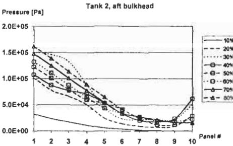
Figure 7: Comparison of computed max. pressures at aft bulkhead of tank 2 for various fill levels.
