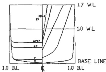
Figure 1: Body plan of a demihull of CATA I
