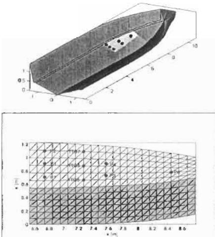
Figure 1: Location of pressure transducers (P1-7) and strain gauges (TTG5-7).
