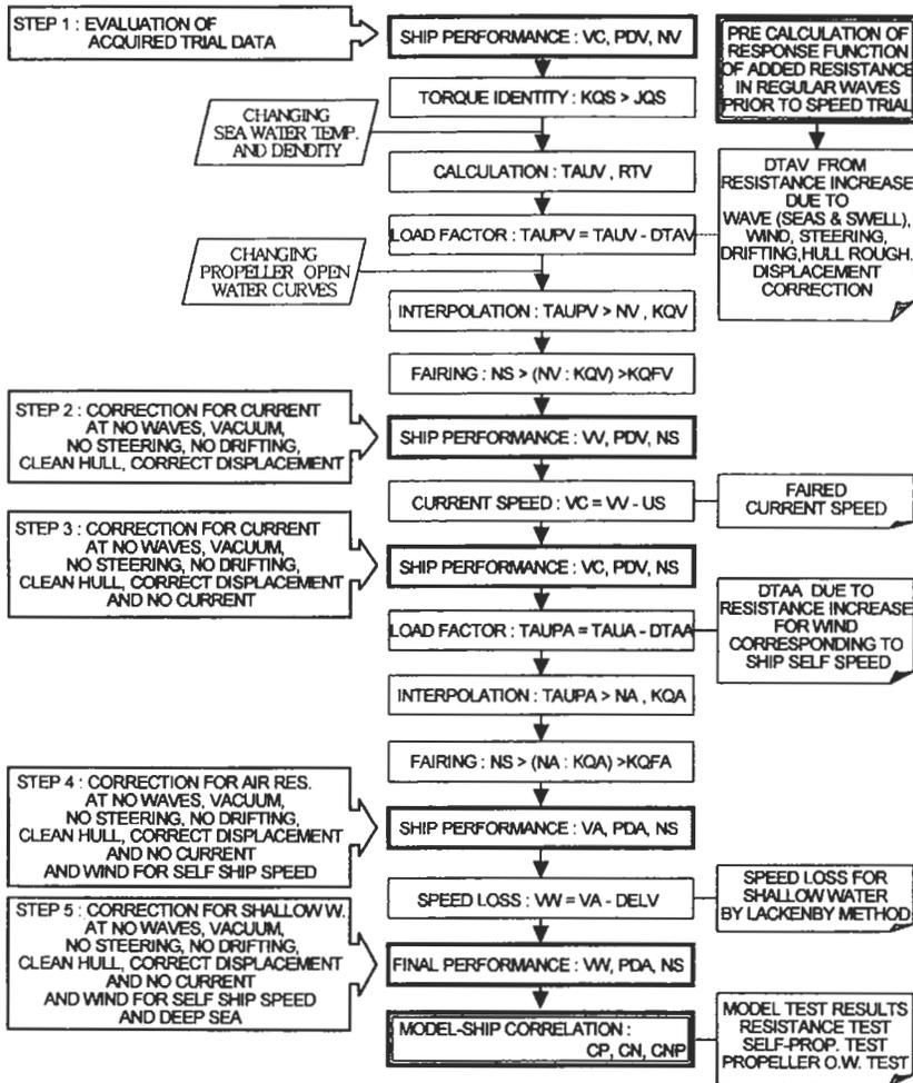
Figure 1: Flowchart of speed trial analysis
