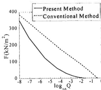
Figure 5 : Comparison between conventional and present method for long-term prediction of shipping water load ( $\chi = 180^\circ$ )
