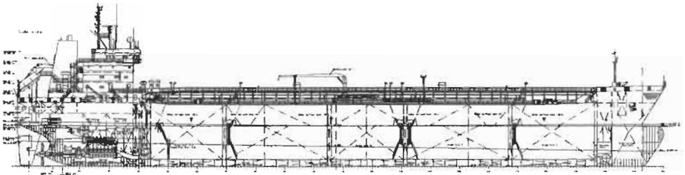
Figure 1: General arrangement of tanker SEATURBOT
