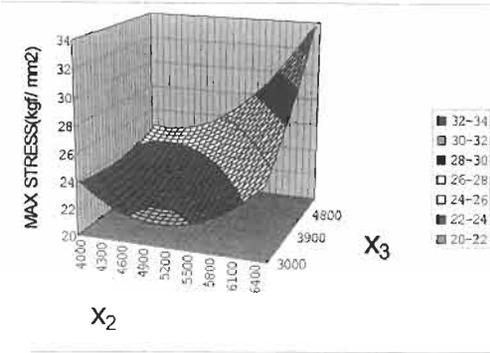
Figure 13: Response surface of maximum stress
