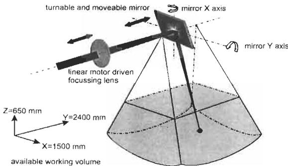
Figure 8: Principle of Remote Welding
