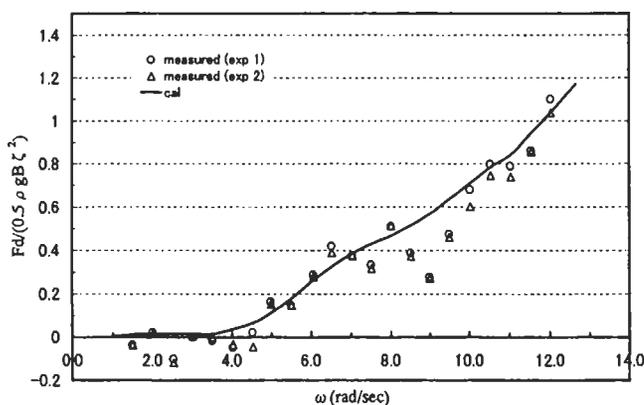
Figure 5: Wave drift force coefficients of pontoon type VLFS
