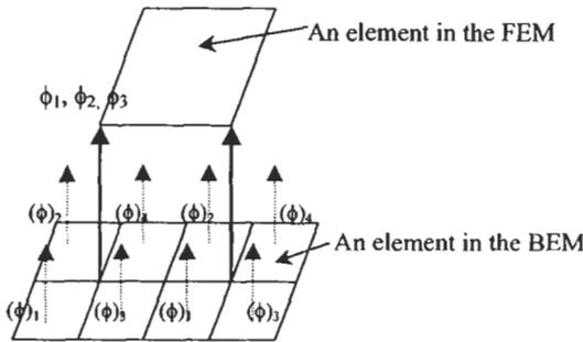
Figure 2: Discretization of a VLFS by quadrilateral elements.
