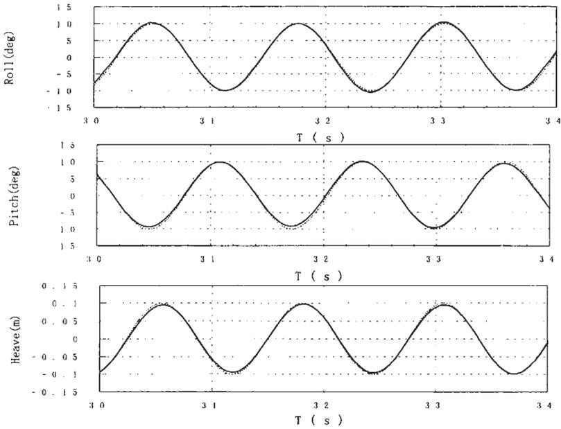
Figure 4: Motions of the 3DOF platform measured by present system and the driving signals
