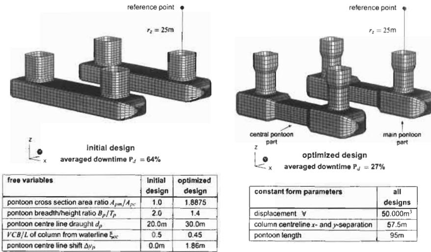
Figure 5. Geometric properties of initial design and the semisubmersible optimized with respect to downtime due to excessive accelerations at the reference point.
