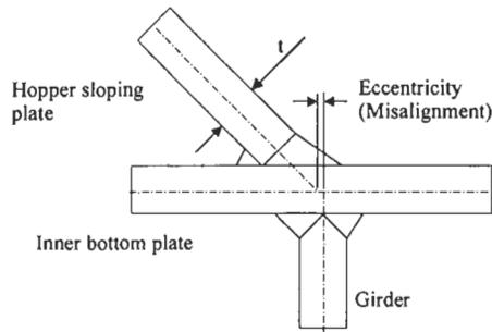
Figure 6: Eccentricity of hopper plate connection
