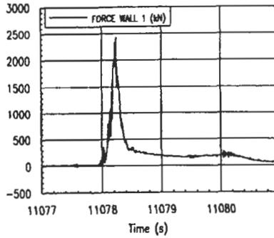
Figure 7: Impact signal from force sensor on deck house.
