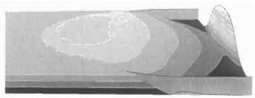
Figure 5: Simulation of water propagation for case vessel according to a dam breaking model. Deck movement neglected
