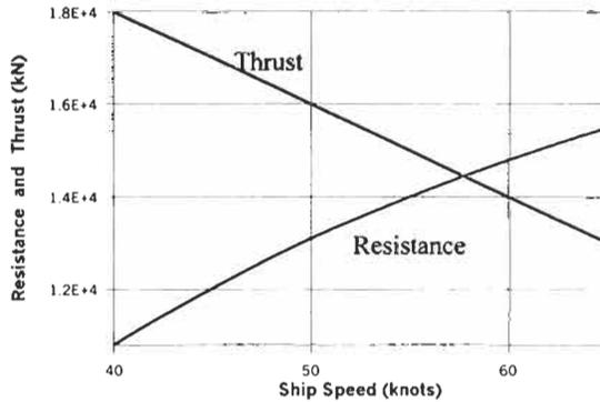
Figure 5: Trial Resistance and Available Thrust
