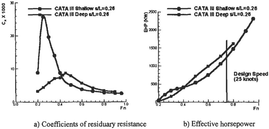
Figure 10: Coefficients of residuary resistance and effective horsepower of CATA III for shallow and deep water conditions(  $S/L = 0.26$ )
