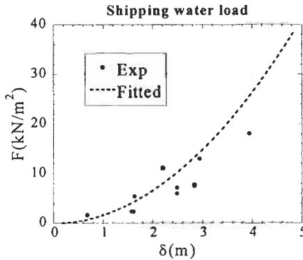
Figure 3 : Relation between shipping water load and relative water height at stem (Fn=0.1)
