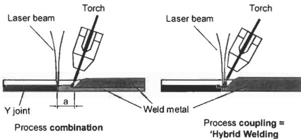
Figure 5: Combination methods of GMA- and Laser Processes
