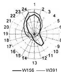
Figure 2: Wave directional probabilities for a FPSO
