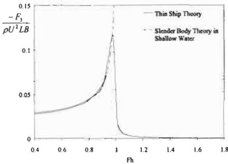
Figure 7: Vertical force  $F_3$  by thin ship theory and the shallow water slender body theory by Tuck (1966) ( $H/L=0.1$ )
