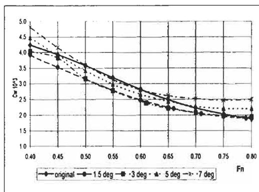
Figure 9:  $C_w$  vs.  $F_n$  for different stern wedge angles ( $\alpha$ )
