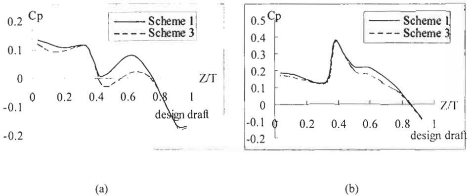
Figure 4: Distribution of  $C_p$  along Z-axis at 3/4-station (a) and 1-station (b)
