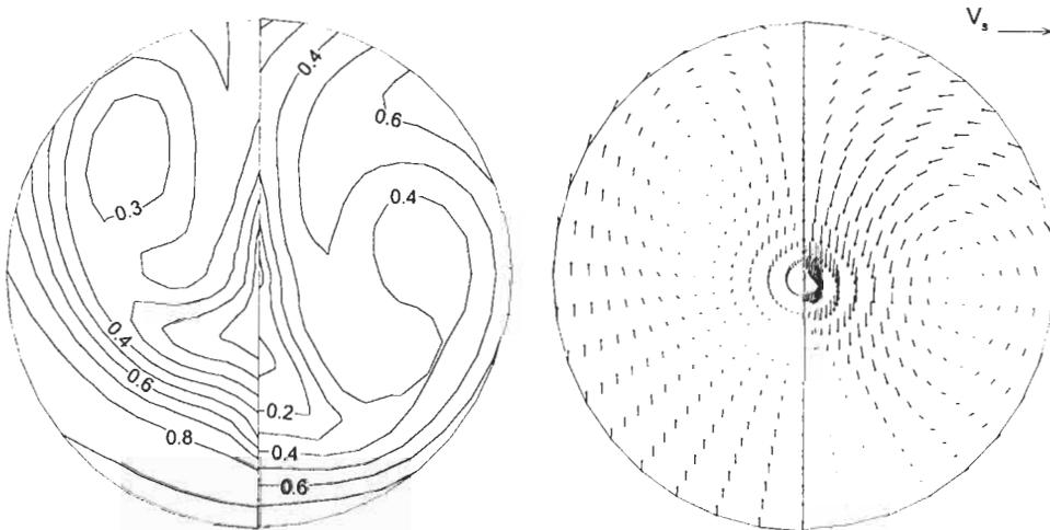
Figure 4: Wake field in the propeller plane calculated for loaded (left) and empty (right) condition
