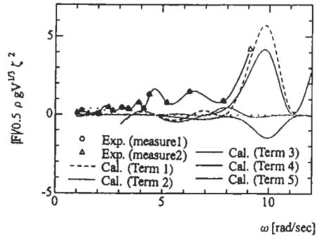
Figure 7: Wave drift force coefficients of semi-submersible type VLFS
