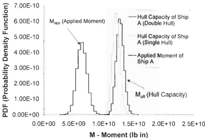
Figure 5: Comparison of PDF of  $M_{app}$  with PDFs of  $M_{ult}$  of Single and Double Hulls of Ship A
