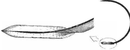
Figure 2 : Panel division and shape of trailing vortex sheet
