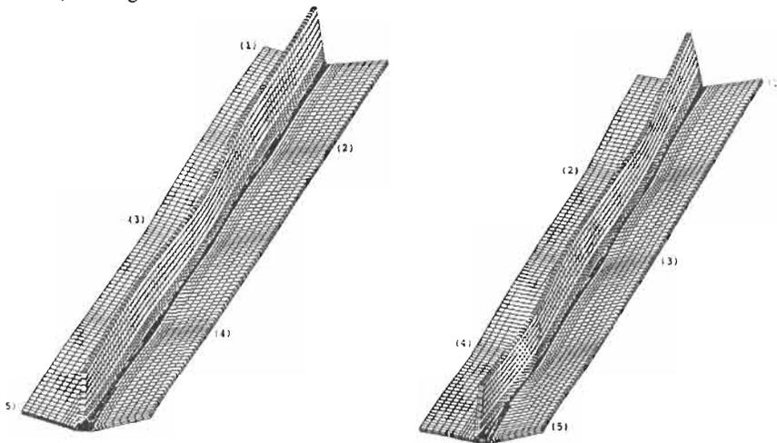
Figure 3: *Deformation mode depending on tack weld positions (scaling factor 30)*
