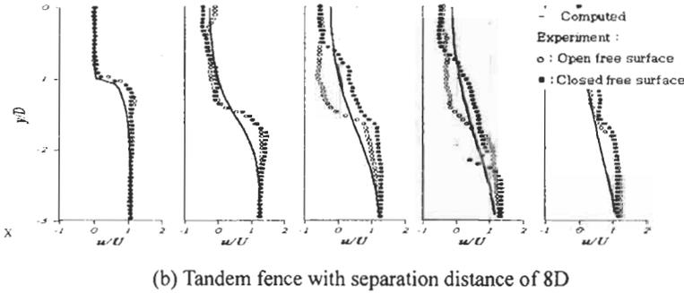
Figure 3: Comparison of horizontal velocity profiles obtained by computation and experiment at  $Fr = 0.16$
