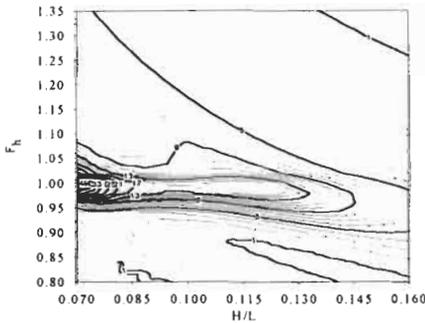
Figure 5: Shallow water wave resistance ratio  $r = R_h / R_{\infty}$  as a function of  $H/L$  and  $F_h$
