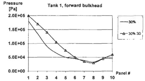
Figure 8: Comparison of 2D and 3D computed max. pressures at forward bulkhead of tank 1.
