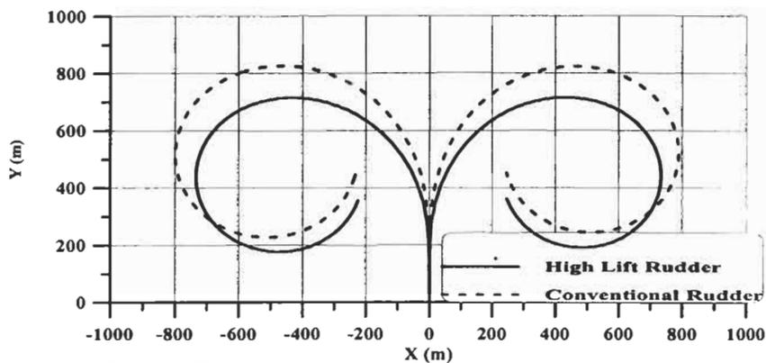
Figure 2: The turning characteristics for two rudders of 2.3% area
