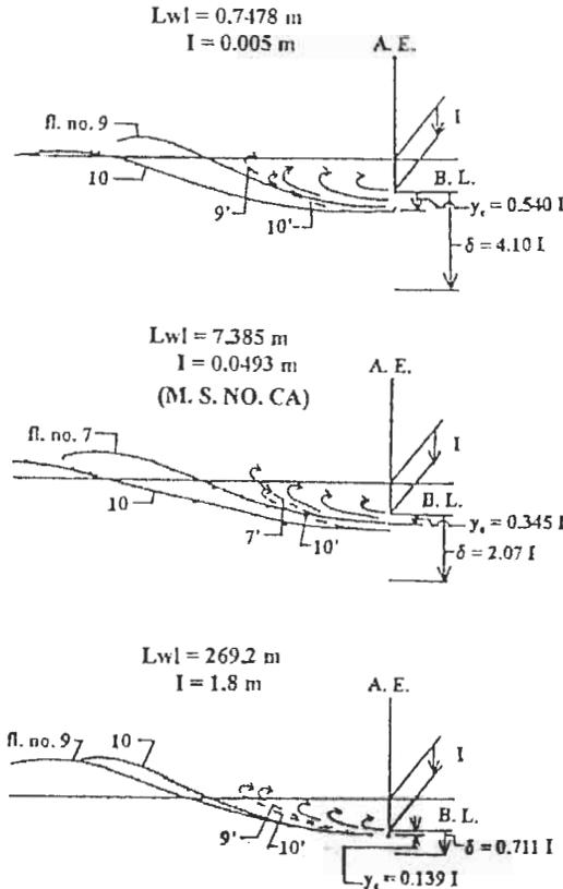
Figure 3: Scale effect of water flow just behind a transom stern on Full-2 (M.S.NO.CA and similar hulls)
