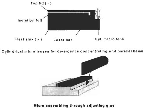
Figure 7: 50 W Diode Laser bar (28 x 13 x 1,5 mm)
