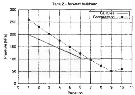
Figure 9: Comparison of computed maximum pressures with rule based design pressures.
