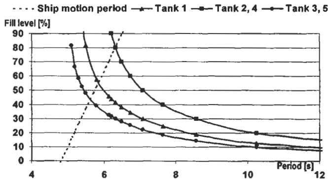
Figure 3: Natural period of fluid inside tanks compared with ship motion period
