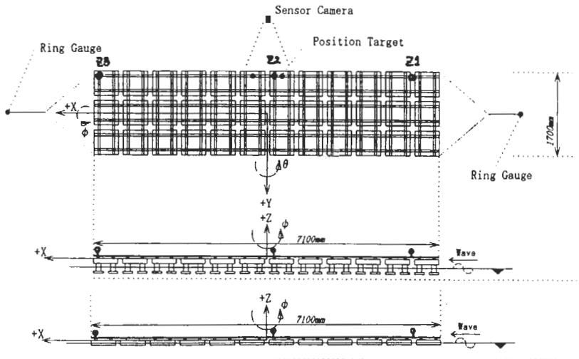
Figure 1: Very large floating models (upper: plan view, middle: side view of semi-sub, lower: side view of pontoon) moored by linear springs
