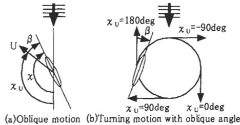
Figure 3: Definition of  $\chi_U$  in oblique and turning motion
