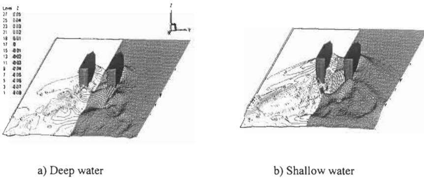
Figure 9: Free surface deformation around CATA III at the design speed for shallow and deep water conditions ( $S/L = 0.26$ ,  $Fn = 0.750$ )
