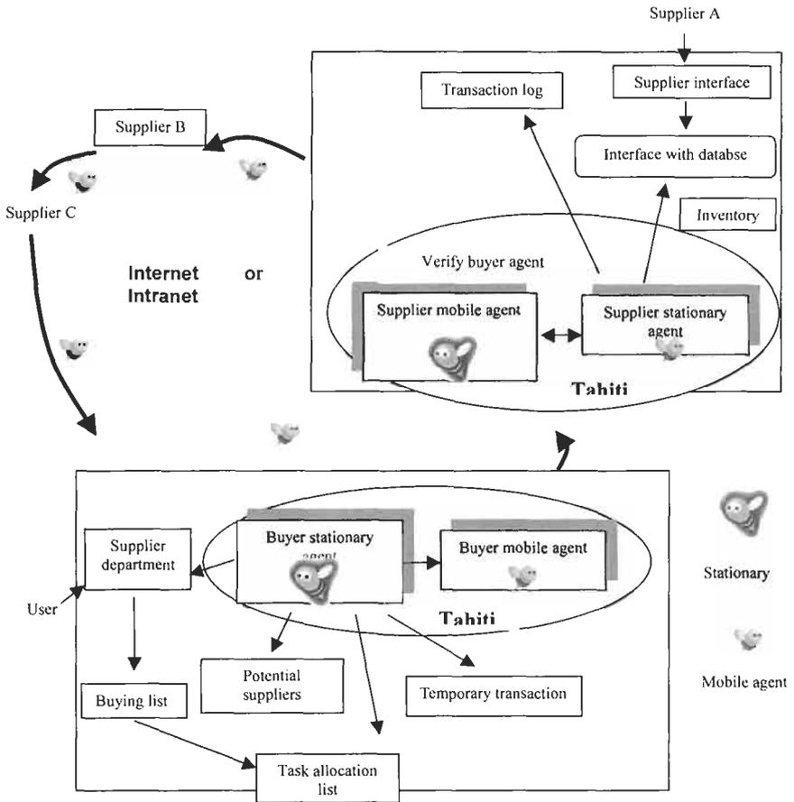
Figure3: The Architecture of Mobile Based SCM
