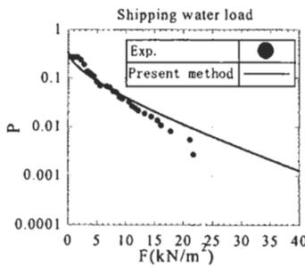
Figure 4 : Comparison between measured and estimated exceedance of probability of shipping water load (  $\chi = 180^\circ$  ,  $T = 1.459\text{sec}$ ,  $H_{1/3} = 0.174\text{m}$ ,  $F_N = 0.1$ )
