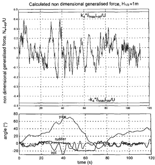
Figure 2: Calculated non dimensional generalised force for the patrol craft HMS Sandhamn at a significant wave height of approximately 1m,  $F_n \approx 0.4$  (during the first 40 seconds).
