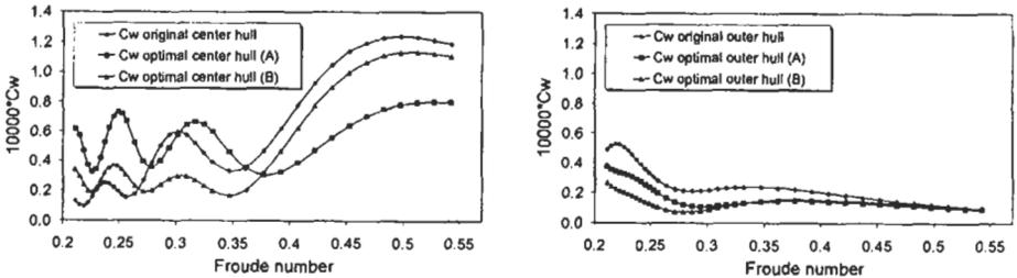
Figure 3: Wave drag coefficient for original and optimal hulls
