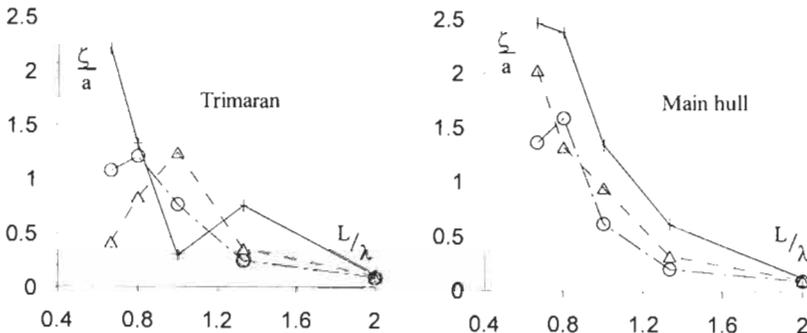
Figure 6: Heave response amplitude operators. Cross:  $F_n=0.45$ ; triangle:  $F_n=0.63$ , circle:  $F_n=0.82$
