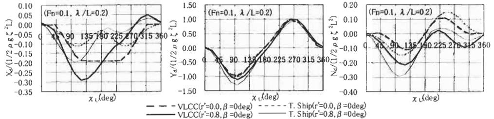
Figure 7: Comparison of steady wave forces for a VLCC and a training ship in turning motion
