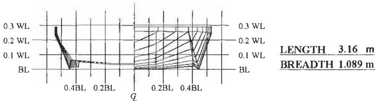
Figure 5: Body plan of the test boat for applications of air lubrication
