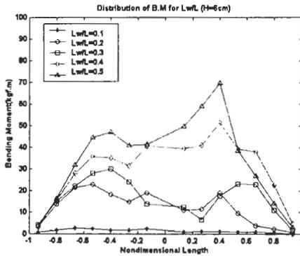
Figure 8 : The Longitudinal distribution of bending moments (h=0.4m, H=6cm, Incident Angle=30 degree)
