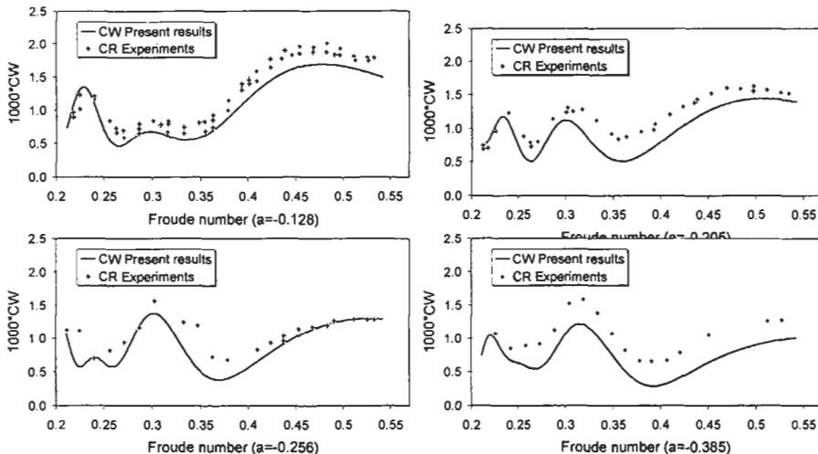
Figure 1: Calculated wave drag and experimental residuary drag
