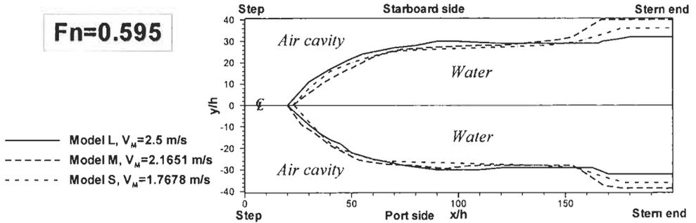
Figure 3: Air cavity shapes formed behind the step under the bottom of each model at  $Fn = 0.595$
