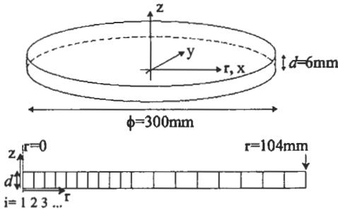
Figure 6: Computational grid used in inverse heat conduction analysis
