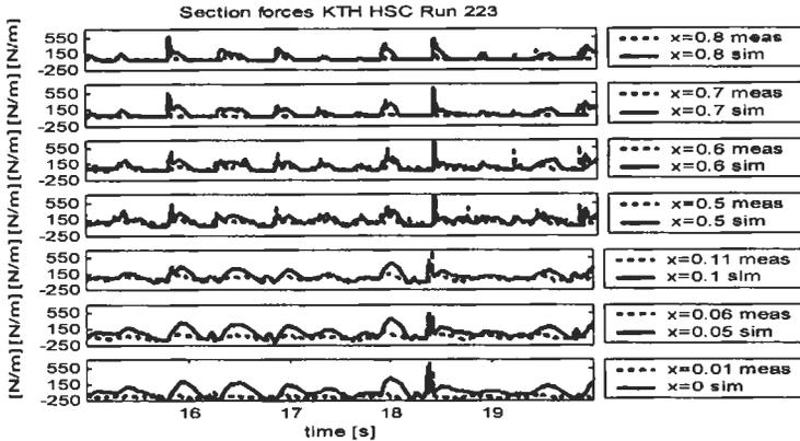
Figure 7: The simulated section forces are plotted together with a section-wise integration of the pressure measurement. Notice the slamming load along the hull. The load fluctuations at the aftmost sections are too pronounced in the simulation.
