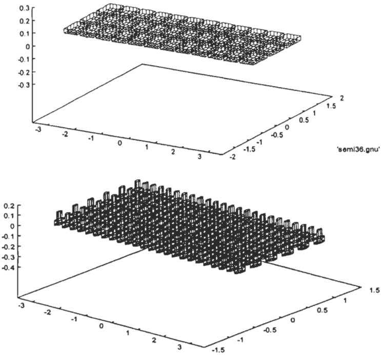
Figure 2: Discretization of models (upper: pontoon lower: semi-sub) for hydrodynamic analyses
