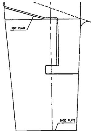
Figure 5: The profile of the high lift rudder
