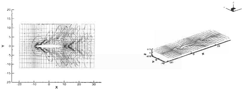
Figure 4: the mesh of the free surface,  $Fn=0.316$ ,  $t=20$  sec, (Wigley ship model)
