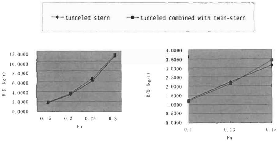
Figure 3: R/D ~Fn curves in deep water
