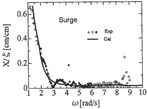
Figure 3: Amplitude of surge motion of pontoon type VLFS in regular waves
