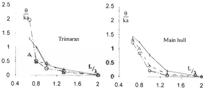
Figure 7: Pitch response amplitude operators. Cross:  $F_n=0.45$ ; triangle:  $F_n=0.63$ , circle:  $F_n=0.82$
