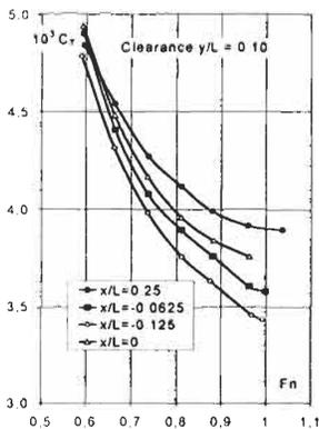
Figure 3: Resistance results for different staggers
