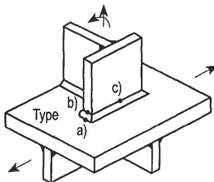
Figure 1: Types of Hot Spots in Welded Structures (From Fricke, 2001)
