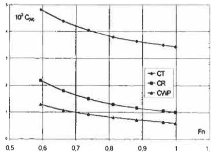
Figure 3: Main hull:  $C_T, C_R, C_{WP}$  versus  $F_n$
