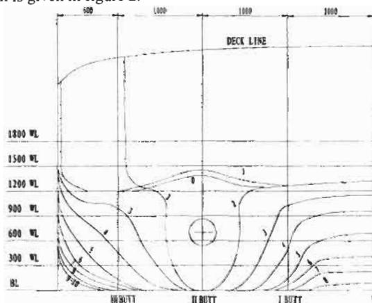
Figure2: Afterbody plan of tunneled combined with twin-stern
