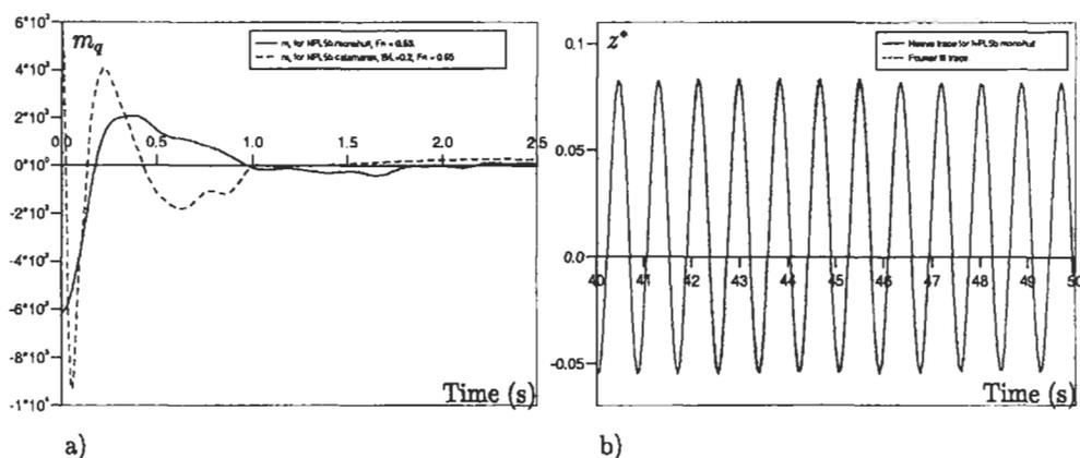
Figure 1: (a) Pitch-pitch ( $m_q$ ) impulse response functions for mono-hull and catamaran configurations and (b) heave response trace for mono-hull,  $F_n = 0.53$ , Heading = 180deg,  $\alpha = 0.05625m$ ,  $\omega_e' = 5.42$
