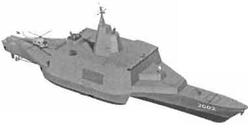
Figure 1: Graphic design model of trimaran
