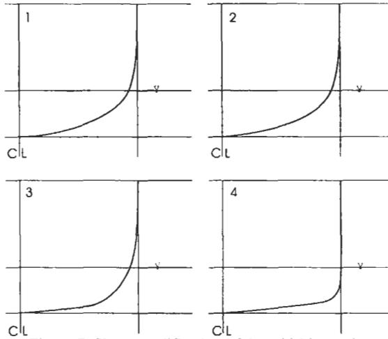
Figure 7: Shape modification of the midship section
