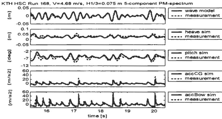
Figure 4: Simulated and measured time series. Quantities are in model scale.
