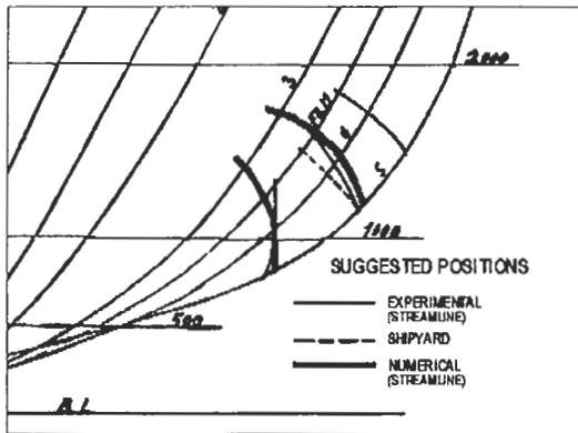
Figure 5: Positioning of Bilge Keels
