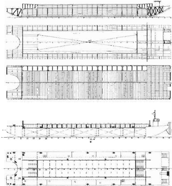
Figure 4: The structure and the general arrangement of the rebuilding barge
