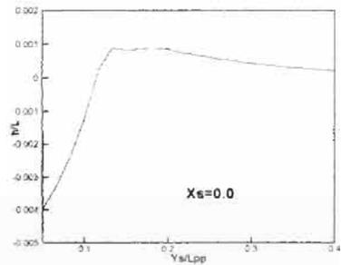
Figure 12: Wave height generated by main hull in transverse direction (30 knots)
