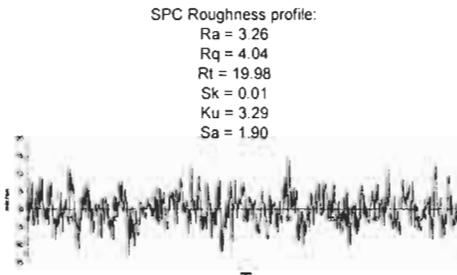
Figure 2: Typical profile of the SPC surface
