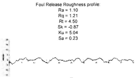
Figure 3: Typical profile of the Foul Release surface
