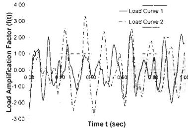
Figure 2b: Two Loading Curves Generated from the Gaussian-Stationary Random Process
