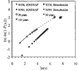
Figure 8: Long-term extremes of stress for deck plate with return period: 20, 50, 100 years
