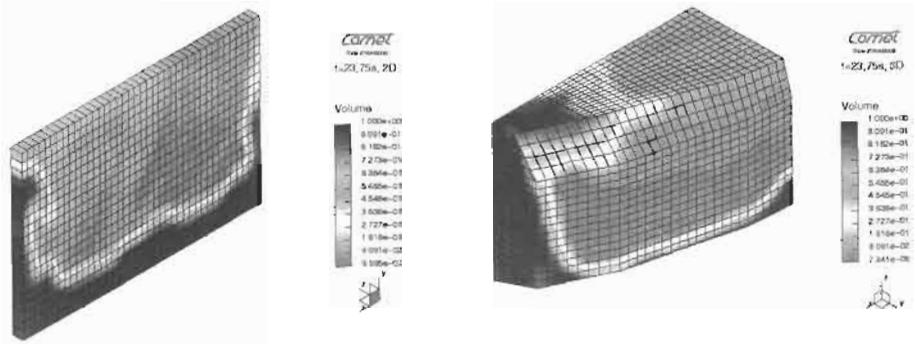
Figure 6: Comparison of computed free surface deformations for 2D model (left) and 3D model (right).
