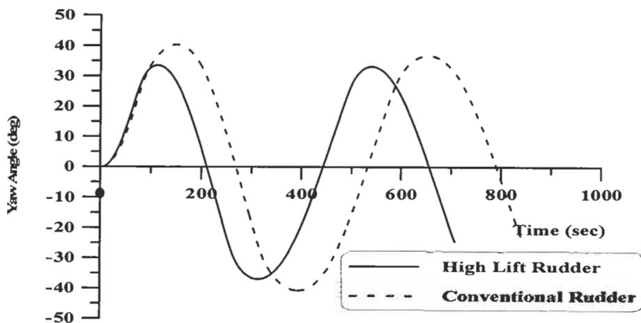
Figure 4: The  $20^{\circ}/20^{\circ}$  zig-zag characteristics for two rudders of 2.3% area
