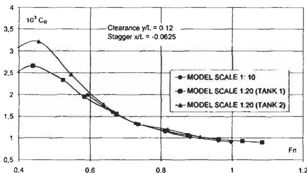
Figure 8: Comparison between geosims results – ITTC-57 correlation
