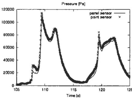
Figure 4: Computed time traces of pressure for a point sensor and for a panel.
