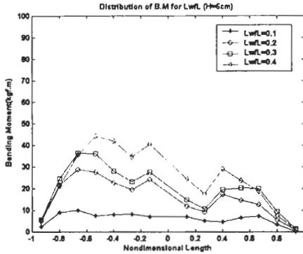
Figure 7 : The Longitudinal distribution of bending moments (h=0.4m, H=6cm, Incident Angle=0 degree)
