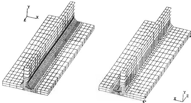
Figure 1: Mesh topology employed for general models.
