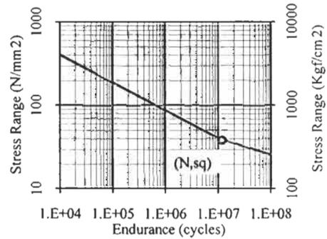
Figure 10: A typical two-segment S-N curve,  $N = KS^{-m}$ :  $(N, S_q) = (10^7, 39.8\text{N/mm}^2)$ ,  $(m', K') = (5, 9.975 \times 10^{14}), (m, K) = (3, 0.315 \times 10^{11})$
