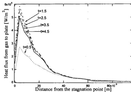
Figure 10: Estimated heat flux obtained by inverse heat conducting analysis
