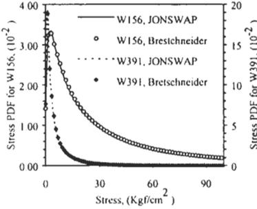
Figure 7: Long-term probability density function  $p(x)$  of stress responses for deck plate
