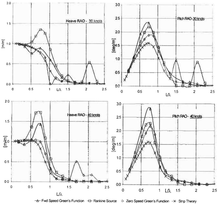
Figure 3: Heave and Pitch RAO for a fast monohull at 30 knots and 40 knots
