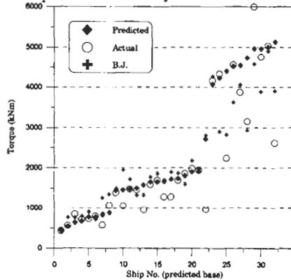
Figure 3: Plot of steering gear torques for regression model, present method and sea-trial results
