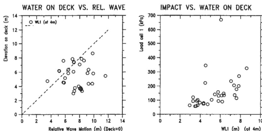
Figure 6: Correlation between relative wave, water on deck and impact load.
