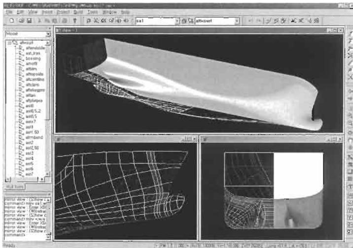
Figure 5: Shaded surface model of a twin skeg hull form produced from the wireframe model in EzHULL
