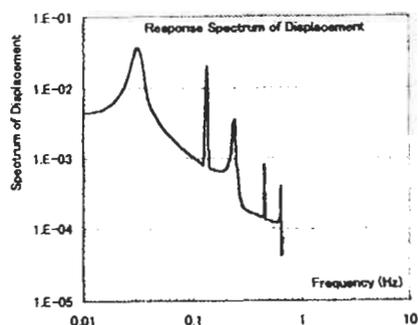
Figure 11: Power spectral density of deflection for a selected point on main structure
