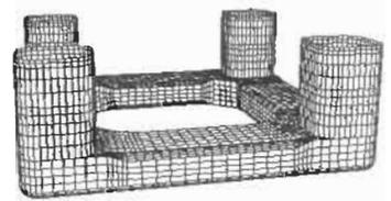
Figure 6: Panel method for the floater used in the case study.
