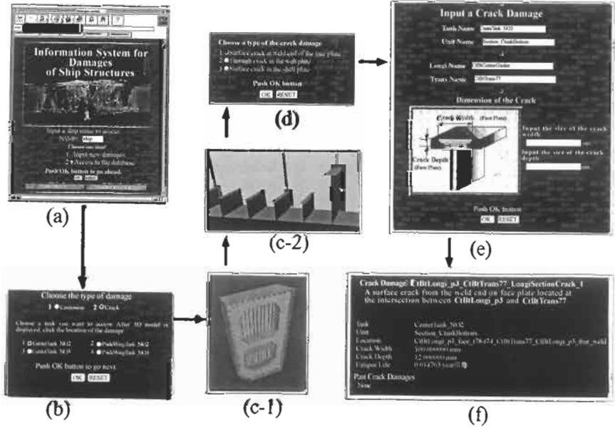
Figure 4: Input and evaluation process in the developed proto-type system
