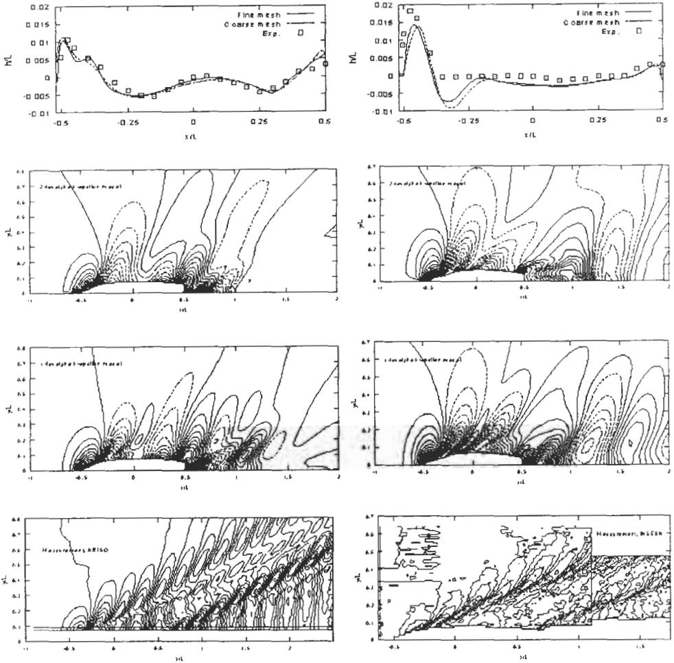
Figure 3: Effect of two grid levels on the waves. Left: the KCS model; right: the DTMB 5415 model. Solid lines for crests; dashed lines for trough; levels: 0.0005
