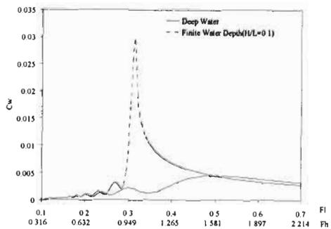
Figure 2: Wave resistance coefficient in deep water and finite water depth
