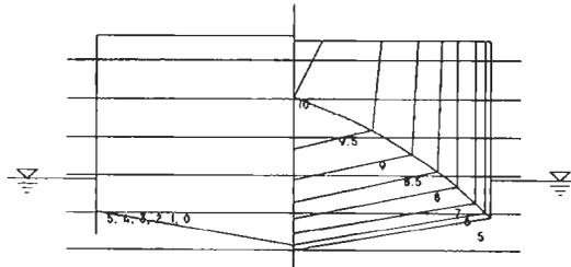
Figure 1: Body plan of geometrically similar model ships
