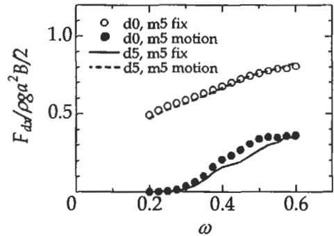
Figures 8: Steady wave drift forces on the model in 0 degrees wave
