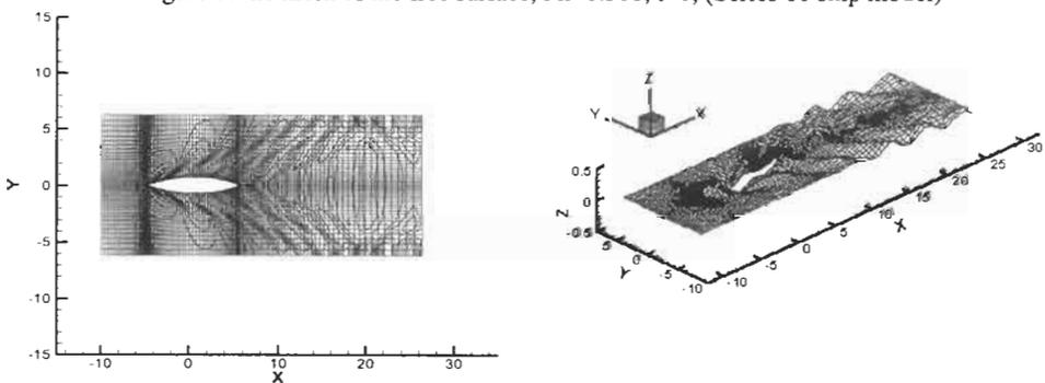
Figure 6: the wave of free surface in acceleration,  $Fn=0.316$ ,  $t=35$  sec, (Series 60 ship model)
