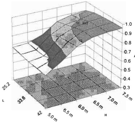
Figure 5: Attained Index A as a function of length L of machinery space and height H from tank top to main deck. SLF 43/3/2
