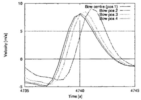
Figure 7: Boundary conditions for water flow deck: Freeboard exceedance at bulwark (ref. Figure 2)
