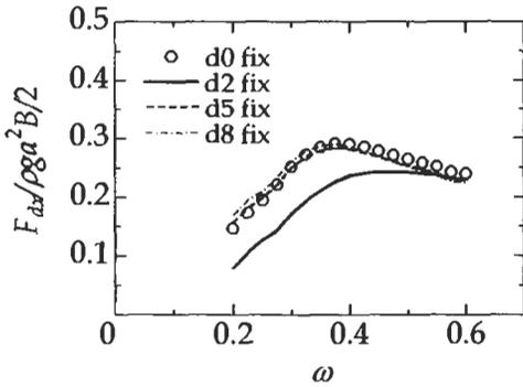
Figures 9: Steady wave drift forces of surge on fixed body in 60 degrees wave (effect of draft)
