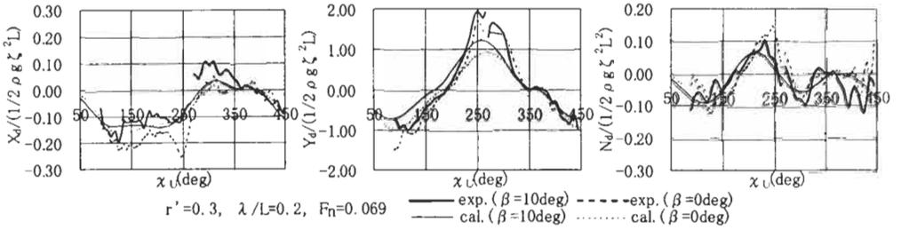
Figure 5: Steady wave forces and moment in turning motion, experiment and calculation for a VLCC
