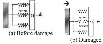
Figure 7: Change of model when fender was damaged
