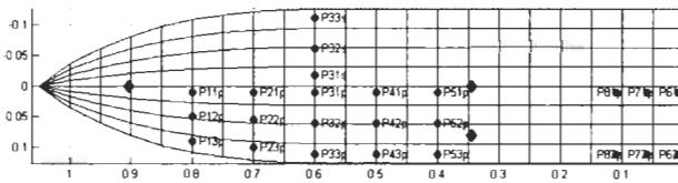
Figure 1: Test set-up and pressure transducer and accelerometer location. At all tests 20 transducers were in use. The transducers at position P51-3 were moved to position P11-P13 for all runs in waves.
