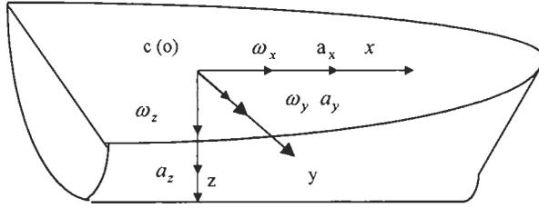
Figure 1: Definitions and the coordinate system
