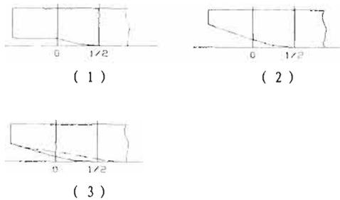
(1) prototype (2) simply cutting stern (3) tunnel cutting stern
