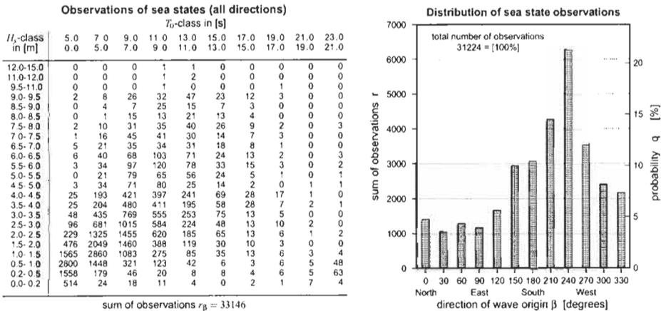
Figure 1. Long-term wave statistic of the Eastern Atlantic Ocean (Hogben and Lumb, 1967). Wave scatter diagram (left) and directional breakdown of occurrence of sea states (right).
