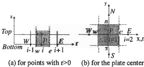
Figure 7: Control volumes used in the inverse heat conduction analysis
