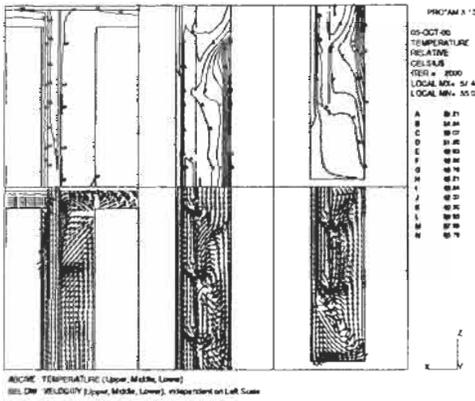
Figure 4 : Flow and temperature in original system (Cascade)
