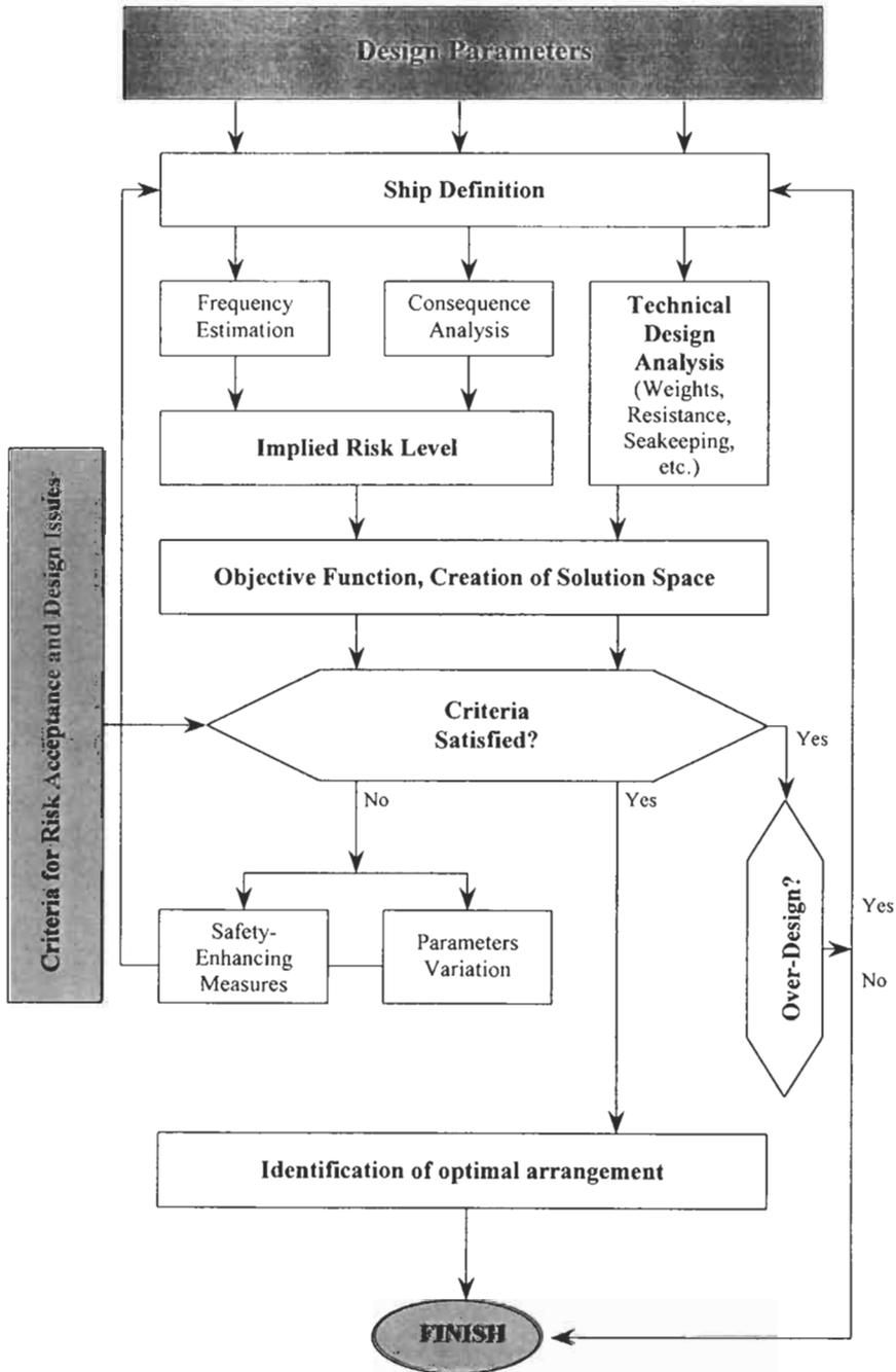
Figure 2: A QRA-Based Design Procedure (Single Risk DFX)
