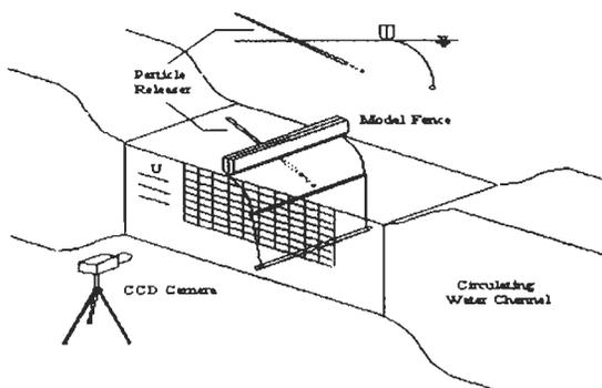
Figure 2a: Experimental setup for measuring the trajectory of paraffin balls
