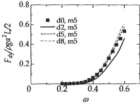
Figures 12: Steady wave drift forces of sway on body with elastic motion in 60 degrees wave (mass corresponds to 5m in draft, effect of draft)
