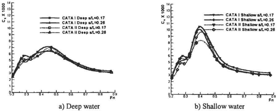
Figure 5: Comparison of residuary resistances of CATA I and II (demi-hull spacing  $S/L = 0.17, 0.26$ )
