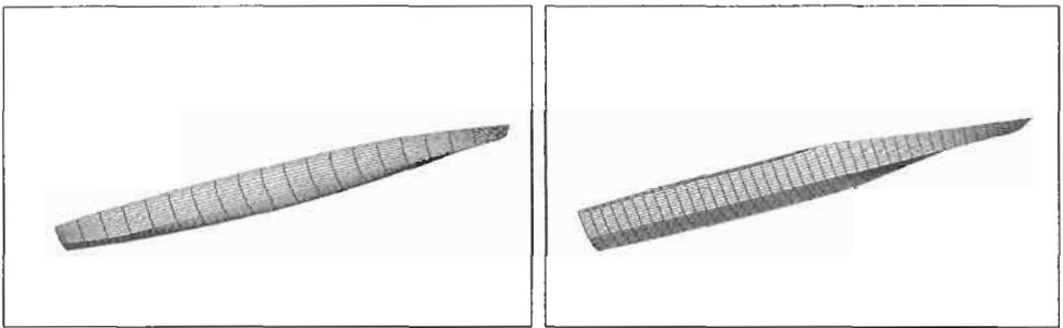
Figure 1: View of the grids for modelling the frigate hull (left) and the fast ferry hull (right)
