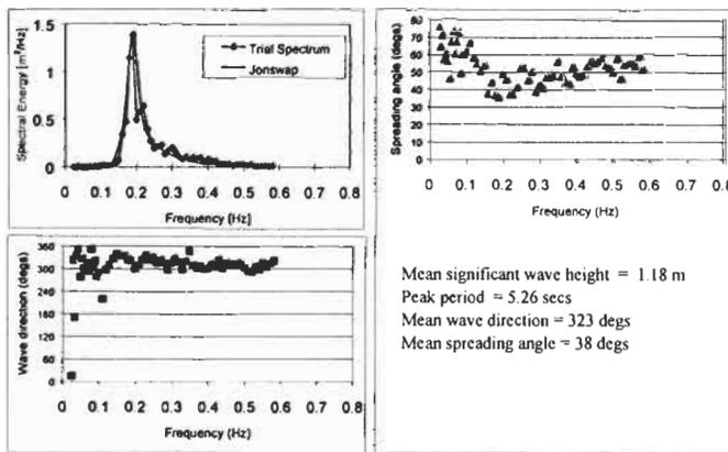
Figure 4. Average wave parameters
