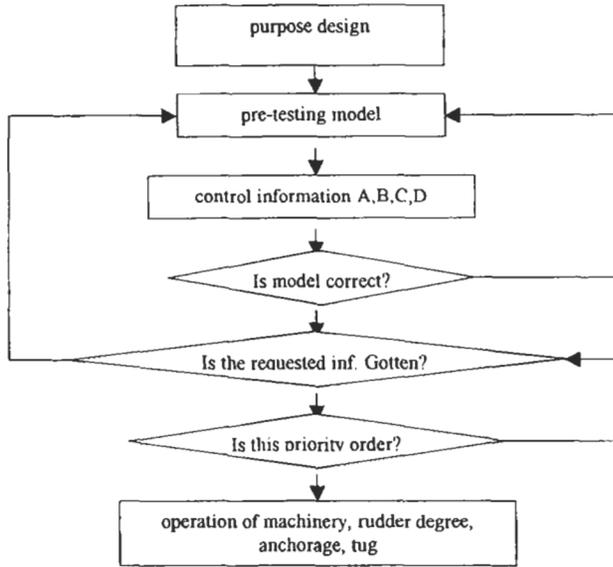
Figure 4: Check for information and control for overall procedure of navigation
