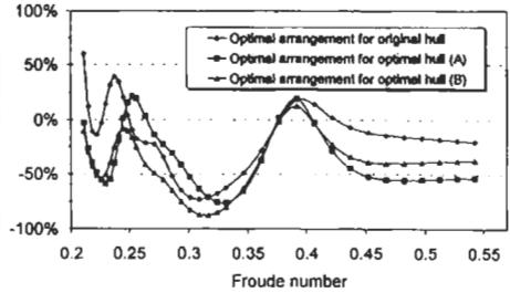
Figure 6: Wave drag reduction for different optimal hull arrangements
