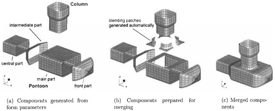
Figure 4. Shape generation process
