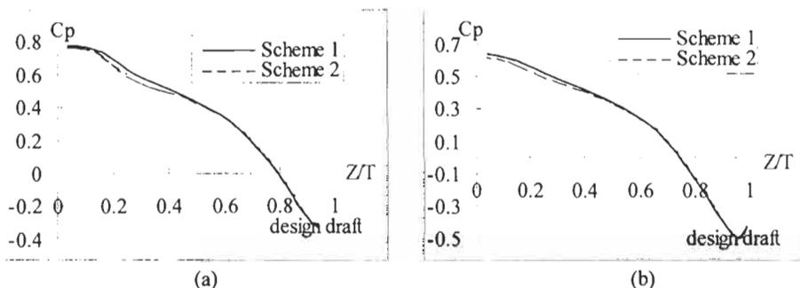
Figure 1: Distribution of  $C_p$  along Z-axis at 19-station (a) and 19 2/3-station (b)
