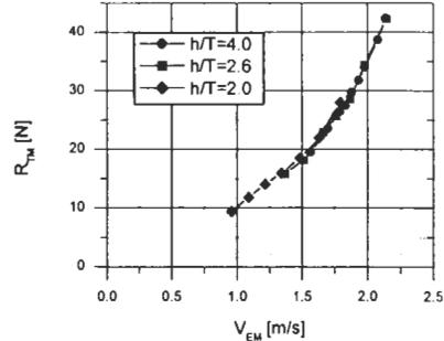
Figure 4: Total model resistance as a function of the effective speed for the subject container ship
