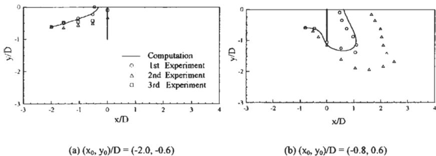
Figure 5: Trajectories of paraffin balls around the vertical model fence for different initial release points at  $Fr = 0.29$ ,  $Re = 53100$
