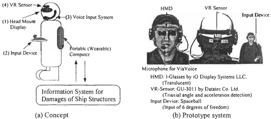
Figure 5: Inspection style with the proposed ship inspection supporting system
