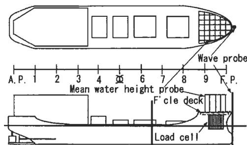
Figure 2 : Setup of measuring instruments
