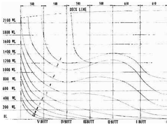
Figure 1: Afterbody plan of tunneled stern
