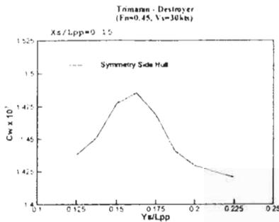
Figure 11: Calculated  $C_W$  curve according to the transverse locations of side-hull
