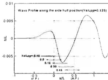
Figure 13: Relation between wave profile and side-hull location (30 knots)
