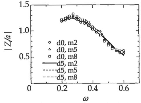
Figure 4: Vertical displacements in 0 degrees wave; effect of the zero-draft and mass
