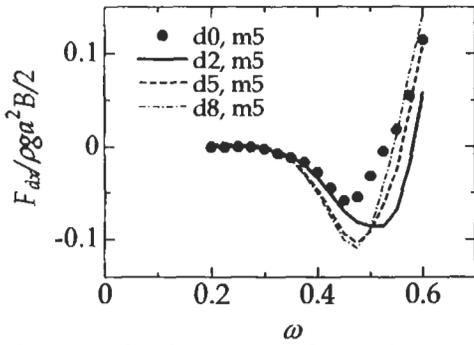
Figures 11: Steady wave drift forces of surge on body with elastic motion in 60 degrees wave (mass corresponds to 5m in draft, effect of draft)
