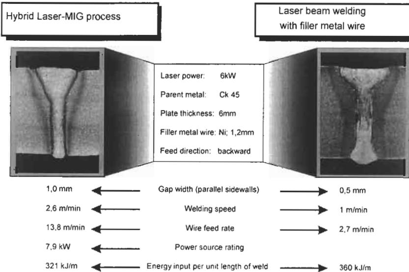
Figure 6: Comparison of Hybrid Welding with Laser Welding
