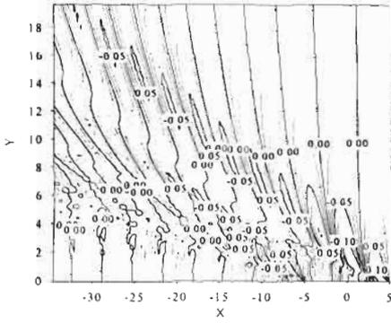
Figure 9: Predicted wash for  $F_h=0.9$ . The ship is located at  $-5 < x < 5$  and  $H/L = 0.1$ . The numbers associated with the different lines are wave elevation divided by water depth.
