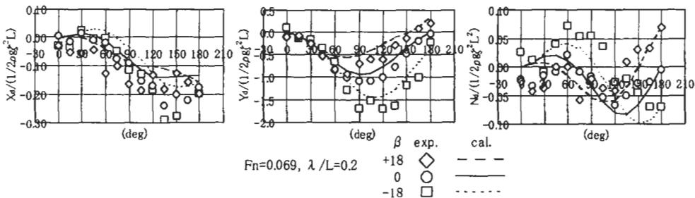
Figure 4: Steady wave forces and moment in oblique motion, experiment and calculation for a VLCC
