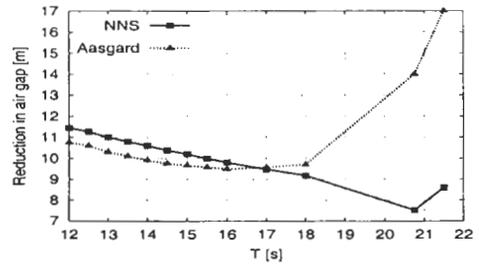
Figure 8: Reduction of air gap for platform in regular waves relative to the air gap in still water.
