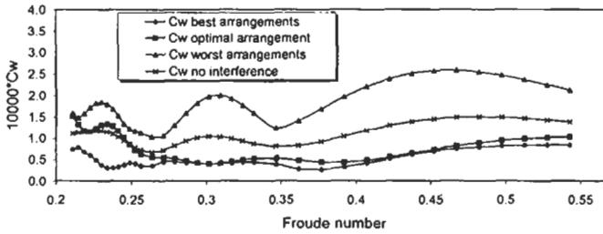
Figure 2: Wave drag coefficient for different hull arrangements
