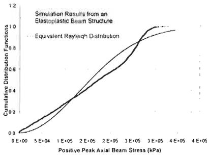
Figure 3a: Statistical Distribution of Positive Peak Values for the Elastoplastic Beam Model
