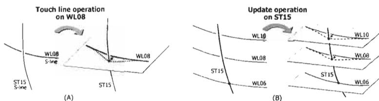
Figure 2: Example of the ‘touch line’ operation (A) and the ‘update line’ operation (B) on station line
