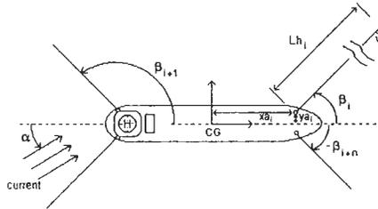
Figure 1: Geometric definition of the mooring system
