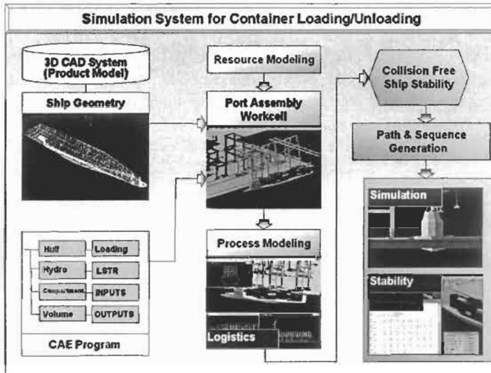
Figure 7. Procedures of Simulation for Container Loading/Unloading
