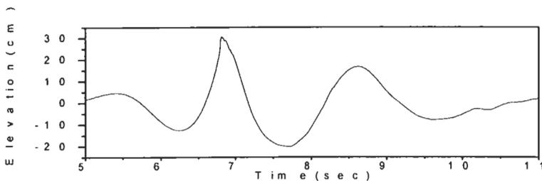
Figure 4: Time history of wave elevation
