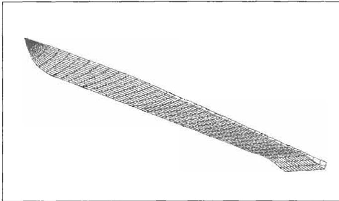
Figure 2: ITTC Model Panelization
