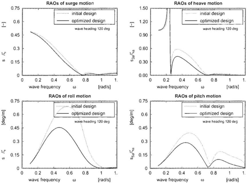
Figure 7. Comparison of motion behaviour of initial and optimized semisubmersible.
