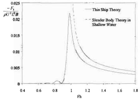
Figure 8: Pitch moment  $F_3$  by thin ship theory and the shallow water slender body theory by Tuck (1966) ( $H/L=0.1$ )
