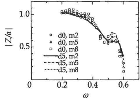
Figures 6: Vertical displacements in 60 degrees wave; zero draft and 5m in draft, (mass effect)
