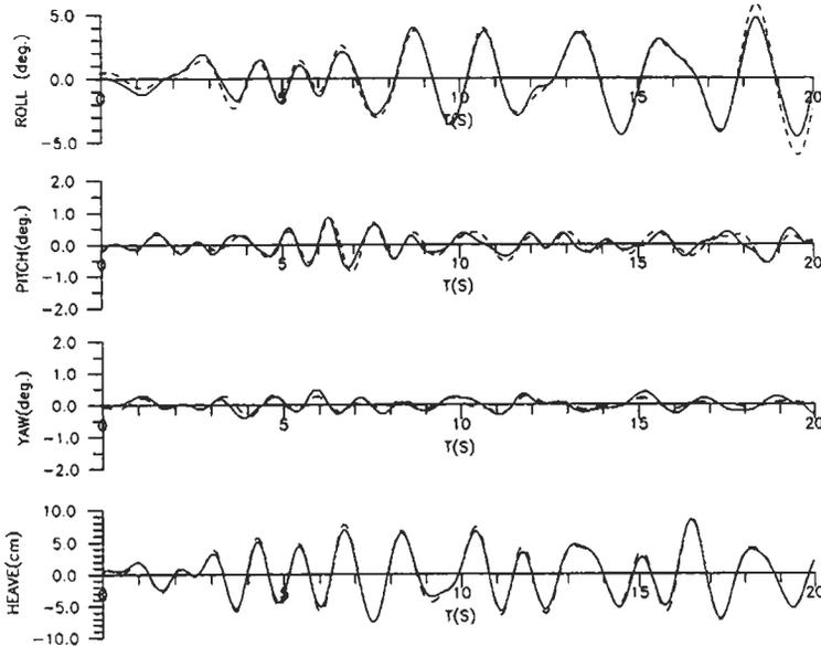
Figure 5: Motions of a container vessel model measured by two system
