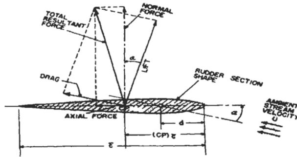
Figure 1: Definitions of rudder forces and its geometry
