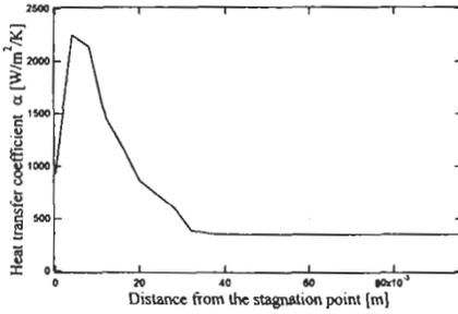
Figure 12: Estimated distribution of local heat transfer coefficient
