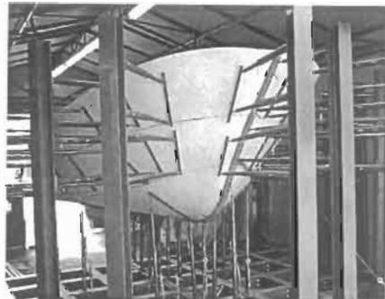
Figure 11: Bow shape supported by line elements
