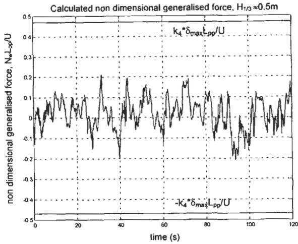
Figure 1: Calculated non dimensional generalised force for the patrol craft HMS Sandhamn at a significant wave height of approximately 0.5m,  $F_n \approx 0.4$ .
