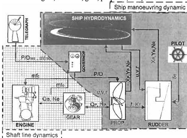
Figure 1: Ship propulsion model functional scheme
