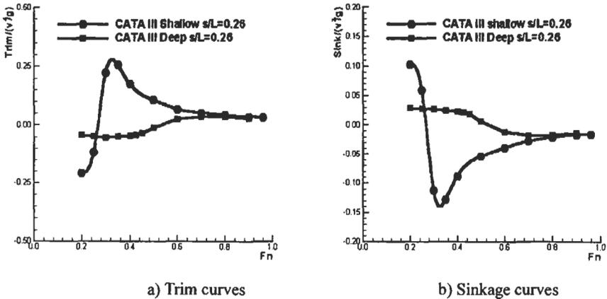
Figure 11: Hull attitudes of CATA III for shallow and deep water ( $S/L = 0.26$ )
