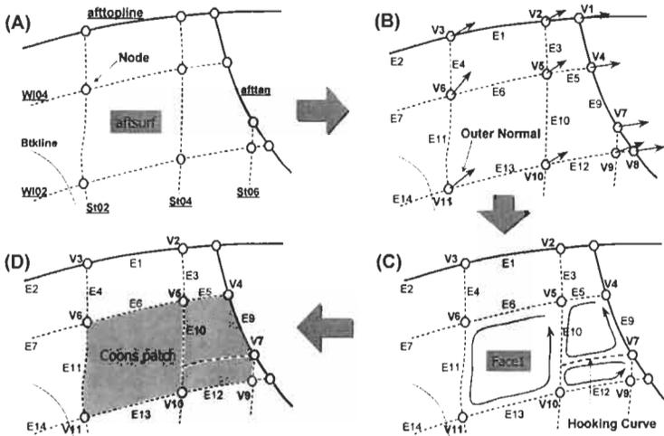
Figure 4: Procedure for generating the non-manifold data structure of the surface model from the X-topology of the wireframe model
