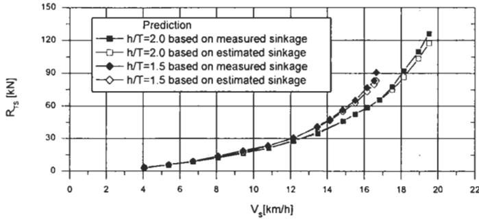
Figure 7: Comparison of the predicted ship-resistance using measured and empirically estimated sinkage
