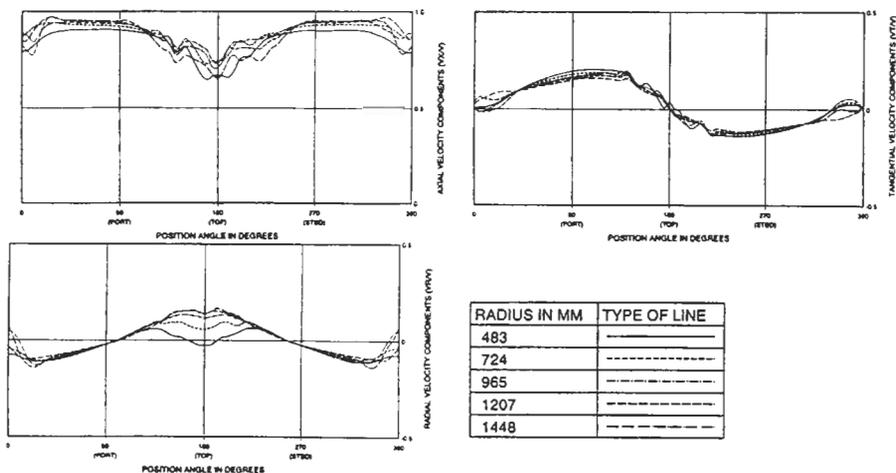
Figure 2: Result of the wake survey
