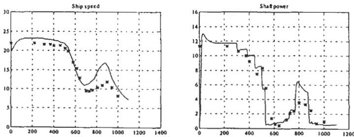
Figure 2: Coasting manoeuvre comparison
