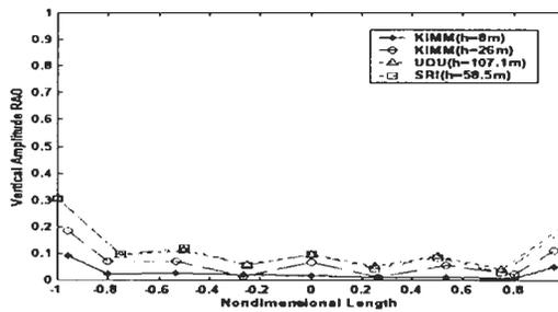
Figure 4 : The Vertical Displacement RAO( $\lambda_w / L = 0.1$ , Incident Angle=0 degree)
