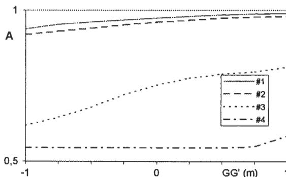
Figure 3: Variation of the Attained Index  $A$  with change in the vertical position  $GG'$  of the centre of gravity. SOLAS Part B-1
