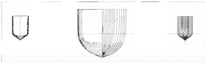
Figure 1: Trimaran hulls body plan
