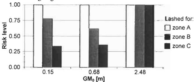
Figure 2: Risk of cargo shifting as a function of  $GM_0$  (route in zone B, at a speed of 15 knots)
