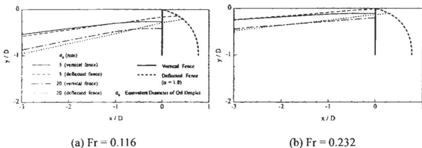
Figure 4: Leakage lines of vertical fence and deflected fence for different oil droplet diameters and current speeds
