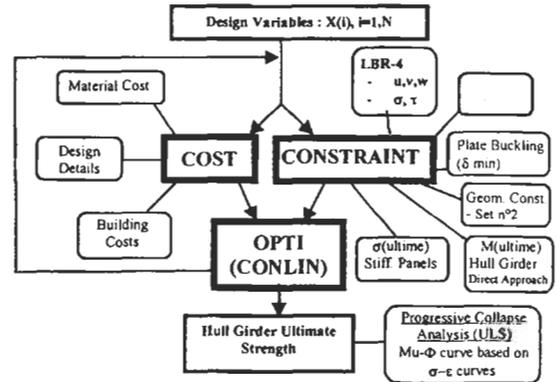
Figure 1: LBR-5 flow chart including some available sub-modules (constraints and cost data).
