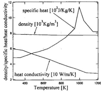
Figure 8: Temperature dependency of the material properties used in inverse heat conduction analysis
