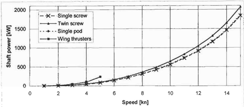
Figure 1: Shaft power of the four investigated concepts.
