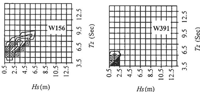
Figure 1: Graphic comparison of Wave Scatter Diagrams for two locations (W156: A site in the North Sea ; W391: A site in the Gulf of Mexico)
