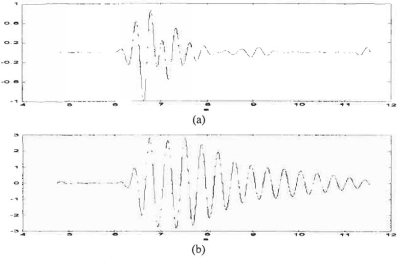
Figure 10: Wavelet spectrum of wave elevation at  $b=0.25$ (a), wavelet spectrum of force at  $b=0.25$ (b)
