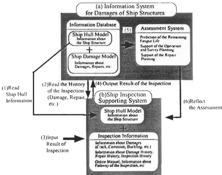
Figure 1: Concept of an information system for damages of ship structures
