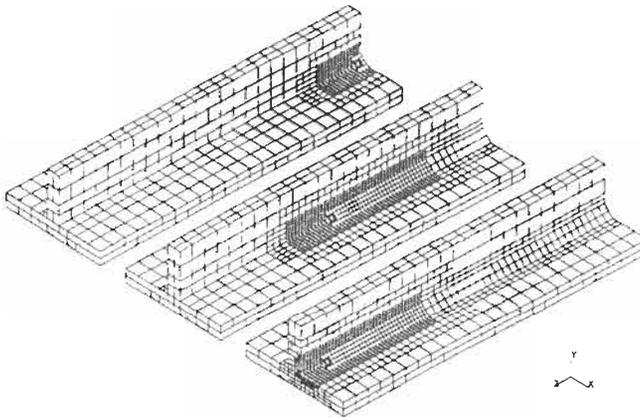
Figure 2: *Examples of meshes in dynamic meshing.*
