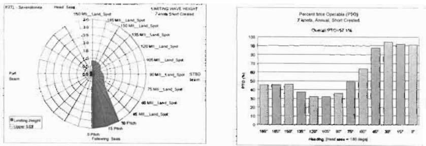
Figure 6: Limiting significant wave height and PTO of the RTTL at Sevenstones
