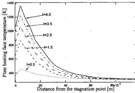
Figure 9: Estimated plate heating face temperature obtained by inverse heat conducting analysis
