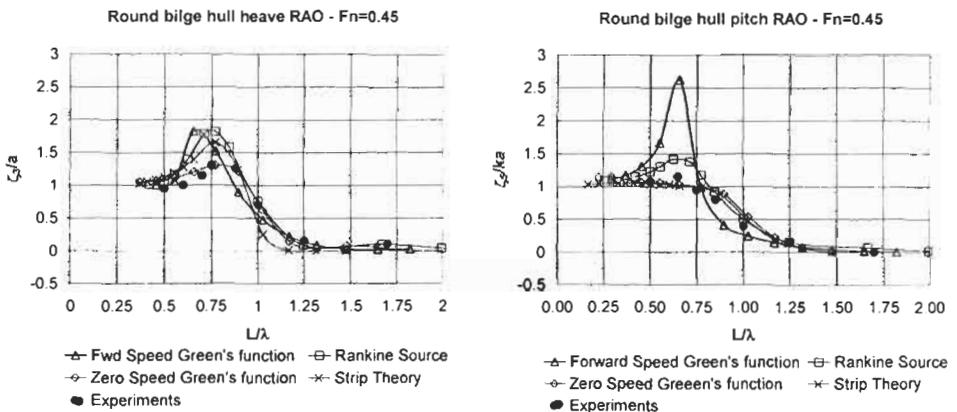
Figure 2: Heave and Pitch RAO for a round bilge frigate hull at  $F_n=0.45$
