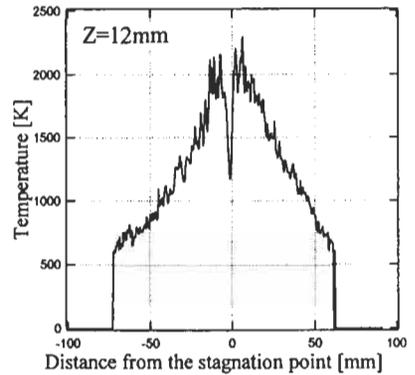
**Figure 4:** Measured gas temperature distribution on the plane 1.5mm upward from the plate surface for the case where Z=12mm
