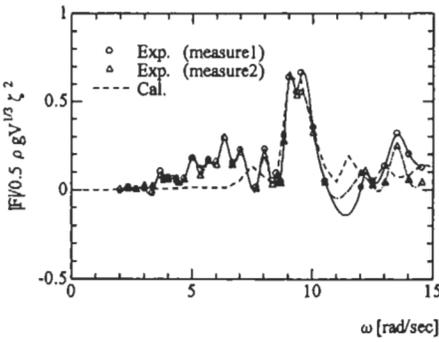
Figure 6: Wave drift force components of rigid semi-submersible type floating structure
