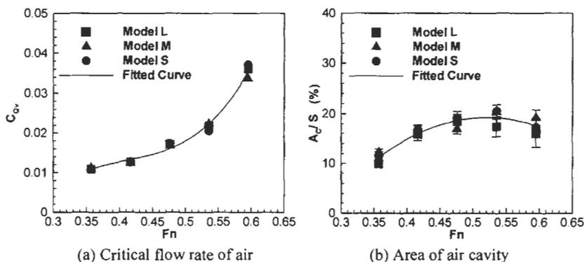
Figure 2: Critical flow rate of air and area of air cavity dependent on Froude number
