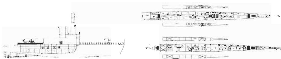
Figure 1: General Layouts of 160 m trimaran frigate
