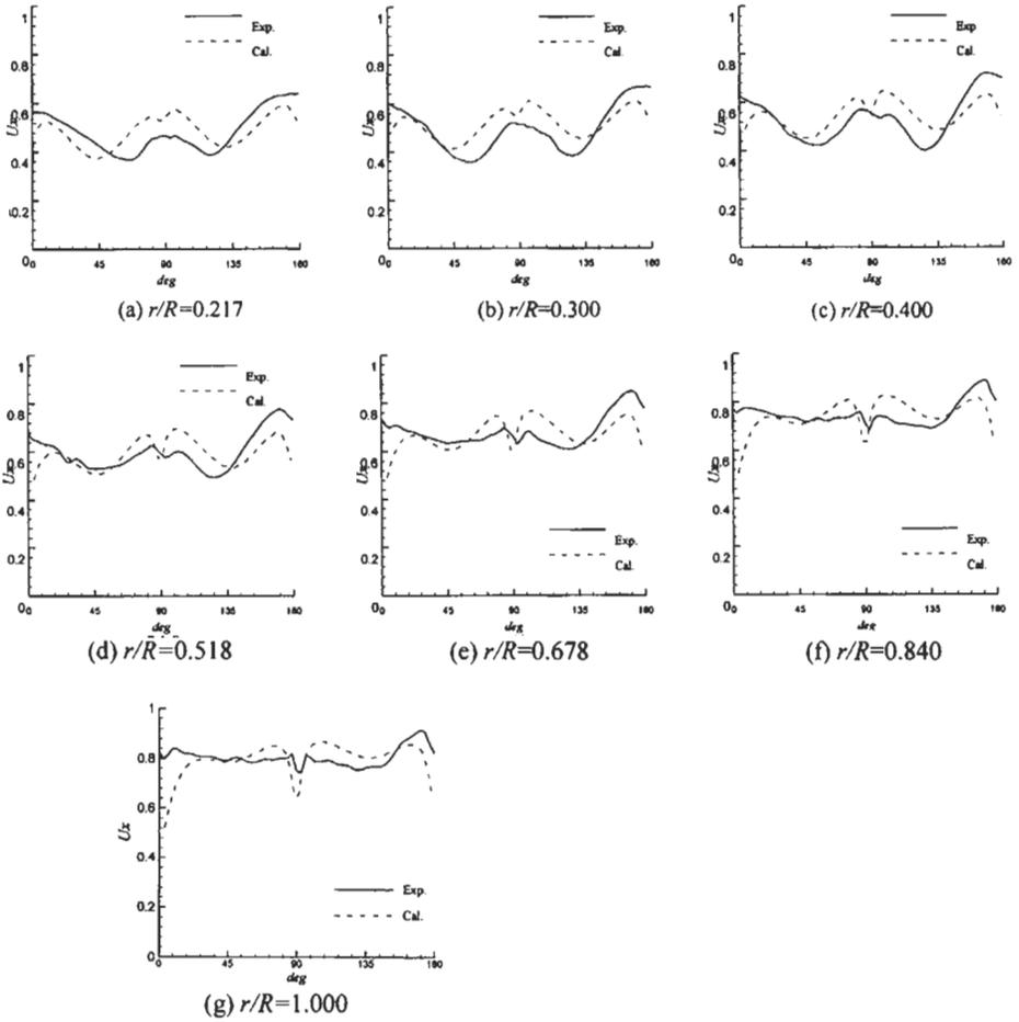
Figure 2: Circumferential variation of axial velocity at different radius station of propeller
