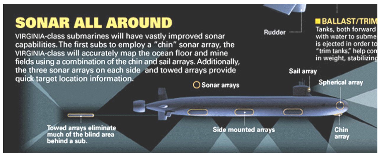
Figure 10 - Overall sonar system [navsource.org]
