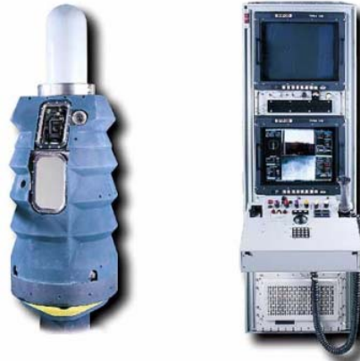
Figure 15 - Kollmorgen PMP and Control Center [Kollmorgen]
