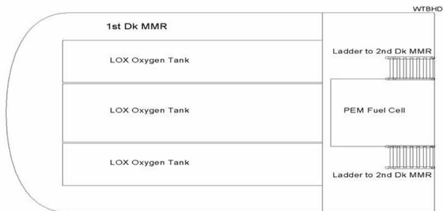
Figure 76 - MMR Deck one equipment layout
